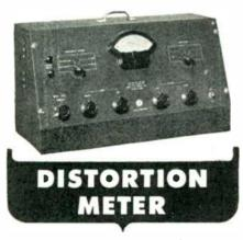
Direct reading device which indicates as a percentage of the fundamental frequency, the square root of the sum of the squares of the harmonic components. It is used for audio frequency measurements in any audio device in the usual range of voice or musical notes from 150 to 15,000 cycles.
