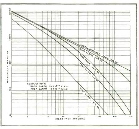
FIG 5. AM FIELD STRENGTH AS A FUNCTION OF DISTANCE AT 550 AND 1470 KC.
