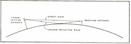
FIG. 7. TRANSMISSION AT VERY HIGH FREQUENCIES IS EFFECTED BY MEANS OF BOTH GROUND-REFLECTED WAVES AND DIRECT WAVES, AS THIS DRAWING SHOWS
