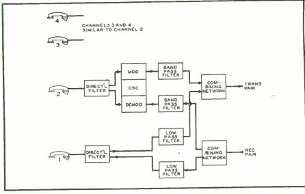
FIG. 2. HOW FOUR CONVERSATIONS ARE PUT ON A SPIRAL-FOUR CABLE
