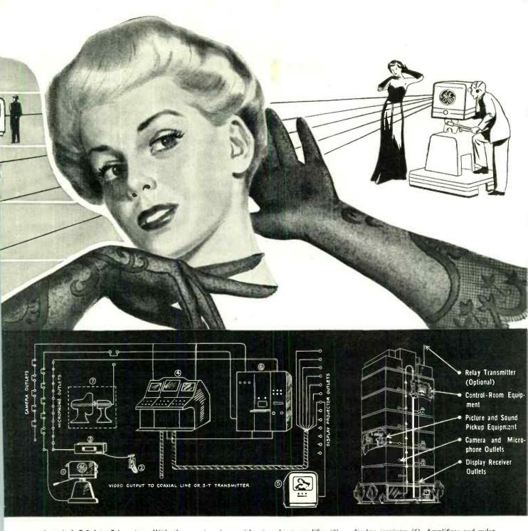
A typical G-E Intra-Tel system. With the Intra-Tel system, portable television cameras and sound microphones can be operated from any place in store or plant. Pictures and sound picked up by cameras (1) and microphone with microphone amplifier (2)and (3) are fed by cable to the control and monitoring console (4). Outlets at the console make it possible to feed picture and sound signals by cable to any number of
