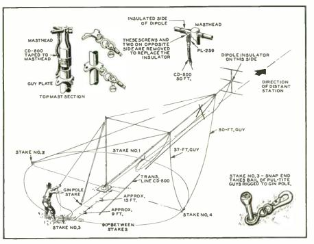
FIG. 13. DETAILS OF THE ANTENNA, AND THE METHOD BY WHICH IT IS ERECTED
