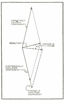
FIG. 8. HOW MODULATION IS ACCOMPLISHED
