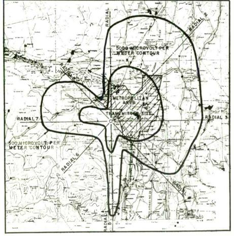
FIG. 33. CALCULATED 500- AND 5,000-MICROVOLT CONTOURS OF TELEVISION STATION WRGB
