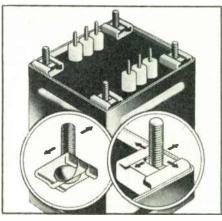
FIG. 10. IMPROVED MOUNTING STUDS
