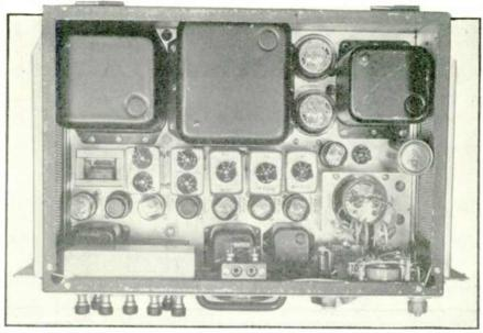
FIG. 5. INTERIOR OF THE 50-WATT TRANSMITTER SHOWS SIMPLE DESIGN
