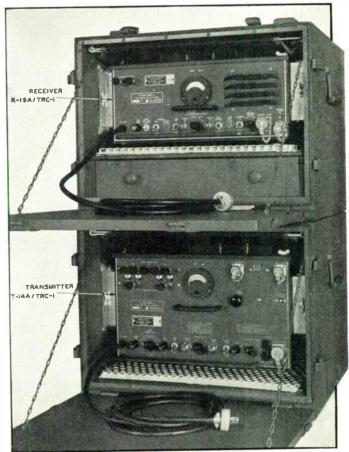
FIG. 3. COMPLETE FM CARRIER TRANSMITTER AND RECEIVER
