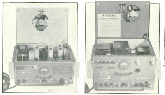
FIG. 4. THE RECEIVER, LEFT, AND THE TRANSMITTER, RIGHT, REMOVED FROM THE CARRYING CASES SHOWN IN FIG. 3
