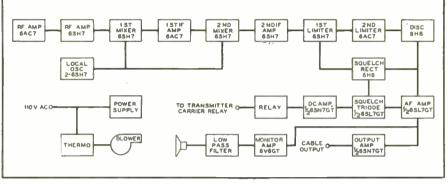
FIG. 10. BLOCK DIAGRAM SHOWING THE RECEIVER TUBE TYPES AND FUNCTIONS
