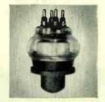
The ML 880 is a radio oscillator tube for use in transmitters, and has a maximum output of 60KW.
