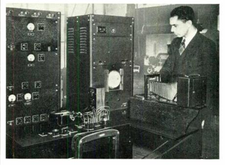
The measurement of tube characteristics in regions where previous test methods were inapplicable has been made possible through the development, by Sylvania Electric, of a new procedure, based on photographing an oscillographic trace.
