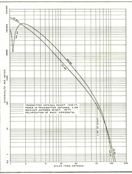
FIG. 8. FIELD STRENGTH AS A FUNCTION OF DISTANCE AT VERY HIGH FREQUENCIES
