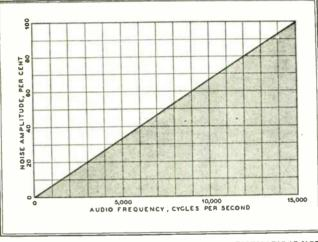
FIG. 10. FM RECEIVER OUTPUT NOISE WHEN DE-EMPHASIS IS NOT EMPLOYED
