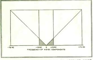
FIG. 7. SPECTRUM DISTRIBUTION OF FM RECEIVER NOISE, INDICATED BY THE SHADED AREA
