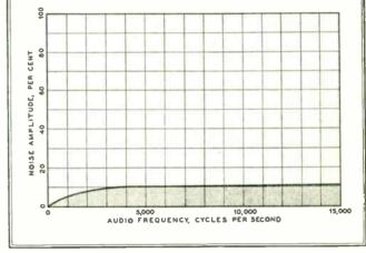
FIG. 11. REDUCTION OF NOISE INDICATED IN FIG. 10 WHEN DE-EMPHASIS IS EMPLOYED
