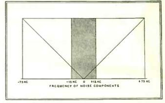
FIG. 8. SPECTRUM DISTRIBUTION OF AM RECEIVER NOISE, INDICATED BY SHADED AREA
