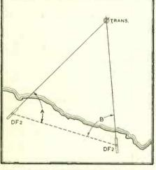
FIG. 1. STANDARD METHOD FOR LOCATING A DISTANT TRANSMITTER
