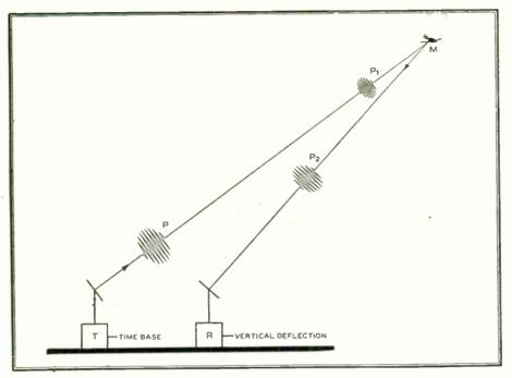
FIG. 3. RADIO PULSES FROM T ARE REFLECTED BY TARGET M TO RECEIVER R
