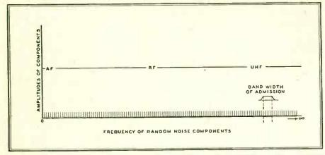
FIG. 4. APPROXIMATE REPRESENTATION OF SPECTRUM DISTRIBUTION OF RANDOM NOISE
