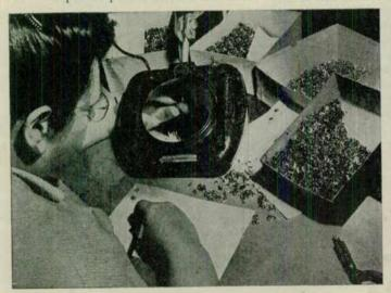
By a sampling method, watchful Sylvania inspectors carefully study each batch of small parts for detailed perfection. To insure that all Sylvania-made radio tubes will be of the very best quality, the well equipped tube plant in Emporium, Pennsylvania, provides extensive facilities for making over 8500 of the delicate small parts that go into Sylvania tubes.
