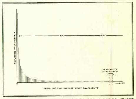
FIG. 5. APPROXIMATE REPRESENTATION OF SPECTRUM DISTRIBUTION OF IMPULSE NOISE
