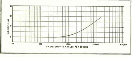
FIG. 9. STANDARD PRE-EMPHASIS CHARACTERISTIC FOR FM TRANSMITTERS
