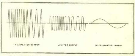
FIG. 3. WAVE FORMS OF LIMITER AND DISCRIMINATOR VOLTAGES IN RECEIVER
