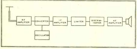
FIG. 2. BLOCK DIAGRAM OF A CONVENTIONAL FM RECEIVER
