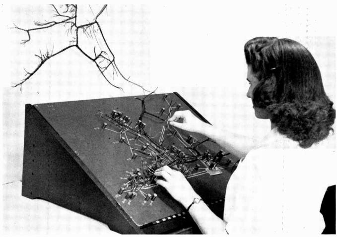
FIG. 1. THE CABLING BOARD USES SPRING BINDING POSTS TO CONNECT THE WIRES TO THE CONTACTS ALONG THE BOTTOM EDGE
