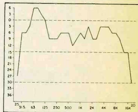
Fig. 11. This diagram shows the sound that a listener hears as he adjusts for best bass.
