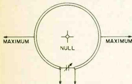
Standard loop antenna is simple and easy to build. Sometimes used in mobile DFing.
