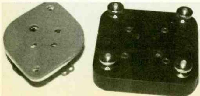
These are two examples of WD-11 tube sockets made by the author. They were made up from parts of World War II vintage tube sockets, and then customized to fit.
