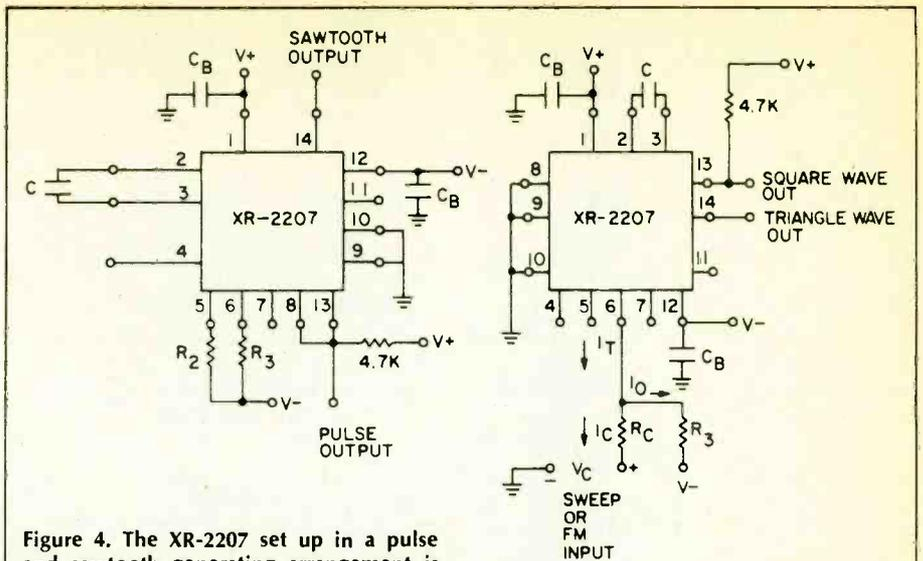
Figure 4. The XR-2207 set up in a pulse and sawtooth generating arrangement is shown in the schematic above. As the text describes, you'll need either a split-voltage 6-volt supply, or 2 6-volt batteries.
