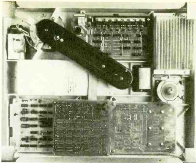
This bottom view of the Shugart SA4000 rigid disk drive shows the electronics controlling the drive, and the motor and pulley mechanism. A 14-inch unit, the SA4000 is an example of the current type of Winchester.
