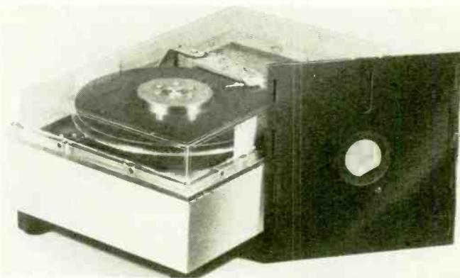
Perlec's Model D8000 offers 20 Mbyte capacity in a sealed disk unit. This Winchester drive uses the 8-inch format; the disk leaning against it is used in this type of unit.
