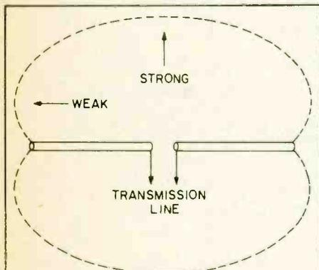
The dipole makes simplest shortwave receiving antenna. Note directivity patterns.
