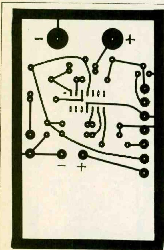
This is the foil side down view of Heat Loss Sentry's PC board. Care must be exercised in etching board.
