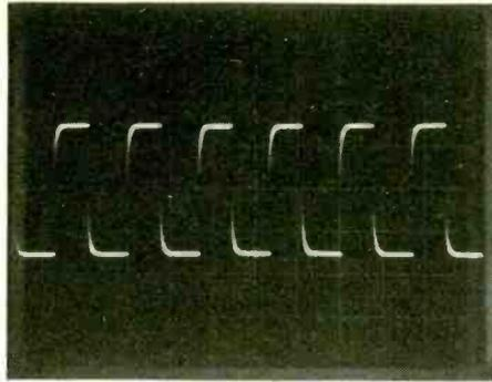
Too much capacity shows up in a rounded leading edge, as shown here in Fig. 2A.
