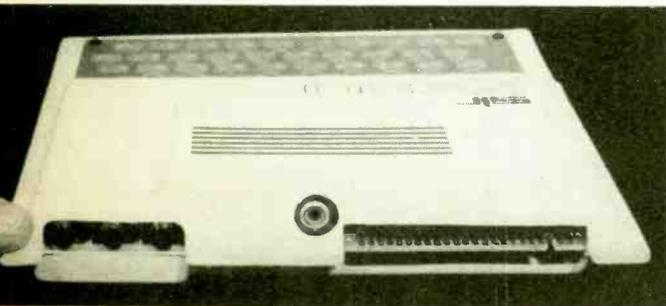
Within the ZX80 computer is an RF modulator with an output on UHF channel 36. A standard phono jack on rear provides RF output to your TV.
