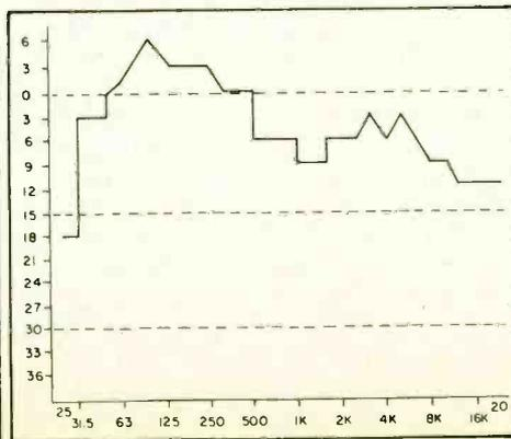
Fig. 4. This dramatic difference in speaker performance results from speakers on floor.
