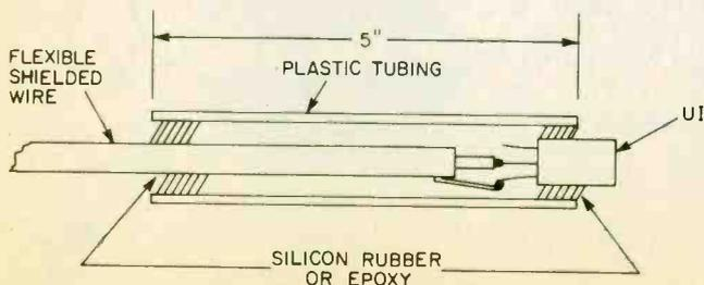
To the left is a drawing of the heat sensing probe. Follow the set-up closely, and use the glue! At right is an exact size drawing of the meter face. Cut it out and paste it right on.
