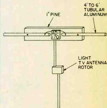
The Datong Active Antenna, Model AD-170 fits within dipole antenna elements!
