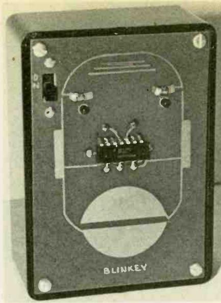
termined by the value of C1 and the resistor. Instead of using a resistor, you place your finger or hand across the touchplate, the resistance of your hand determines the frequency of oscillation. As you press harder, the resistance decreases and the frequency of oscillation increases. Now, if we connect U1C and D to the oscillator, LED (left) and LED (right) will simultaneously blink. U1C and D are buffers which provide enough current for the two LEDs to turn on.
