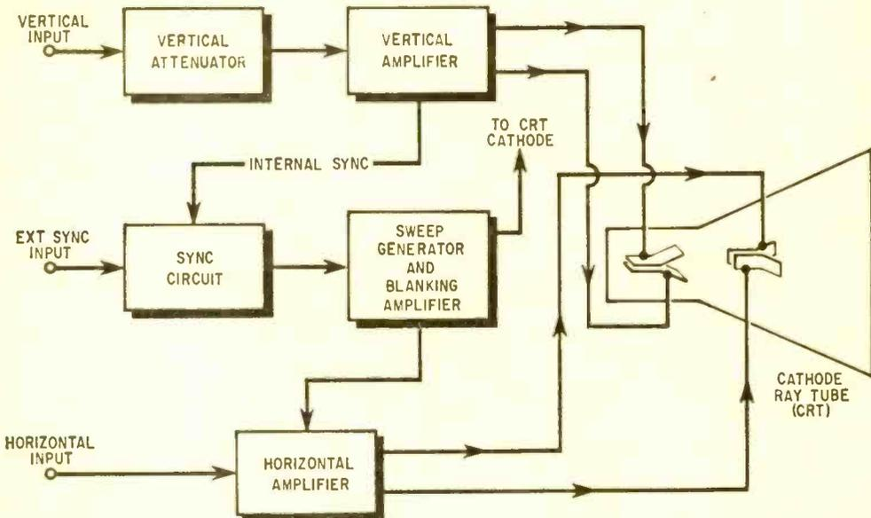
Fig. 20. Block diagram of a Heath oscilloscope using electrostatic deflection.
