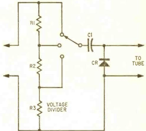
Fig. 19. Typical diode circuit used by VTVM to rectify AC voltages that'll be measured.
