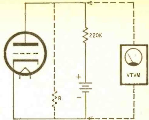
Fig. 18. Diagram shows a VTVM connected to a circuit for voltage measurement. Extreme high internal resistance of the VTVM does not change circuit parameters during testing.
