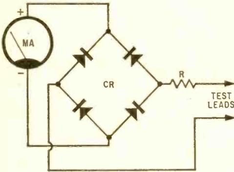
Fig. 11. Full-wave bridge rectifies AC.
