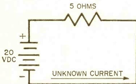
Fig. 14. Use Ohm's law to determine the unknown current in this simple series circuit.
