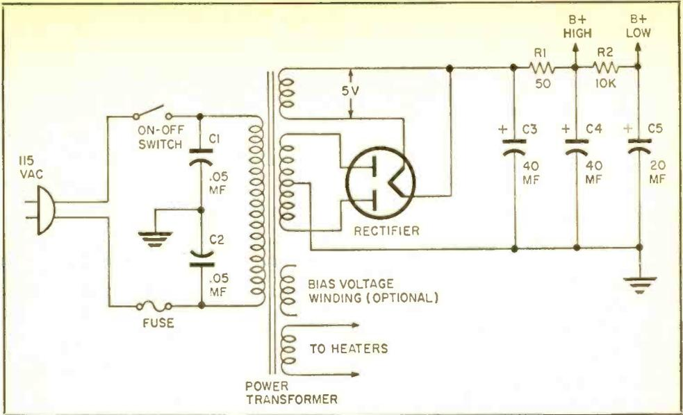
Fig. 6. Typical full-wave rectifier circuit used in high-fidelity components.
