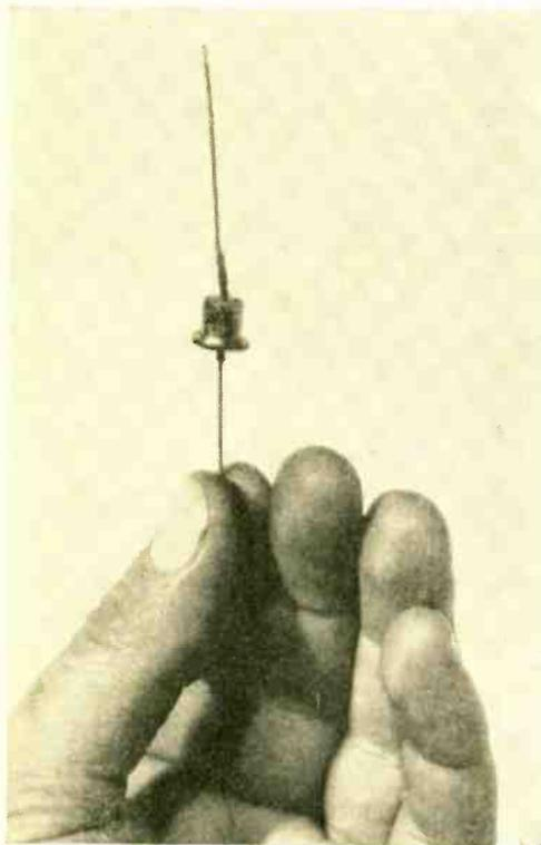
All it takes is any silicon diode (top) soldered across the AC switch terminals of the volume control (below) to do the job.
