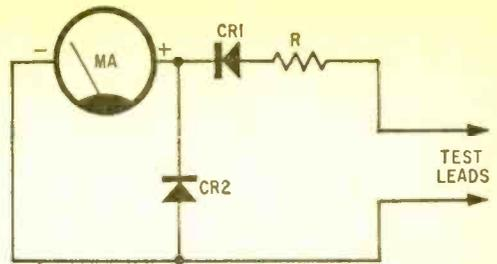
Fig. 10. CR2 eliminates negative pulses.
