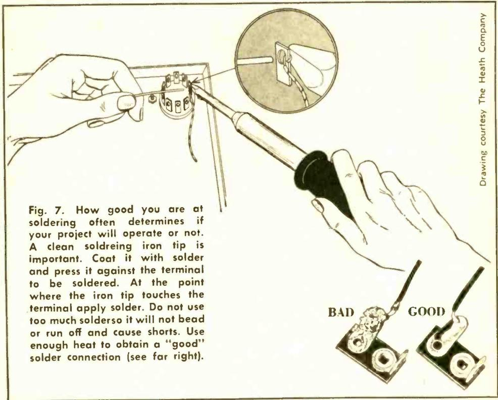
Fig. 7. How good you are at soldering often determines if your project will operate or not. A clean soldreing iron tip is important. Coat it with solder and press it against the terminal to be soldered. At the point where the iron tip touches the terminal apply solder. Do not use too much solder so it will not bead or run off and cause shorts. Use enough heat to obtain a "good" solder connection (see far right).
