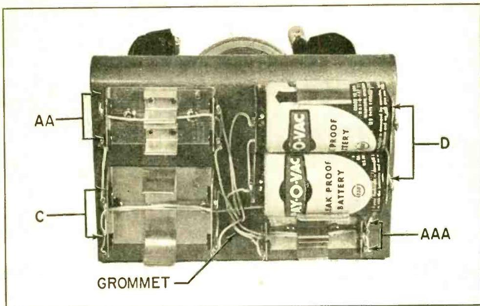
Back of the tester's cover is just large enough to hold the four dual battery holders.
