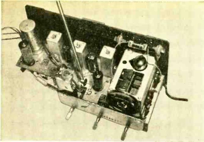
Installing the silicon power diode rectifier is a simple matter. If there is not enough room on the off-on switch or under the chassis, mount it on the chassis top away from tubes.
