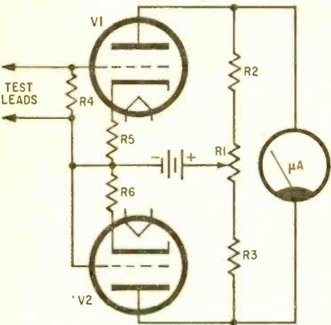
Fig. 15. A balanced VTVM circuit using two vacuum tubes. With no input signal, plate voltages are equal and meter reads zero.
