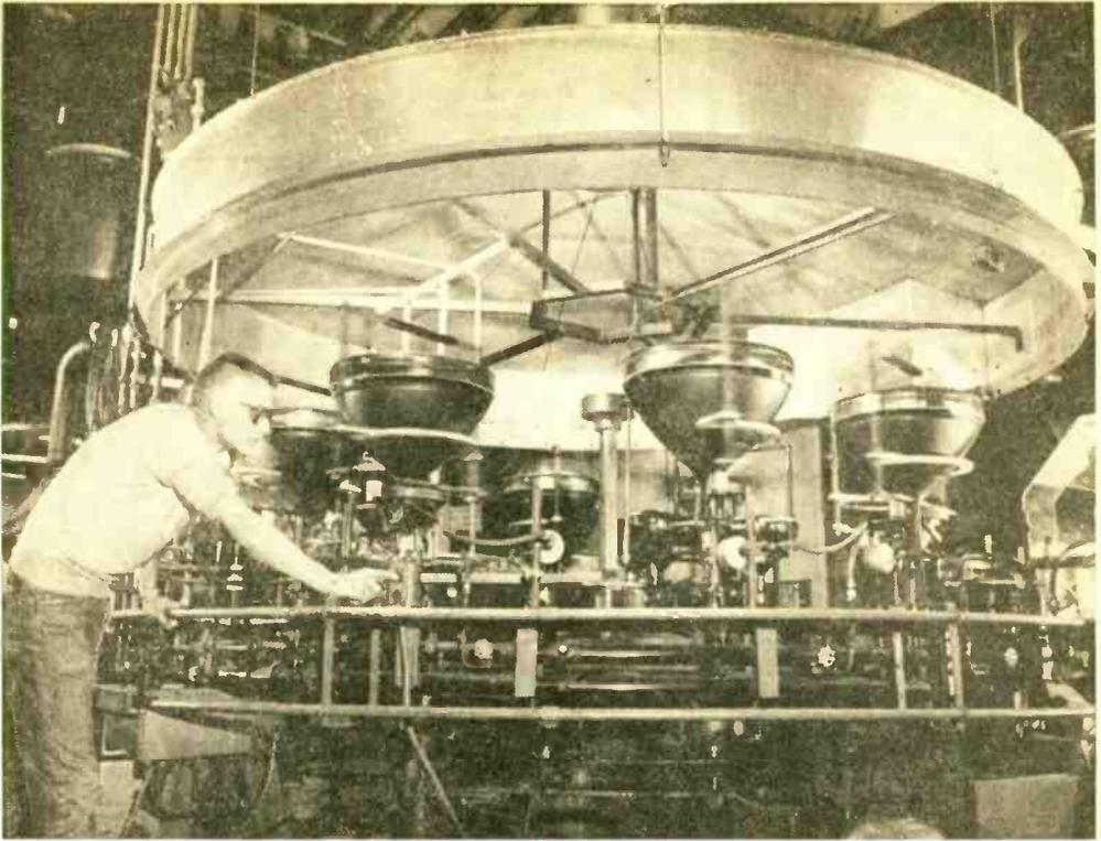
Fig. 10. This machine, which installs the electron gun, removes the air and then seals the television picture tube, is typical of automatic equipment in modern vacuum tube plants.
