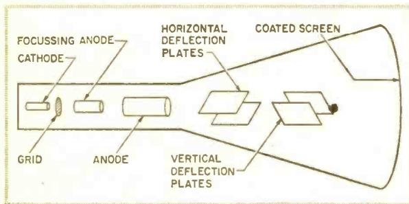
Fig. 11. A cathode ray tube of the type used in small TV sets and oscilloscopes. The electron stream from the cathode is shaped into a pencil beam by the anodes and positioned up and down, left and right by the deflection plates. Where the beam strikes the coated screen light rays are generated.
