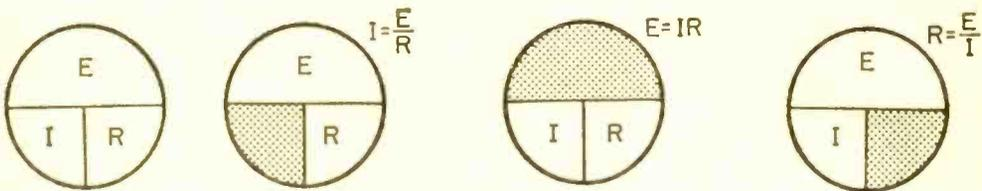
Fig. 11. The Ohm's law memory wheel—cover one value with your finger and the equation is given by the remaining two values.
