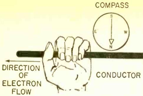
Fig. 7. Using the left hand rule to find the direction of electron flow in a conducting wire.
