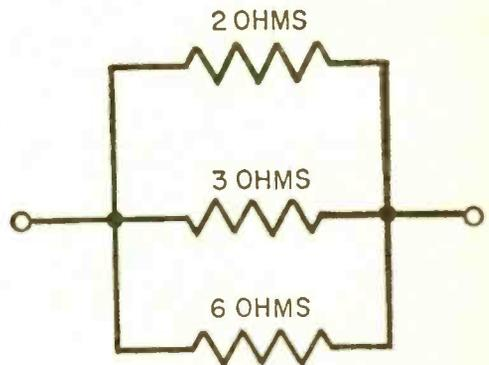
Fig. 20. Three resistors in parallel can be solved by calling on Ohm's law to help.
