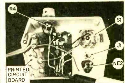
The 600-ohm resistor is unsoldered from the circuit board at the location shown.
