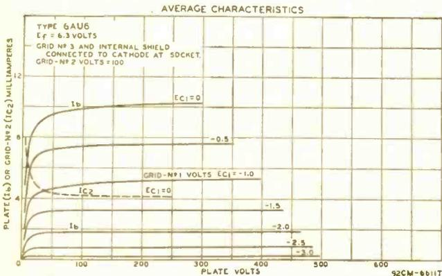
Fig. 9. Characteristic curves for a typical pentode (6AU6). Note that the dip in the curves common to the tetrode does not appear here. Also, plate current reaches a peak at a very low plate voltage and increases after that are small.
