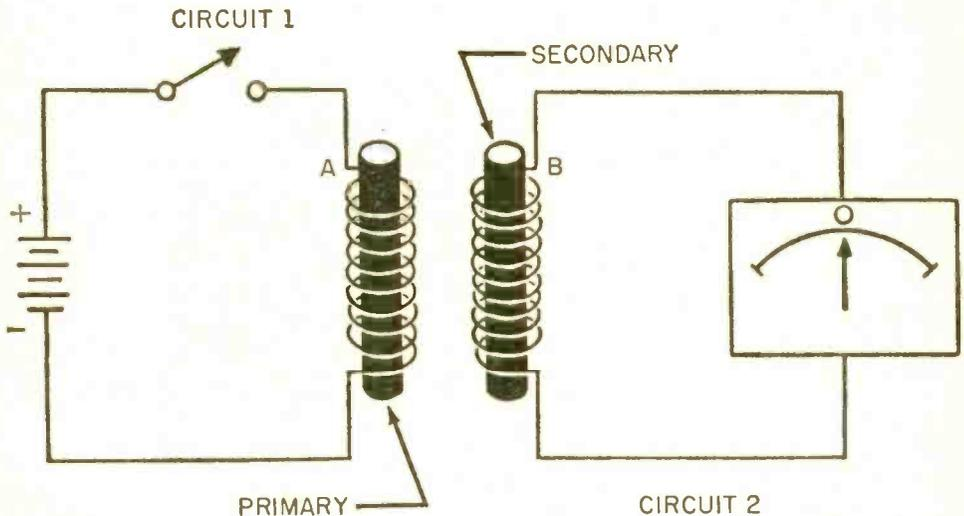
Fig. 25. A simple demonstration that illustrates how currents are induced.
