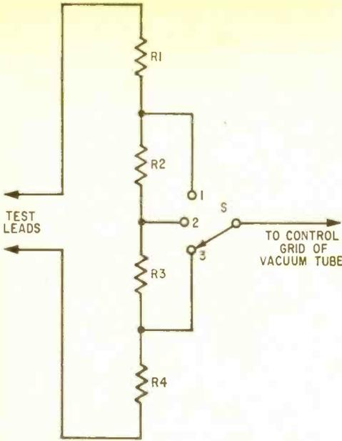
Fig. 17. Voltage divider resistors provide rapid and accurate VTVM range selection.
