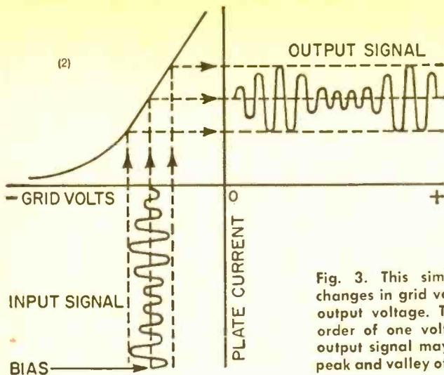
Fig. 3. This simple diagram shows how small changes in grid voltage causes changes in the plate output voltage. The input signal is usually in the order of one volt or less in audio amplifiers. The output signal may have swings in voltage between peak and valley of 300 volts with gains in the 1000's.
