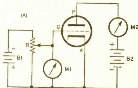
Fig. 2. The schematic diagram shown in (A) above is a typical test setup circuit for determining a triode's characteristic curves. One such curve of a family of curves is shown below (B) when the voltage is fixed.
