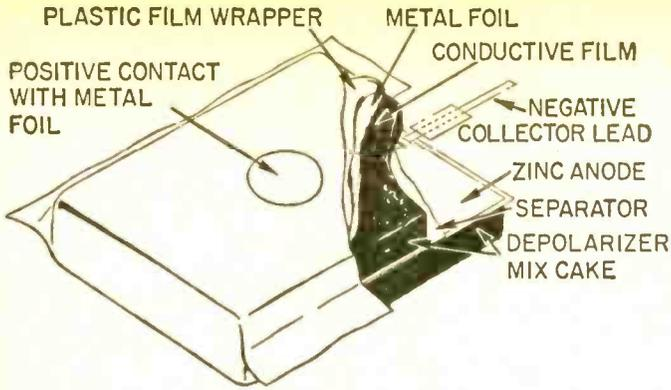
Fig. 3. "Cut away" detail drawing of a flat cathodic-envelope dry cell. Many of these cells are connected in series to obtain high voltages for portable transistor radios and many other gadgets such as hearing aids and test gear.
