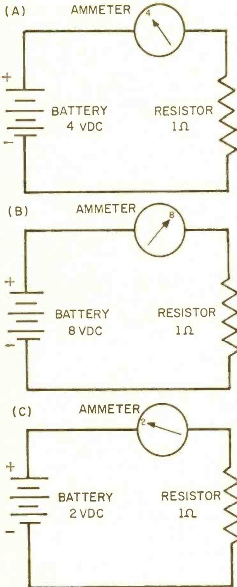
Fig. 10. Simple demonstration showing that current in a circuit is inversely proportional (1 over R) to the resistance in the closed circuit.
