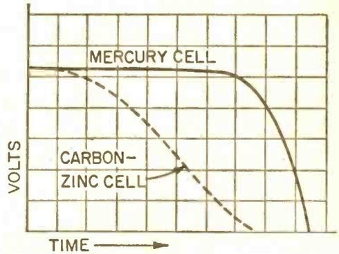
Fig. 4. Comparison of dry cell output voltages and how they decrease under constant load for equal time/work periods.
