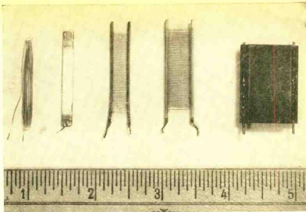
Fig. 6. Left-to-right: filament, cathode, grid, screen grid and plate of a small receiving tube shown life size. Each element fits inside the element to its right.
