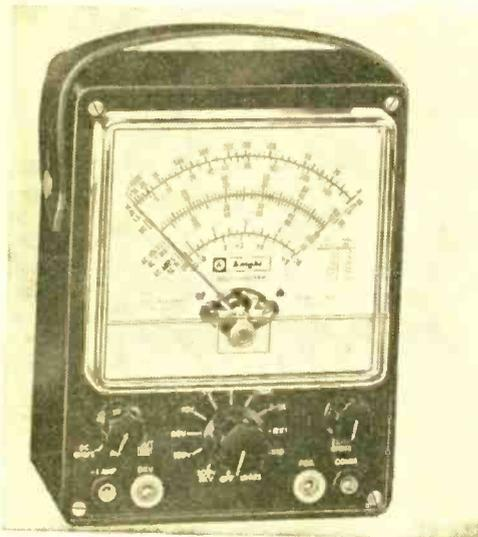
This is a Knight volt-ohm-meter which was constructed from a kit in only a few hours. The "VOM" measures AC/DC volts, current and resistance, just about a must for any ham operator who likes to build or fix gear.
