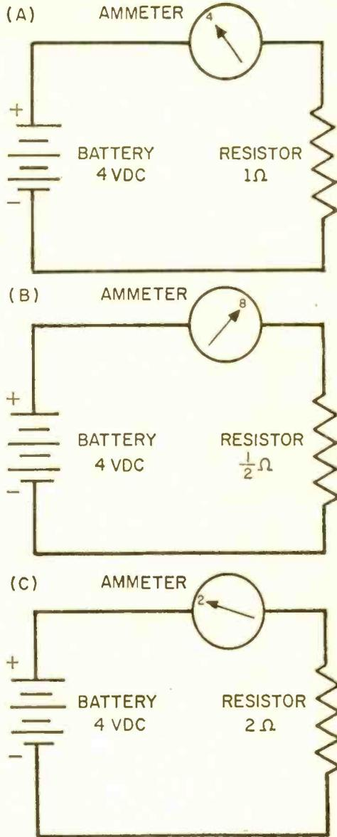
Fig. 9. Simple demonstration showing that current in a circuit is directly proportional to the voltage impressed across the circuit.
