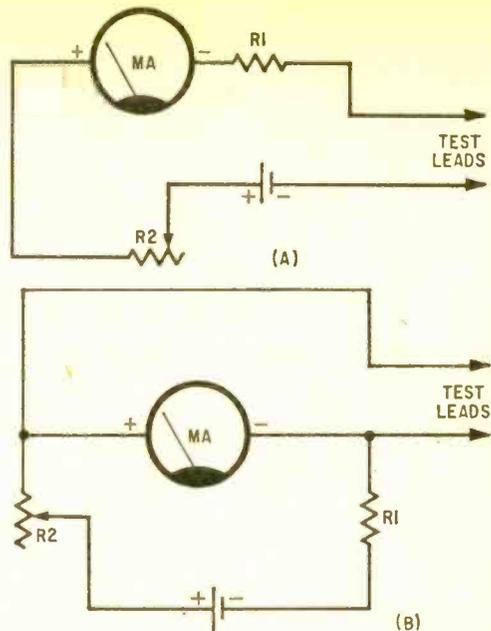
Fig. 8. Diagram (A) above shows a milliammeter with series battery used as an ohmmeter. Diagram (B) shows a modified ohmmeter circuit useful for measuring low resistance values.
