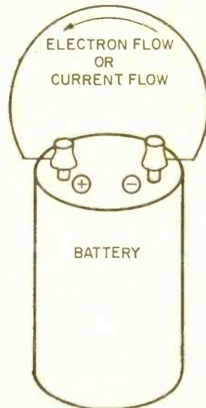
Fig. 8. Electron flow caused by a dry cell.
