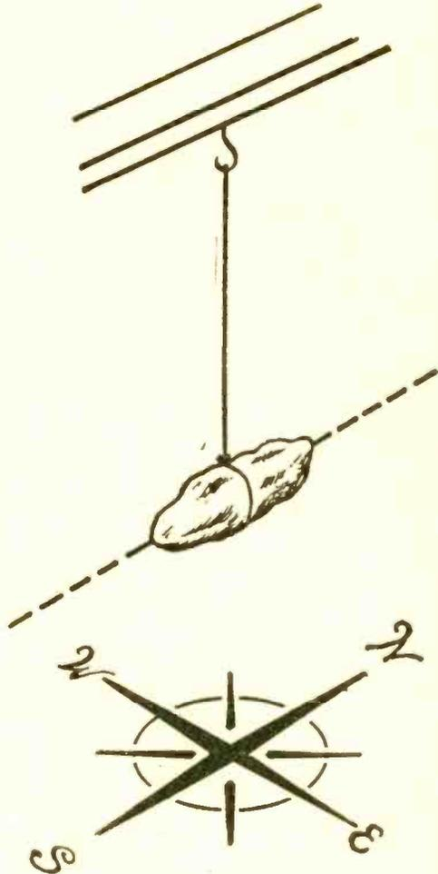
Fig. 22. The lodestone is a ferrous rock that was the first useful magnetic compass.
