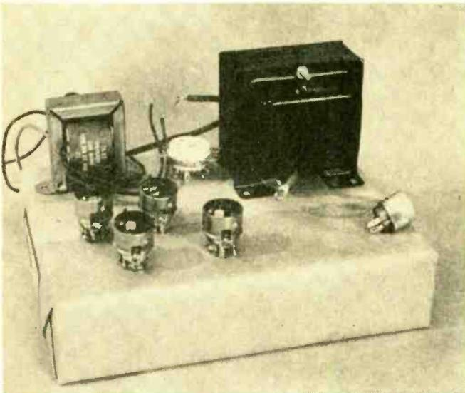
Fig. 2. Unless you are a design engineer with years of experience in electronics, it would be wise to place parts on a chassis to see if there will be ample room.
