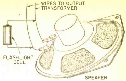
Fig. 4. Cell causes speaker to "thump."
