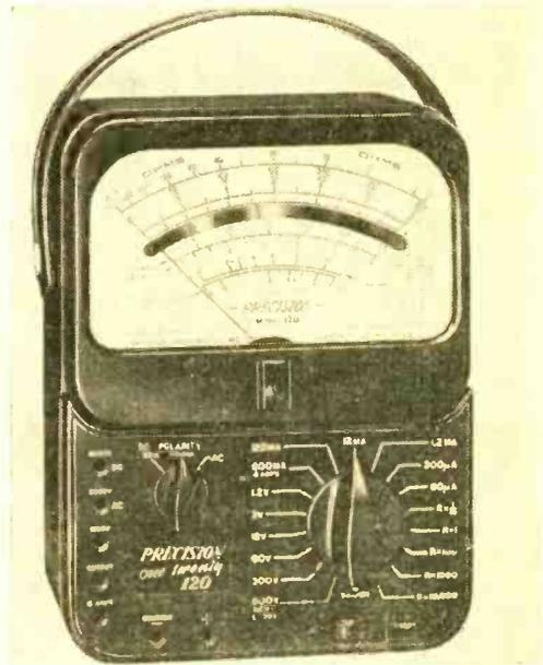
Figs. 12 and 13. Shown above is the Precision 120 VOM. Below is the Knight-Kit volt-ohmmeter that is available in kit form.
