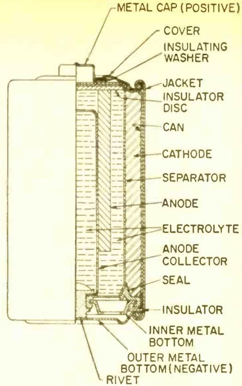
Fig. 5. Internal construction details of an alkaline cell. In this cell the electrolyte is a highly alkaline (opposite of an acid) solution.
