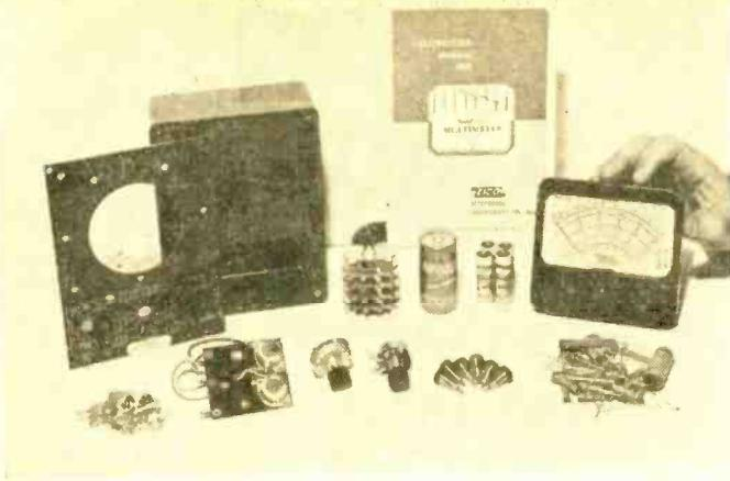
This assortment of parts assembles into a multimeter, or "circuit analyzer," as it is sometimes called. It permits the ham to have the functions of several types of test instruments in a single enclosure. These meters are available from a number of manufacturers (this one is by EICO) in kit or wired form. Assembling a kit of this type takes a few hours but has the advantage of relatively low cost. In addition, the kit building venture is both fun and experience for new hams.
