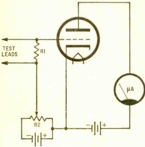
Fig. 14. A basic single-ended vacuum tube voltmeter circuit—R2 provides meter zero set.
