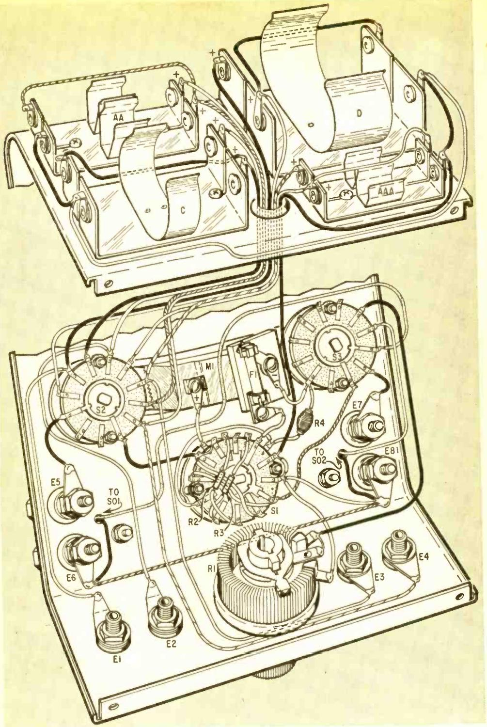
Considering the crowding of parts in the Universal Battery Tester, it is wise to follow the parts layout and wire placement as illustrated in the pictorial diagram above.
