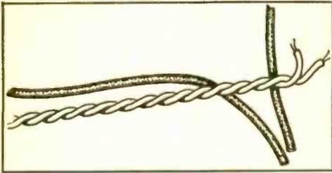
Fig. 5. Twisted AC heater leads reduce hum.
