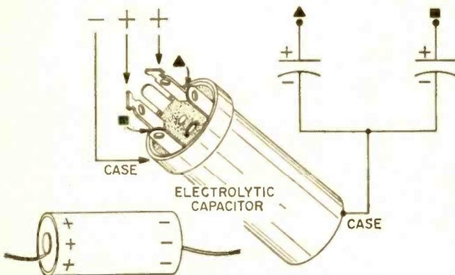
Fig. 5. Electrolytic capacitors come in two standard types. Single units and transistor circuits type usually come with wire leads. Can types are multiple units as a rule and very often have large microfarad ratings that can handle high plate voltages.
