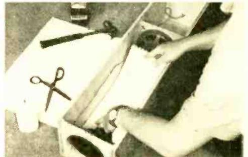
**FOAM RUBBER** is used as acoustical padding to line all sides of the airtight upper chamber.
