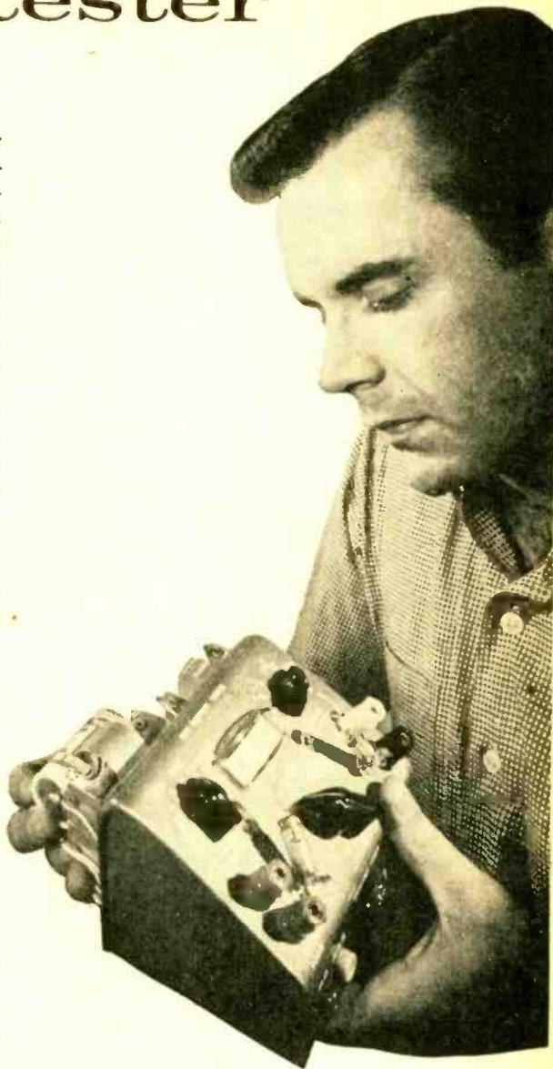
The second of these is a 25 ohm, 25 watt rheostat, R1. The VARIABLE LOAD position of the LOAD SELECTOR switch, S3, connects the 25 ohm rheostat, R1 across any battery selected by the BATTERY SELECTOR switch, S2. Load currents up to 500 milliamperes are possible through the meter. The meter is protected by a type 8AG instrument fuse rated at 0.5 ampere.
