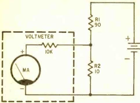
Fig. 7. The DC voltmeter shown simplified as a meter and series resistor connected to an external circuit of much lower resistance.
