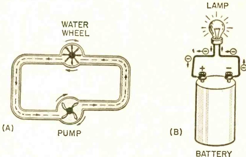
Fig. 6. The action of a water pump (A) compared to the electrical battery (B).
