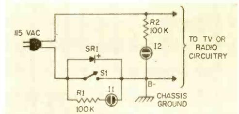
Schematic diagram of AC circuit additions that can be made in any AC/DC receiver.
