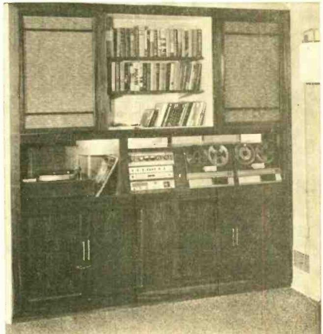
Fig. 4E. This custom system consists of all Allied and Knight-Kit components. From left to right on equipment shelf: professional turntable and tone arm, record amplifier, transistorized stereo amplifier and receiver with clock, and finally a pair of KN-4000 tape decks. Cost less wood cabinet—\$790.
