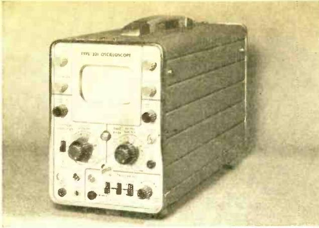
Fig. 21. The advanced experimenter who works on elaborate and critical projects will find the oscilloscope a valuable piece of test gear. The 'scope (such as the Tektronix Type 321 at left) lets you look at waveforms as they occur in the operating circuit. Modern units are compact and easy to tote from job to job.
