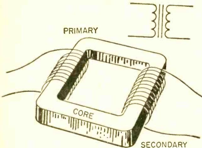
Fig. 26. A simplified drawing of a two winding transformer on an iron core. The primary winding is determined by its connection to the input circuit. Schematic diagram (upper right) is typical for a ferrous-core transformer.
