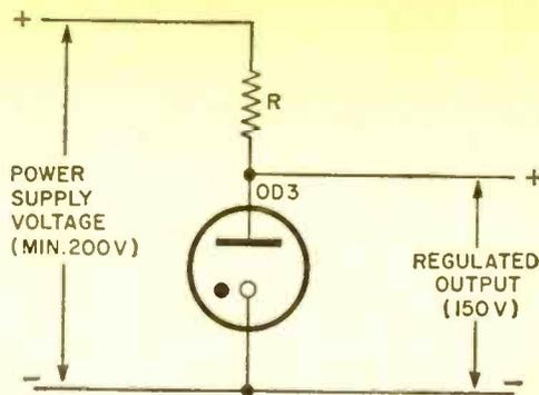
Fig. 12. The voltage regulator tube is not a vacuum tube but a gas filled tube that glows with a weak "neon-like" glow when on.
