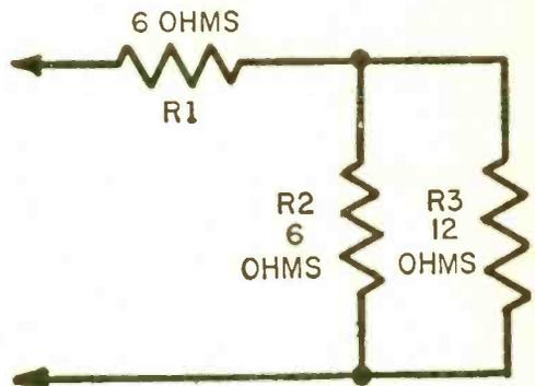
Fig. 21. Series-parallel combinations of resistors require some thinking to solve.
