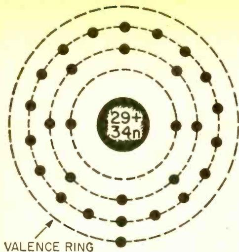
Fig. 3. Flat diagram of the copper atom.
