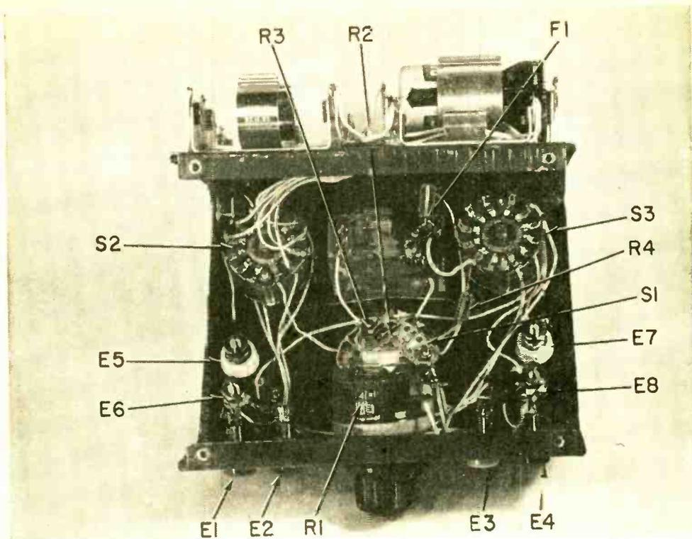
Bottom view of the tester showing location of parts. Follow construction hints on pages 29-34.
