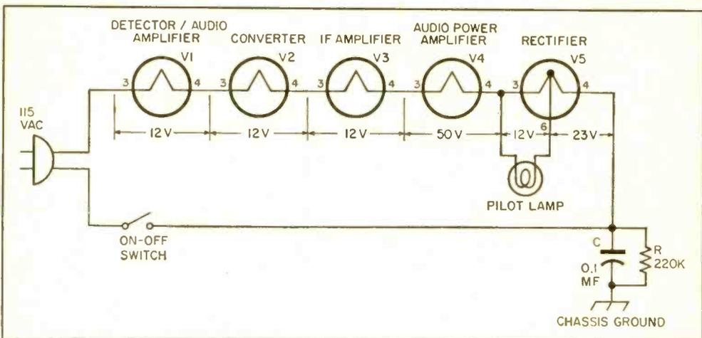
Fig. 2. Filament line-up for a typical "all American five" superhet table radio.
