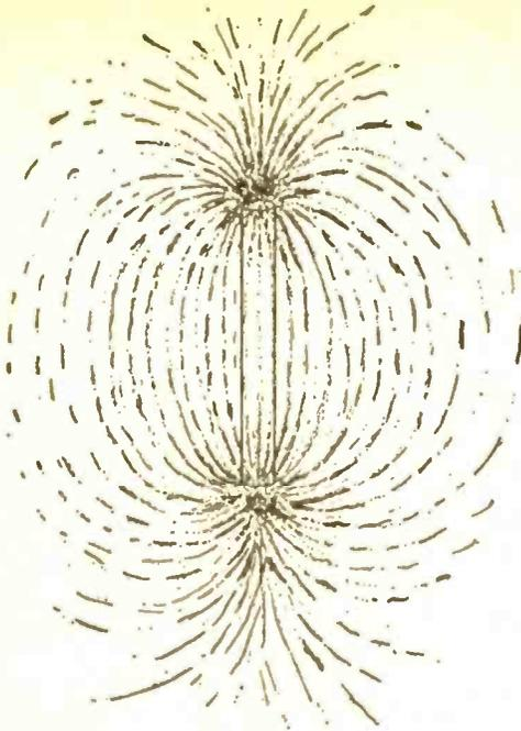
Fig. 23. Place a bar magnet under a piece of paper and sprinkle iron filings on top. Filing will trace out the magnetic field's force lines when the magnet aligns them.
