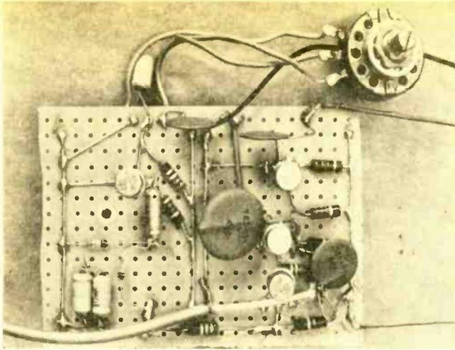
Fig. 8. Wiring up transistor circuits calls for different wiring techniques. Parts are smaller and can be placed on a phenolic board stamped with many evenly spaced mounting holes.
