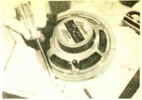
**SPEAKER** is mounted on 7-in. square of plywood. Screwdriver points to two solder lugs.
