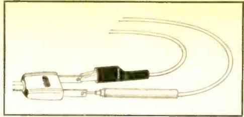
Fig. 1. The ohmmeter is the best instrument for checking out the appliance's major Nemesis—the open line cord. Wire breaks are common.
