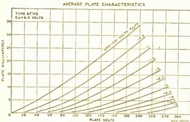
Fig. 5. The average plate characteristics for a triode tube. Note that a curve is drawn for several control grid voltage potentials. This tube is best operated at a bias of -1 volt at a plate voltage of about 135.
