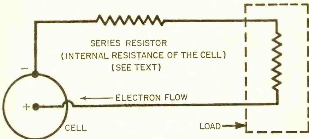
Fig. 10. Diagram shows how a cell's internal resistance limits current flow.
