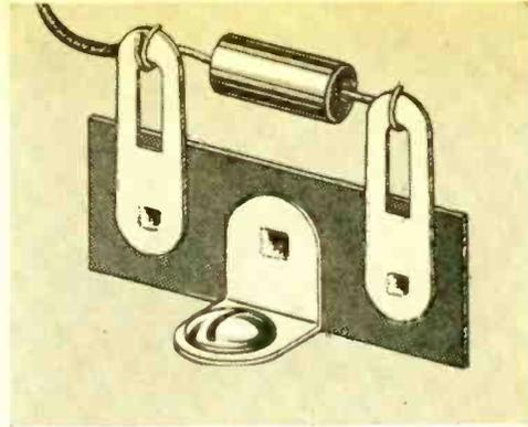
Fig. 6. Mechanically secure leads to lugs.
