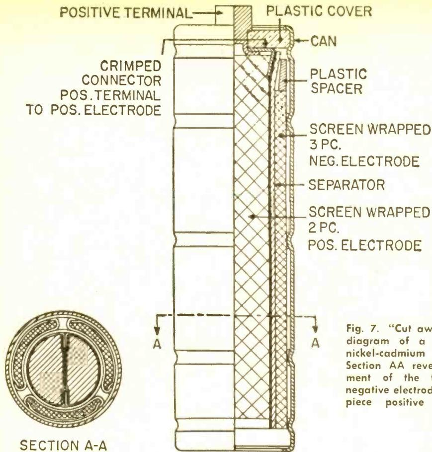
Fig. 7. "Cut away" detail diagram of a cylindrical nickel-cadmium dry cell. Section AA reveals placement of the three-piece negative electrode and two-piece positive electrode.
