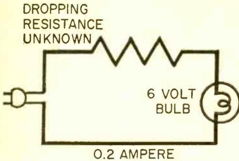
Fig. 17. Series dropping resistors can be calculated by Ohm's law and some reasoning.
