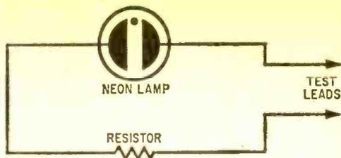
Fig. 2. A neon bulb with series resistor makes an excellent line voltage checker. Use an NE-51 bulb with 200,000-ohm  $\frac{1}{2}$ -watt resistor.
