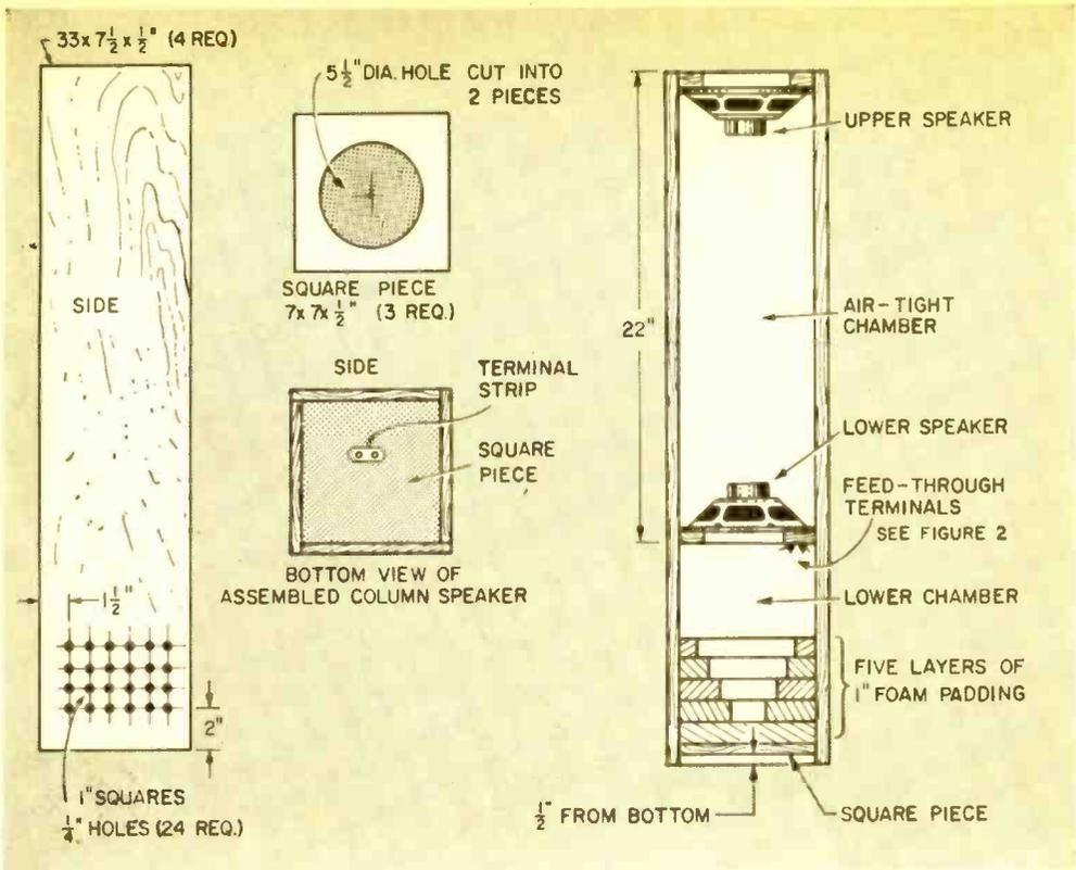
Column speaker can be assembled by following construction details shown above. Construction can be speeded up by having lumber dealer cut plywood to exact sizes.
