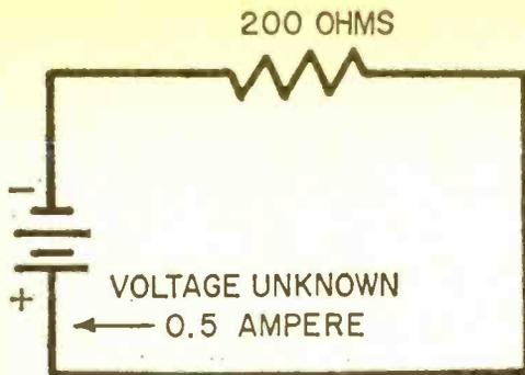
Fig. 12. Using Ohm's law to determine voltage from values of current and resistance.
