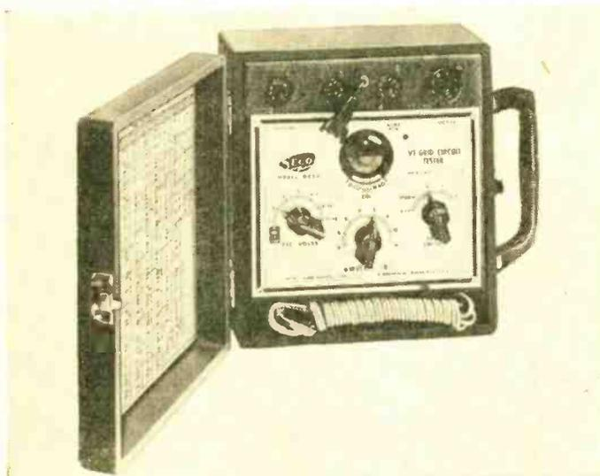
Fig. 23. There are a host of specialized test instruments designed to be used in limited applications but occur repeatedly in certain professions and hobby areas. The Seco Model GVT-9 grid circuit tube tester checks for vacuum tube grid emission, leakage, shorts and gas. This easy to operate test gear is carried by repair men on service calls.
