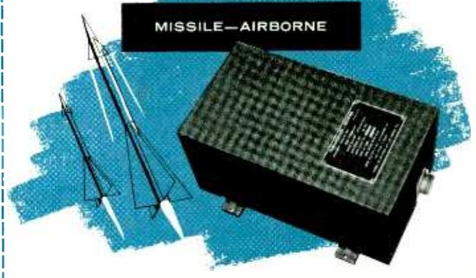
Perkin airborne power supplies more than meet both military specifications MIL-E-5272A and MIL-C-7115. The use of silicon rectifiers provide a much more compact package with higher efficiency ratings and longer life expectancy. The unit illustrated provides 27.5 volts DC (26 to 30 volt range), 20 amperes continuous duty. The input is 115/200V AC, 3 phase; frequency range 400 CPS  $\pm 6$  CPS. The regulation is less than  $\pm 0.5$  volts.
