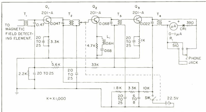
FIG. 1—Amplifier-indicator unit of cable detector is tuned to 250 cps by the series L-C circuit in the emitter of the second stage. Three transistors give overall gain of 85 db
