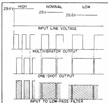
FIG. 12—Overall regulation action for different input line levels
