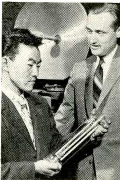
Helitron tube, displayed by its inventor D. A. Watkins and his assistant G. Wada. Tube is purported to be a major improvement over the backward wave oscillator and costs about half as much to produce. Operating frequencies range from 200 to 10,000 mc. Tube is voltage tuned and a two-to-one change in voltage causes a two-to-one change in frequency. Development was done at Stanford University
