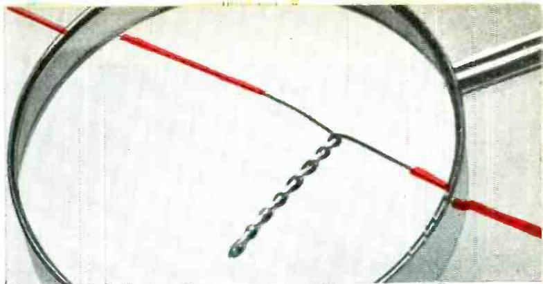
**1. STRONG JOINTS**—as strong as the same joints made in bare copper wire—are produced. Here in laboratory test, joint holds under high stress.
