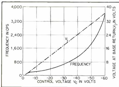
FIG. 4—Characteristics of variable-frequency circuit shown in Fig. 3
