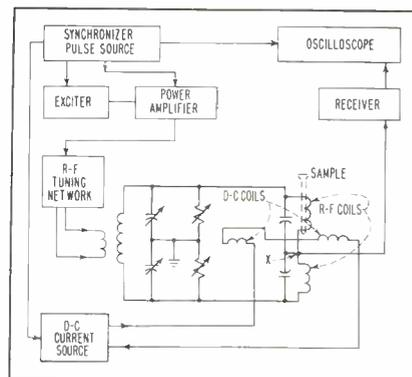
FIG. 4—Basis of the spin echo storage technique
