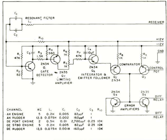
FIG. 5—Resonant filter, gate detector, limiting amplifier and the electronics of the servo-system in the ship model
