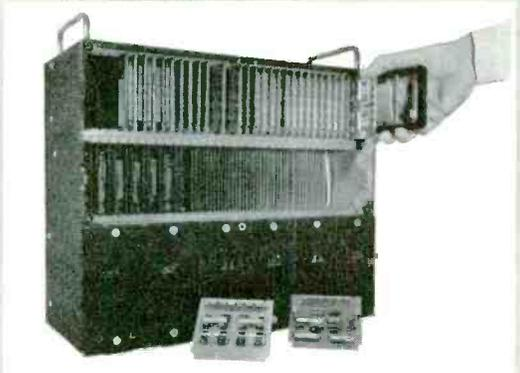
Input-output unit of the Ramo-Wooldridge RW-30 airborne digital computer
