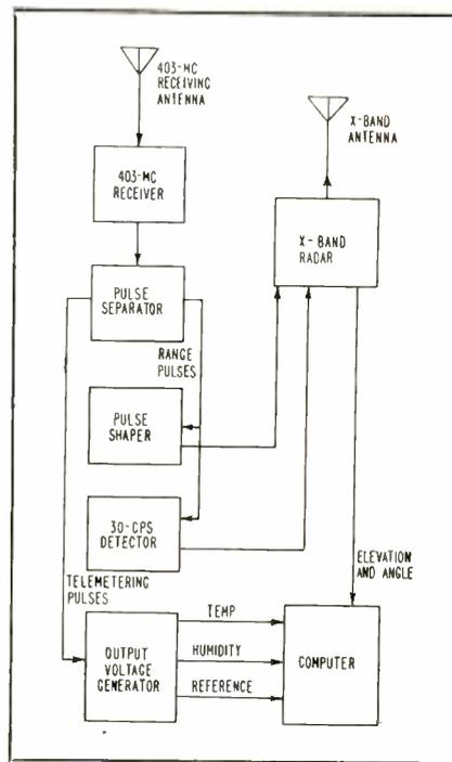
Fig. 3—Shipboard equipment includes non-directional 403-mc receiver
