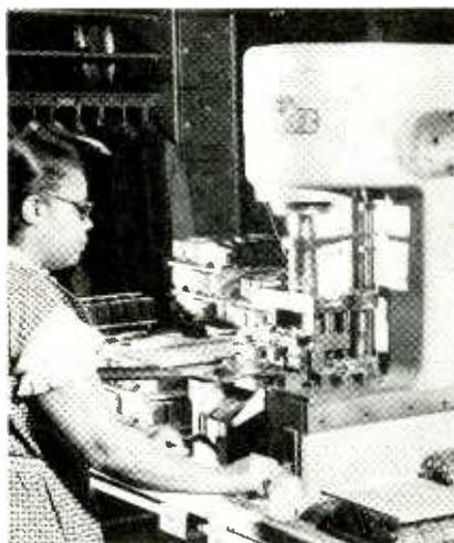
Shearing press. Operator has pushed in slide by moving lever in front of her, and is here actuating controls of press
