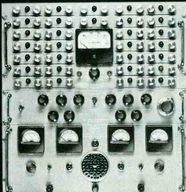
The new Arnoux Model TDS30-1 Decommutation System is completely self-contained within three chassis assemblies consisting of: Gating Unit (TOP), Pulse Selector (MIDDLE) and Regulated Power Supply (BOTTOM). The unit handles 28 channels of information and occupies only 19½ inches of panel height in a standard relay rack. Overall depth behind panel is 13 inches.
