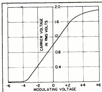
FIG. 4—Modulation characteristic of IN54A-diode 10.5-kc subcarrier modulator
