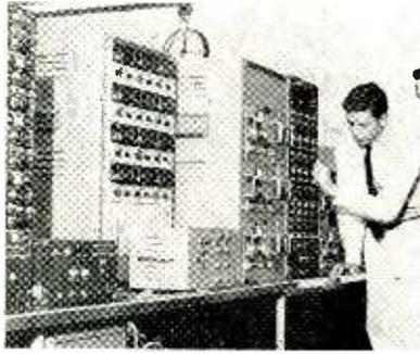
are amplified by oscillograph recording amplifiers for display on a 12-channel oscilloscope. These units monitor the signals from the strain-gage translators on separate channels.
