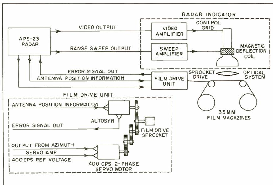
FIG. 1—Block diagram of the recording system. A cathode-ray tube trace is intensity-modulated with the radar video signal and is swept in synchronism with the range sweep of the radar
