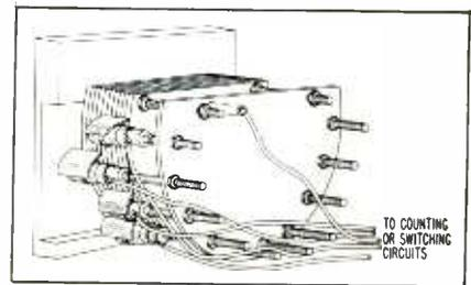
FIG. 1—Complete assembly of the illuminated indicator
