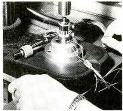
Operator has placed yoke rings in position on thimble and is preparing to operate press controls with both hands to push rings down against those already on stator. Complete stator with yoke rings can be seen on bed of press
