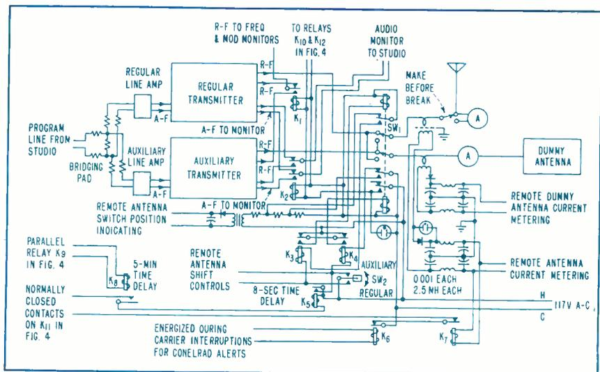
FIG. 3—Complete automatic antenna shift circuit. Audio is fed simultaneously to both transmitters through bridging pad and additional line amplifier
