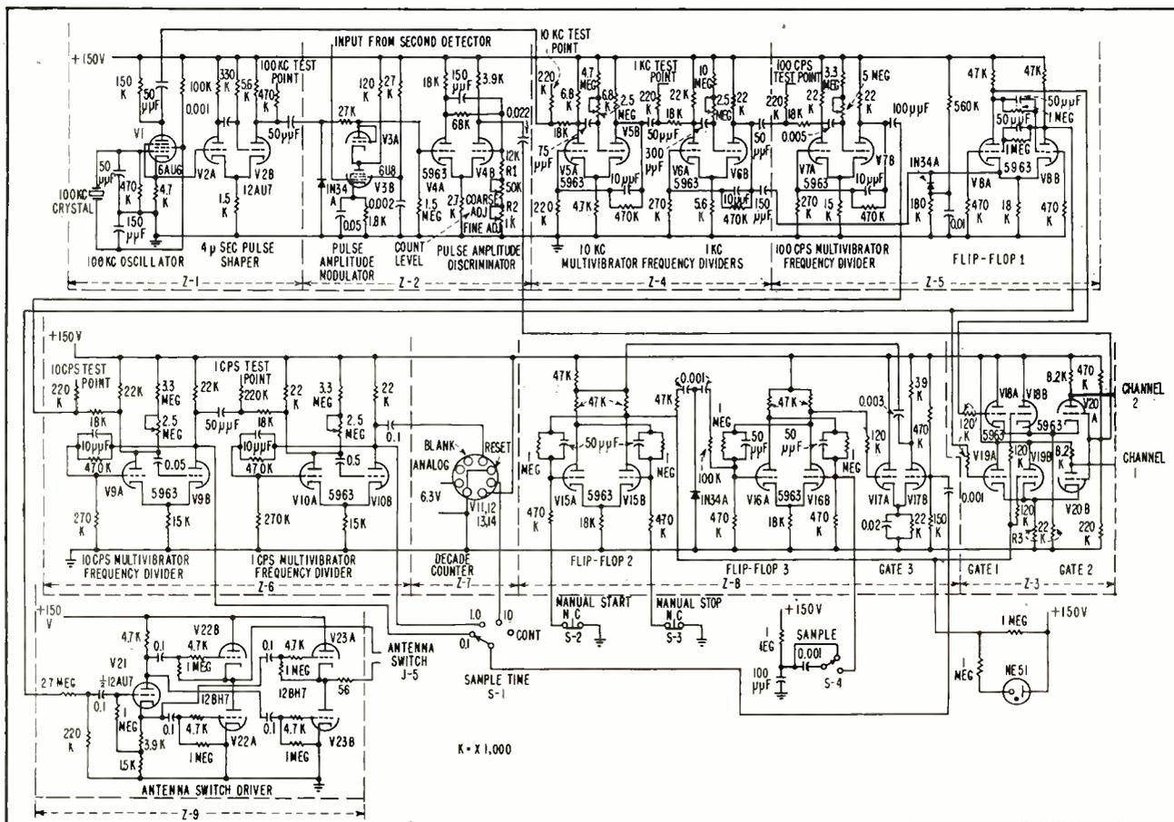
FIG. 3—Schematic diagram of integrating receiver. Output of each channel feeds counters shown in Fig. 4.
