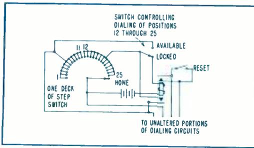
FIG. 1—Modification of step-switch control circuit at remote control point. With switch in locked position as shown, dialing above 11 makes switch return to home position
