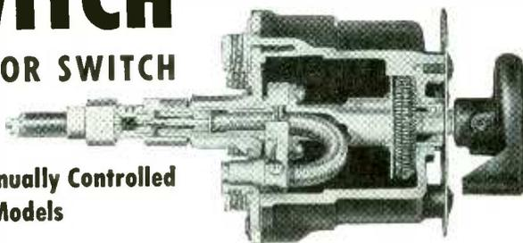
The COAXWITCH is an RF switch for use in coaxial circuits where it is important that the 50 OHM impedance of the cables be maintained. In a circuit sense, this switch consists of two pairs of "N" connectors spaced 4 1/2" apart using RG-8/U as the connecting link. The COAXWITCH itself introduces no VSWR other than that of connectors. Characteristic impedance is maintained thru all switch details. Cut-a-
