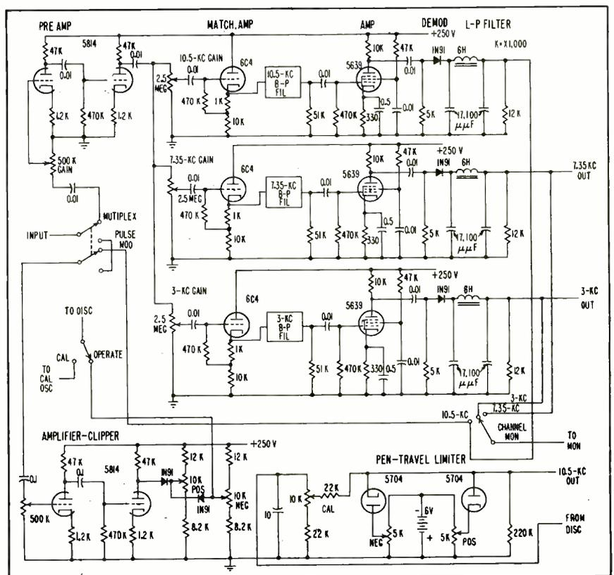
FIG. 8—Data-reduction system employs pen-travel limiters to prevent loss of calibration in the event of violent striking of the pen stops during periods of signal interference
