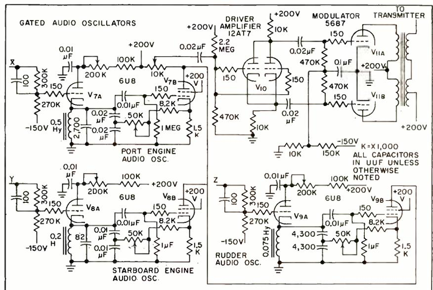
FIG. 3—Gated oscillators, modulator and transmitter in the control unit. Each gate is fed to points X, Y and Z, turning off triodes  $V_{7A}$ ,  $V_{8A}$  and  $V_{9A}$  connected across an oscillator resonant circuit, raising the circuit Q enough to sustain oscillation
