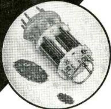
Insulating mica bridge for high-temperature electronic tube.
