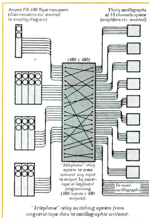
of Ampex FR-100 Tape Reproducers plays the tapes through a high-speed analog-to-digital conversion system which finds and converts selected sections to digital form at a rate of 45,000 conversions per second.
