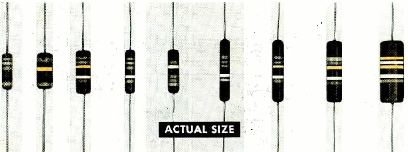
PVZ CAPACITORS range in size from .175" diameter by .625" length to .375" diameter by 1.0625" length. Capacitance ratings are available with  $\pm 20\%$ ,  $\pm 10\%$ , and  $\pm 5\%$  tolerances. The color code indicates microfarads, volts, and capacitance tolerance.
