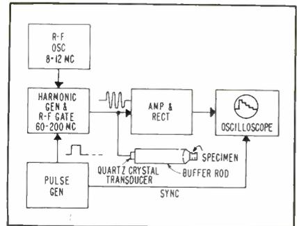
FIG. 1—Oscilloscope indicates when reflections from specimen are in phase
