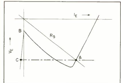
FIG. 2—Characteristic curve for typical ring counter element
