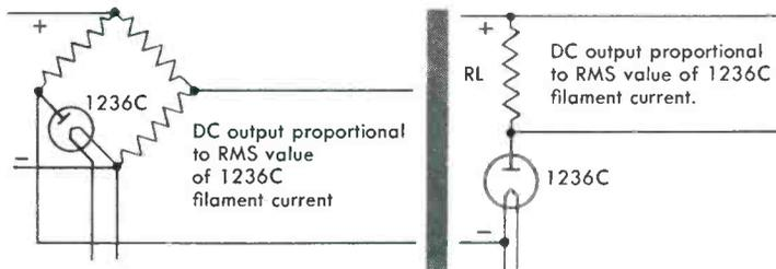
Temperature limited DIODE type 1236C is designed for service as an RMS detector for a-c voltage and current stabilizers . . . as a detector for d-c voltage and current stabilizers . . . as an RMS detector for differential voltmeters and in other similar applications.
