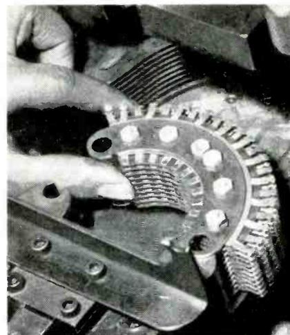
STEP 4—Removing sheared bank assembly from press after removing pins
