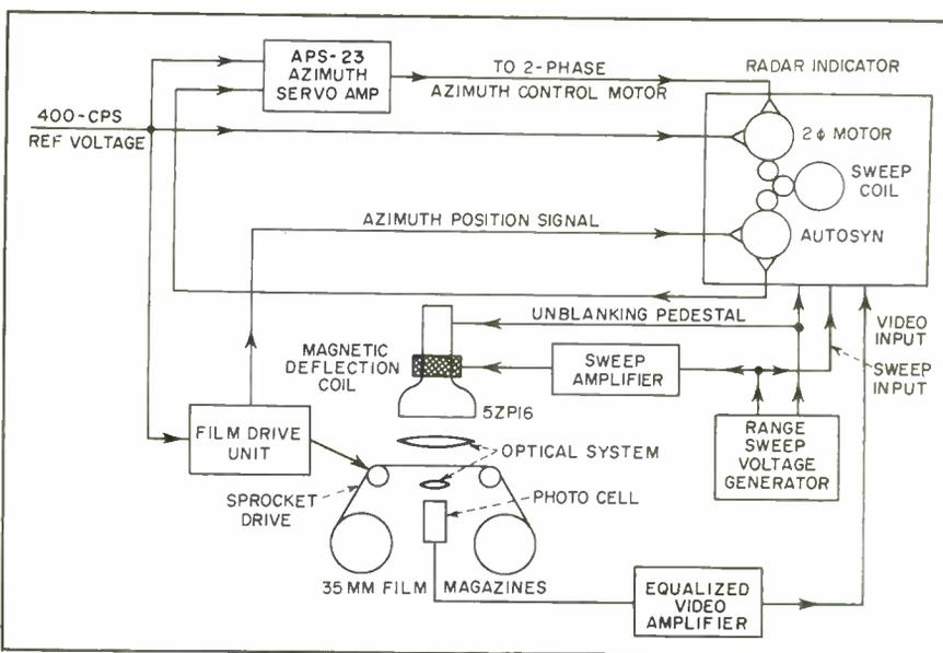
FIG. 2—Block diagram of the playback system. A phototube, located behind the focal plane, receives the light transmitted through the film and converts the light intensities into video voltage variations
