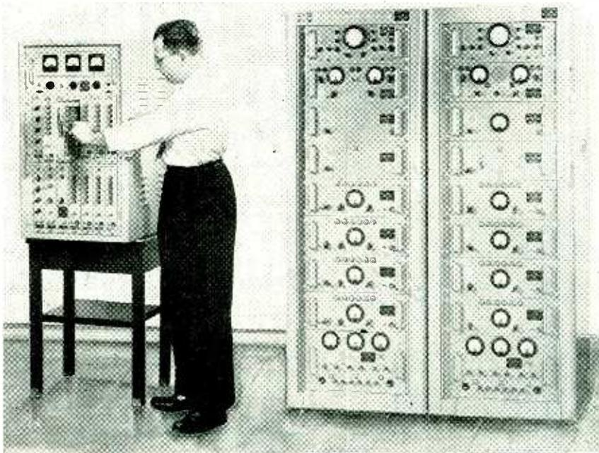
New transistorized multiplex AN/UGC-1 on table has volume of only 10.9 cu ft. compared to 55 cu ft for older two-rack electron-tube version on floor at right
