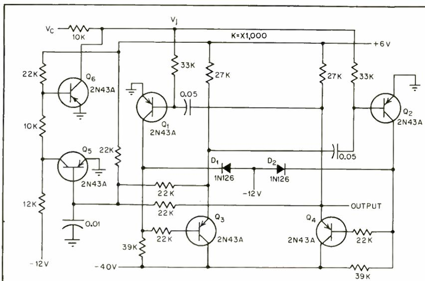
FIG. 3—Frequency of multivibrator is determined by varying return voltage of  $Q_1$  and  $Q_2$
