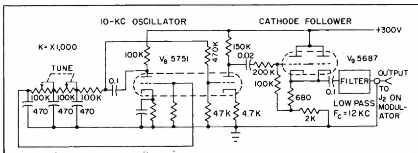
FIG. 5—The 10-kc test oscillator generates the sine-wave test signal. Dual triode  $V_8$  is a phase-shift oscillator. The test signal at the output gives less than one-tenth of one percent distortion
