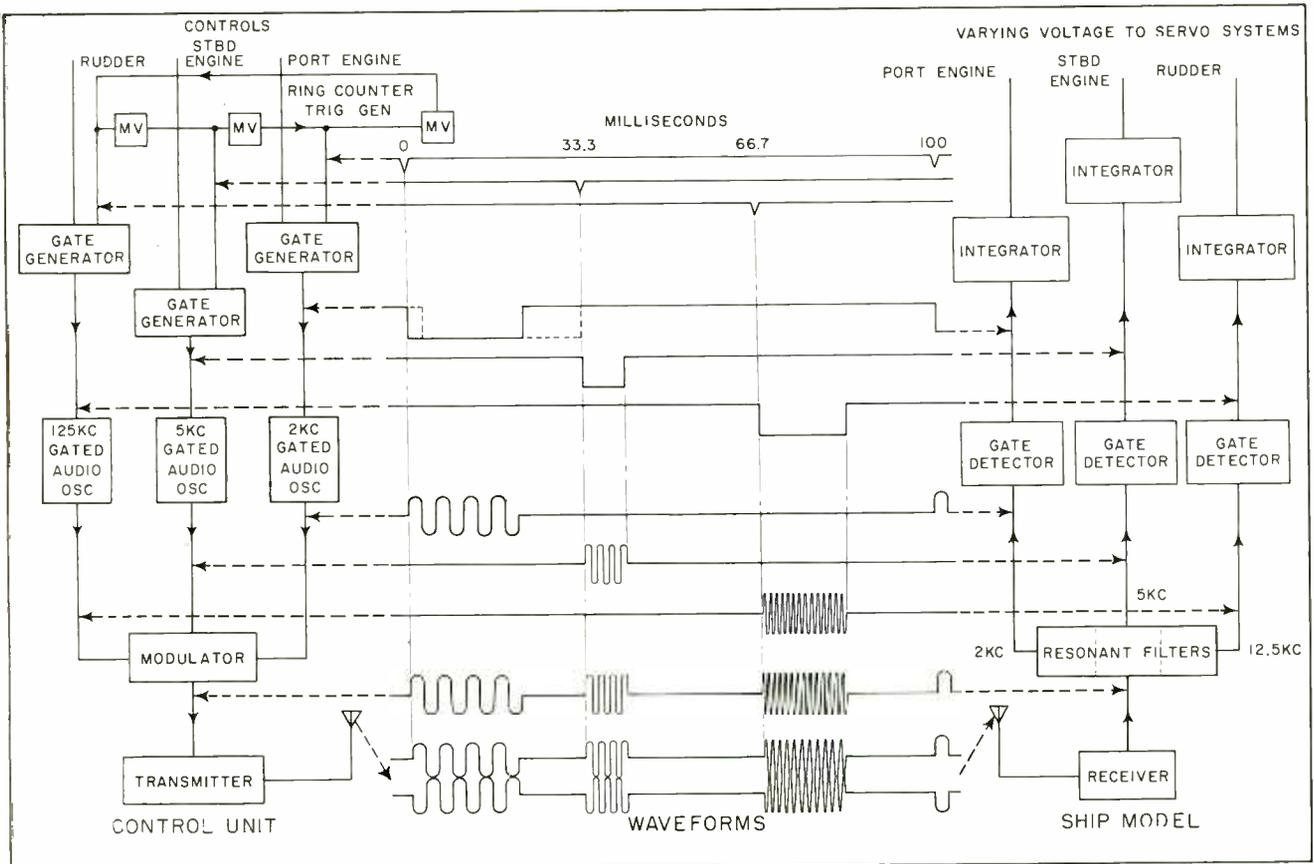
FIG. 1—Information transmission link of naval trainer showing waveforms. Control information is transmitted at 10 cps
