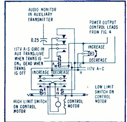
FIG. 5—Power output control and in-use alarm for auxiliary transmitter. Controls for regular transmitter are same except for omission of alarm
