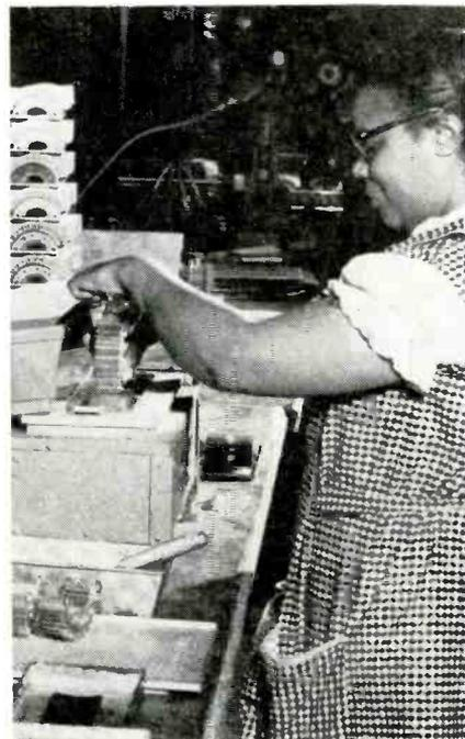
STEP 5—Tinning terminals in solder pot
