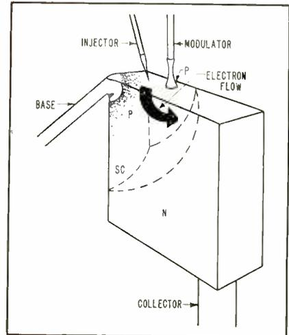
Fig. 1—Construction of present experimental spacistors
