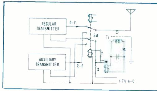
FIG. 2—Simplified automatic antenna shift circuit. Loss of antenna current makes relay drop out, thereby energizing switch solenoid for transferring antenna and power to auxiliary transmitter
