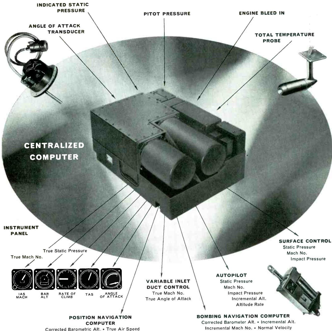
All illustrated components are designed, developed and manufactured by AiResearch
