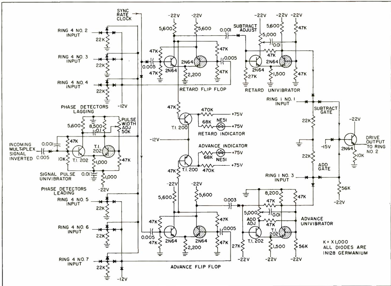
FIG. 8—Synchronizer circuit compensates for effects of oscillator drift and long-term signal distortion resulting from multipath radio transmission
