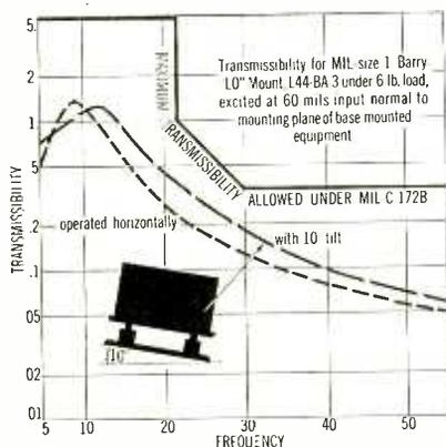
This low transmissibility — below 2 at resonance in all load ranges — is a major advantage of the Model L44 isolator. It accommodates high-amplitude inputs, even at resonance, without snubbing. Typical isolation at 10° inclination is also shown above.
