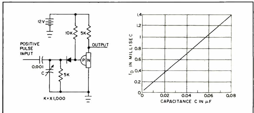
FIG. 7—Experimental delayed pulse generator and delay characteristics. Transistor used is similar to 4JD5A1
