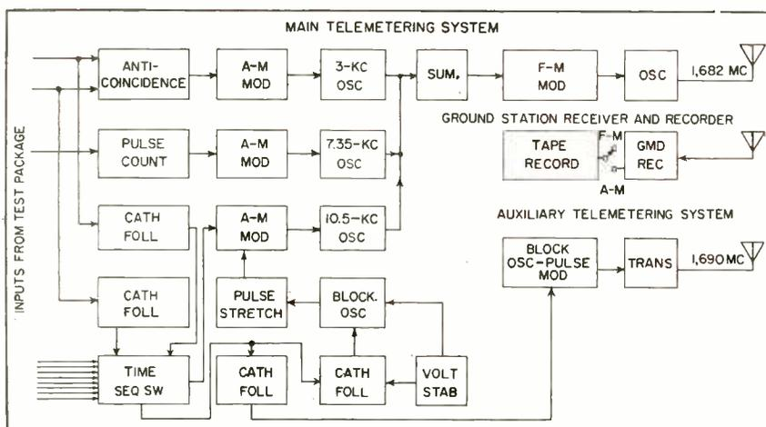
FIG. 1—Block representation of main telemetering system and auxiliary equipment
