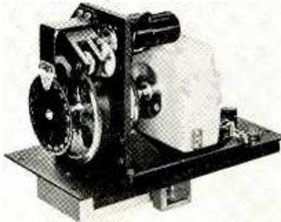
and the encoder shaft is driven  $\pm 170$  deg from null. Full scale corresponds to 10 v rms 400 cps, in phase with the line. The static error is 0.15 percent of full scale, and fast rates can be followed with a velocity error constant of  $500\text{ sec}^{-1}$ .
