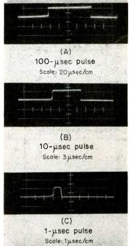
FIG. 4—Output pulse shapes of the delay multivibrator are shown for widths of 1, 10 and 100  $\mu$ sec at 4.2-v amplitudes
