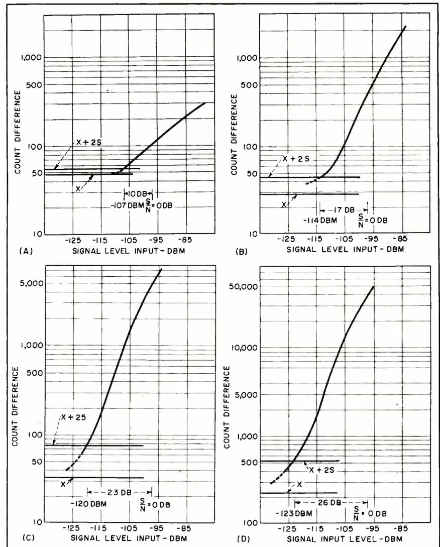
FIG. 5—Sensitivity for 0.1-sec (A), 1.0-sec (B), 10-sec (C) and 100-sec (D) samples. Slight inequalities in switching cycle tend to make count difference negative, so a constant value X is added to each quantity in order to permit positive plotting on the logarithmic scale
