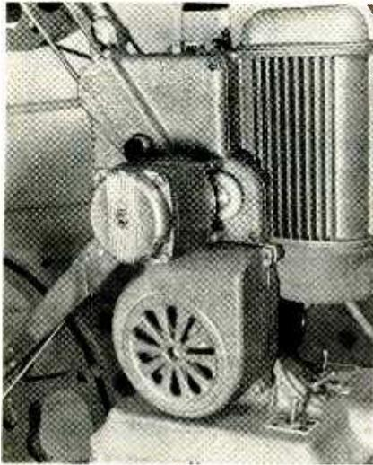
Control motor coupled to projector drive
