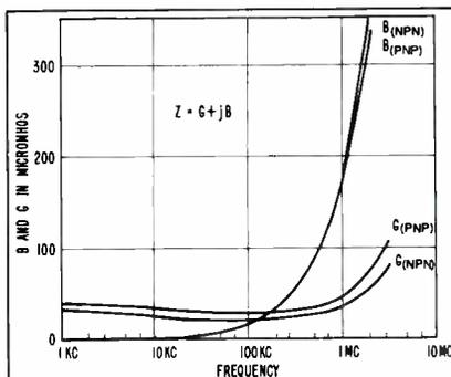
FIG. 5—Output impedances of two transistors
