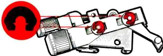
**LOCKING PRONG RINGS PERMIT SIMPLE DESIGN.** Shift slide assembly uses two Truarc series 5139 bowed locking prong rings to lock the parts together in a sliding fit. Precise amount of spring tension prevents objectionable wobble and noise, permits the key to slide smoothly in operation. Easy radial assembly and disassembly of rings facilitates field maintenance and repair. Alternative construction would have required cut washer, spring washer and hairpin-type spring clip on each stud.
