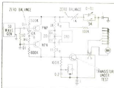
FIG. 3—Circuit with transistor complementary symmetry
