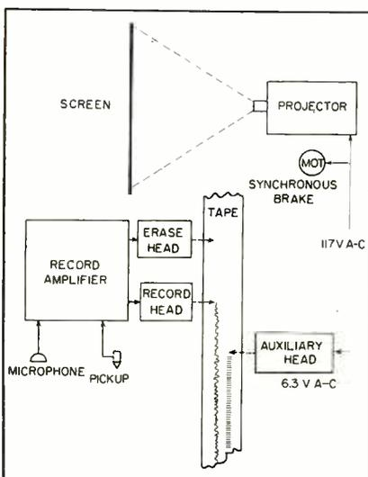
FIG. 1—Stepped-down projector voltage supplies sync signal during recording
