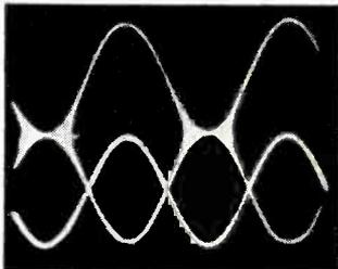
Test Oscillogram 320 kc Carrier modulated at 400 cps—audio source on lower trace shows fidelity.
