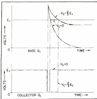
FIG. 8—Effect of change in return voltage on pulse width
