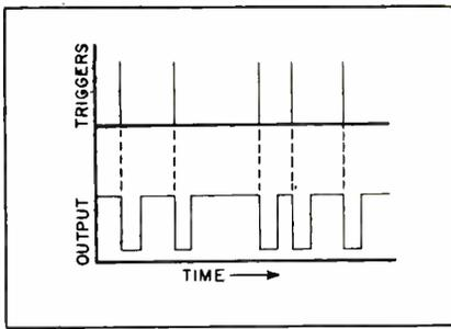
FIG. 5—Input and output of circuit of Fig. 1 for monostable operation
