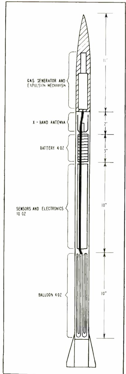
FIG. 1—Telemetering missile is 40 in. long, 1 $\frac{3}{8}$  in. outside diameter and weighs 6.3 lbs. About 26 cu in. is for electronics
