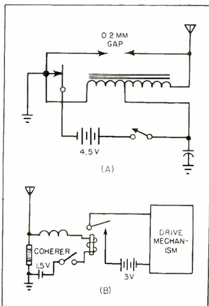
Fig. 1—Schematic of transmitter (A) and receiver housed in bus (B)
