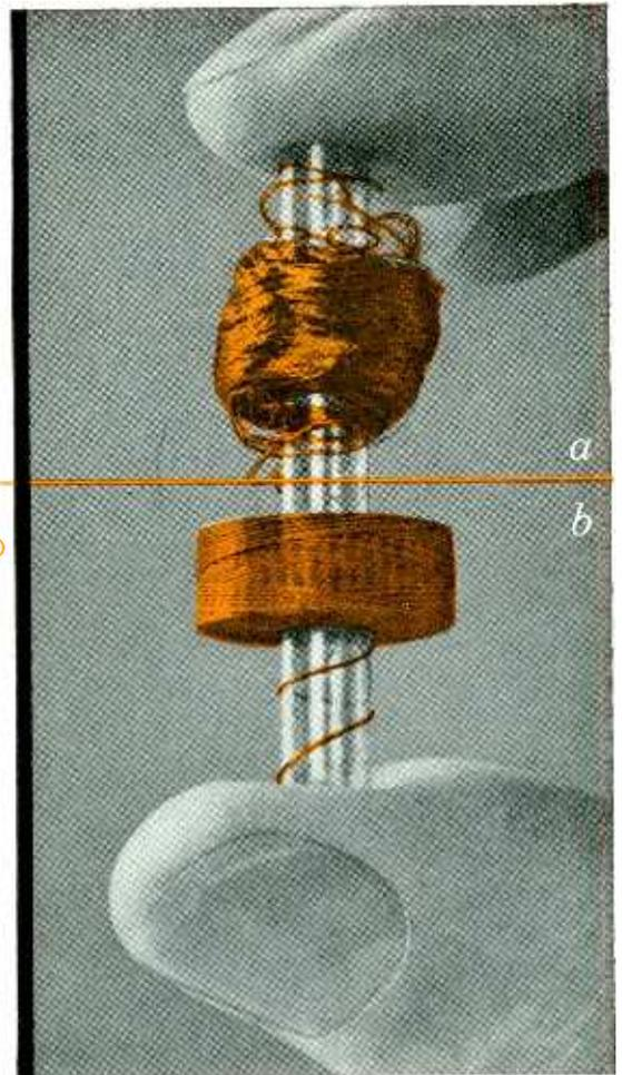
**THE PROBLEM:** To develop a solderable film-coated wire without fabric for winding universal lattice-wound coils without adhesive application.
