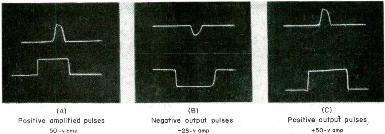
FIG. 6—Amplifier output waveforms (A) for 1 and 10- $\mu$ sec pulses. Negative (B) and positive (C) output pulses from the bases of the emitter followers  $Q_{10}$  and  $Q_8$  respectively
