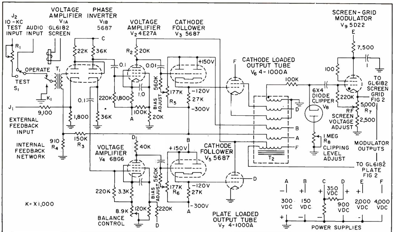
FIG. 3—The modulator has a cathode-loaded output tube,  $V_6$ , and plate loaded output tube,  $V_7$ . The grids of these tubes are driven push-pull at 180 degrees difference but plates are in phase
