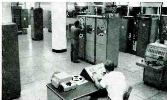
Four of the twenty-four Ampex FR-100 Tape Transports at the General Electric Missile and Ordnance Systems Department facility in Philadelphia.
