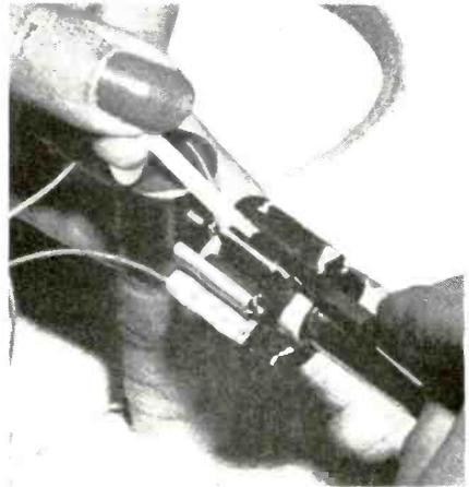
Pushing insulating wedge into slot
