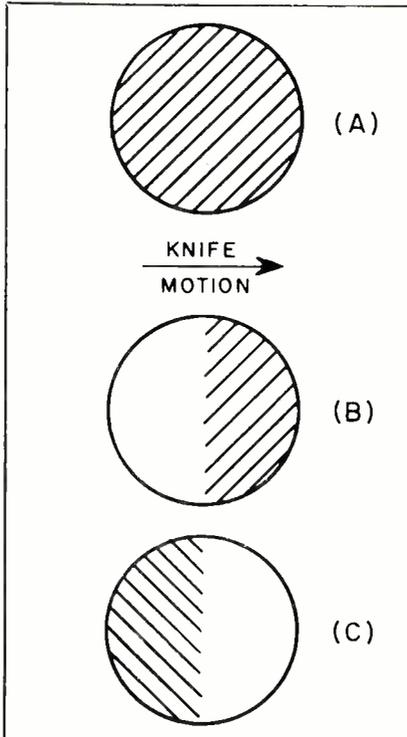
FIG. 2—Focus is at off where uniform diminution of illumination is obtained
