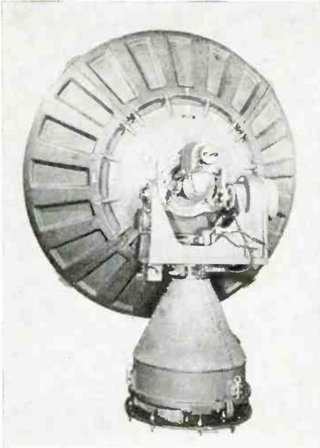
Lightweight, ground-based, air-transportable tracking antenna pedestal for mounting 8-ft. diameter, s-band segmented parabolic reflector and nutating scanner; highly accurate 2-speed data systems in elevation and azimuth.
