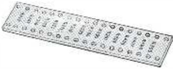
**Terminal board** for a complex circuit in an electronic spectrophotometer is made of Taylor Grade LE laminate . . . selected for its insulating and mechanical properties.
