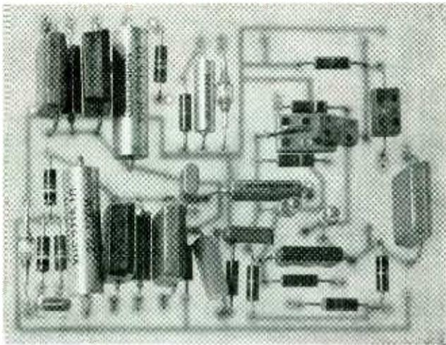
Repetition-rate generator and time-delay circuits excluding controls. Back-lighting shows the printed circuitry
