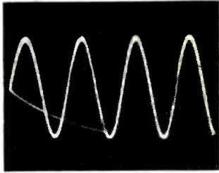
Test Oscillogram 15 kc Unmodulated Carrier showing good waveform.
