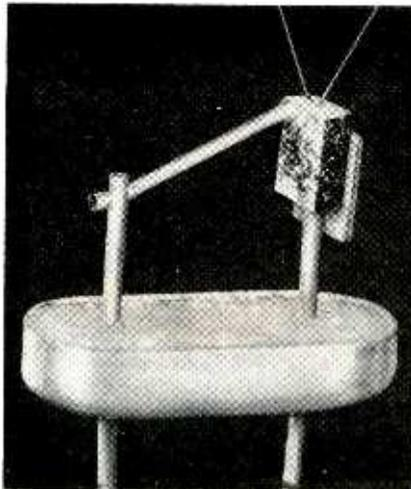
Extreme closeup of experimental spacistor assembly on transistor mount
