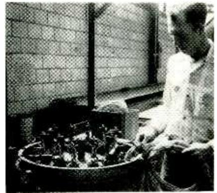
STEP 11—Pressurizing test barrel used for testing feed-through bushings at pressures up to 15 psi
