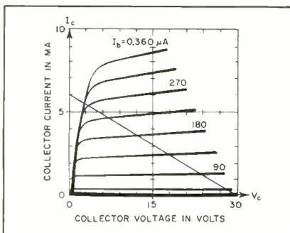
FIG. 3—Common-emitter characteristics
