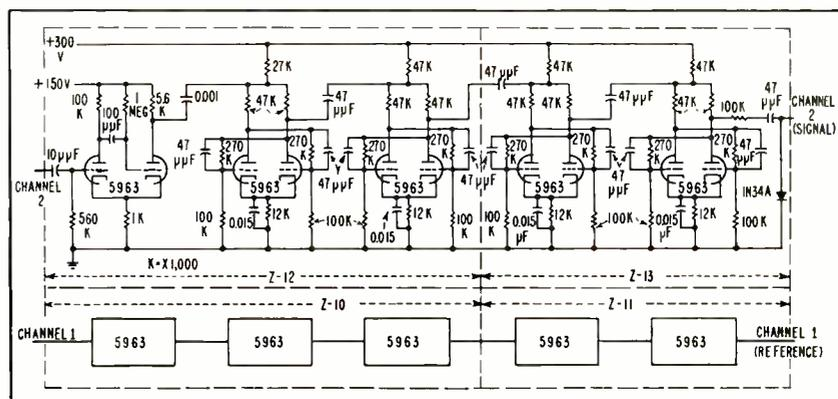
FIG. 4—Schematic of counters following integrator. Channels 1 and 2 are identical
