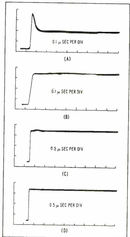
Fig. 3—Waveforms showing operation of attenuator-equalizer. Final response of the system is seen in Fig. 1E and Fig. 3D to different scales
