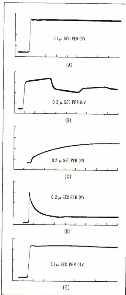
FIG. 1—Significant waveforms on scope with 12 μsec rise time
