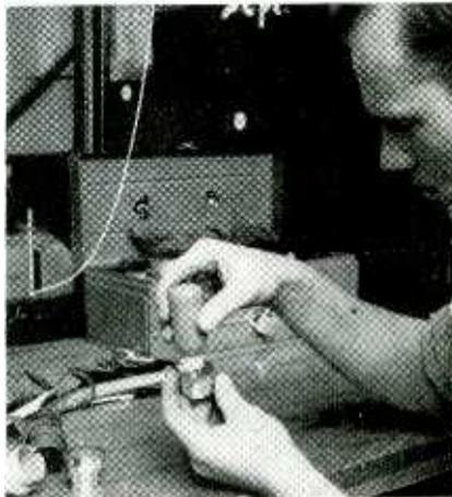
**STEP 4**—Filling holes in split-back shells with potting compound in squeeze bottle
