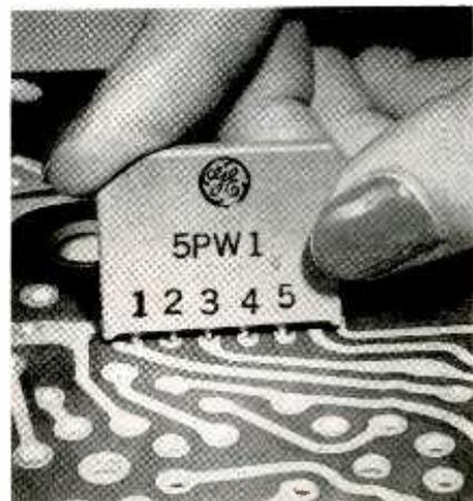
Manual placement in plated wiring board. Molded projections on phenolic housing keep unit above board so solder can form fillets around leads on top of board
