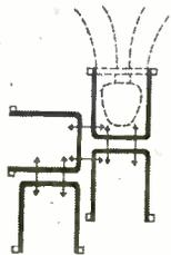
The 'U' mounting bracket of the Model CLH is specially designed to link two or more projectors into any configuration, achieving *exactly* the sound distribution pattern required. Even diagonal or alternating projections are just as easy to achieve as "standard" patterns.
