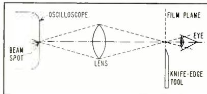
FIG. 1—Foucault knife-edge test requires a point source of light
