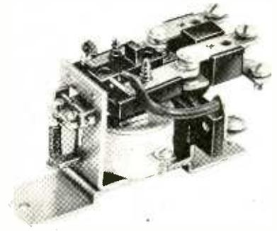
at 20 amperes, 115 v 60 cycle a-c or 24 v d-c, are single-and-double pole, single-and-double throw. Mounting arrangements are provided for auxiliary spdt contacts if desired. The relay is 2 1/8 in. high with a base measuring 1 in. by 3 3/8 in.
