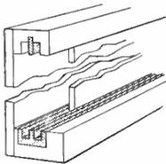
**Guides for sliding doors**, made from Taylor vulcanized fibre, last longer because of high strength and resistance to abrasion.
