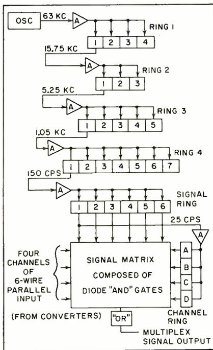
FIG. 6—Transmitting terminal frequency dividers and multiplexer
