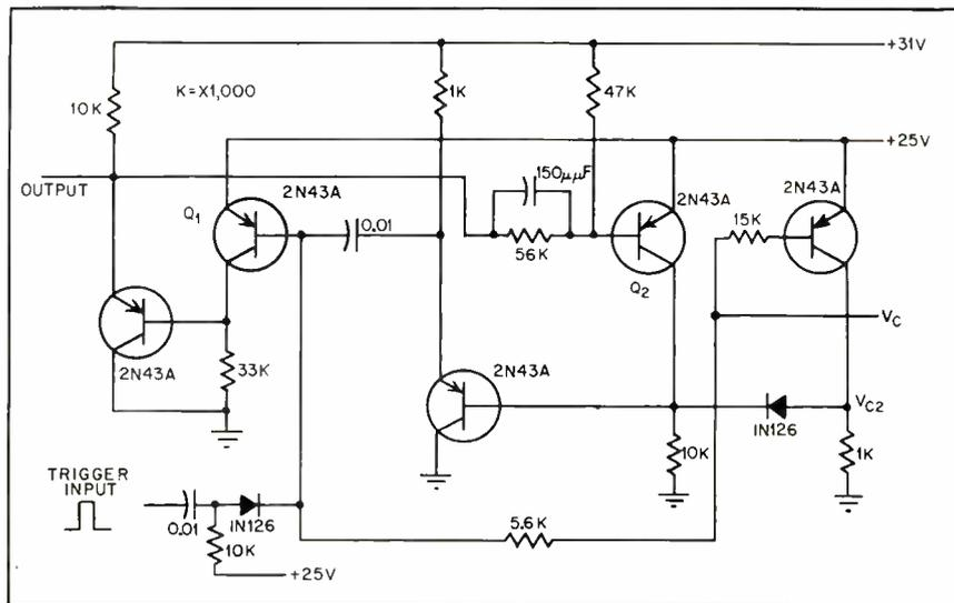
FIG. 10—Variable pulse-width monostable multivibrator with compound control
