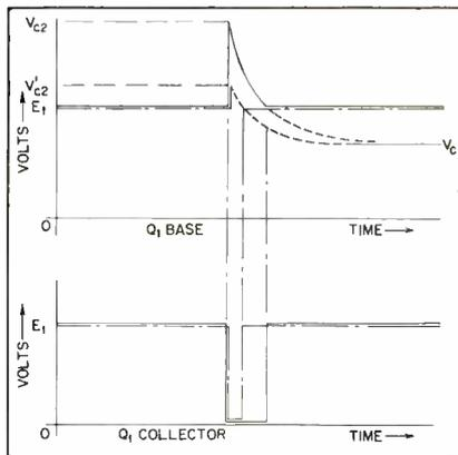
FIG. 9—Effect of change of  $Q_2$  collector clamp voltage on pulse width
