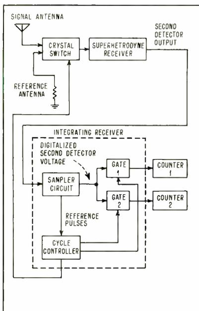
FIG. 1—Block diagram of complete system
