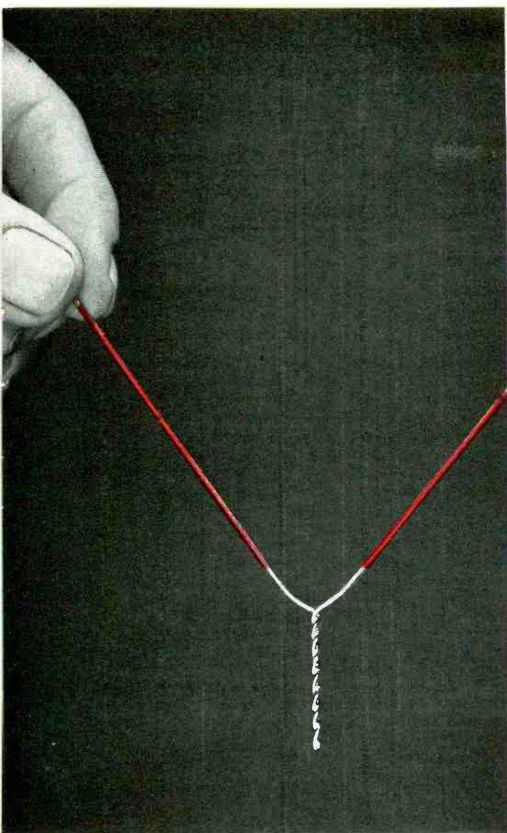
**JOINT IS COMPLETED WITHOUT STRIPPING WIRE** with Analac wire dipped in a 50-50 tin-lead solder at 360°C (680°F). The insulation is removed at the temperature of molten solder.
