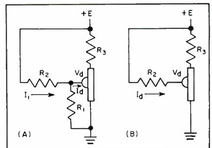
FIG. 2—Direct-current (A) and steady-state (B) equivalent circuits
