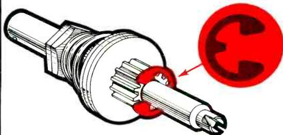
**E-RING SECURES PARTS AGAINST SPRING THRUST.** Slip clutch assembly uses Truarc series 5133 E-ring to hold parts on shaft. Functioning of the assembly is dependent upon the ring's ability to withstand thrust exerted by the heavy barrel spring.
