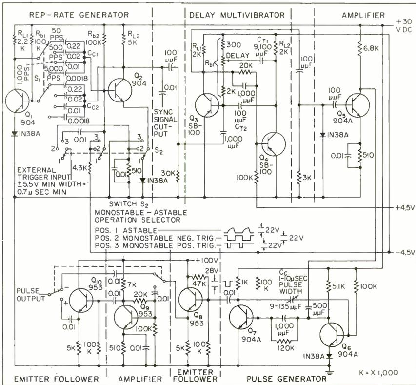
FIG. 2—Pulse generator circuit uses 904 junction transistors and produces pulses with amplitude of 100-v width, continuously variable from 0.1 to 10  $\mu$ sec
