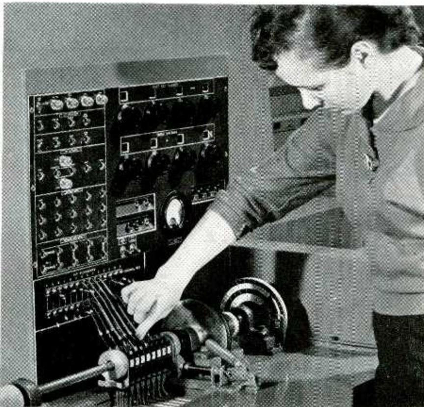
Making clip corrections to eight-cup ganged potentiometer in preparation for completely automatic card-programmed testing. Lamps give go and no-go indications
