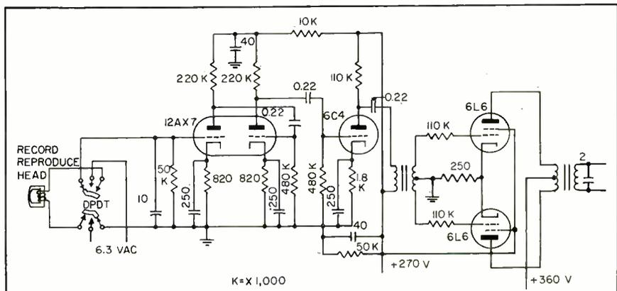
FIG. 4—Circuit of synchronizing amplifier. Resistors in push-pull grids provide voltage limiting, and capacitors across input and output resonate head and motor
