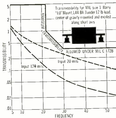
of center-of-gravity of the equipment. The natural frequency of the system shown above is below 5 cps.
