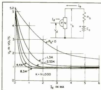
FIG. 4—Characteristics of experimental transistor similar to 4JD55A1
