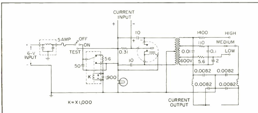
FIG. 2—Signal generator of cable detector. A range of output impedance allows matching the cable under test to provide maximum signal current
