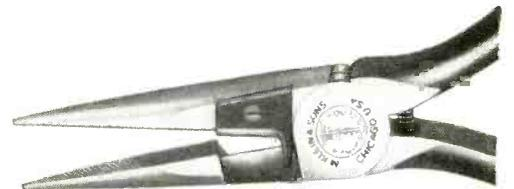
208-6C long nose shear cutting plier. A 6 1/2-inch long nose plier with shear blades. Will cut dead soft or extremely hard wire. Blade replaceable. Plier never needs sharpening. Point of nose 1/16-inch diameter. Coil spring keeps jaws open ready for use.
