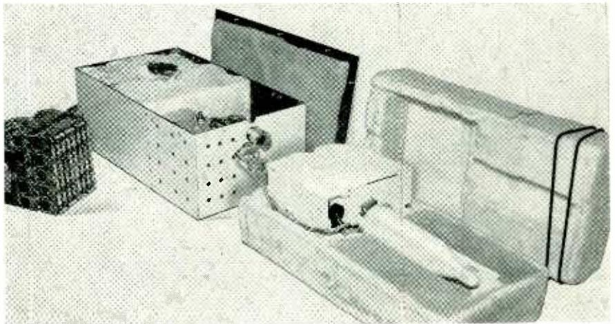
Complete balloon-carried telemetering system has subcarrier oscillators and transmitter embedded in foamed plastic shell for protection against rough launchings and landings
