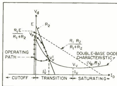
FIG. 3—Graphical load-line analysis of unijunction transistor characteristics
