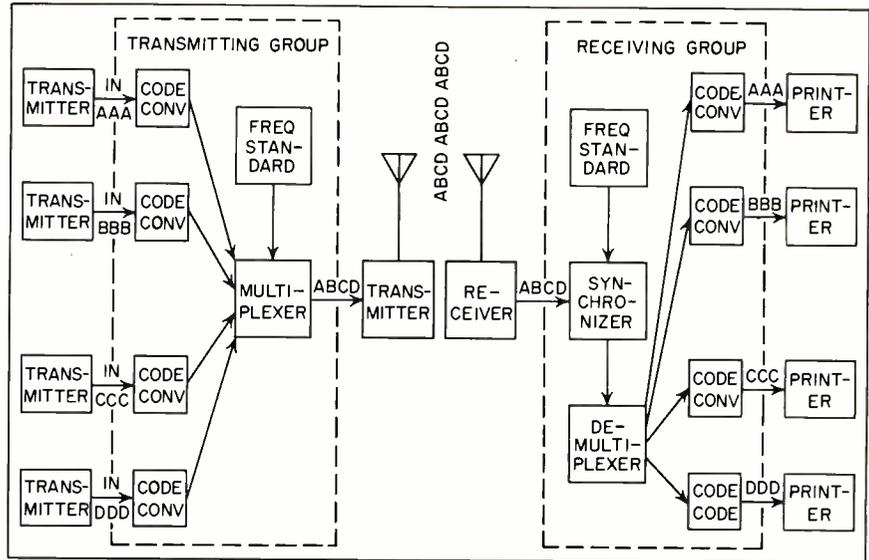
FIG. 5—Complete new multiplex system
