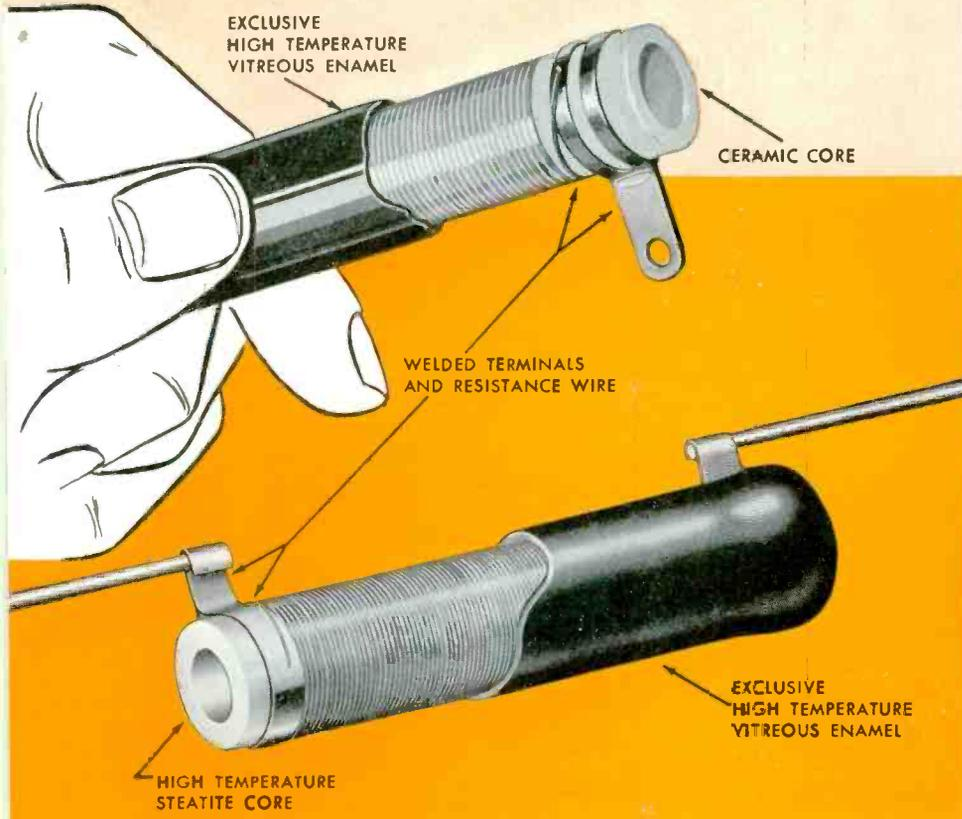
**WELDED RESISTANCE WIRE** Ohmite Resistors have the resistance wire welded to the terminals instead of soldered or brazed. This provides a perfect and permanently stable electrical connection that is unaffected by vibration or high temperature.
