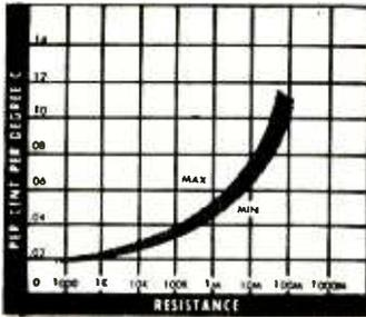
Typical temperature coefficient characteristics
