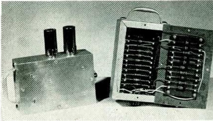
Typical modules, with side removed showing internal construction and wiring method
