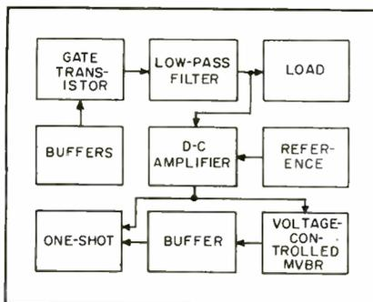
FIG. 1—Block diagram of regulator
