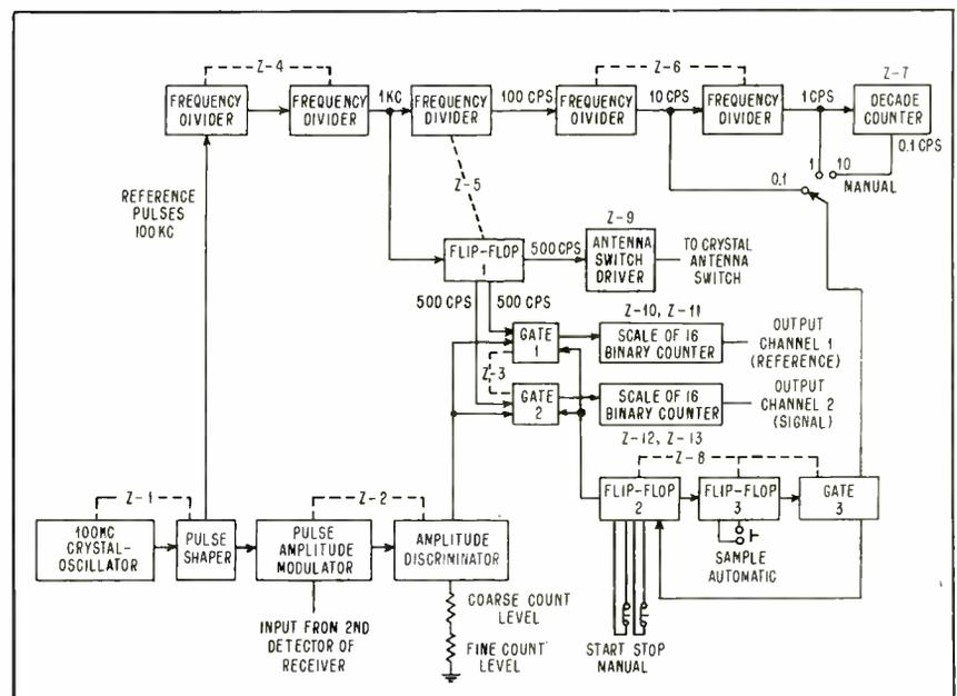
FIG. 2—Detailed block diagram of integrating receiver functions outlined in Fig. 1
