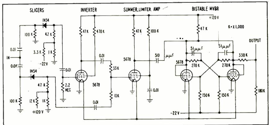
FIG. 7—Pulse counter uses biased limiters and bistable multivibrator to count randomly occurring pulses of either polarity and of 0.5 to several  $\mu$ sec width
