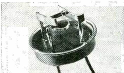
View of uncapped G-E silicon NPN diffused-meltback transistor, showing mounted silicon bar with aluminum base lead connected. Bar ends attached using a gold-alloy mounting technique. No solders or fluxes are used.
