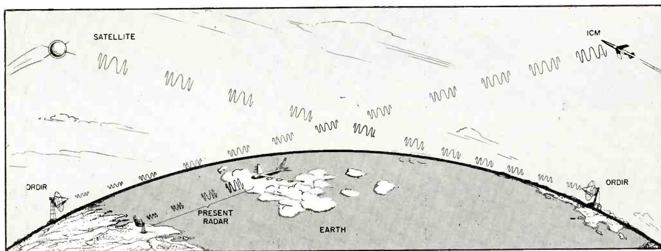
**ORDIR**, for OmniRange Digital Radar, is the name given a new radar technique using f-m that is also applicable to pulsed systems and may be applied to radar system engineering as . . .
