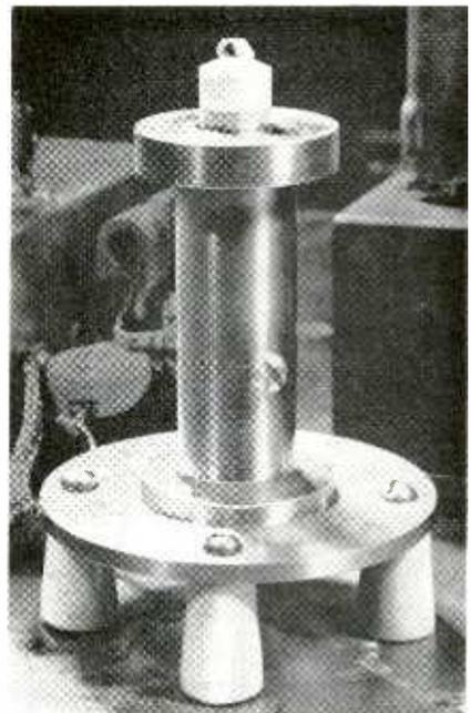
Diamond specimen to be measured in place on top fused-silica buffer rod. Quartz transducer is at lower end of rod.
