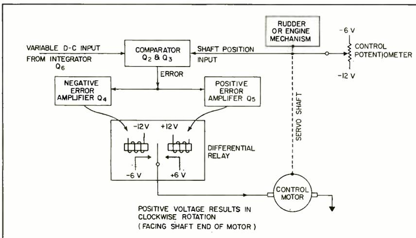
FIG. 6—Servo system in ship models. Relay-type servo achieves proportional control
