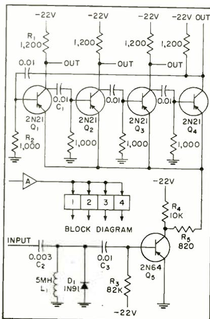
FIG. 1—Ring counter and drive amplifier
