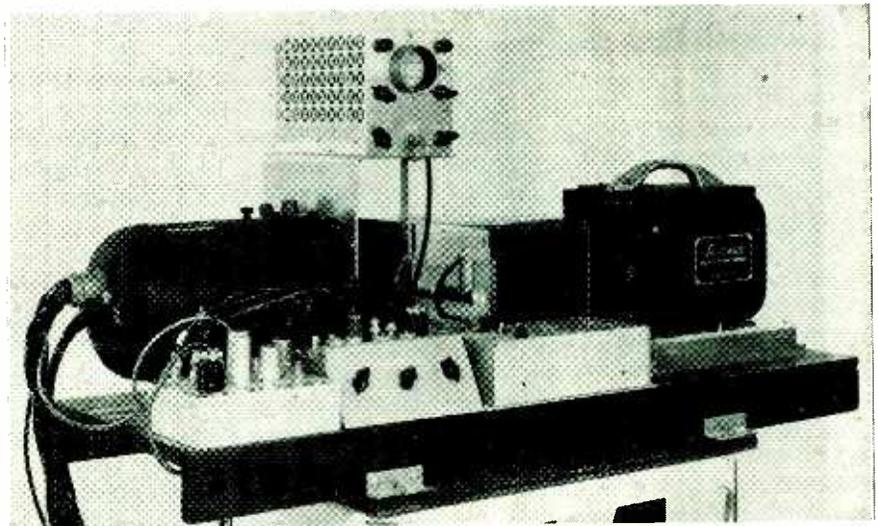
Breadboard model of the airborne recording unit employs an indicator from the AN/APS-23 radar unit
