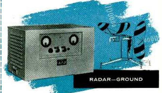
Hundreds of Perkin Ground Radar Systems are in operation throughout the country. Built to specifications MIL-E-4158, this unit was conservatively designed and will operate at 150% load continuously without damage to the unit. Specifications are: AC Input-120/208V  $\pm 10\%$ , 3 phase, 60 cycle  $\pm 2$  CPS, 4 wire system; DC Output-24-32V @ 100 amps.; Regulation-  $\pm 1/2\%$  (for any combination of line and load changes); Ripple-1% RMS or less.
