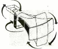
Horn bell rotates full 360° on its axis, while the 'U' mtg. bracket provides better than 180° vertical and 360° horizontal adjustment of projector positioning. Thus, sound can be distributed in any direction regardless of projector location.
