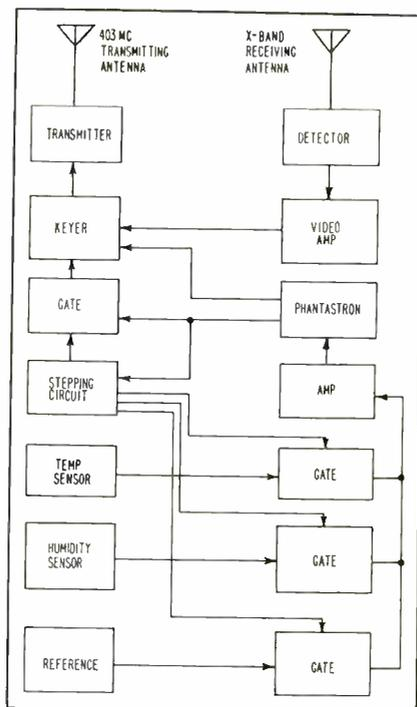
Fig. 2—Block diagram of system contained in DART missile
