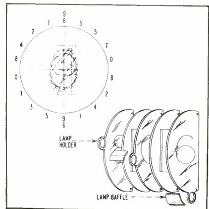
FIG. 2—Arrangement of lamps (top) and baffles alternating with plastic (bottom)
