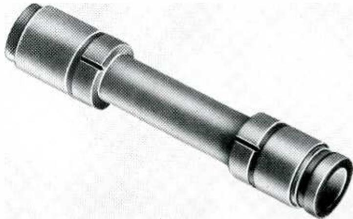
This coil form for radio frequency transformers is fabricated by Taylor of Grade XX laminate plastic tubing for Collins Radio Co. The O.D. of the center section is held to a tolerance of  $.230" \pm .0005"$ . Material was chosen for its good electrical properties, dimensional stability and machineability.
