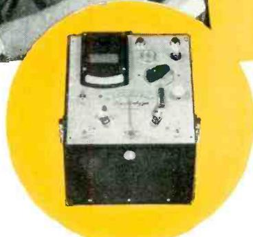
The Breathalyzer is an instrument for determining immediately the degree of alcoholic intoxication. This instrument is used widely by law enforcement agencies and Laboratories.
