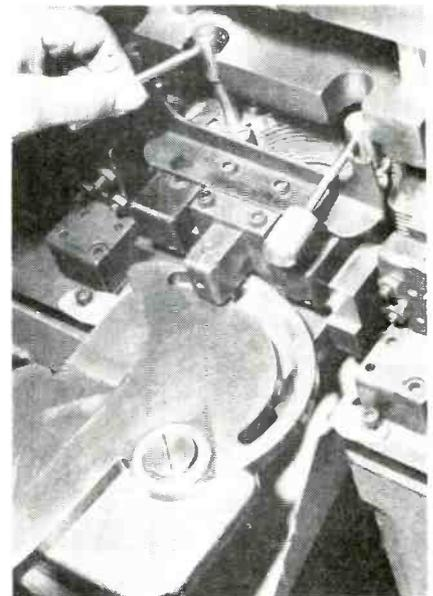
STEP 3—After shearing, operator removes positioning pins, then retracts slide
