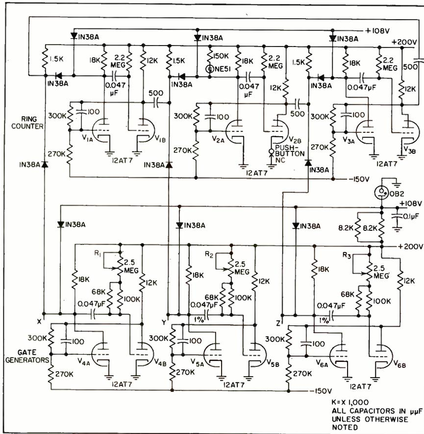
FIG. 2—Control unit of ship demonstrator showing ring counter and gate generators. A diode clamp returned to 108-v limits the plate voltage of the normally-off triode sections  $V_{1A}$ ,  $V_{2A}$  and  $V_{3A}$  and determines the initial amplitude of the timing waveforms
