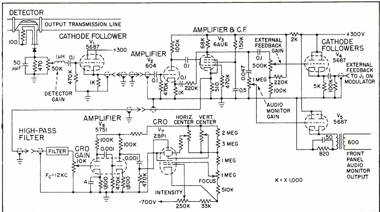
FIG. 4—Detector and amplifier reduce distortion and control phase shift. Output of  $V_4$  is external feedback that returns to the modulator. Output of  $V_5$  monitors the test
