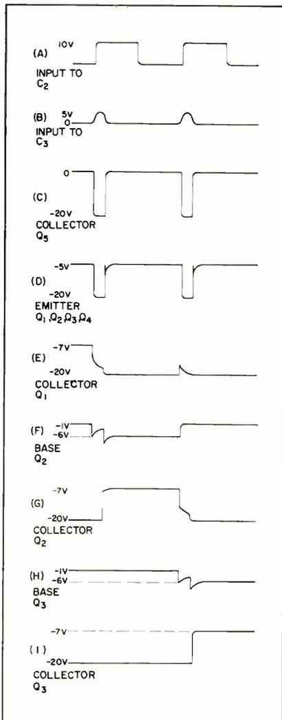
FIG. 4—Waveforms of ring counter
