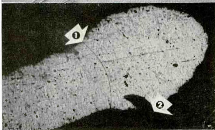
Before going through the diffused-meltback operation, a crystal of silicon is sawed into wafer-form: wafers are then diced to produce 4000 to 5000 individual silicon bars. Photomicrograph at left shows size-comparison of a silicon NPN bar, or pellet, with human hair (Arrow 2). "Tear drop" at end of bar is formed during meltback process. Micro-thin base, or "P", region (Arrow 1) is created through G-E diffusion technique. Base regions of 2-micron size are made with relative ease.
