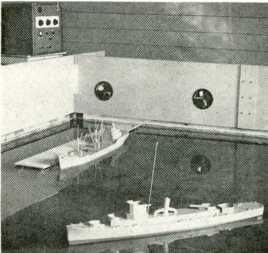
Control unit on table, upper left, has three knobs which control the cargo-vessel model beside the pier and the destroyer-escort model in foreground. Fans and ductwork are seen around the tank
