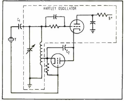
FIG. 3—Modified Hartley oscillator circuit
