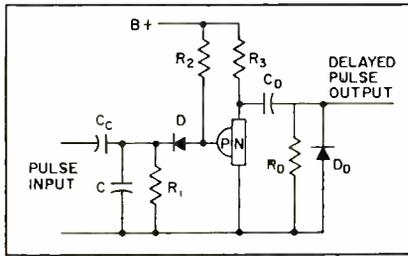
FIG. 6—Basic delayed-pulse generator
