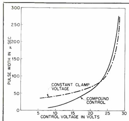
FIG. 11—Operating characteristics of multivibrator of Fig. 10
