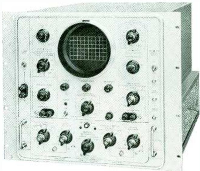
**High Frequency Rack Mount Oscilloscope, Model 150AR.** Same as *-hp-* 150A except for mounting in standard relay rack. Fitted with "pull-out" slides for maximum servicing accessibility. \$1,200.00.
