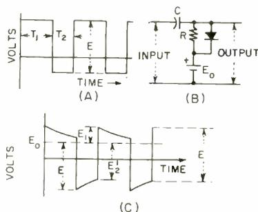
**FIG. 1—Input with arbitrary d-c level (A) to diode clamp circuit (B) and output (C)**
