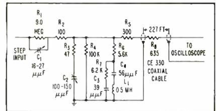
**FIG. 2—Total cable resistances of 350 to 700 ohms may be used, but cables between 400 and 500 ohms perform best**
