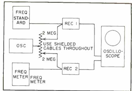
Arrangement of the calibrating equipment
