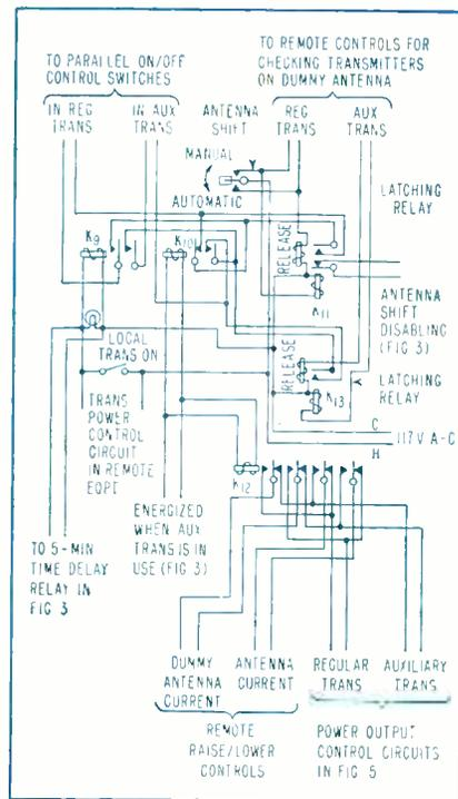
FIG. 4—Fail-safe controls for regular and auxiliary transmitters, with provisions for overriding automatic control when required
