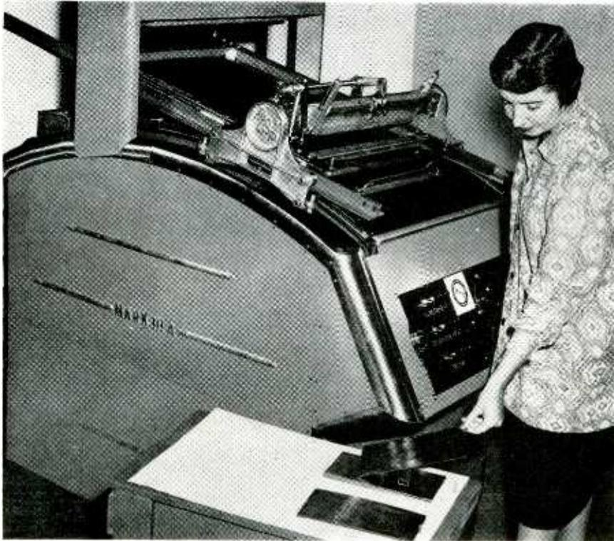
Mechanized squeegee forces molten thermoplastic resist through stainless steel cloth screen, which may be either 180 or 230 mesh depending on detail required
