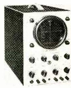
**5" OSCILLOSCOPE WO-88A**—An all-purpose scope for general lab use, production-line alignment and testing. Built-in voltage calibrating facilities permit simultaneous waveshape display and peak-to-peak voltage measurements. Sync polarity instantly reversible with front panel switch. Directly coupled, push-pull amplifiers in vertical circuit provide flat response down to dc. User Price **\$179.50\***
