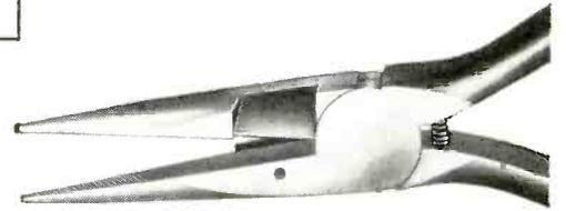
208-6NC. Similar in design to 208-6C but reverse side designed to put a positive 3/16-inch hook on the end of a resistor wire. Smooth one-motion operation saves production time on every television or radio set.
