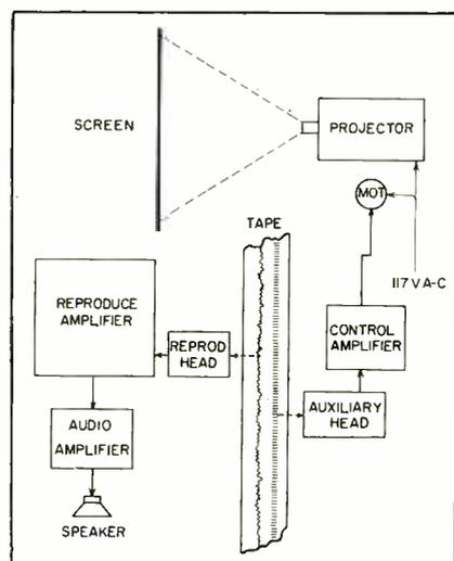
FIG. 2—Amplified control signal holds picture to sound speed during screening
