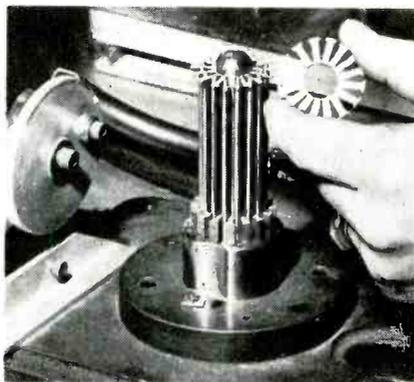
Method of loading laminations on fixture. About half an inch of stack in position
