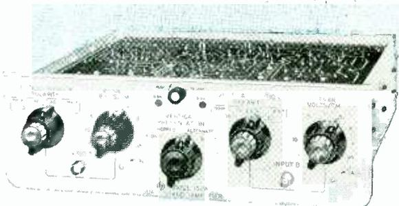
**Dual Channel Amplifier, Model 152A.** Designed for plug-in use with *-hp-* 150A or 150AR Oscilloscopes. Permits two phenomena to be presented on CRT simultaneously. Either amplifier usable separately. For dual presentation, electronic switch applies outputs to alternate traces, or switches outputs at a 100 KC rate. 50 mv/cm sensitivity, 9 ranges, 1, 2, 5, 10 sequence. \$250.00.
