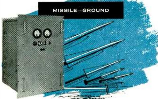
Perkin has developed Magnetic Amplifier Regulated DC Power Supplies for missile launching and check-out, with ratings of 30, 50, 100, 200, 300, 400, 500 amperes and above. The unit shown here is a 24-32V, DC @ 100 amp. unit, 19" rack panel mount, with a regulation of  $\pm 1/2\%$  over the range of 24-32 volts. There are provisions for remote operation and sensing. Perkin ground power supplies are now being used in the Thor, Atlas, Bomarc, Vanguard and other missile programs.
