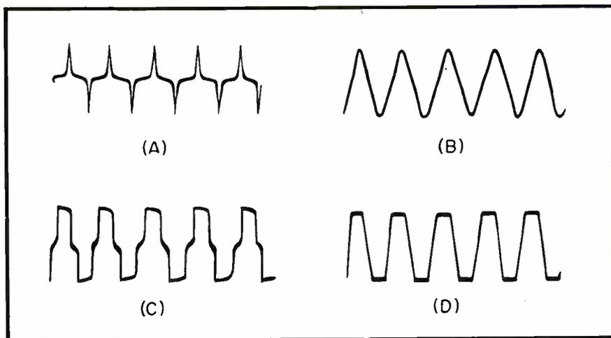
FIG. 3—Control-signal waveforms at output of auxiliary head (A), input to sync amplifier (B), output of amplifier after limiting (C) and input to motor (D)
