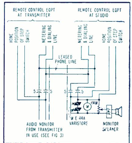
FIG. 6—Audio monitor is fed from transmitter to studio continuously over line used also for metering and dialing in remote control equipment. Varistors suppress dialing clicks from audio
