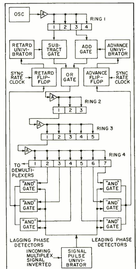
FIG. 7—Receiving terminal frequency dividers and synchronizer
