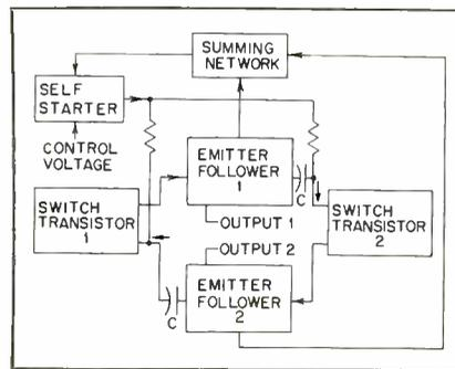
FIG. 2—Basic of monostable multivibrator
