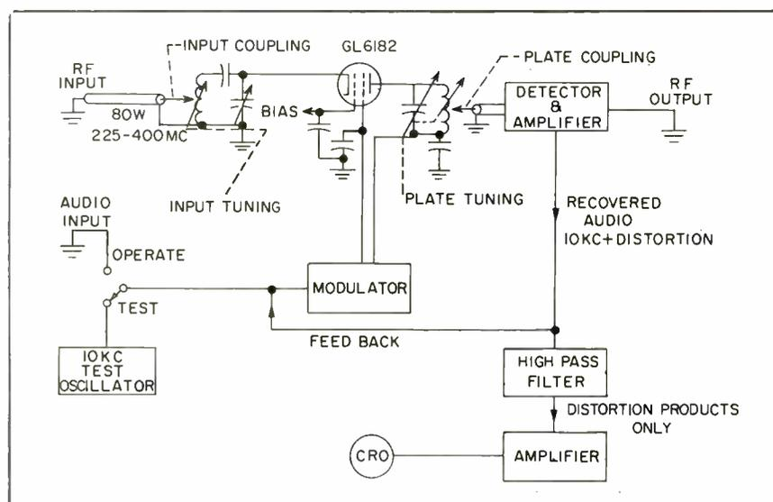
FIG. 1—Block diagram of the 1-kw high-level modulated uhf amplifier
