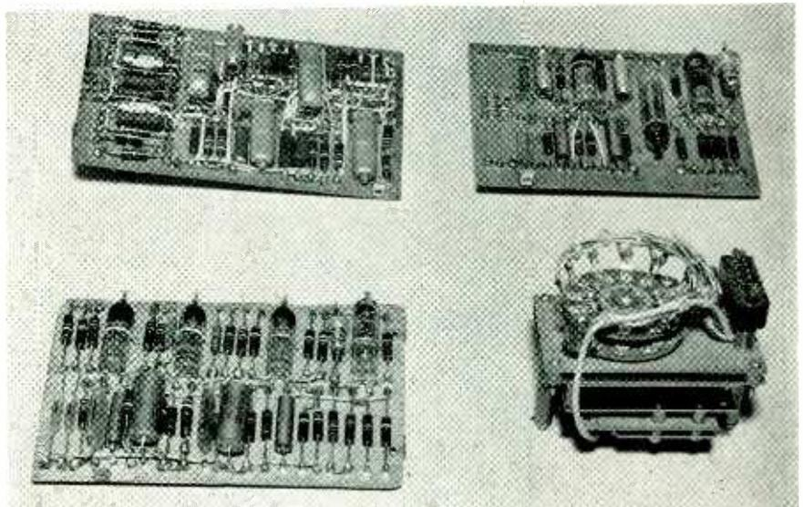
Measuring circuit subchassis include: pulse counter, upper left, cathode followers, upper right; anticoincidence circuit, lower left and sequence switch, lower right
