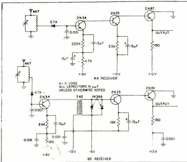
FIG. 4—Receivers in the ship models. In each receiver, a diode detector drives a high-gain three-stage transistor audio amplifier
