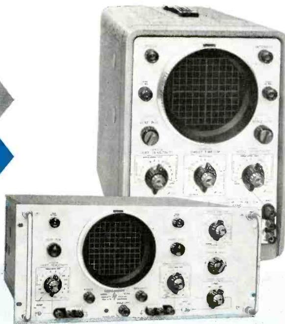
**Low Frequency Cabinet Oscilloscope, Model 130A.** Covers dc to 300 KC. Similar horizontal and vertical amplifiers. Input circuits balanced on 5 most sensitive ranges. Single ended input may be dc or ac coupled. Direct reading, linear sweep times. With most transducers, needs no preamplification to produce brilliant, high resolution trace. Universal automatic triggering; one preset condition provides optimum triggering for almost all inputs. \$650.00.
