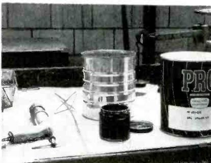
STEP 1—Preparing potting compound. After accelerator is added, whipper in slow-speed air motor is used to achieve thorough mixing
