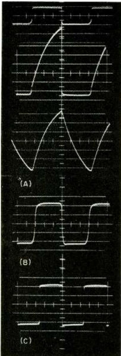
Waveforms for circuit of Fig. 1 operating as 10-kc astable mvbr (A); output waveforms for 55 kc (B) and 7 kc (C)
