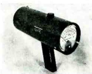
New Self-Calibrating Ion Chamber
