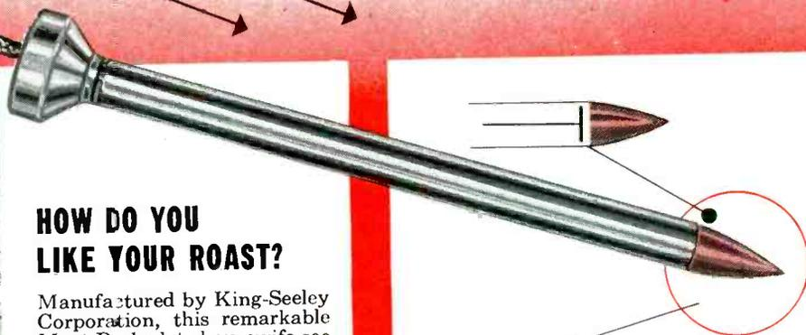
KEYSTONE NTC Thermistor in nose of stainless steel probe decreases in electrical resistance as temperature rises, permitting greater circuit current flow, thus actuating external temperature gauge. Circuit consists of regulated voltage supply with thermistor and gauge connected in series.
