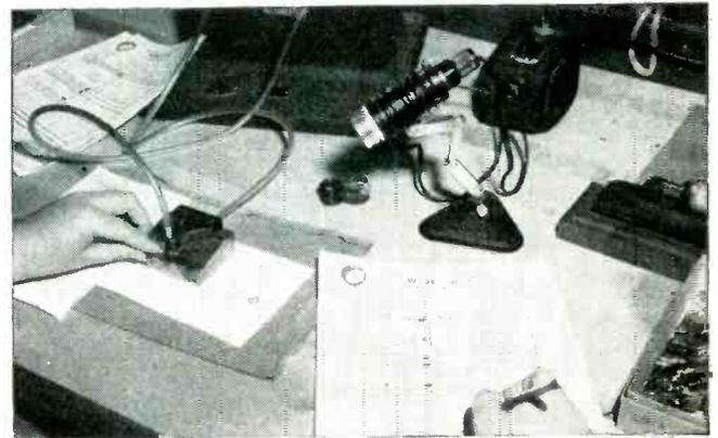
**4. CHECKING OF MECHANICAL DIMENSIONS.** Rigid quality control inspection standards assure constant checks on the finished cathode dimensions: length, diameter, bead position, etc. Must fall within close tolerances specified. The very latest precision measuring instruments are employed.
