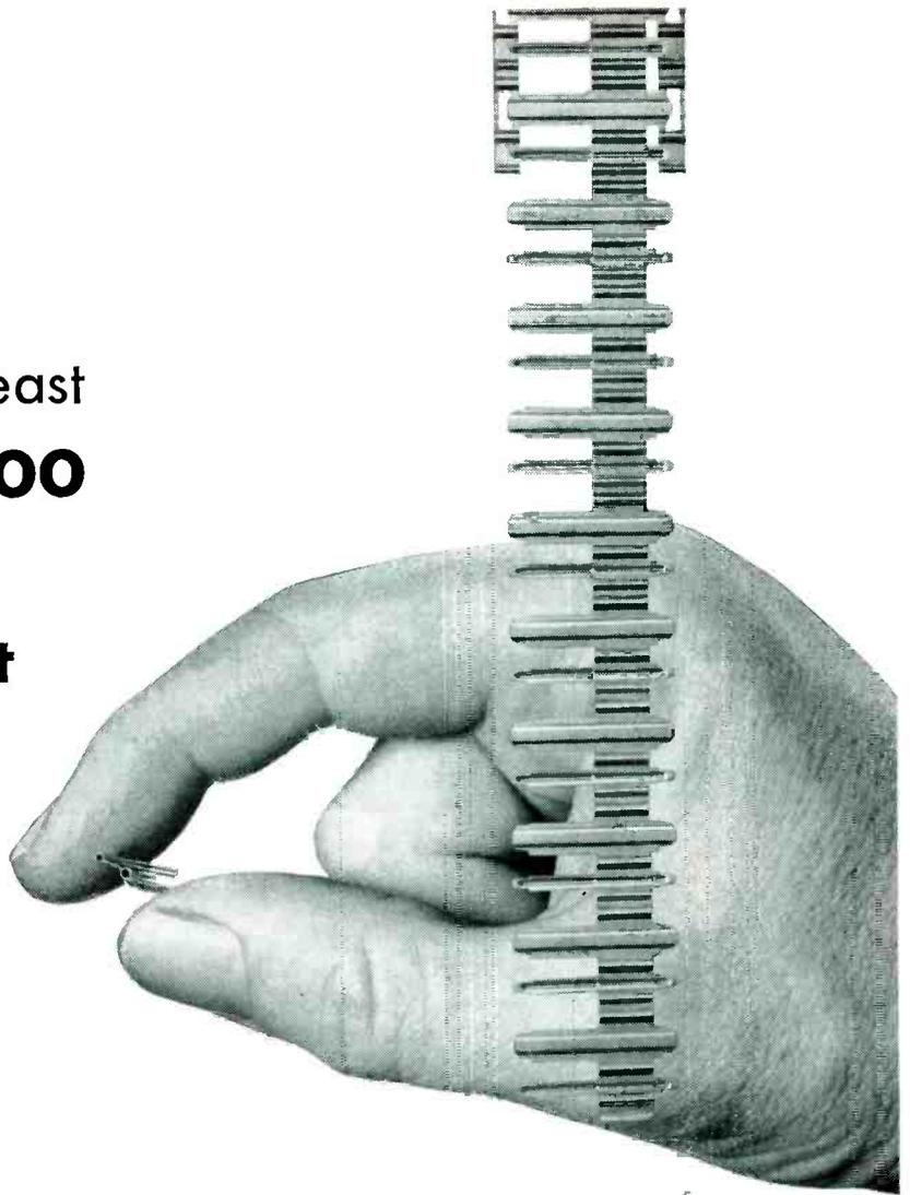
The diode plate shown above is an example of the complex, mass-produced, parts turned out to close tolerances by The Metal Stampings Plant, Sylvania Electric Products, Inc., at York, Pennsylvania. Tolerances run to  $\pm .001$ "; as many as 10 dimensions must be held, including inner and outer diameters. Yet even on parts more difficult than this—parts with tolerances of  $.0005$ " and forming rates of 9,000 per hour—Sylvania gets an acceptance rate of over 98%.
