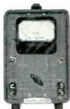
**-hp- 400AB**, for general ac measurements. Covers 10 cps to 600 KC, 0.3 mv to 300 v. Accuracy  $\pm 2\%$ , 20 cps to 100 KC. 10 megohm input impedance plus 25  $\mu\text{f}$  shunt insures circuits under test against disturbance. Readings direct in volts or dbm. \$200.00
