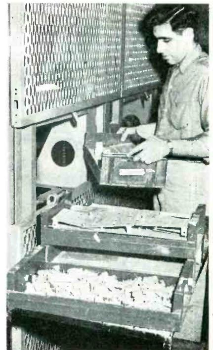
Transferring tote tray from storage machine to cart, for moving to work position. Tray design includes conical steel pegs for safe stacking and raised handles to protect parts when trays are stacked
