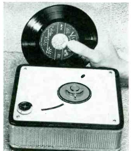
Japanese ingenuity is displayed in the transistor record player shown above. The pickup presses against the underside of the record, which is effectively locked onto the turntable. According to Sony engineers, the motor requires 50 and the amplifier only 15 milliamperes.
