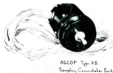
APPLIED SCIENCE CORP. OF PRINCETON, P. O. Box 44, Princeton, N. J. Type AB high speed sampling switch provides single pole sampling of 60 contacts at rates up to 30 rps. Only 3 oz.-in. torque is required. This compact switch is built to provide long life under
