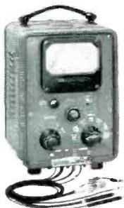
**-hp- 410B**, industry's standard for vhf-uhf voltage measurements. Wide range 20 cps to 700 MC, response flat within 1 db full range. Diode probe places 1.5  $\mu\text{f}$  capacity across circuit under test; this plus 10 megohm input impedance prevents disturbance. Instrument combines highest quality ac voltmeter with dc voltmeter (122 megohm input impedance) and ohmmeter covering 0.2 ohms to 500 megohms. \$245.00
