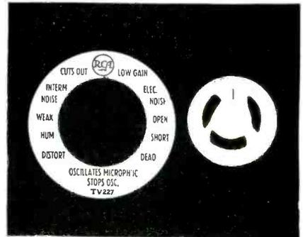
Examples of disks used for identifying tube faults. Smaller disk, for miniature tubes, is made at same time as large disk by punching the three holes in the otherwise wasted center area of the larger disk
