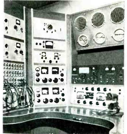
White House communications car the *General Albert J. Myer* was recently used by amateur radio station W3WTE to try out single sideband radiotelephone equipment of a type that may later be used for point-to-point service under the call WTE. Permanent antenna shown atop the car (left) is a capacitance-feed grid net-
