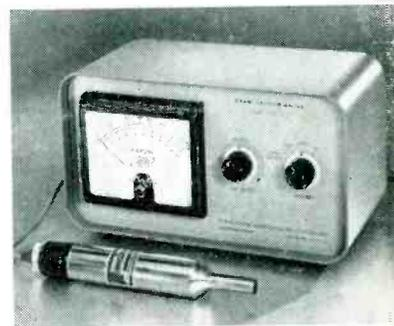
**A NEW Pirani Gauge.** Continuous, direct readings over entire 1 to 2000 microns range. Single and one to four station models. Automatic voltage regulation. High sensitivity with greatly reduced zero drift. Serves as leak detector up to 10mm Hg.
