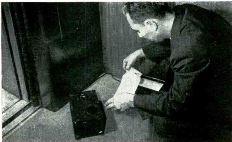
**"Mechanical stomach" for elevators.** Westinghouse makes sure that its elevators give you a smooth ride. Instrumentation consisting of an accelerometer and a Brush portable oscillograph is shown here on a "trial run". Recorded test data helps develop elevator controls that produce the best acceleration pattern for passenger comfort.
