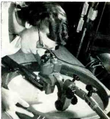
sequence blue, green and red, the face plate is inspected for alignment, using Mineralight or Black Light Eastern Corp. ultraviolet equipment and a microscope. The excited dot pattern shown in the cover insert is seen by the inspector.
