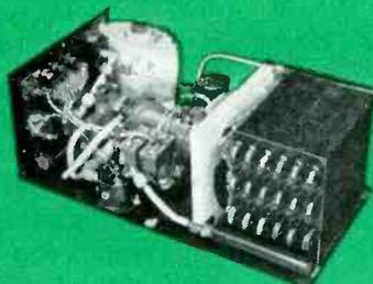
**MODEL MB-177, TYPE 202 DISSIPATION:** 1,700 watts. **ALTITUDE RANGE:** sea level to 50,000 feet. **POWER REQUIRED:** 110 volt, 400 cycle, 3 phase. **WEIGHT:** 27 pounds. **SIZE:** 10" x 19 15/32" x 7 3/8" high, per JAN-C-1720A, size 81-D1.
