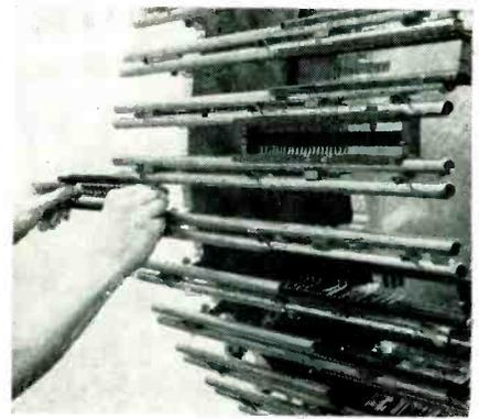
Loading component magazine onto rotating magazine carrier of machine
