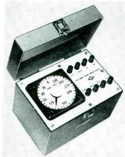
able phase angle meter which offers a direct way of checking relay and instrument connections, particularly directional over-current relays, differential relays or similar equipment. It may also be used to measure the prevailing power factor in each phase of a polyphase watt-hour meter installation.
