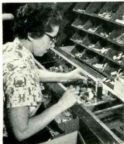
PACKAGED circuits are inserted in plated circuit boards at Motorola. Finished chassis, right, shows how
