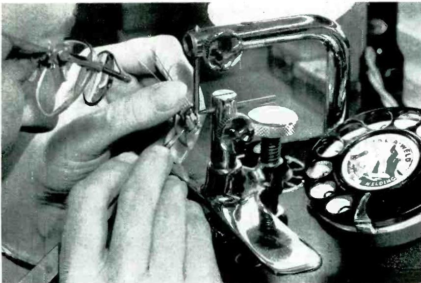
Welding relay coil lead to header wire with dental welder. Dial controls weld time
