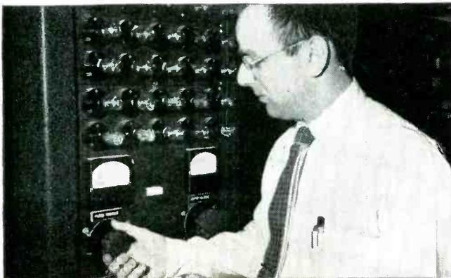
**3. TESTED IN ELECTRON TUBE.** Samples of each heat of Cathaloy are fabricated into cathodes and assembled into ASTM standard diodes. They are operated under controlled conditions. These tests evaluate each heat for emission and sublimation characteristics. Satisfactory results approve the heat for production.
