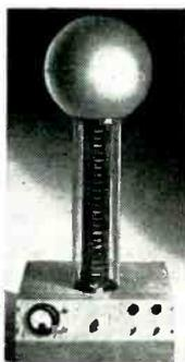
Generator with beam tube removed produces 1/2 million volts, 16-inch sparks for high-voltage experiments. With beam tube inserted, Rayotron produces diffuse high-energy X-ray beam for all basic X-ray experiments. Height 2 1/2 ft. Comes with manual of 8 fascinating experiments and newly published Accelerator Syllabus. Rayotron, complete with beam tube, \$295; Generator alone, \$175. Small fluoroscopic screen and X-ray film, \$20. Optional instrumentation, \$25.00.
