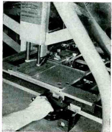
Trigger handle is bolted to table that holds master template (in foreground) and wiring board being loaded with components
