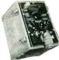
Covers 40-500 Mc in 2 ranges. Harmonics above 2000 Mc. A calibrated (dial accuracy ± 0.7%) I.F. source for testing receiving Output 3MW or more to 400 Mc, less on harmonics. C.W., mod. pulse or sine wave output. 115/230 60 Cy. or batteries. New with inst. book.
