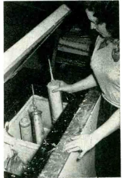
Method of storing dispensers in deep freezer. Some compound is placed in plastic bag as at left; this can be taken to an aircraft for filling plugs that are already in position. This is done by cutting off a tiny corner of the bag and then squeezing the bag to force out the compound
