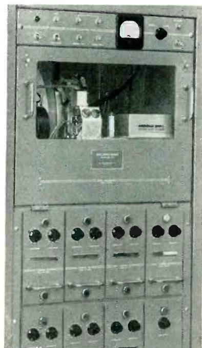
Truck-mounted seismic recorder contains seven dual-channel modulators
