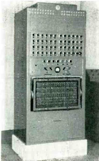
accessibility. Provision for 3 servo multipliers, or 3 electronic function generators, is also incorporated. An overall accuracy of 0.1 percent of full range from  $-100 \text{ v}$  to  $+100 \text{ v}$  is achieved. Color coding and labeling of the 800 jacks on both patch bay and problem board are identical. Programming may be carried out directly on the machine as well as on the removable boards.
