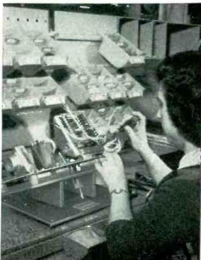
Method of using chassis-holding fixture during assembly of missile control
