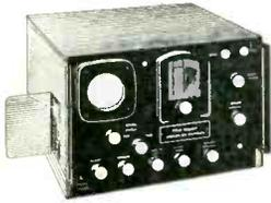
Field type X Band Spectrum Analyzer. Band 8430-9580 Megacycles. Will Check Frequency and Operation of various X Band equipment such as Radar Magnetrons, Klystrons, TR Boxes. It will also measure pulse width, c-w spectrum width and Q or resonant cavities. Will also check frequency of signal generators in the X band. Can also be used as frequency modulated Signal Generator etc. Available new complete with all accessories, in carrying case.
