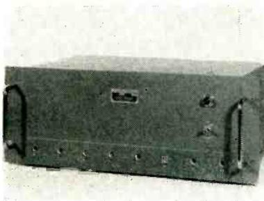
and a gain in each channel of nominally 2 db. Radiation suppression is greater than 60 db and isolation between any two receivers is greater than 55 db.
