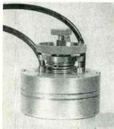
Micrometric screws on top of pressure gage assembly adjust position of balancing coil to compensate for static water pressure on hull
