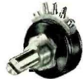
Precision wire-wound construction. Three watts continuous at 80° C. Resistances 10 to 50,000 ohms. Diameter 7/8 in., depth is 3/8 in. Weight is only 1/2 ounce. Independent linearity 3% standard.
