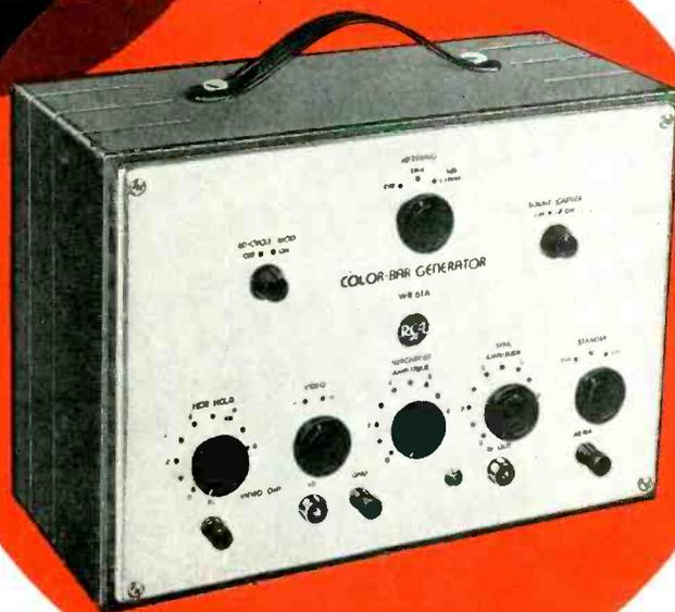
Additional features include: adjustable color subcarrier amplitude for checking color sync-lock action in receivers. Built-in metering circuit facilitates adjustment of relative amplitudes of subcarrier and horizontal sync. 300-ohm rf output. Both high- and low-impedance video output with "plus" and "minus" polarity selector.
