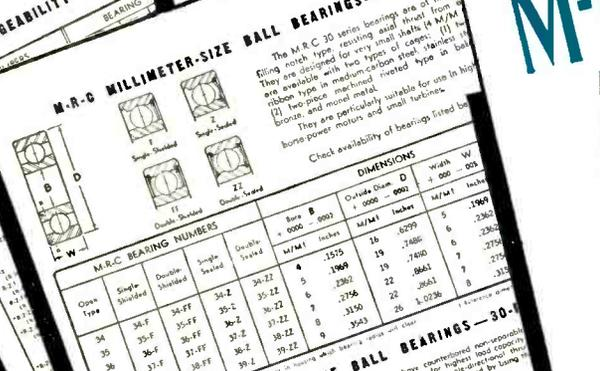
**M-R-C MILLIMETER-SIZE BALL BEARINGS—30 SERIES**
