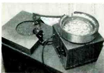
Jigging designs available to accommodate practically any electronic component to be tested and sorted by the Auto-Bridge. Application shown is sorting disc ceramic capacitors.
