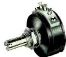
Four watts continuous at 80° C. Resistances 10 to 100,000 ohms. Diameter 1-1/8 in., depth 1/2 in. Weight is less than 3/4 ounce.
