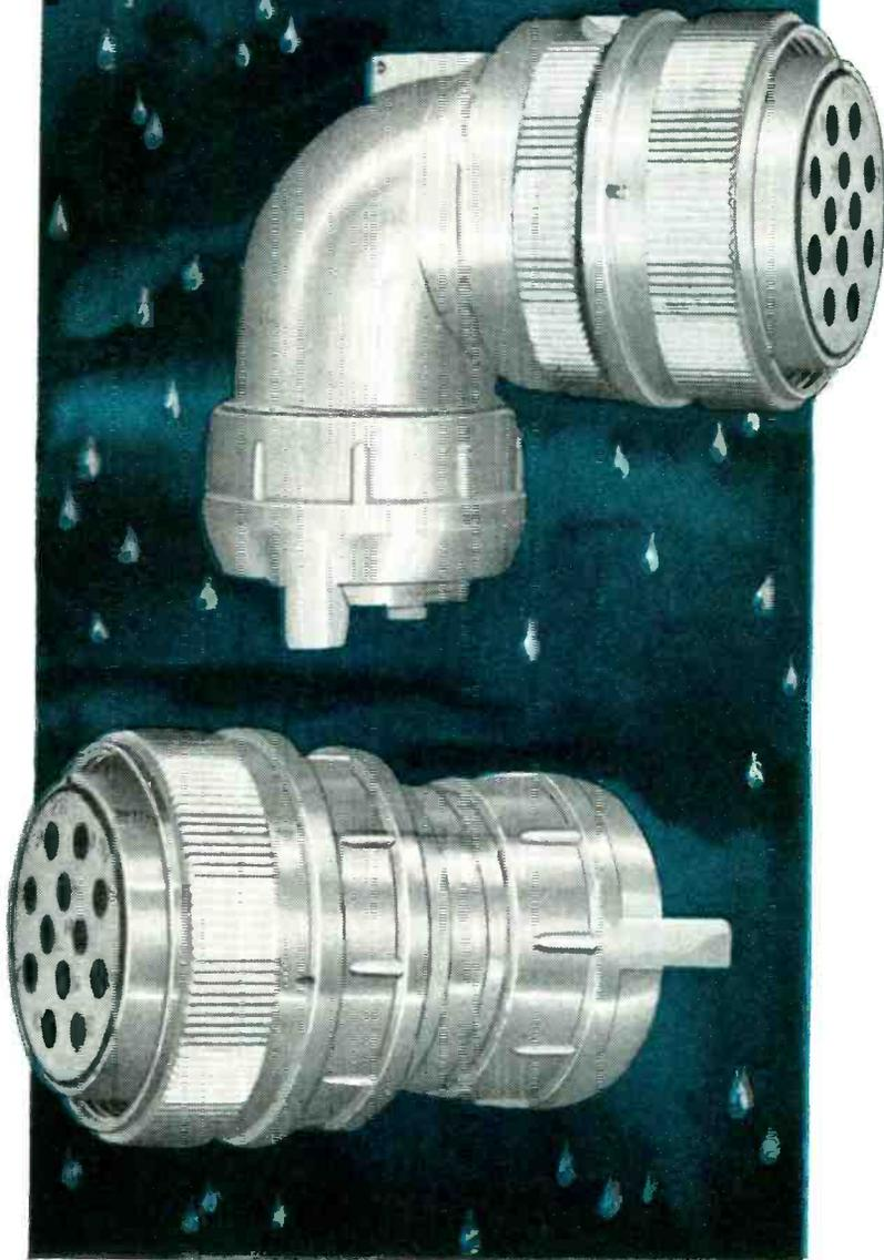
These new Bendix\*-Scinflex *waterproof* plugs are a modification of our standard AN type "E" (environment resistant) connector. They are designed to meet all "E" performance requirements when used with multi-conductor cables. Each plug includes a modified AN3057B cable clamp which provides inward radial compression on multi-conductor cables. This unique feature completely eliminates cable strain—a common source of circuit trouble.
