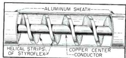
Section of cable cut out to show copper center conductor and helical windings
