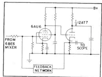
FIG. 8—Selective amplifier circuit
