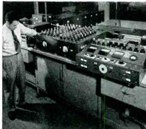
Life testing of standard diodes which compares various cathode alloys.
