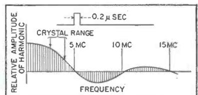
FIG. 2—Harmonic distribution of 0.2-microsecond pulse
