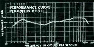
This average laboratory response curve of the Permoflux 8T-8-1 proves that it compares with the finest speakers regardless of size or price.
