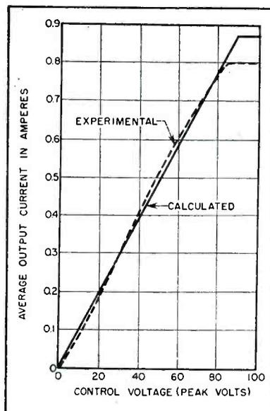
FIG. 2—A linear transfer characteristic is one feature of an NRL-designed experimental parallel magnetic amplifier which is also characterized by high gain and short response time
