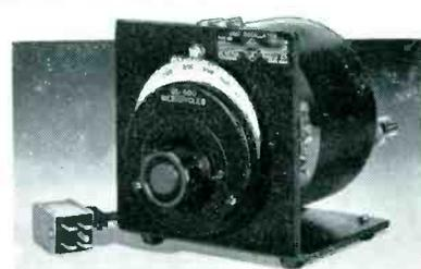
**Type 1208-A V-H-F Oscillator** This unit oscillator is similar to the Type 1209-A in construction and operation. The tuning circuit employs a sliding contact which makes possible a wider frequency range of 65 to 500 Mc. The frequency calibration is accurate to  $\pm 2\%$ . Into 50 ohms the output power is 100 mw at any frequency and 500 mw in the center of the range.
