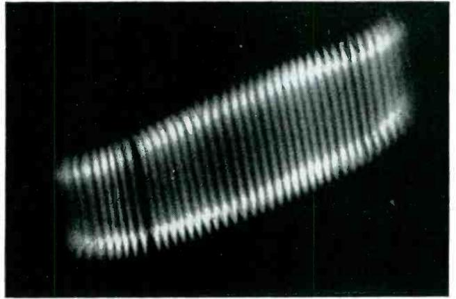
**NEW FILAMENT.** By redesigning the filament supports of G-E radio dial lamps, General Electric engineers matched the frequencies and greatly reduced the effects of vibration (above). As a result, G-E radio dial lamps give longer, more dependable service.
