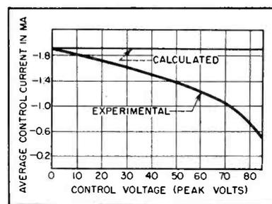
FIG. 3—Curves show theoretical and experimental input characteristics. Theoretical curve is for matched cores with vertical magnetization loops and ideal rectifiers
