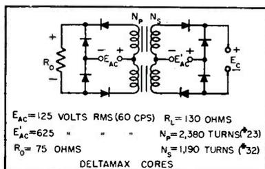
FIG. 1—Circuit diagram of parallel-connected magnetic amplifier
