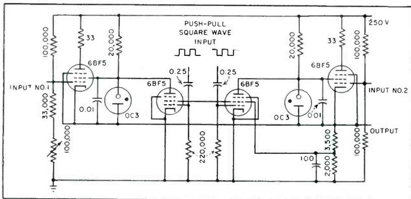
FIG. 1—Electronic switch for video frequencies
