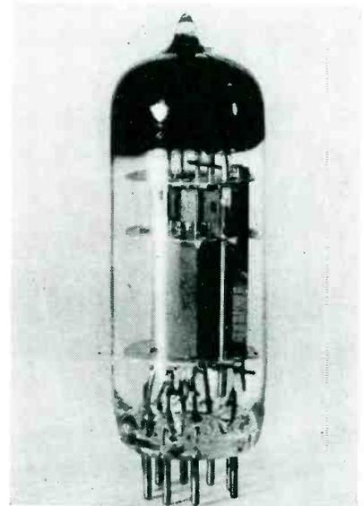
Combined pentode and triode for tv reception, tube type ECL 80, is shown in x-ray silhouette in the accompanying photograph
