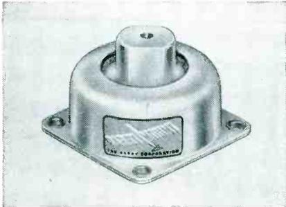
These new Barrymounts provide the aircraft and electronic engineer with a vibration isolator designed to meet the unusual temperature and environmental conditions encountered in high-altitude, high-speed flight. Employing no organic materials, these mountings are not subject to temperature influences that may affect the performance of other mountings.
