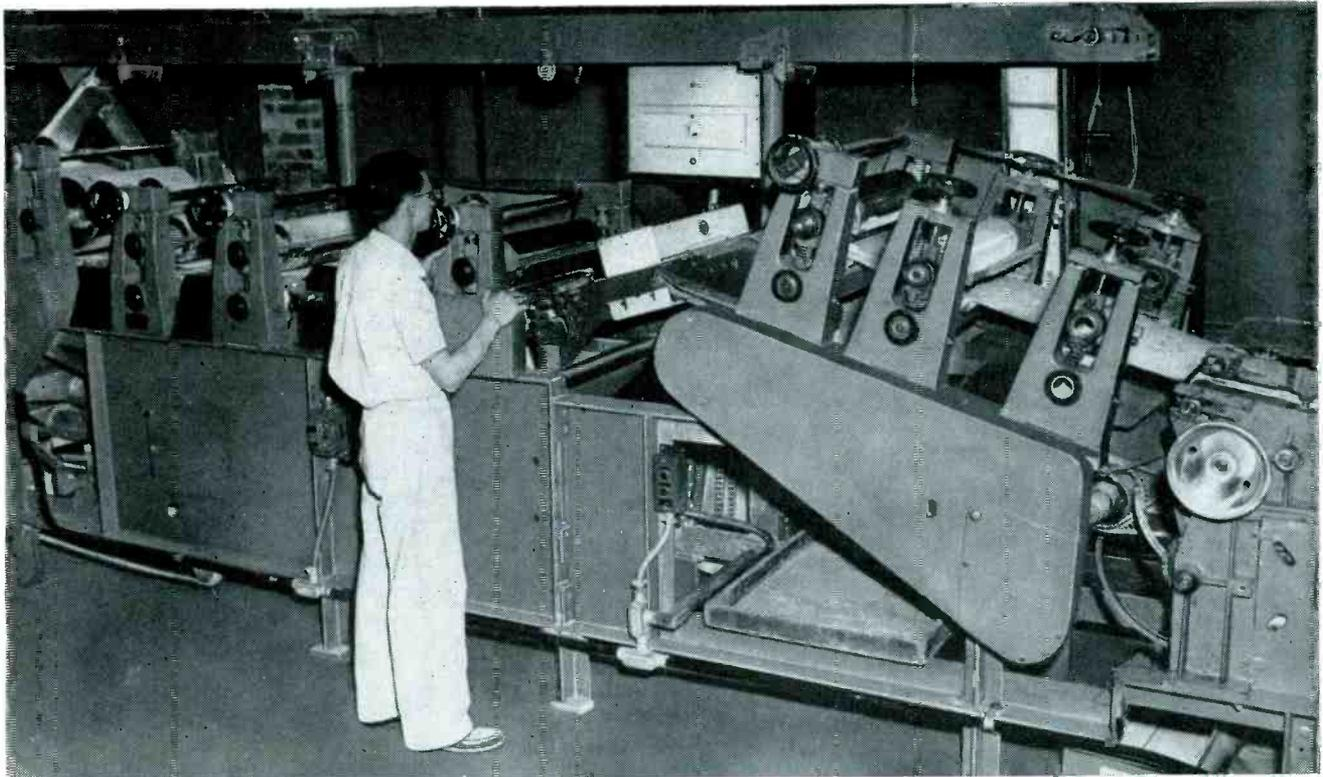
A commercial metal detector used for inspection of chewing gum. Inspecting coil is shown mounted on the machine in about the center of the picture with control box directly above it
