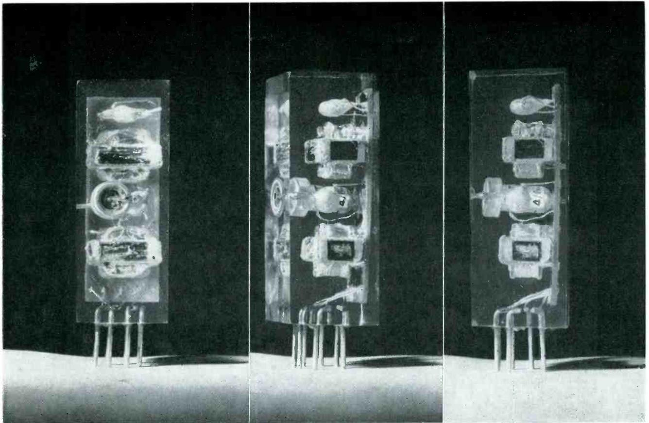
Three views of the transistor amplifier shown in photograph on left page. Experimental model transistors are visible in the amplifier as white plastic-covered beads. Transformers and other components are also visible. Unit will operate continuously for months with one penlight cell as sole power source
