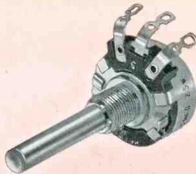
Quality control assures maximum uniformity in IRC's small 15/16" Type Q Controls. Construction features one-piece dual contactor of special alloy—simplified single-unit collector ring—molded voltage baffles—special brass element terminals that will not loosen when bent or soldered. Type Q Controls have unusual durability and efficiency—adapt to a great variety of small-space applications. Send coupon for full details in Catalog A-4.
