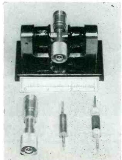
FIG. 1—The magnetic attenuator, a new, inexpensive type of microwave attenuator that requires no movable components, mechanical controls, or slotted sections in the waveguide or coaxial transmission line
