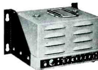
**Model 1411 INDUCTRONIC D-C AMPLIFIER**—stable amplifier provides high degree of resolution even at fractional loads. Reaches steady full scale deflection in fraction of a second. Interchangeable plug-in range standards for either microamperes or millivolts.
