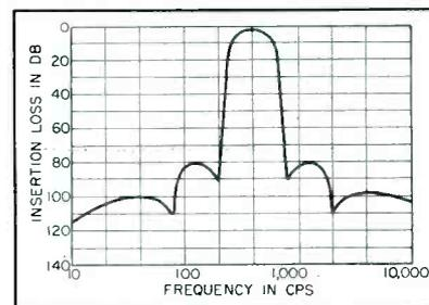
FIG. 4—Frequency response of band-pass filter
