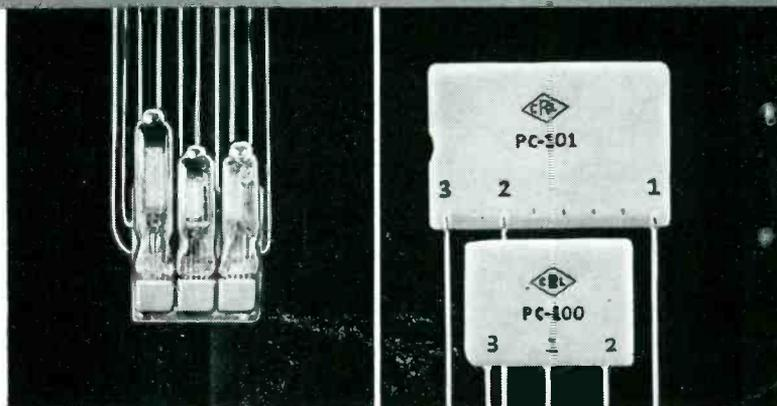
New Model 3 Ampec — a sub miniature 3 stage speech amplifier . . . dimensions: 1-1/32" x 15/16" x 11/32". Check coupon for Technical Bulletin 42-130.
