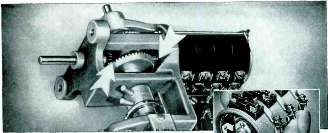
**CRUCIAL PRECISION IN A RADAR CONTROL ASSEMBLY** The gears on this radar control assembly were precision cut to eliminate backlash and binding, but the care that went into their manufacture could have been completely nullified if the potentiometer coupled to them was not mechanically precise. In this case, overall accuracy is assured by using a Fairchild precision unit.
