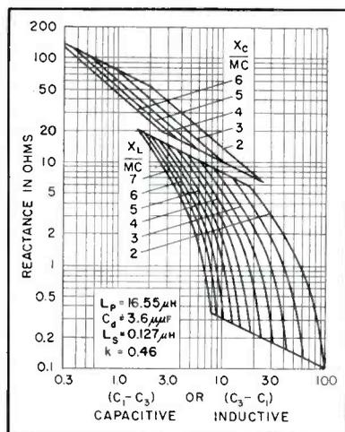
FIG. 6—Sample chart used to determine reactance of individual transformers
