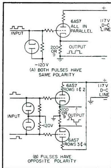
FIG. 4—Simplified circuit of power amplifier for the two settings of the polarity-changing switch
