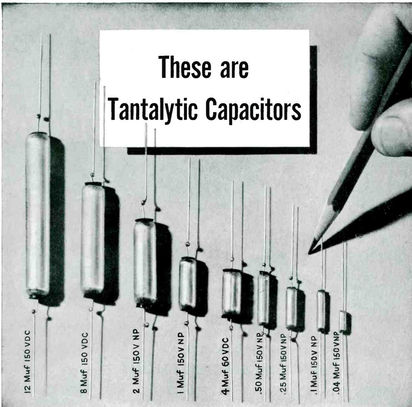
Here is one of the fastest moving developments in recent years—General Electric's new electrolytic-type capacitors. These Tantalytic capacitors with their small size and large capacitance per unit of volume have excellent low temperature characteristics, long operating life and in many cases can replace bulky hermetically-sealed paper capacitors. Ratings presently available for consideration range from .02 muf up to 12 muf at 150 volts dc. Units pictured are representative of these ratings.
