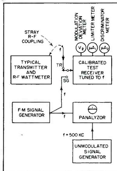
FIG. 2—Setup for calibration of modulation deviation of test receivers
