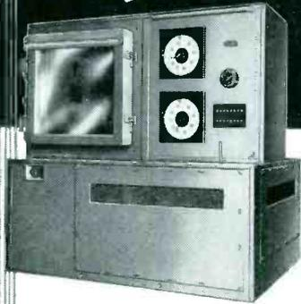
Bowser High Altitude Test Chambers furnish complete yet compact facilities for the testing of aircraft instruments and equipment at any and all altitudes. Included in the chamber are provisions for testing under wide conditions of temperature ranging from +200°F. to -150°F., as well as relative humidity from 20% to 95%. Bowser Test Units produce conditions within the limits called for in all Government environmental testing specifications.
