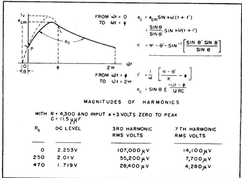
FIG. 6—Output waveform and representative magnitudes of video i-f harmonics
