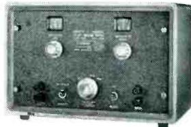
For use in the d-c path of a servo loop to obtain either proportional-plus-integral or proportional-plus-derivative correction for experimental determination of optimum filter characteristics.
