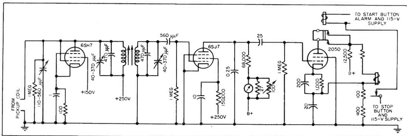
FIG. 6—Receiver section for one model RCA metal detector
