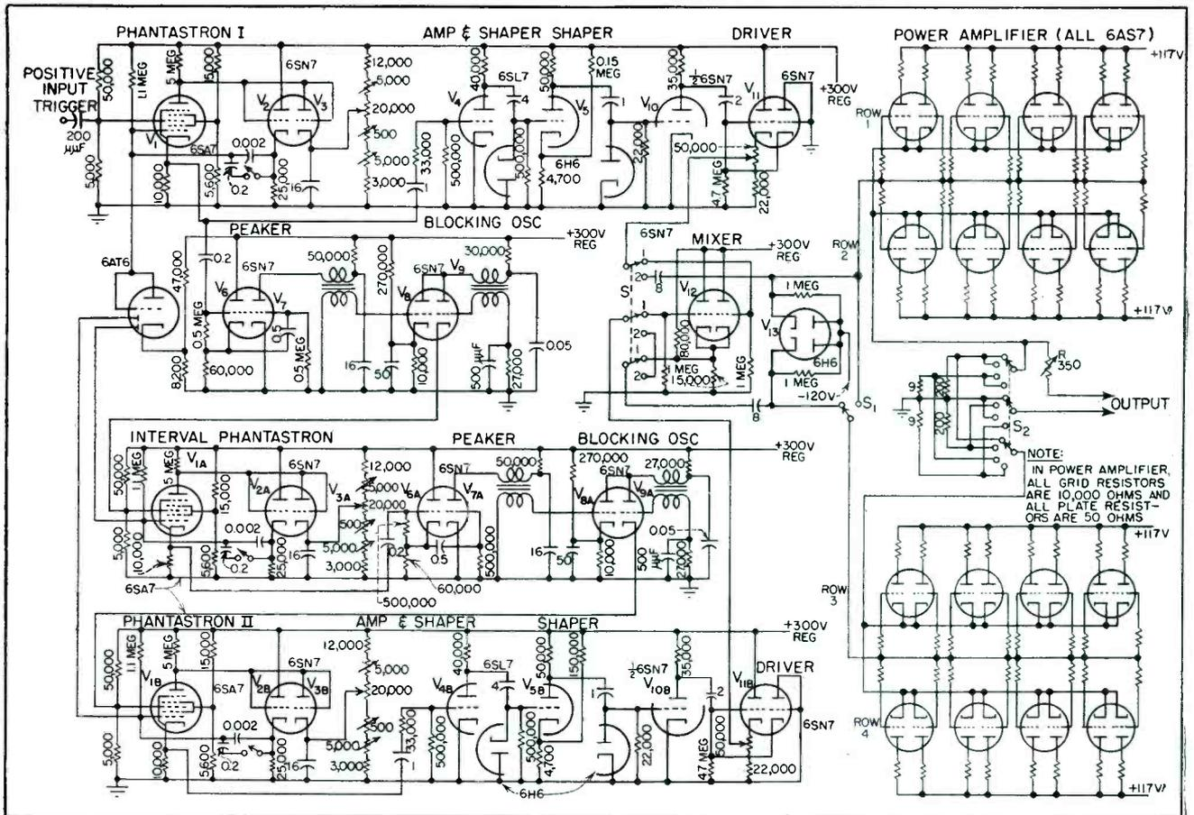
FIG. 3—Circuit of pulse generator and synchronizer. Power amplifier requires 117-volt d-c power line, and all other stages operate from a common 300-volt regulated power supply
