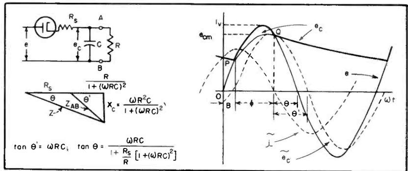
FIG. 5—Simplified video detector with diode resistance
