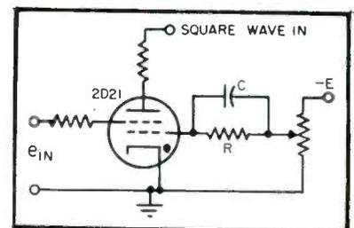
FIG. 2—Thyratron circuit with R-C compensation network
