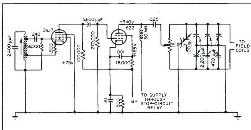
FIG. 7—Oscillator section of the RCA detector
