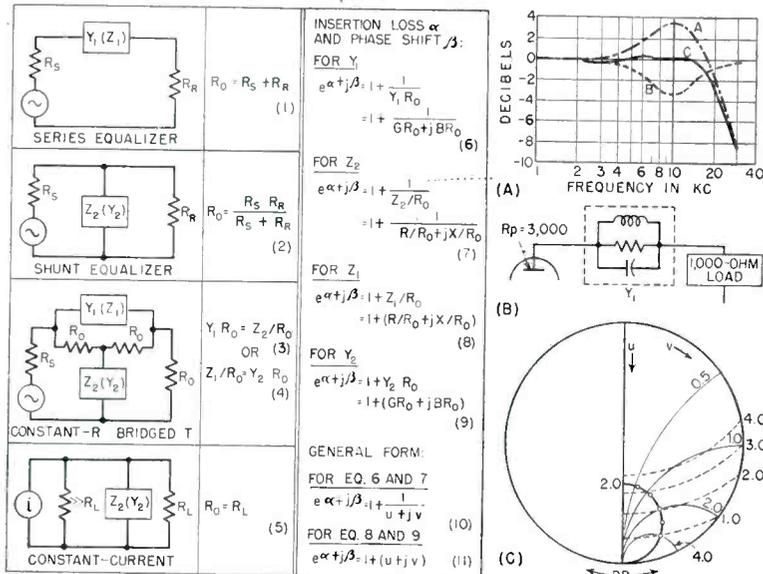
FIG. 2—Basic equalizer circuits, pertinent equations, and example
