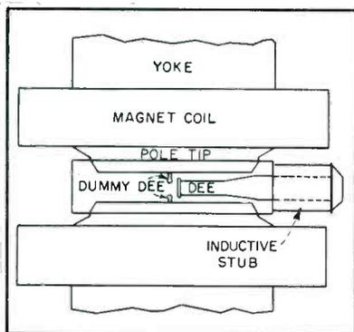
FIG. 1.—Side view of the dees and cavity of the cyclotron
