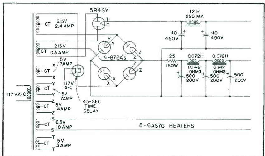
FIG. 4—Unique power supply used to operate the cathode-follower multitube output stage
