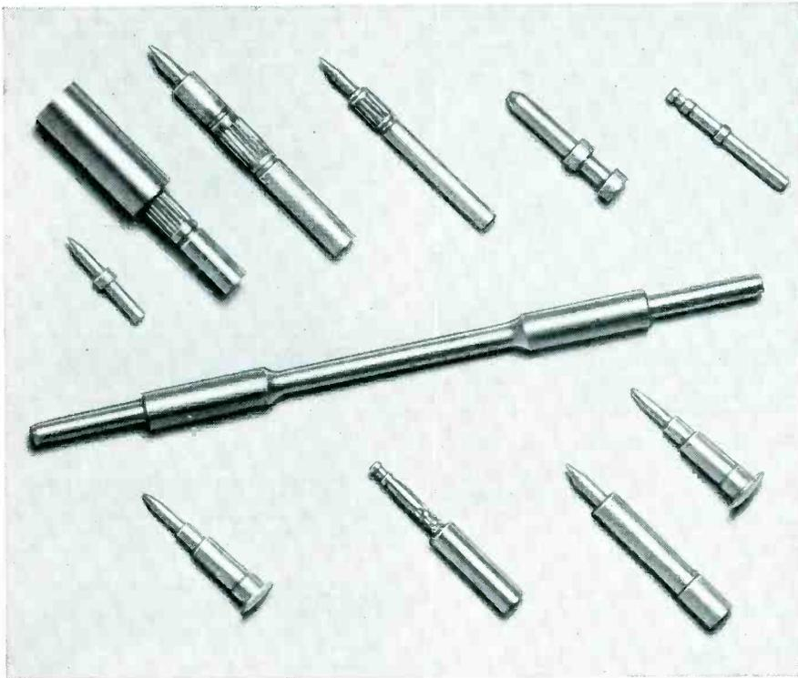
Examples of small parts produced accurately and economically on Swiss screw machines. Tapers on some parts generated on cutoff end to eliminate secondary machining operations. Courtesy Newtown Mfg. Co., Newtown, Conn. (samples enlarged 35%)
