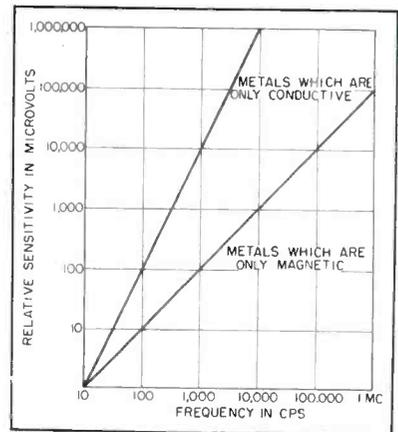
FIG. 1—Voltage induced in secondary coil as a function of frequency
