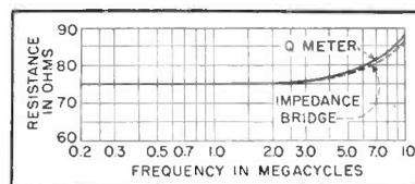
FIG. 2—Input resistance of an unterminated video attenuator at maximum attenuation, 62.5 db
