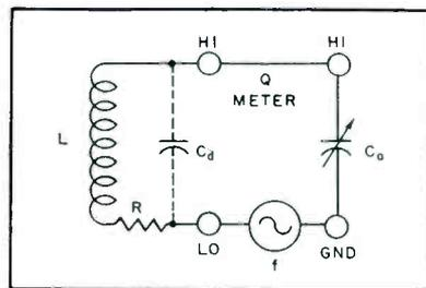
FIG. 9—Basic Q-meter circuit with the primary inductance of a transformer and its distributed capacitance connected to inductor terminals. Secondary not shown
