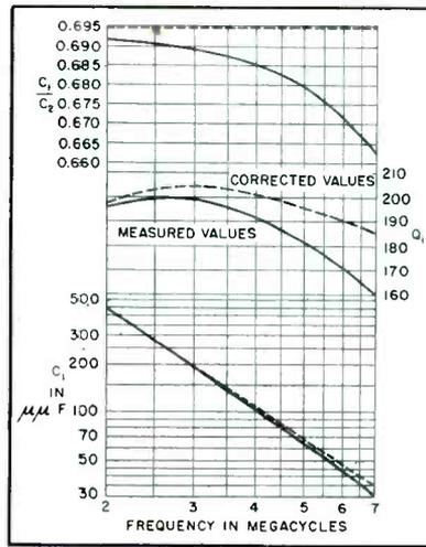
FIG. 7—Curves showing the extent of correction required for transformers with moderate distributed capacitance in the primary
