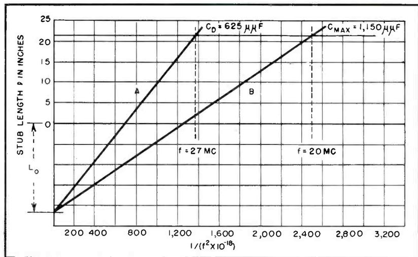
FIG. 3—Determination of  $L_0$  and effective  $C_D$  is possible from curve A. Desired capacitance change is obtained by using curve B in addition
