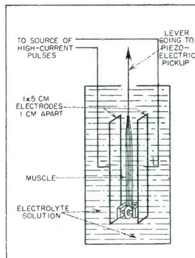
FIG. 1—Method of electrically stimulating a muscle with so-called massive electrodes connected to output of high-current electronic pulse generator. Muscle is clamped at its lower end, and upper end is connected through a lever to a piezoelectric pickup. Muscle (of frog) can live for many hours in the salt solution serving here as electrolyte
