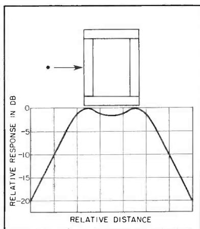
FIG. 3—Relative-amplitude response of quadrant coil system
