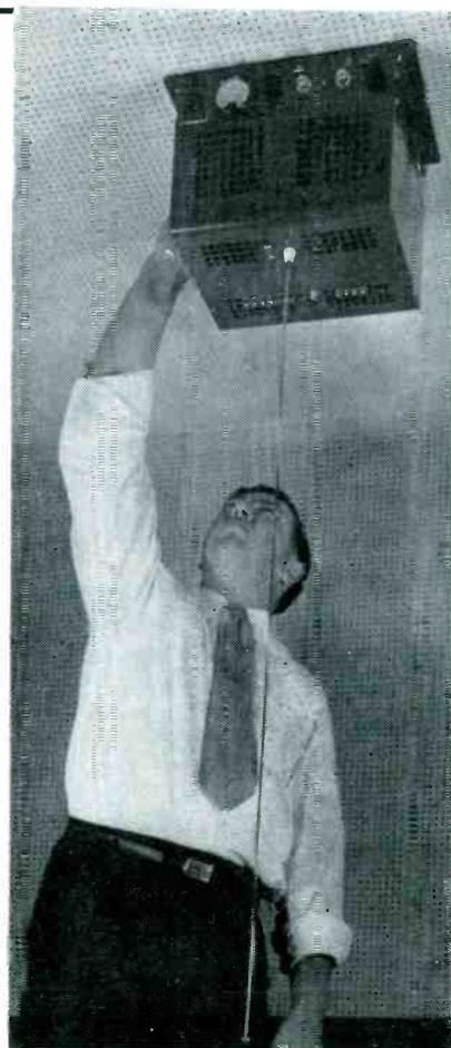
Transmitter is hung from ceiling as near center of studio as possible. Forty-inch whip is electrically short for 27 mc but inefficiency can be tolerated because of reserve of power available
