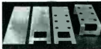
**Basic Chassis Construction** proceed as flat piece — Without stacking — it flows from one operator to next, similar to progressive die. Bending is last. Finish and plating is done by automatic conveyorized equipment. Means fast delivery — minimum delay.
