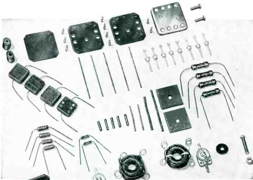
All of these 66 parts are from a single B&W Toroidal-coil type discriminator only 1¾" square by 3½" long exclusive of terminals!
