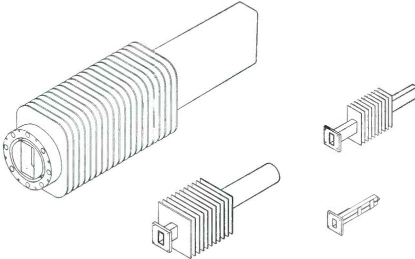
**HI POWER X BAND TEST LOAD**, dissipates 350 watts of average power for  $\frac{3}{8}$ " x  $\frac{1}{4}$ " waveguide, VSWR less than 1.15 bet. 7 and 10 KMC ... \$150.00
