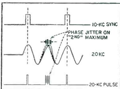
FIG. 6—Illustration of phase jitter in tuned frequency multiplier
