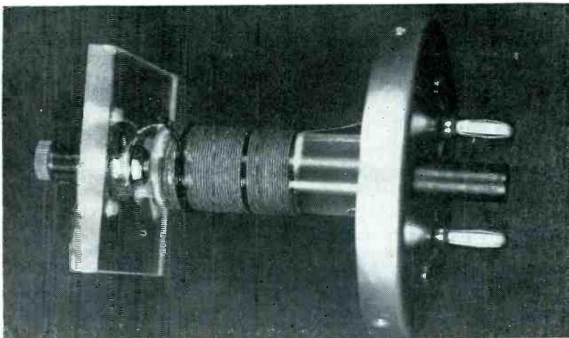
Transformer with shield removed has primary wound in two sections. This arrangement allows adjustment of inductance
