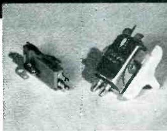
Dow Corning 4 packed in phonograph pick-up head cartridges increased crystal service life 20 times. The silicone compound prevents Rochelle Crystals from deteriorating due to absorbed moisture. It also acts as a viscous damping medium, thereby reducing excess vibration and enabling the head to handle a much higher frequency.
