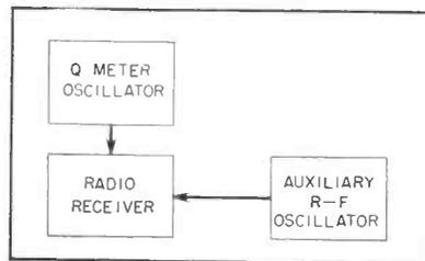
FIG. 4—Block diagram of precise system for determining distributed capacitance of a coil
