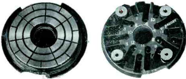
**High stresses** are set up by wide differences in expansion coefficients of brass inserts and phenolics, and by mold shrinkage. Yet not one of these distributor blocks and collector plates has ever cracked. Molder: Scintilla Magneto Div., Bendix Aviation Corp., Sidney, N. Y.
