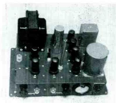
Top view of transmitter shows placement of components. High audio frequency pre-emphasis compensates for falling response of receiving units
