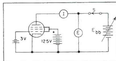
was opened when  $E_{bb}$  was 60 volts. The reading of voltmeter  $E$ , an ordinary 250-volt full-scale, 1,000-ohm-per-volt meter, increased to 75 volts instead of dropping to near zero. How can this be explained?
