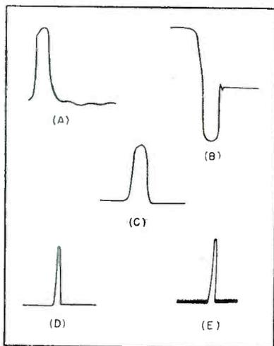
FIG. 4—Circuit waveforms: (A) sync pulse from pulse-repetition-frequency oscillator; (B) delay multivibrator output, showing firing of triggered blocking oscillator on trailing edge; (C) modulator output pulse; (D) generator output with strong signal input and agc; (E) generator output at low signal-to-noise ratio, with no agc
