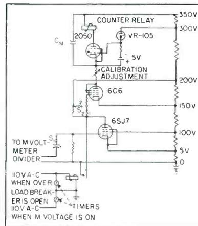
FIG. 2—Spark outage integrator instrument for recording outage time resulting from sparks in d-c high voltage systems
