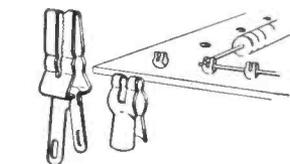
**Miniature Terminals — 650 Series** punch press configuration — ratchet slot holds various size component leads for soldering — no twisting of leads with pliers. Figure "eight" shape accommodates cross wiring and buss leads. Punch press parts — so take a minimum of solder, reduce solder time, eliminate danger of cold solder joints.
