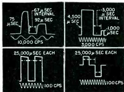
Examples of trains of pulses produced by stimulator, as recorded with dual-beam oscillograph to get timing wave
