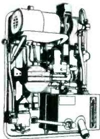
A complete hydraulic system. Necessary units completely assembled and ready to work. Includes tank, gear pump 2 1/2 HP dc electric motor, electric pressure unloading switch, relief valve, filter, accumulator, and connecting plumbing. 1500 PSI, 1 1/2 GPM at 1800 RPM. Mounted on 19" x 25" aluminum frame.
