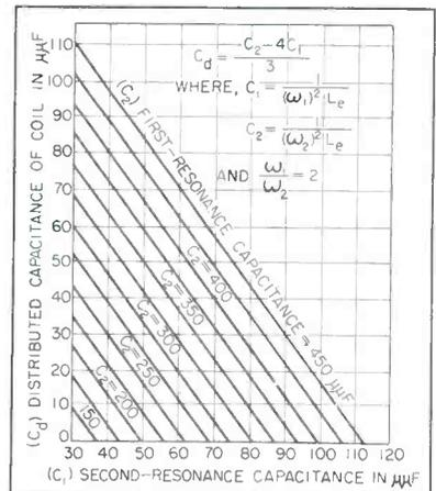
FIG. 3—Distributed capacitance curves
