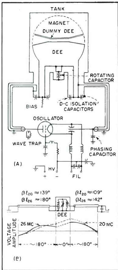
FIG. 6—Schematic circuit of the oscillator (A) showing connection to the dee, and qualitative phase and amplitude behavior of the circuit (B)
