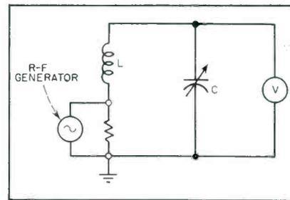
FIG. 1—Basic circuit of Q-meter method for measuring inductance
