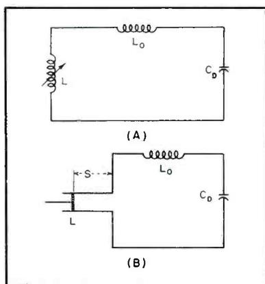
FIG. 2—Lumped circuit equivalent of dee (A), and variation using tuned stub (B)
