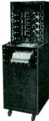
Model 67 provides for the direct, simultaneous registration of up to four phenomena on one record, using the same principles and methods as the two systems described above. In addition, there is a selection of eight paper speeds: 50, 25, 10, 5, 2.5, 1.0, 0.5, and 0.25 mm/sec., and provision for the use of 4-, 2-, or 1-channel recording Permapaper. As in Model 60, above, amplifiers and preamplifiers are readily interchangeable.
