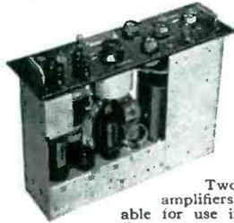
Two types of amplifiers are available for use in Sanborn recording systems—a DC General Purpose Amplifier, and a Strain Gage Amplifier (shown above). The amplifiers used in the 2- and 4-channel systems are generally identical with those in the 1-channel system, which are available, as are also all the recorders, for separate application.
