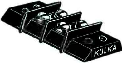
Blocks of high tensile strength Bakelite (or other plastics to gov't spec.) and come in 4 sizes—with 1 to 23 terminals. Screws and solder lugs of nicked brass. Lugs in several styles, also eyeletted to block. Marker strips come plain or printed, or blocks can be engraved.
