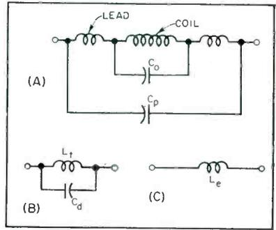
FIG. 2—Simplifying equivalents used in calculation of distributed capacitance
