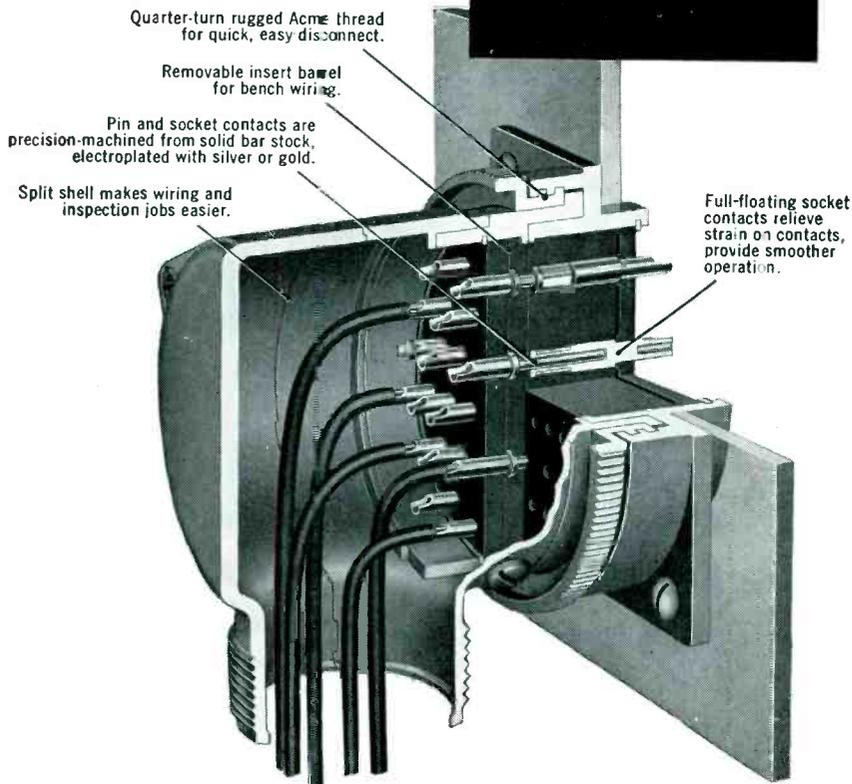
Recognition of Cannon's 36 years of sound engineering and fine, uncompromising construction has built the demand for Cannon Plugs. Here we take an inside look at the lightweight Type "K" 90° connector, forerunner of the Army-Navy Series. More features of the "K" were incorporated into the "AN" design than any other connector.
