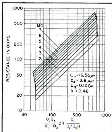
FIG. 5—Sample chart used to determine resistance of individual transformers
