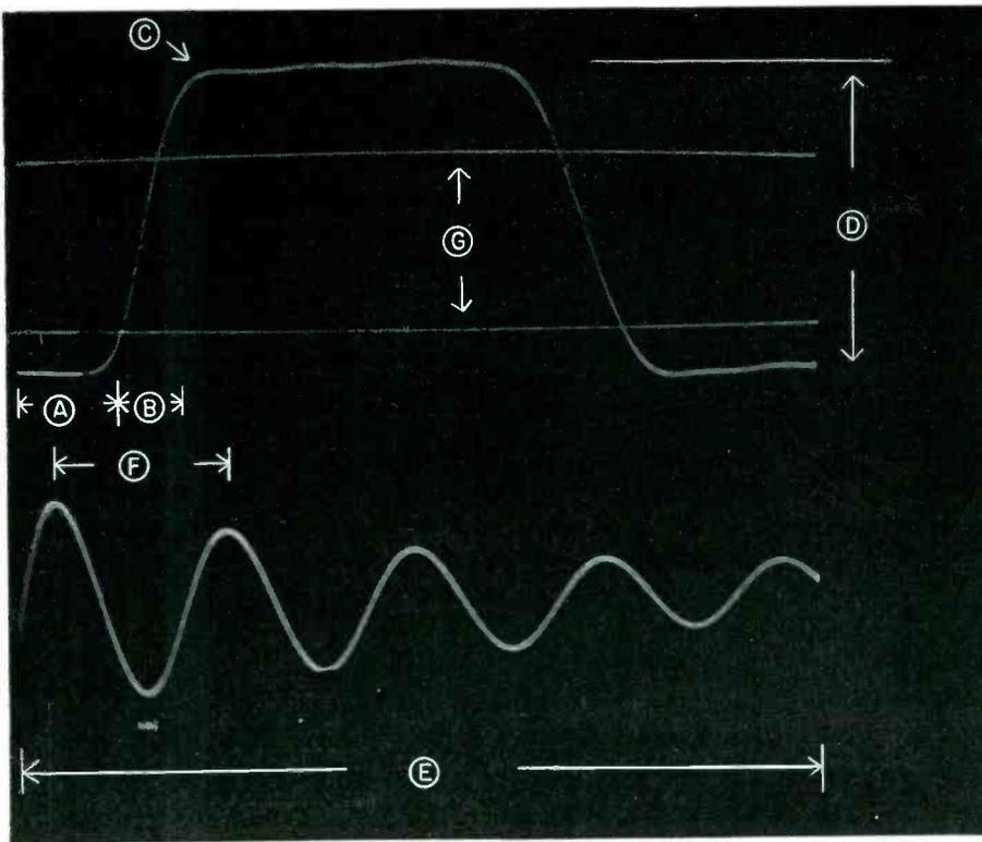
Here, woven around the quantitative investigation of a 0.25 microsecond pulse, is a graphic account of the performance features which make the Type 303 an exceptionally fine, high-frequency cathode-ray oscillograph.
