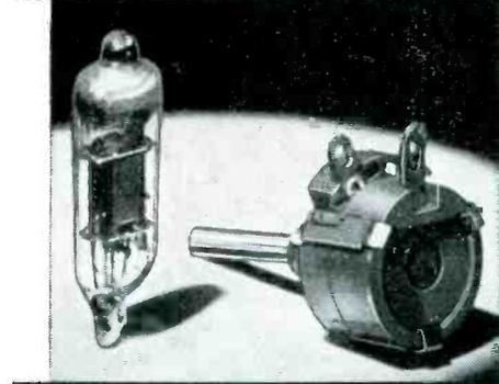
Shown alongside a miniature tube is this Clarostat Series 48 sub-miniature potentiometer. Only 5/8" dia. — no bigger than a dime! Carbon element up to 3 megs. linear; slightly higher in taper. 0.4 watt rating. Single, dual, triple units. Essential in ultra-compact electronic assemblies. Here's *precision* in diminution.
