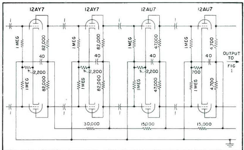
FIG. 3—Suggested resistance-coupled preamplifier with good square-wave response from 20 to 20,000 cps
