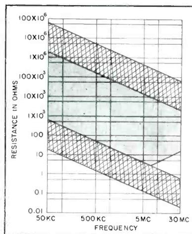
FIG. 1—Latticed portions show present range of measurable resistance with Q meter and shaded portion gives range using transformers
