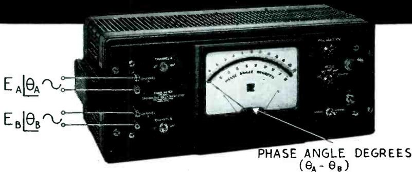
TIC's New 320-A Phase Meter is the first commercially available instrument for the direct measurement of the phase difference between two recurrent mechanical motions or two electrical signals independent of amplitude, frequency, and wave shape.
