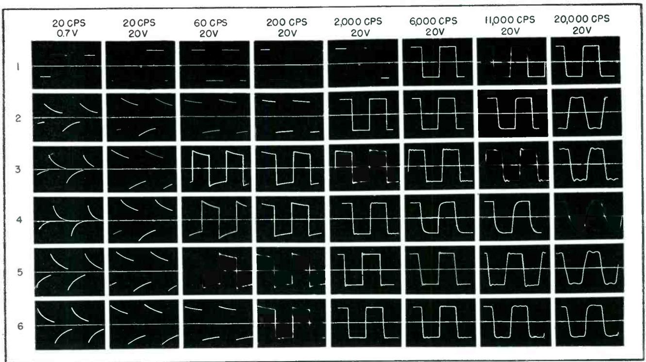
FIG. 5—Square-wave oscillograms obtained in comparison between follower output stage and various high-quality transformers. Top row shows the follower results. Transformer types are listed in the text
