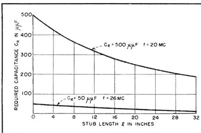
FIG. 4—Stub length versus required terminal capacitance for a representative cyclotron oscillator
