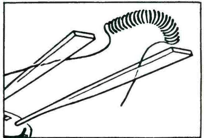
**IMPROVED JOINT.** To prevent dial lamps from being "noisy", General Electric developed a better joint—one with tungsten filament legs pressed firmly into the softer metal of the lead-in wire. It's another reason why G-E dial lamps insure customer satisfaction!
