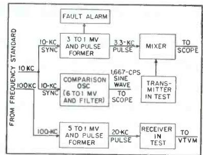
FIG. 1—Block diagram of synchronized-pulse system of frequency measurement
