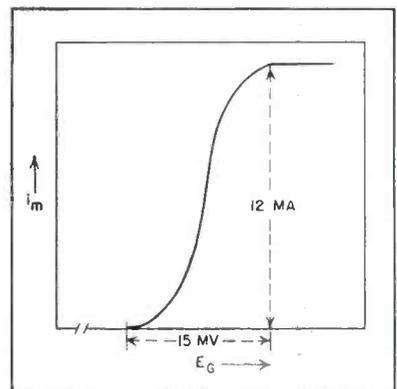
FIG. 1—Average plate current vs grid voltage curve for 2D21 in neighborhood of firing point
