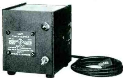
**Type 1203-A Unit Power Supply** This new unit supplies voltages of 6.3 for cathode heaters at 3 amperes maximum, and 50 ma at 300 volts dc, maximum. The no-load voltage is 410. Hum level is 250 mv at 300 volts and 50 ma d-c output. Connections to associated unit equipment are made through a standard multipoint connector mounted in the ends of the unit. A mating multipoint connector for connecting the supply to other equipment is furnished.
