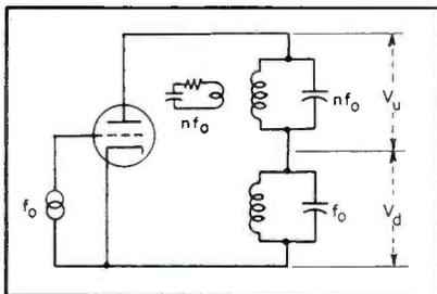
FIG. 7—Plate-line resonances owing to harmonic components
