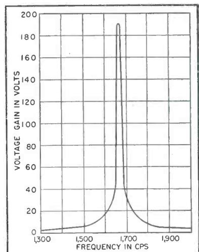
FIG. 4—Response of selective amplifier in mixer unit for narrow-band operation
