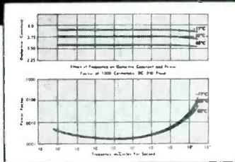
As indicated by these curves, neither frequency nor temperature changes have any pronounced effect on the power factors or dielectric constants of Dow Corning 200 Fluids. Power factor and dielectric constant of 1000 cs. fluid at  $-17^{\circ}$ ,  $23^{\circ}$ , and  $83^{\circ}$  C. are plotted against frequencies ranging from 10 to  $10^{10}$  cycles per second.
