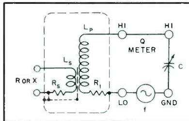
FIG. 8—Basic Q-meter circuit with a transformer connected to the inductor terminals. Electrostatic shield and dotted connections optional
