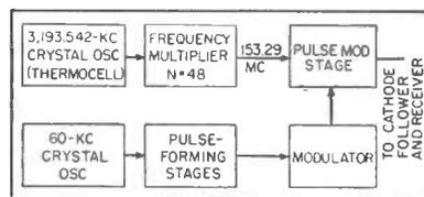
FIG. 7—Receiver checker for 148-to-174 mc band
