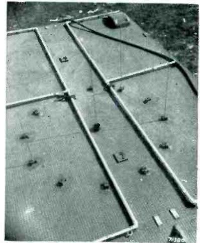
On the reinforced roof of the transmitter coach, a choice of mounts is provided for proper parasitic whips for the 1-m audio transmitting system of Signal Corps mobile television caravan
