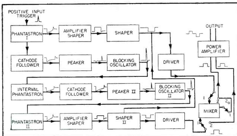
FIG. 2—Major stages of stimulator and waveforms of pulses at various points
