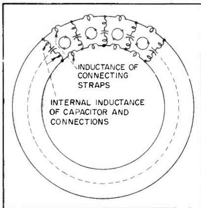
FIG. 8—Capacitor ring resonances
