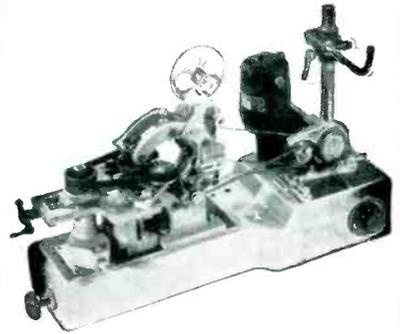
Wide-range, laboratory-type machines available for winding samples and small production runs of toroid coils. Production machines built to meet specific requirements.
