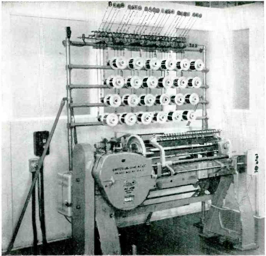
**25 INSERTS A MINUTE** Single or laminated insulating sheets, either paper or acetate, are fed into the Leesona No. 107 Coil Winder at rates as high as 25 per minute. Thus, on a coil containing 100 wire turns per layer, the machine can be run at speeds as high as 2500 rpm.
