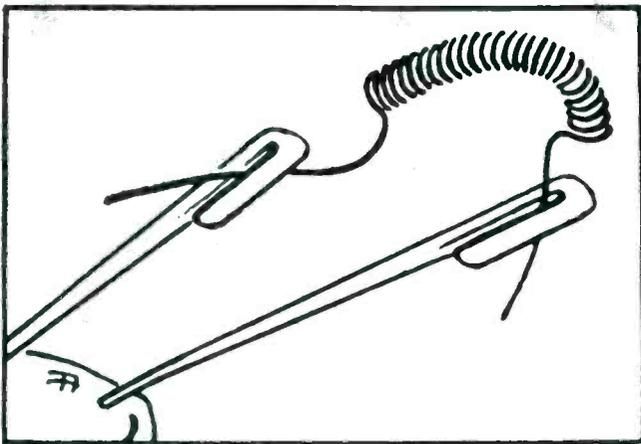
**OLD-TYPE JOINT.** Some types of dial lamps actually cause "static". Old-type clamp joints in the bulb (above) often permit changes in resistance or tiny arcs that cause the lamp to radiate bothersome interference.
