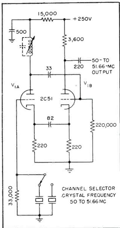
FIG. 1—Cathode-coupled oscillator
