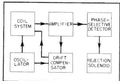
FIG. 2—Block diagram of an ideal metal detection system
