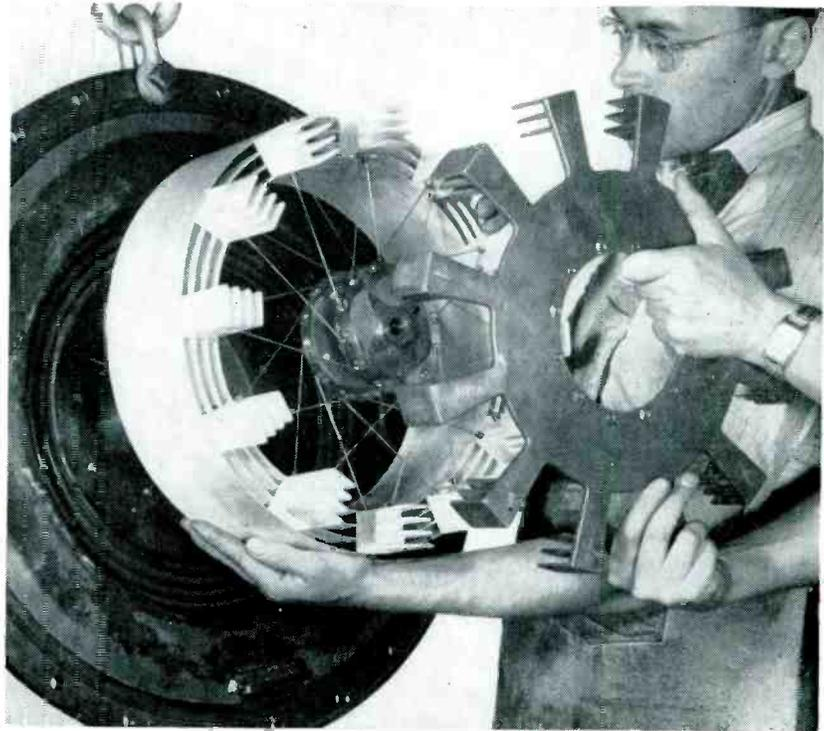
Variable capacitor to produce f-m. Note capacitance takeoff at left
