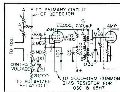
FIG. 5—Automatic drift compensation circuit
