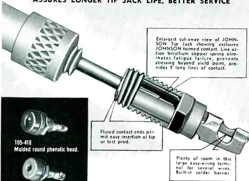
Enlarged cut-away view of JOHNSON Tip Jack showing exclusive JOHNSON formed contact. Live action beryllium copper spring eliminates fatigue failure, prevents stressing beyond yield point, provides 2 long lines of contact.
