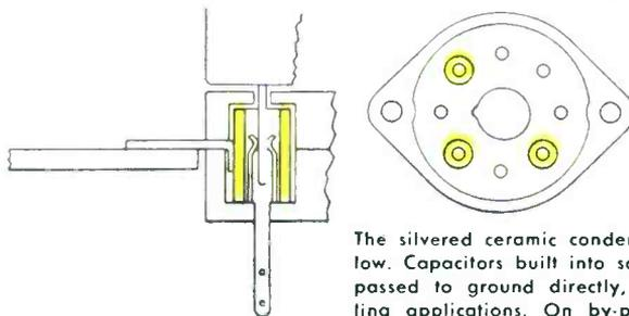
The silvered ceramic condensers are shown in yellow. Capacitors built into socket may be either by-passed to ground directly, or left open for coupling applications. On by-pass applications, ground strap contacting outer plate of capacitor is connected to metal chassis when tube socket is mounted.
