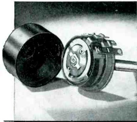
This precision potentiometer has a tapered winding held to plus/minus 1½% linearity as measured at 10 test points. Mechanical tolerances held to plus/minus 0.00025". Unit operates dependably over extreme ranges of temperature, humidity, altitude or barometric pressure, and severe vibration. Obviously built to a *quality* standard rather than to a price.
