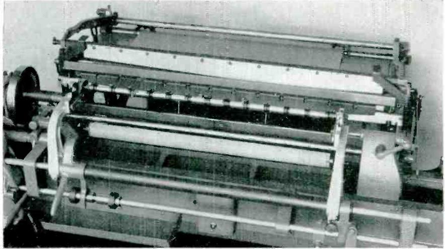
**EASY MANUAL OPERATIONS** Photo shows coil arbor in position for quick transfer. Wire turn counter can be reset quickly. No cam transfers are required when changing wire layer length, wire spools are easily changed.
