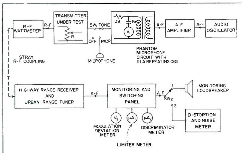
FIG. 1—Arrangement of major units in transmitter testing set
