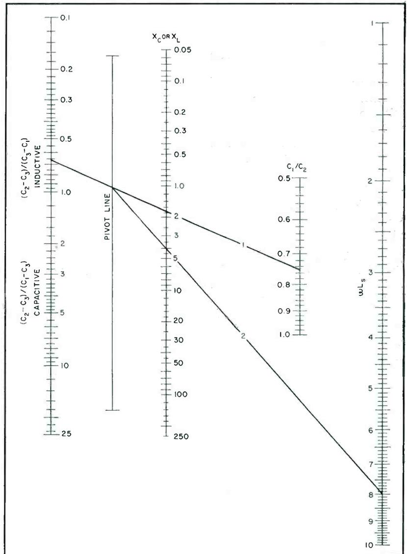
FIG. 4—Nomograph for reactance  $X$  in Eq. 17 and 18. If  $C_1$  equals  $150 \mu\mu\text{f}$ ,  $C_2$  equals  $200 \mu\mu\text{f}$ ,  $C_3$  equals  $180 \mu\mu\text{f}$  and  $\omega L_s$  equals 8 ohms, then  $X_L$  equals 4 ohms
