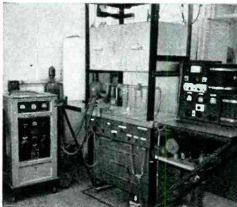
Trolley exhaust for sealing-off standard diodes.
