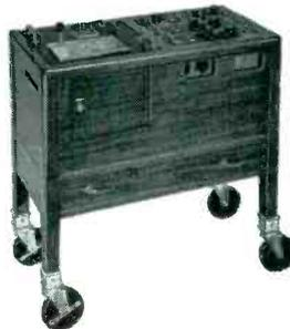
The two channels of Model 60 operate independently of each other, but record simultaneously. Ten paper speeds are standard equipment, in pairs of: 5 and 0.5, 10 and 1, 25 and 2.5, 50 and 5, 100 and 10 mm/sec. Ready interchangeability of amplifiers (DC and Strain Gage) and preamplifiers (DC and AC) makes possible the availability of a variety of input circuits. Timing and coding are built-in features. Each channel has a 5 cm recording width.
