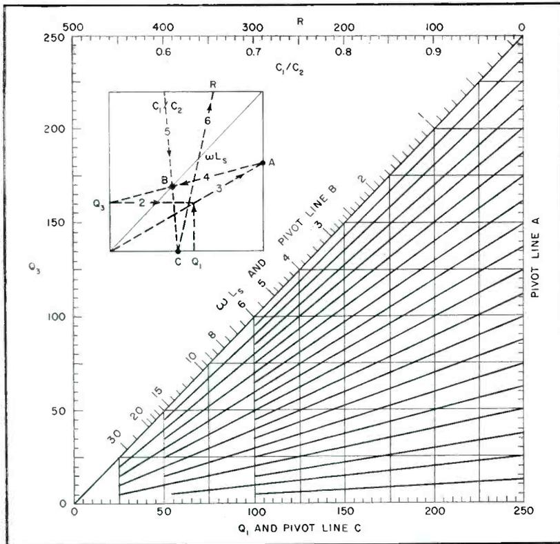
FIG. 3—Nomograph for resistance  $R$  in Eq. 10. If  $Q_1$  equals 200  $Q_3$  equals 100,  $C_1/C_2$  equals 0.75 and  $\omega L_s$  equals 40 ohms, then  $R$  equals 2,000
