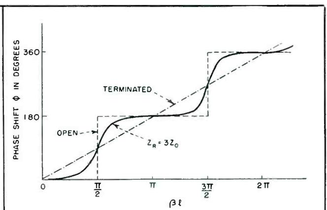
FIG. 5—Phase characteristics of a transmission line under various conditions of termination
