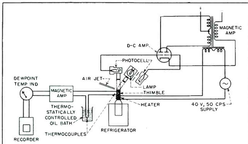
FIG. 1—Photoelectrically controlled dew-point hygrometer
