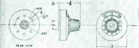
Microdial... turn-counting dial, primarily designed for use on Micropot ten turn linear potentiometers... use it on any multiturn device having ten turns or less.
