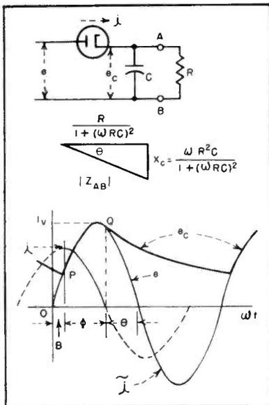
FIG. 4—Simplified video detector neglecting diode resistance
