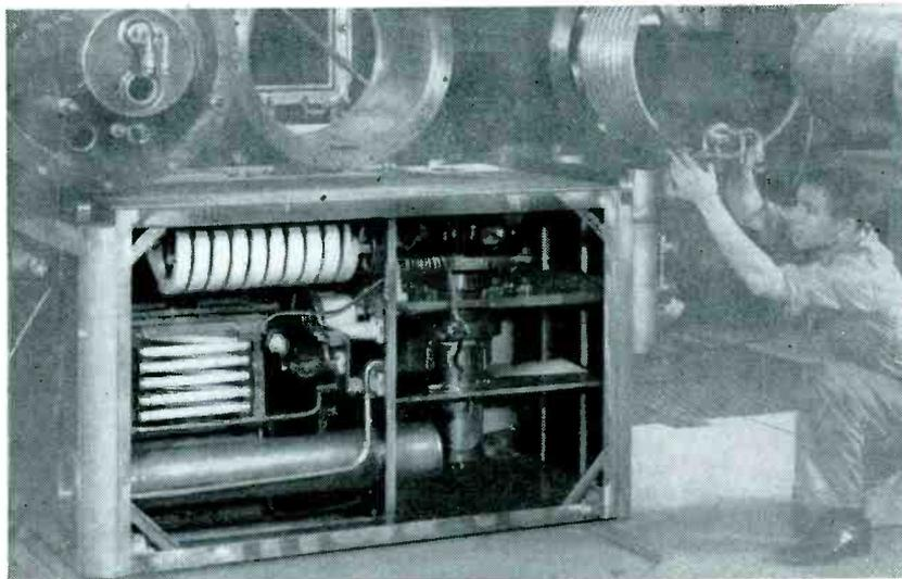
Oscillator dolly with attached dee partially removed. Type 9C21 oscillator tube at right, grid leak, metering circuits and ceramic water coil at left
