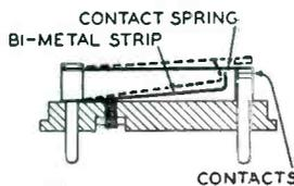
Standard and hermetically sealed Stevens Type C thermostats are carefully pre-calibrated in pots simulating actual service conditions; spot life-tests assure quality control. Specify Stevens Type C thermostats for closer temperature control—*longer life.*
