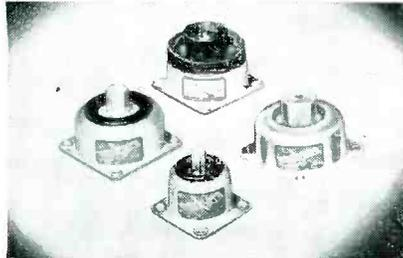
“Ruggedized” Barrymounts are available in both the air-damped type and the ALL-METL type. Air-damped Type 770R covers load ranges between  $\frac{1}{4}$  lb. and 9 lbs. Air-damped Type 780R covers load ranges between 4 lbs. and 35 lbs. ALL-METL Type 6600R covers load ranges between 4 lbs. and 35 lbs. Type M-112R covers ranges between 2. and 10 lbs.
