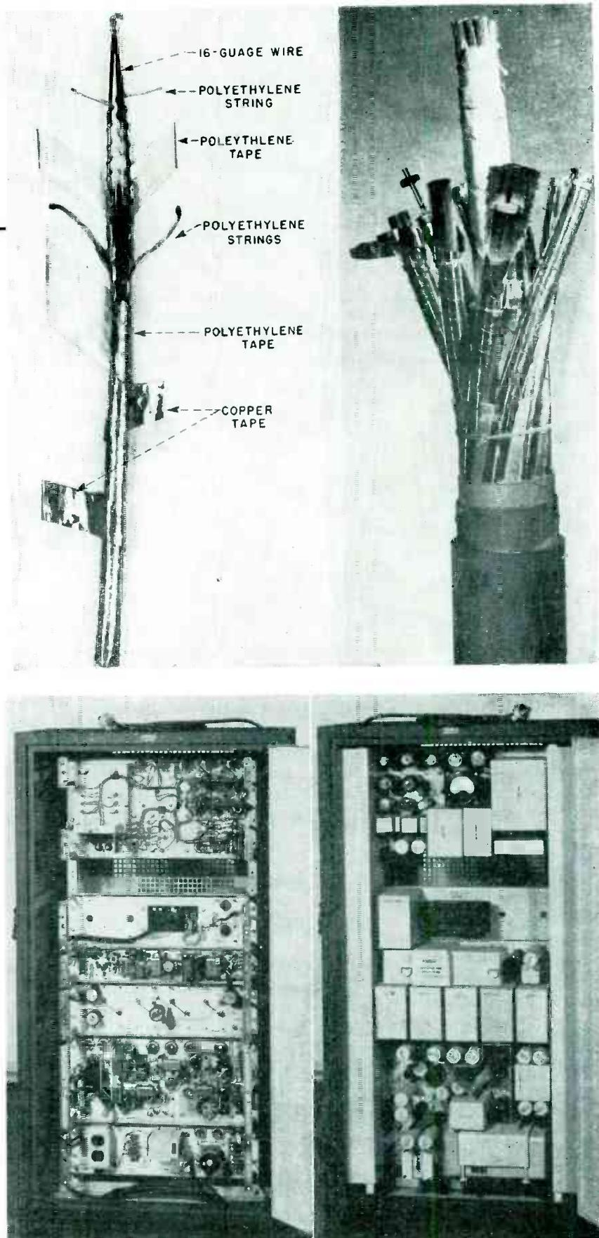
FIG. 2—Front and rear views of video amplifiers used in short haul circuits
