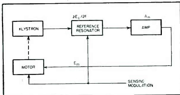
FIG. 3—A basic motor-operated automatic frequency control
