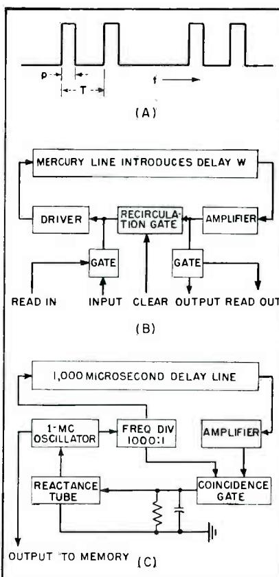
FIG. 1—For use with delay lines, information is in the form of pulse chains (A). These chains can be recirculated (B) through gates and the line so as to be stored as long as necessary. To compensate for temperature effects on the mercury lines, a timing oscillator (C) can be frequency controlled by an auxiliary line, the output being used to time pulses to the bank of mercury memories.
