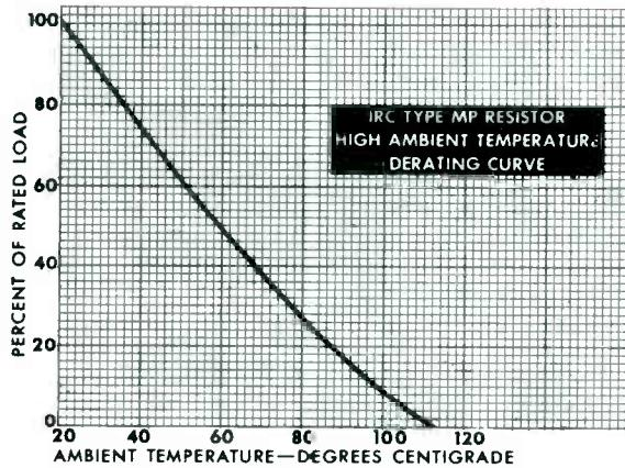
**DERATING.** Type MP Resistor power ratings are based on an ambient temperature of 20°C. When operated at any higher ambient, it is recommended that they be derated according to the following curve. For example, suppose an MPO Resistor is to be operated in an ambient temperature of 40°C. From the curve it is seen that the permissible load is 74% of the rated load. Since the MPO is normally rated at 30 watts, then at 40°C., it should not be loaded to more than 74% of 30 watts, or 22.2 watts.
