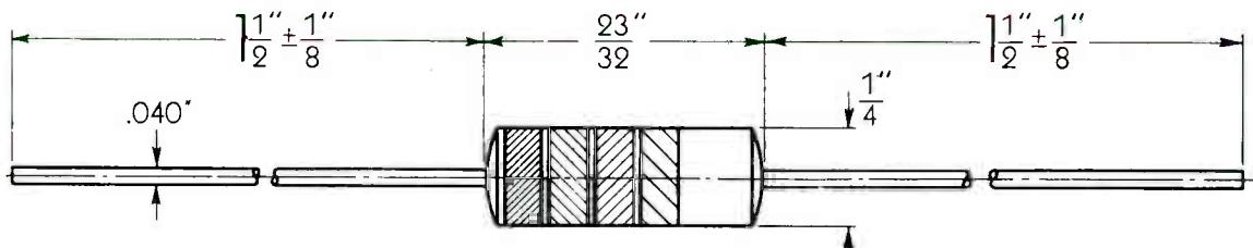
**POWER AND VOLTAGE RATING:** 1 watt (at 40°C. ambient)
