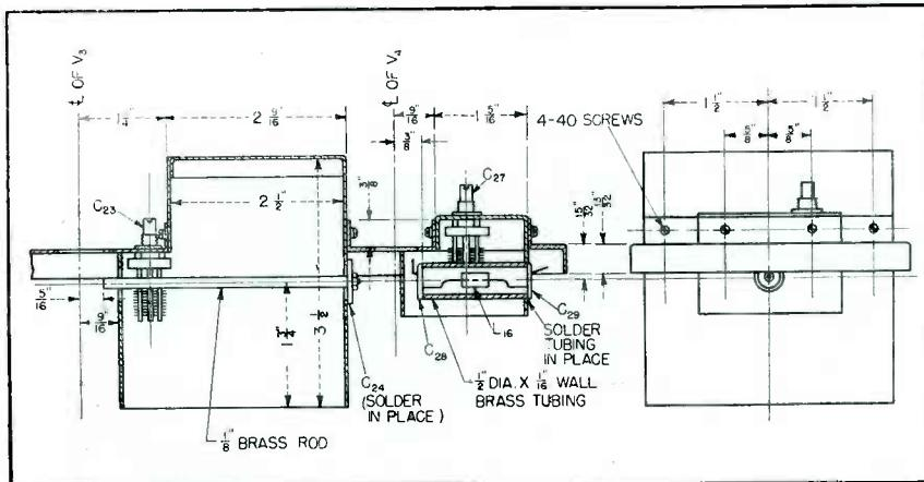
**FIG. 4**—Side view of chassis, showing constructional details of resonators operating at 232.5 and 465 mc.
