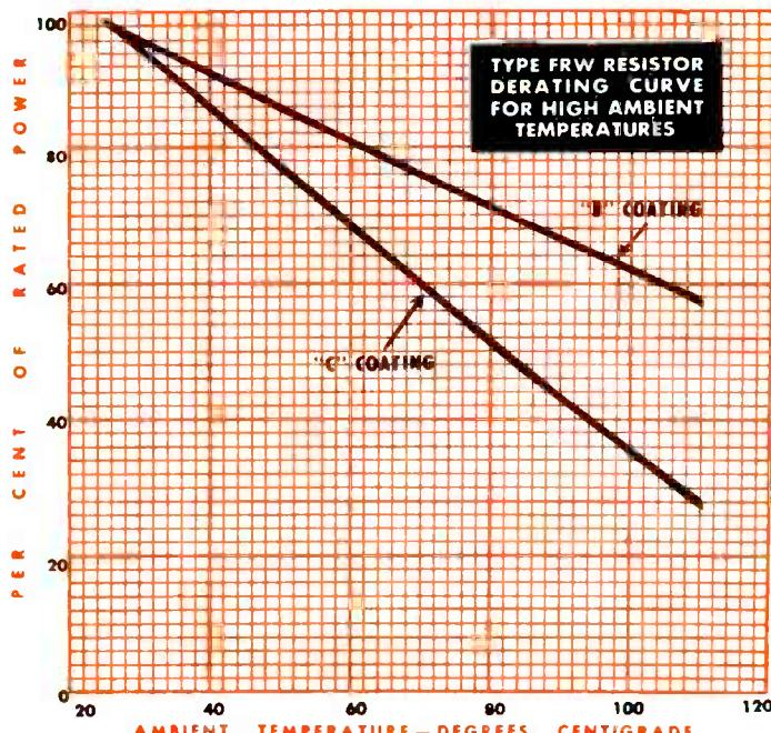
**DERATING.** If necessary to operate Type FRW Resistors in an ambient higher than 25° C., it is recommended that they be derated according to the Derating Curve for High Ambient Temperatures. For example, if the resistor is normally a 50-watt type and is to operate at 60° C. ambient, it should not be loaded to more than 82% of 50 watts, or 41 watts.
