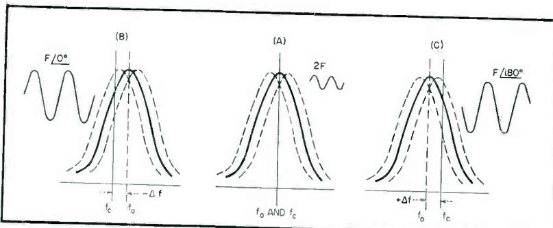
FIG. 1—Phase method of obtaining frequency drift sense
