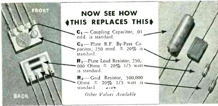
**8** First commercial application of the "printed circuit", CRL's new *Couplelate* offers a complete interstage coupling circuit consisting of an integral assembly of *Hi-Kap* capacitors and resistors closely bonded to a steatite ceramic plate and mutually connected by metallic silver paths "printed" on the base plate.
