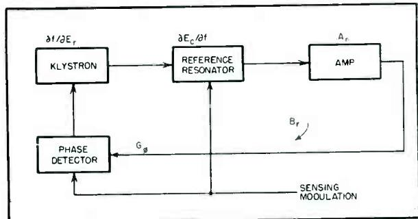
FIG. 4—A basic electronic automatic frequency control
