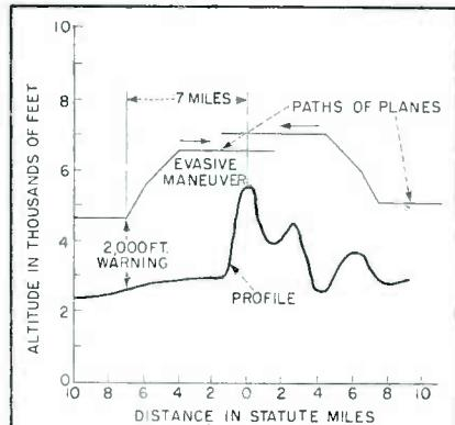
FIG. 2—Typical terrain profile
