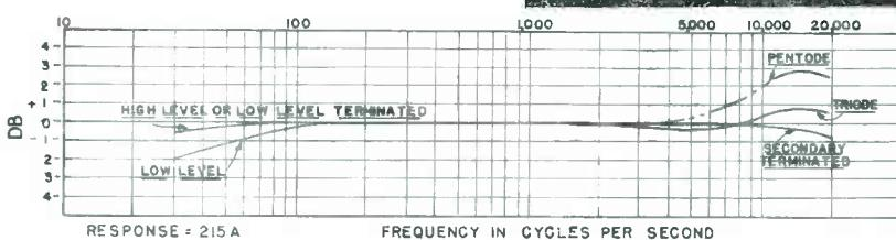
Low frequency response—(referred to 1000 cps) (High level + 26 vu, Low level -15 vu):
