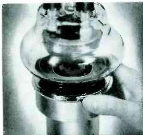
**AUTOMATIC SEAL WATER JACKET.** No tools needed to open and close the new Machlett water jacket. No worry about tube breakage or water leakage. Jacket cannot be opened unless water pressure is off, nor closed unless tube is properly seated. Your hand opens and closes a perfectly safe seal with just a single twist.
