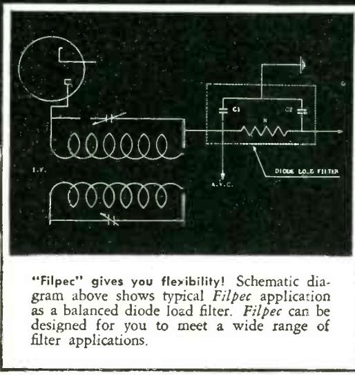
"Filpec" gives you flexibility! Schematic diagram above shows typical Filpec application as a balanced diode load filter. Filpec can be designed for you to meet a wide range of filter applications.
