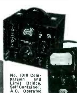
No. 1010 Comparison and Limit Bridge. Self Contained. A.C. Operated
