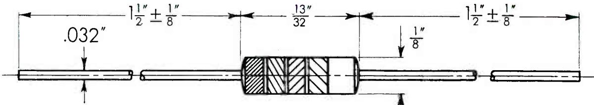
**POWER AND VOLTAGE RATING:**  $\frac{1}{2}$  watt (at 40°C. ambient)
