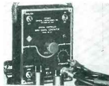
draws 17 watts, and comes equipped with a 6-foot cord and 53-inch leads with insulated clips.
