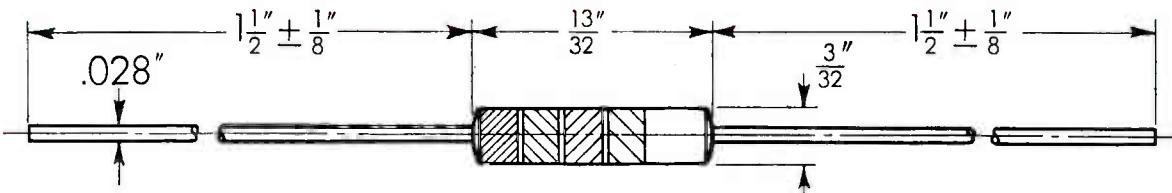
**POWER AND VOLTAGE RATING:**  $\frac{1}{3}$  watt (at 40°C. ambient)
