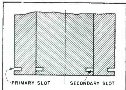
FIG. 2—Cross section of probe coil form
