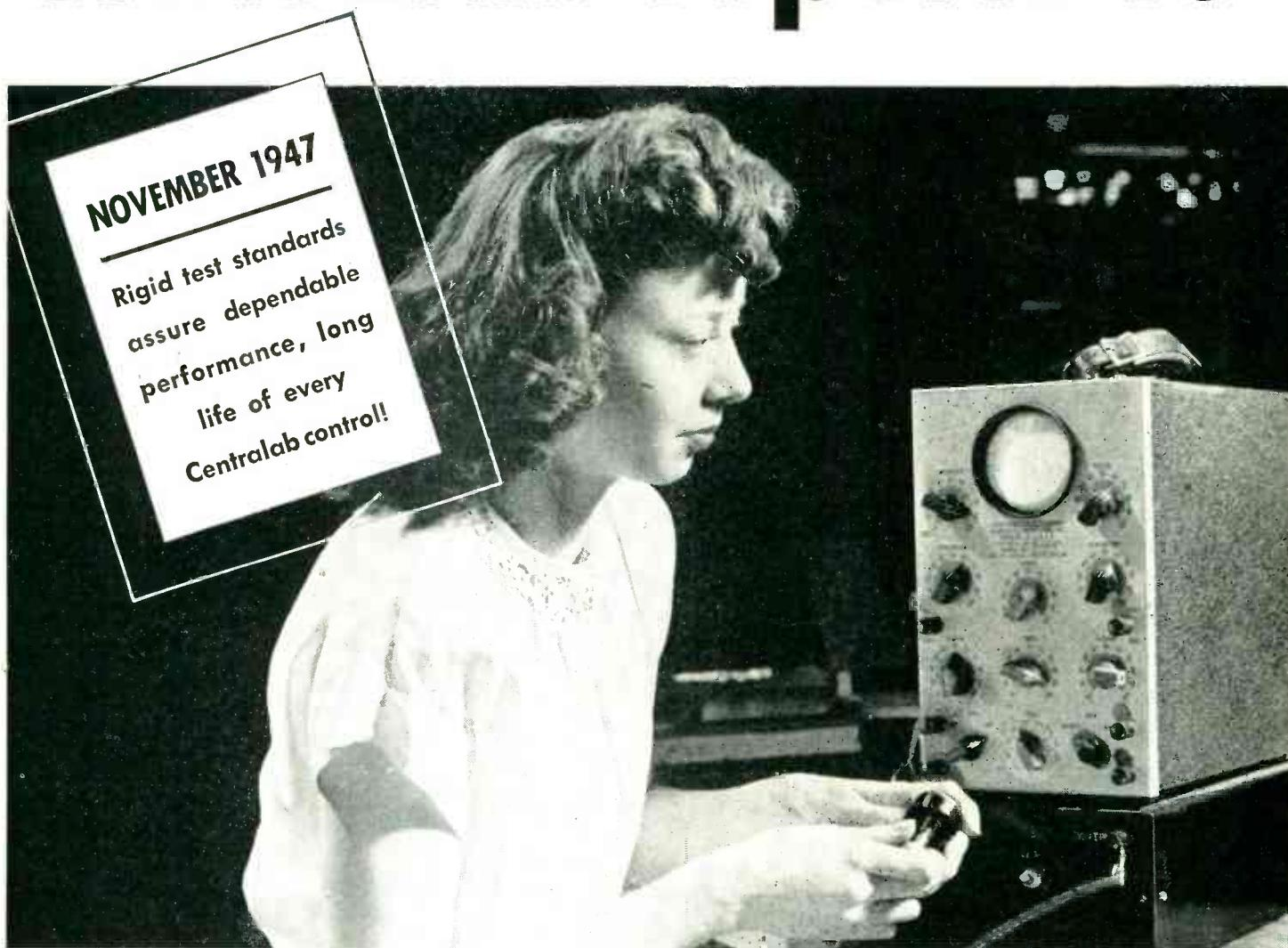
**1** 100% electrical test for continuity and "shorts" completes Centralab's program of tests for each control before it is shipped. This includes testing for resistance at various degrees of rotation, taper, noise, mechanical dimensions, etc. It's the
