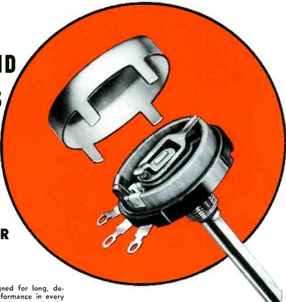
The IRC Type W Control is designed for long, dependable service and balanced performance in every characteristic. A 2 watt variable wire wound unit, this control provides maximum adaptability to most rheostat and potentiometer applications within its power rating. It's small  $1\frac{1}{4}$ " by  $9/16$ " design features the exclusive IRC spiral spring connector, a long-wearing alloy contactor, and welded connections between resistance element wire and terminals.
