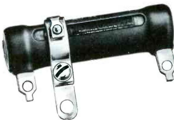
The IRC Adjustable Power Wire Wound Resistor consists of a standard tubular resistor with a track of exposed wire. Contact is kept with the wire by means of a metal band which, when power is turned off, can be adjusted to any position along the resistor.
