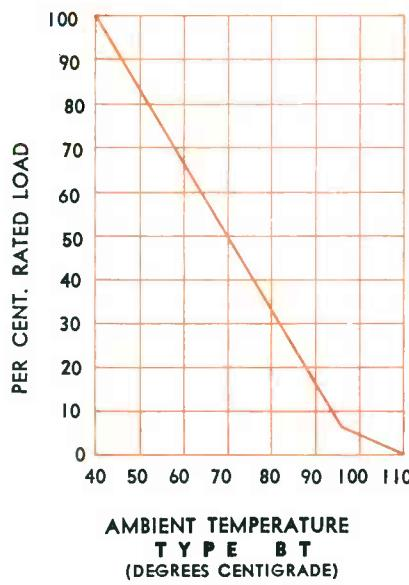
Ratings of Type BT are based on an ambient temperature of  $40^{\circ}\text{C}$ . Ambient conditions as well as voltage ratings and actual power requirements should be considered when determining the proper size of resistor for any application. When BT's are used at ambient temperatures exceeding  $40^{\circ}\text{C}$ ., load should not exceed that indicated by the JAN-R Derating Curve reproduced here.
