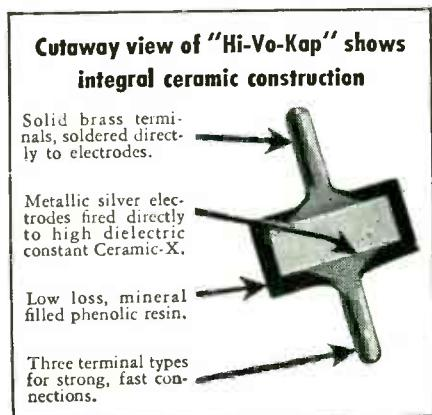
**4** CRL *Hi-Vo-Kaps* combine high voltage and small size for television applications. For use as filter and bypass capacitors in video amplifiers.
