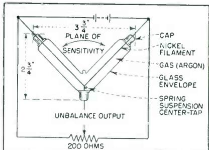
Convection vertical position sensing tube made by Eclipse-Pioneer Div. of Bendix changes resistance of its two arms when displaced in the plane through its legs
