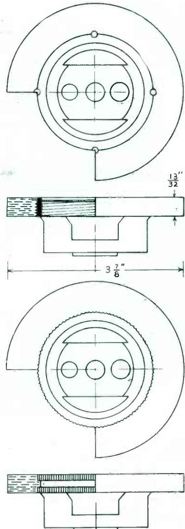
**SOLUTION:** RICHARDSON PLASTICIANS RECOMMENDED ADOPTION OF MOLDED PROCEDURE. INSTEAD OF THREADING THE SPIDER, THIS SECTION WAS DEEPLY KNURLED & A CENTRAL GROOVED RECESS WAS CUT AFTER KNUURLING. THE SPIDER WAS MOUNTED IN A SUITABLE MOLD & DISKS OF SATURATED MATERIALS WERE MOLDED INTO PLACE. MATERIAL FILLED RECESS & KNURLED PORTIONS TO GIVE PERFECT BONDING.
