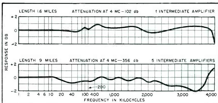
FIG. 5—Frequency characteristics for two video circuits of the type shown in Fig. 3
