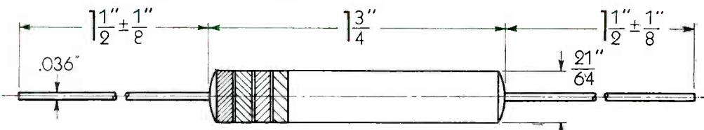
**POWER AND VOLTAGE RATING:** 2 watts (at 40°C. ambient)
