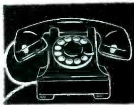
YOUR TELEPHONE TRANSMITTER AND RECEIVER, voice gateways to the telephone plant, are so essential to satisfactory service that they have been under study in Bell laboratories for seven decades.
