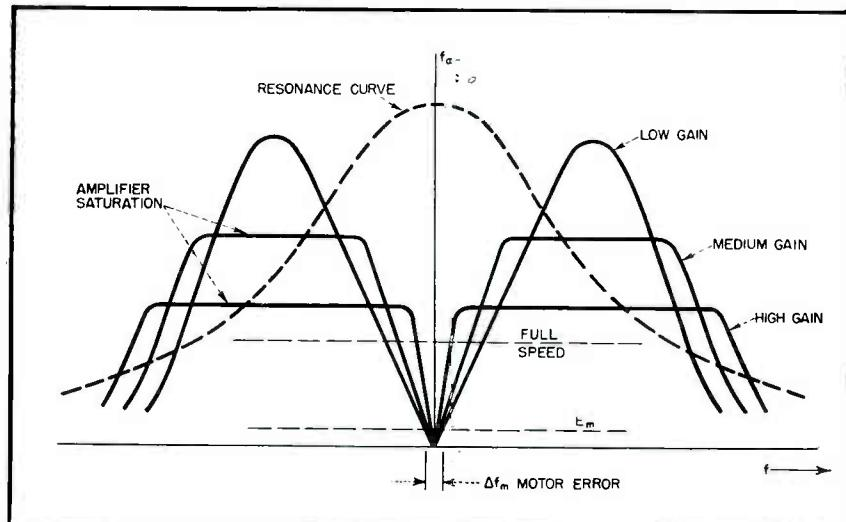
FIG. 6—The hold-in characteristic versus motor-amplifier gain indicates how well motor error can be compensated
