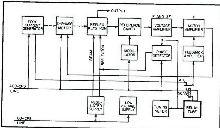
FIG. 7—Block diagram of a motor afc system connected for antihunting
