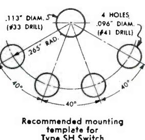
Recommended mounting template for Type SH Switch
