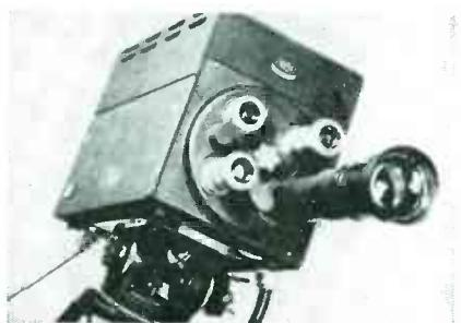
camera features a lens turret that takes up to four lenses of various focal lengths. Turret, diaphragm setting, and focusing are controlled from the rear of the camera. Hinged and removable panels make components and circuits immediately accessible. The electronic viewfinder avoids parallax difficulties.
