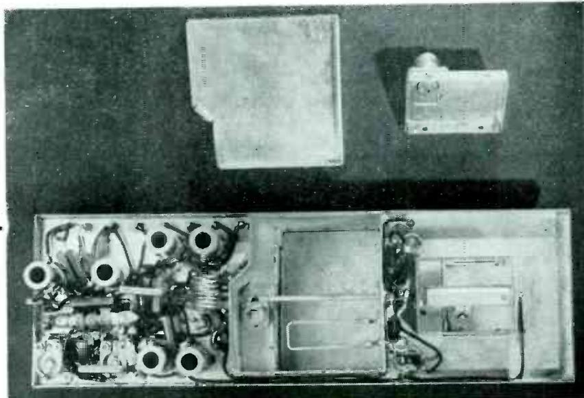
Bottom view, showing interior of resonators and coupling loops. Conventional coils are used up to 116 mc
