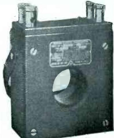
Weston Model 481 Type 4 (see illustration). This unit can be used with any precision 5 Amperes A.C. Meter to extend the ranges of the meter to 50, 100, 200, 250, 500 or 1000 Amperes A.C. Accuracy within  $\frac{1}{4}$  of 1%; Normal Secondary Capacity = 15 Va; Binding Posts for 50 Ampere tap; Inserted primary for 100, 200, 250, 500 and 1000 Amperes; Insulated for use up to 2500 volts. List Price \$98.00.....NET fob, NY \$35.00
