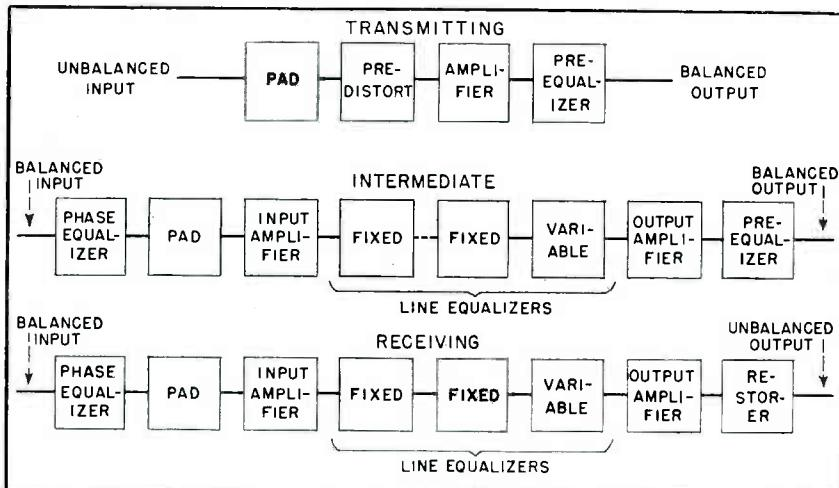
FIG. 3—Unbalanced-input transmitting amplifiers and unbalanced-output receiving amplifiers readily permit interconnection of broadcasters' equipment
