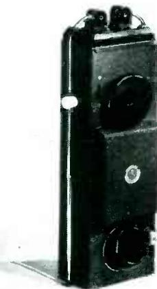
complete with batteries. It operates in the 144 to 148-mc band up to three miles or farther. Featured in the design is adjustable tuning on both transmitter and receiver.
