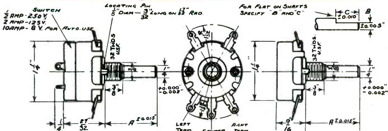
Depth from Mounting Face. Dual 1 1/4" Triple 1 1/3" For Switch Add  $\frac{9}{32}$ "
