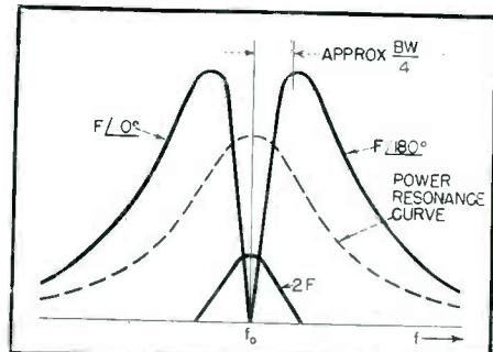
FIG. 2—Resonator-detector output
