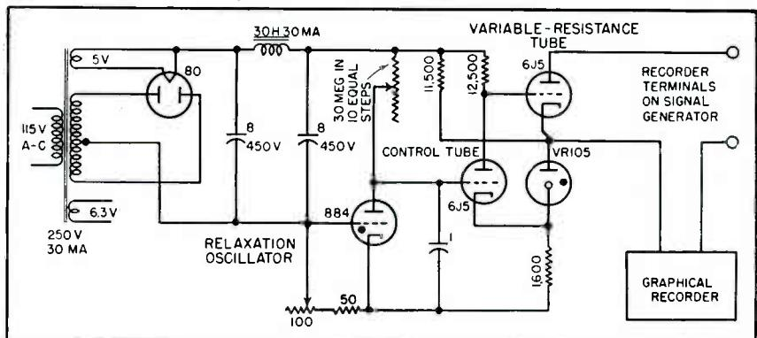
FIG. 2—Cycler circuit for sweeping pen of recorder periodically back to zero, to black in entire area between signal strength curve and zero. Rate of sweep may be varied from once per second to once every 5 seconds by adjusting 30-megohm resistor
