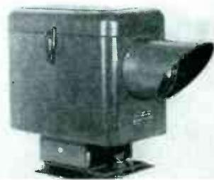
distances up to 1,000 ft. Its applications include traffic control, counting and limiting, and the like. The light source contains a lamp, transformer, and motor-driven slotted disk which modulates the light beam at about 900 cps. The relay, because of its tuned circuit, is responsive only at this frequency.
