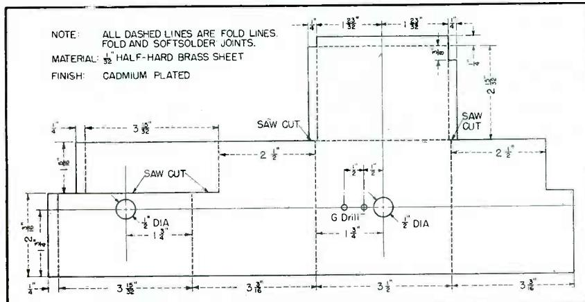
FIG. 5—Shield can for 232.5-mc resonator. Made from brass sheet, this structure can be bent into shape without machining.
