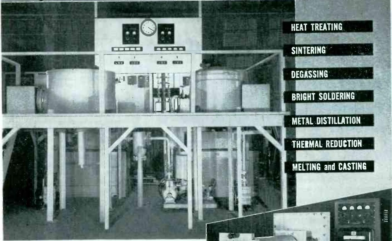
FRODUCTION FURNACES — MELTING AND CASTING
