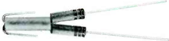
**IRC Matched Pairs**—two resistors matched in series or parallel to as close as 1% initial accuracy provide a dependable low cost solution to close tolerance requirements.
