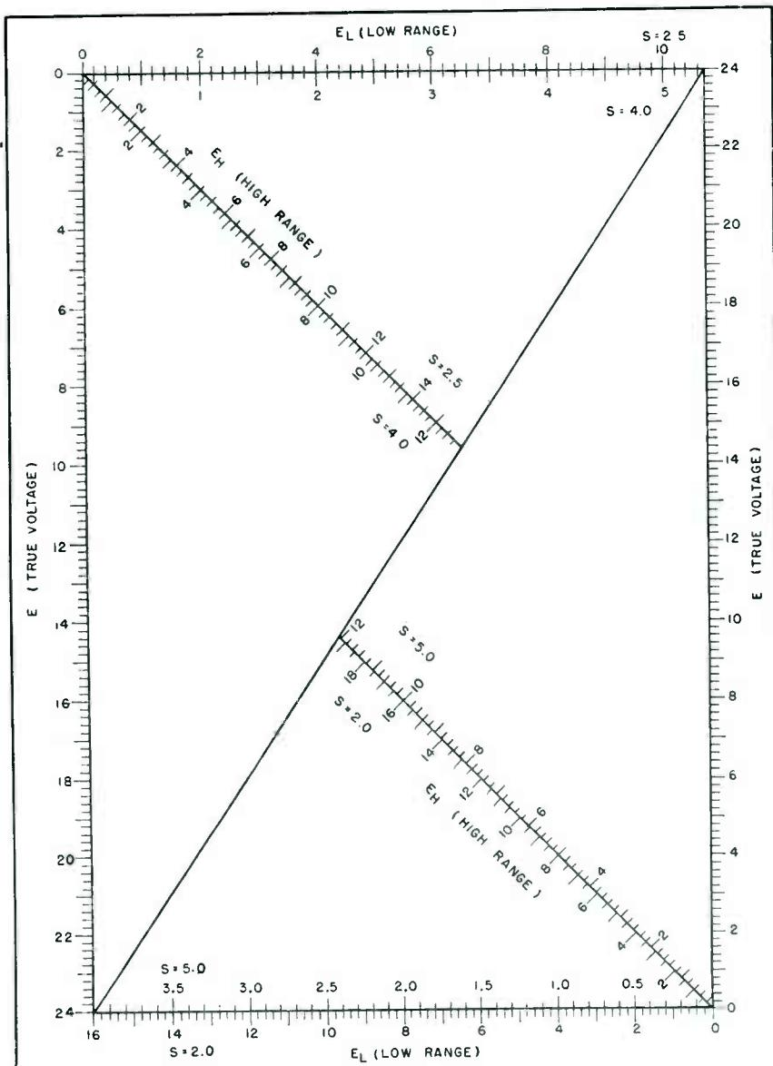
FIG. 2—Voltmeter loading nomograph. Take voltage readings on two ranges, divide higher range scale by lower to get  $S$  (either 2, 2.5, 4, or 5 on standard volt-ohm-milliammeters), then place straightedge on measured values ( $E_L$  and  $E_H$ ) for  $S$  scale in question and read true voltage on adjoining  $E$  scale. If range of any scale is inadequate, multiply all scale values by 10, 100, or any other convenient factor
