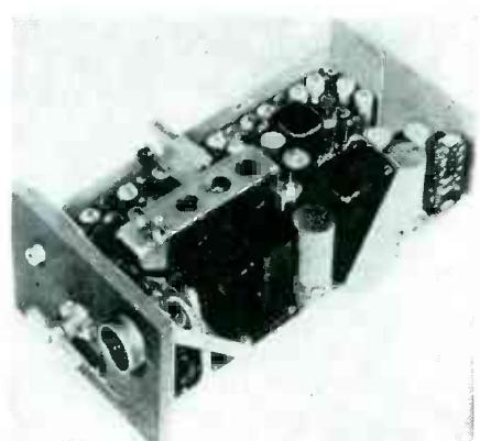
output is from 7 to 10 watts for a total transmitter drain of 20 amperes and a transmitter-receiver standby of 9.2 amperes. Full details of this equipment are available from the manufacturer.
