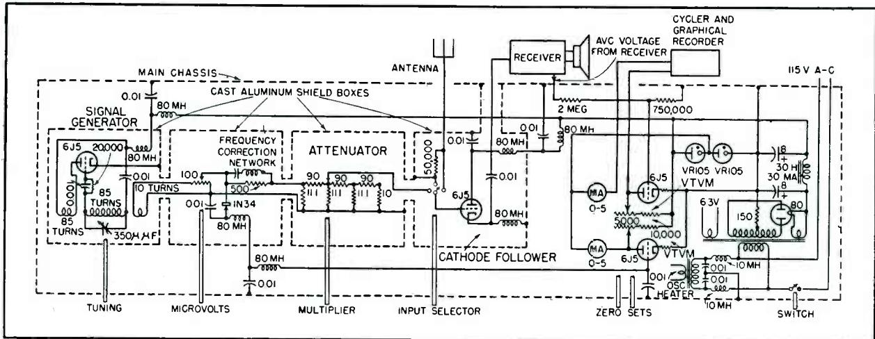
FIG. 1—Circuit of signal generator used for calibration in connection with recording of sky-wave signals, showing elaborate shielding technique employed and relationship to other units of recording system
