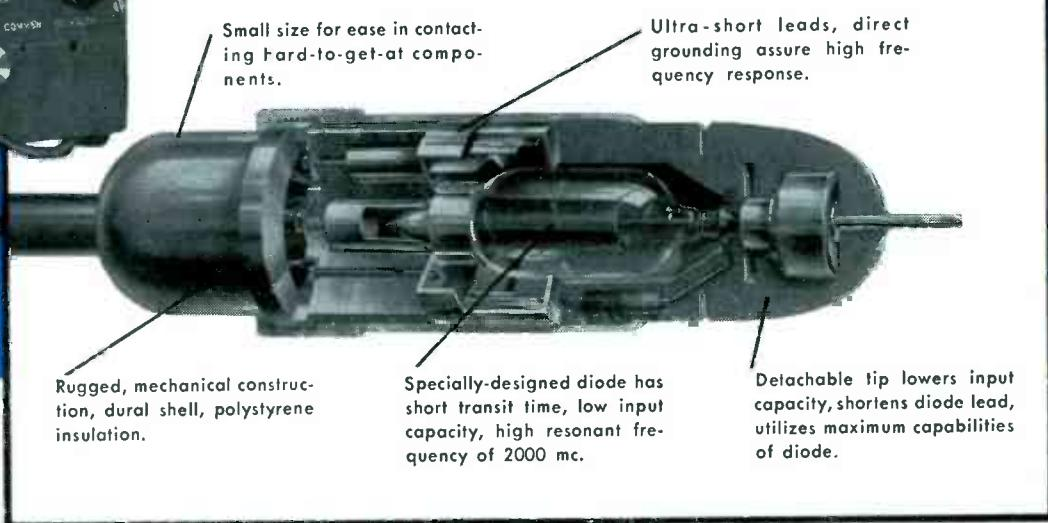
**The specially-designed diode,** in combination with the -hp- probe design, makes possible the exceedingly flat frequency response shown graphically in Figure 1.
