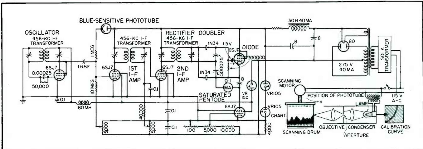
FIG. 3—Circuit of electronic scanner used for analysis of charts. Arrangement of optical system is shown at lower right; phototube is mounted on carriage along with lenses and lamp, and picks up light reflected from spot on chart
