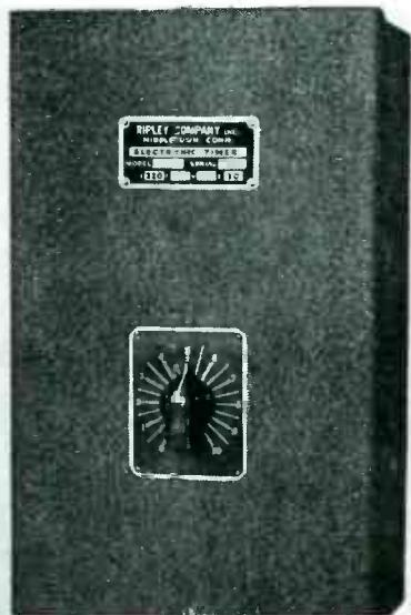
any timing range desired. Once set for a particular thickness of metal, timing becomes automatic for the entire production run.
