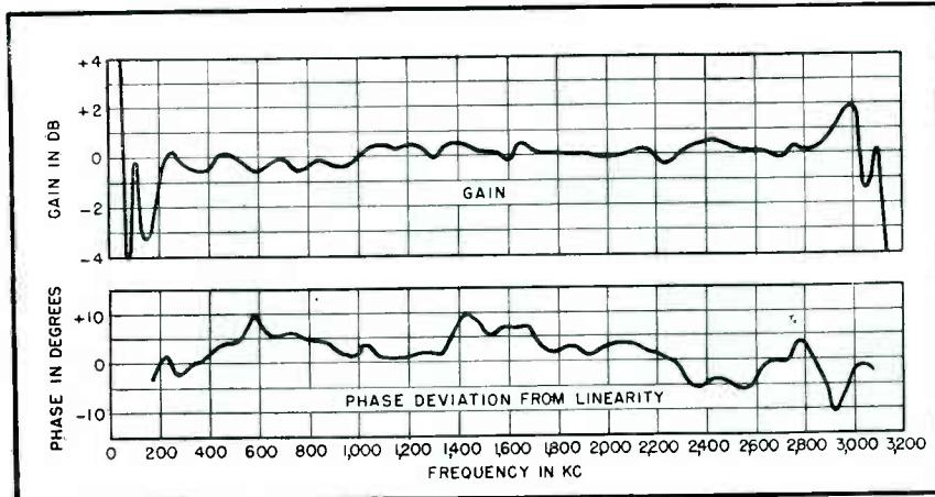
FIG. 7—Transmission and phase characteristics of the New York-Washington coaxial television circuit. Video bandwidth is limited to about 2.8 mc by the characteristics of the repeaters used
