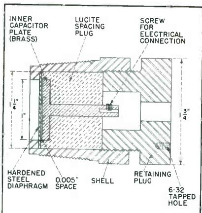
FIG. 1—Cross-section of capacitance-type pressure pickup. Sound waves act on steel diaphragm at left, causing capacitance between grounded diaphragm and insulated brass plate behind it to vary. Shell and retaining plug are turned from 1½-inch hexagonal steel stock.
