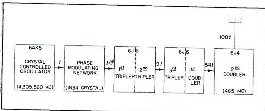
FIG. 1—Block diagram of transmitter. Tubes are conserves by operating three 6J6 triode sections as triplers. Phase modulation network produces 25-kc deviation
