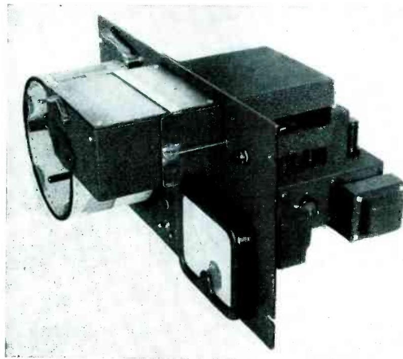
**Electronic scanner unit used at Radio Standards Office in Ottawa for analysing sky-wave charts obtained with recording equipment. Logarithmic calibration chart is placed under pointer on table just above drum. Pointer is mechanically coupled to optical system**
