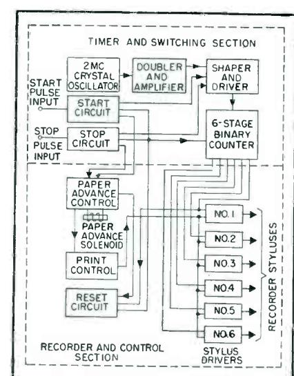
connections. The components are arranged physically in two groups and are mounted accordingly on two chassis units. The upper section contains the 4-mc source, the switching circuit, and the counter chain. The lower section contains the recorder, its control circuits, and the reset circuit which restores the upper section to its standby condition after each measurement.
