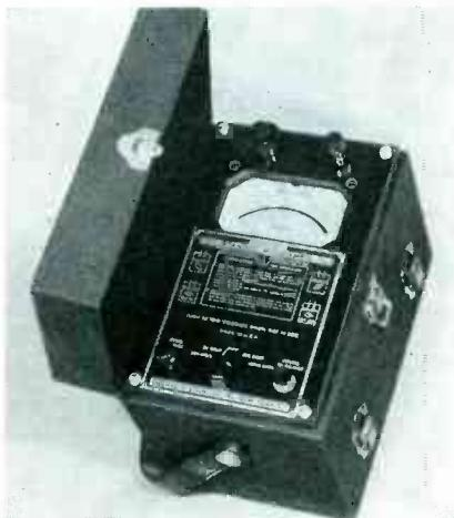
ohm scale testing to 0.1 ohm is possible. Bulletin No. 440, with complete description and pertinent information, is available on request.
