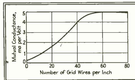
Fig. 1—Effect of pitch of grid wires on transconductance of receiving triode
