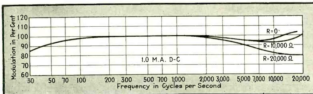
Fig. 6—Typical calibration curves at 100% modulation, 1 ma. direct current, and various values of circuit resistance
