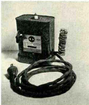
single-pole, double-throw type with silver-alloy contacts of 100 watts capacity. Relay sensitivity is controlled by a small bakelite knob on the side of the case. In operation, the antenna is connected to an insulated terminal at the top of the case. The relay may be used in a number of applications such as counting metallic objects, control of certain industrial operations, animated advertising displays, opening doors, etc. The CR-1 relay lists at \$25.00 complete.
