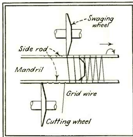
Fig. 2—Details of grid winding machine
