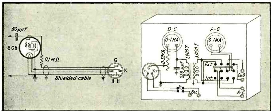
Fig. 3—Schematic wiring diagram and layout of the complete meter. The tube is connected through the shielded cable to the measuring circuit
