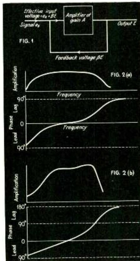
Fig. 1.—Fundamental feedback circuit, showing relation between input, output and feedback voltages
