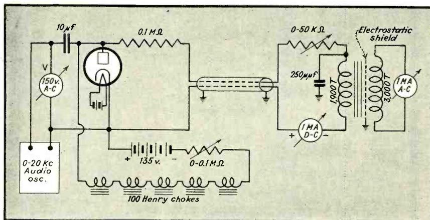
Fig. 4—Circuit arrangement for making accurate meter calibrations
