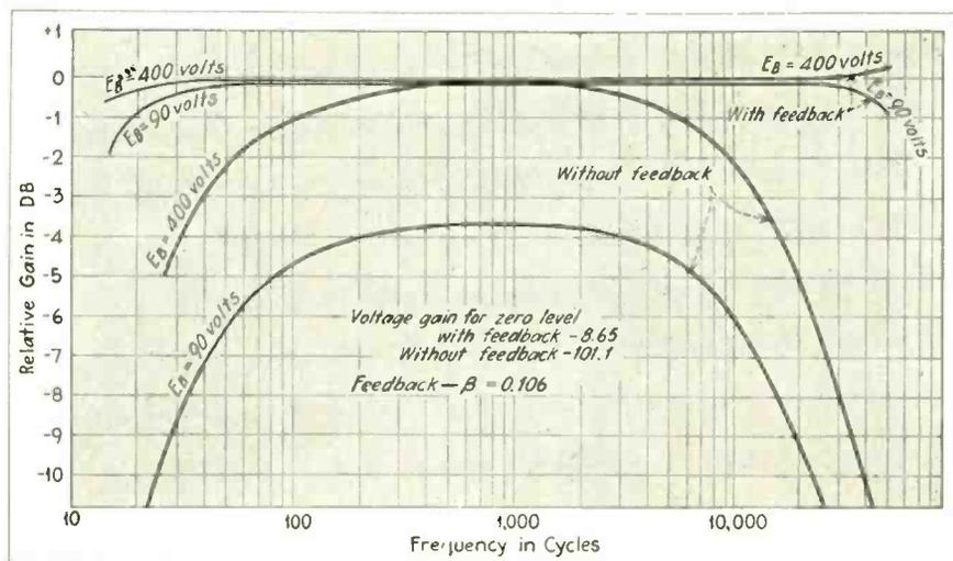
Fig. 7—Experimental characteristics of amplifier built by the author
