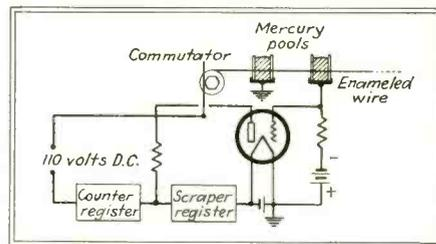
*Circuit for testing enamel wire*
