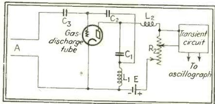
Gaseous discharge tube circuit for transient oscillograph
