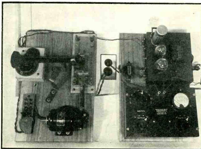
Fig. 1. Pick-up surface tester and amplifier
