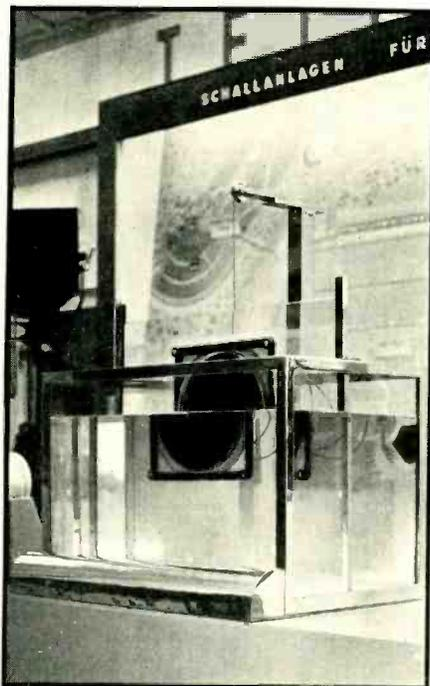
At a recent Berlin Radio Show, a water-proof speaker was shown. The demonstration above, proved its submarine qualities by dipping the unit into water while operating
