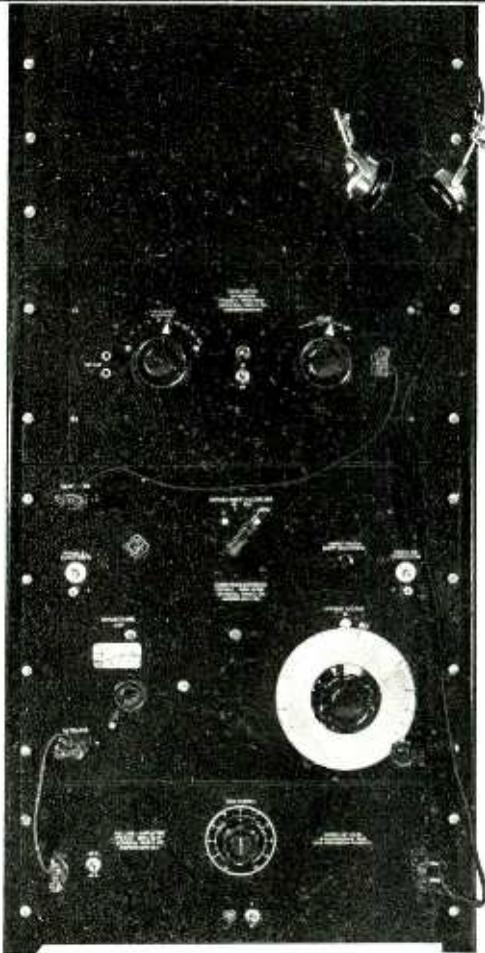
*THE assembly above is completely a-c operated. It is composed of the Type 508-A Oscillator (top), Type 716-A Capacitance Bridge, Type 714-A Amplifier and Type 480-B relay rack. Price, complete with bench-mounting relay rack (without headset), \$660.00*
