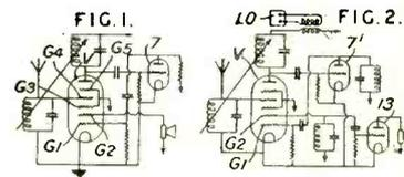
quency are fed back to another grid of the same tube for reamplification. Marconi Co. No. 439,047.
