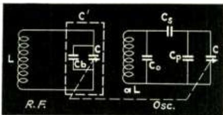
Fig. 1—Radio frequency and oscillator circuits
