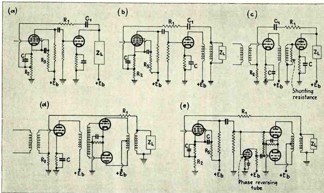
Fig. 4. Two-stage feed-back circuits. The advantages of coupling over two stages can be realized without oscillation troubles if proper procedure is followed
