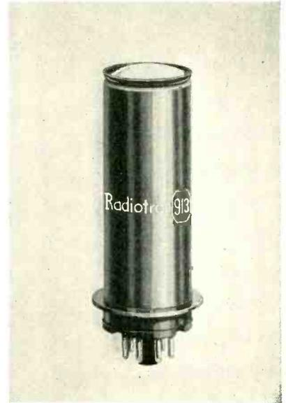
is encased in a metal can which may be grounded to eliminate the effects of local magnetic fields. The tube is provided with the standard 8-prong octal base and is designed to operate with an anode voltage of between 250 and 500 volts.
