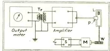
Fig. 2. Pick-up surface tester
