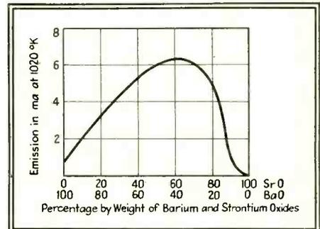
Fig. 3—Electron emission of oxide cathodes as a function of the relative percentages of barium and strontium oxides
