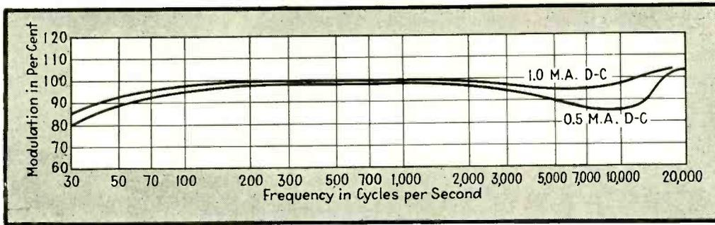
Fig. 5—Typical calibration curves at 100% modulation and carrier levels giving d-c readings of 0.5 and 1.0 milliampere
