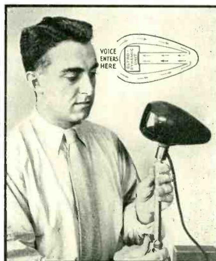
The stream-lined housing in this electrodynamic unit concentrates the sound input and, with the aid of close tolerances in the air-gap, is claimed to produce a very high output level
