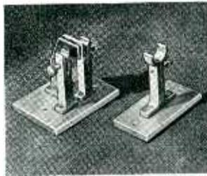
Mycalex at ultra high frequencies makes this dielectric material particularly suitable for use in sockets and other r.f. circuit components. The illustration shows a transmitting tube socket designed for the 204A, 849, 869 and 881 tubes. Large contact area of the terminals combined with their spring action and locking features insures positive tube connections.
