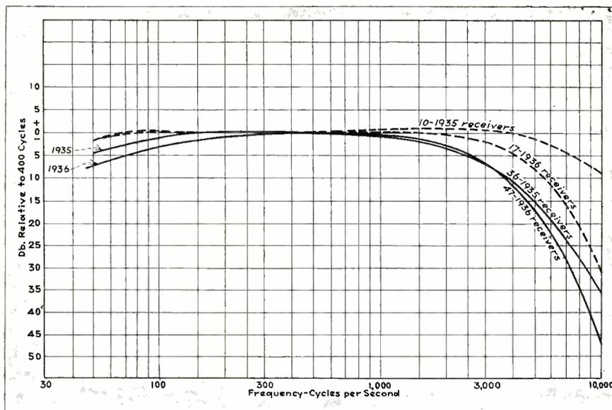
Electrical fidelity of 1935 and 1936 receivers. Dotted curves of variable selectivity receivers in the wide band position
