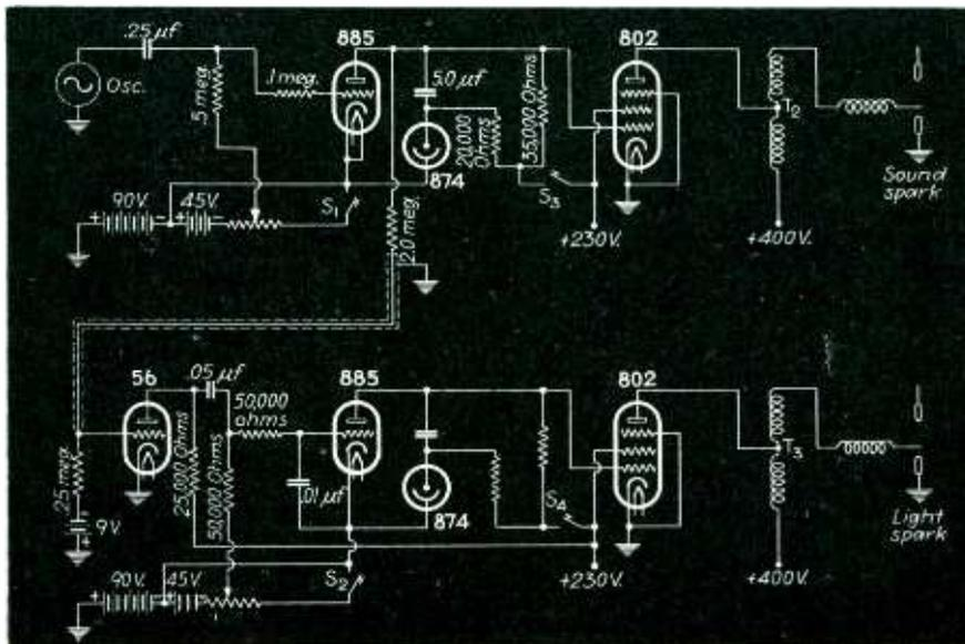
New timing circuit for sound wave photography
