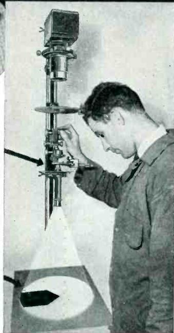
This cutting needle costs only a few cents but if it is defective it will ruin the recording of a big program. Presto engineers never take chances with needles. They examine each needle under this microscope before it is shipped to you.
