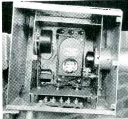
*Photronic cell cases in lightning arrestors —one of many Bakelite Molded applications in radio transmission.*
