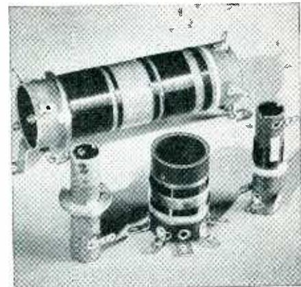
*Coils for many radio purposes are protected with Bakelite Varnish.*
