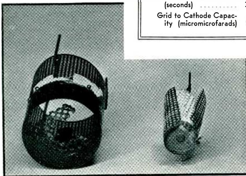
Grid (left) melted away by overload. Cathode (right) unharmed
