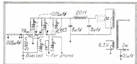
the 6E5 operates at zero bias, but the bias for the 79 tube is obtained from a Mallory cell.
