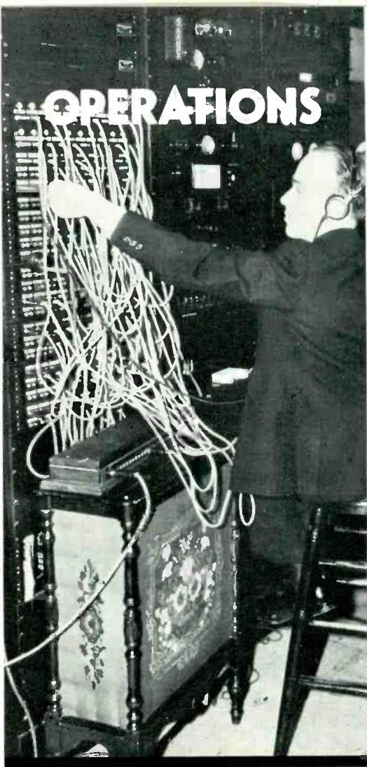
*Test board, Master Control Room, during the Stratosphere Flight. Note complicated patch-cord connections*
