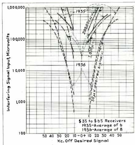
Two-signal interference measurements made at 1000 kc. on 1934, 1935 and 1936 receivers
