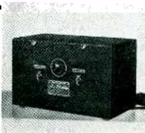
0 and 40 m. a., with line voltage 110 volts  $\pm$  10%, or 120 volts  $\pm$  10%, with load voltage variation not over 2%. Will also deliver simultaneously both 90 and 135 volts. The 90-volt tap will deliver up to 20 m. a., while the output from main section is 40 m. a. at 135 volts.
