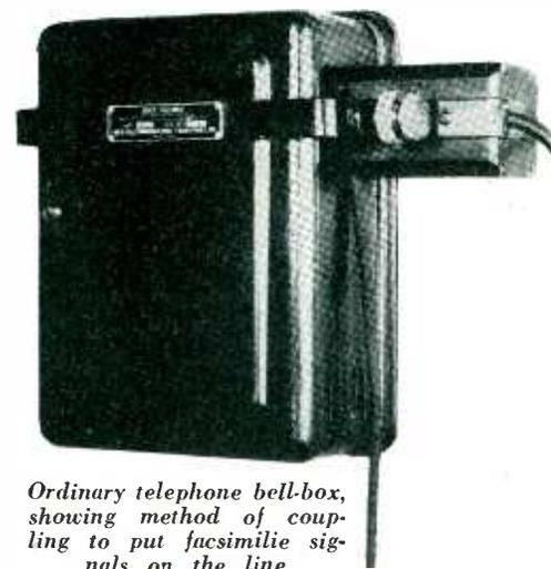
Ordinary telephone bell-box, showing method of coupling to put facsimile signals on the line
