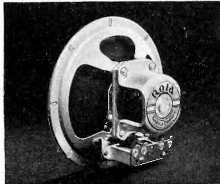
This new construction embodies a dome center cap, entirely new spider construction and novel acoustic filter assembly, which protects the voice coil and air gap against the entrance of metallic particles of dust and other foreign substances. This, however, in no way restricts the free movement of the voice coil.
