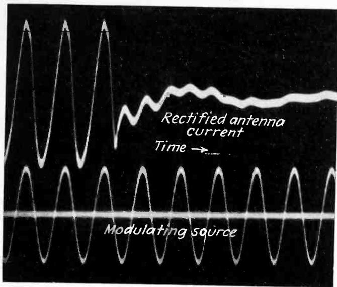
Fig. 3a—Transient occurring with sudden removal of modulation
