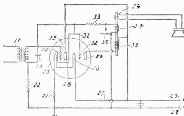
**Modulation system.** Modulation circuit employing a light sensitive cell as modulating means. Tomomasa Nakashima and Kenjiro Takayanagi, Hamamatsu-Shi, Japan. No. 1,953,769.
