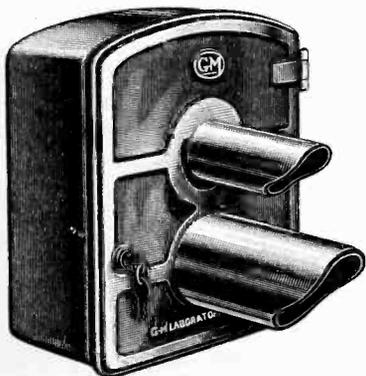
circuits can be furnished with this unit to provide the best operation for a given photoelectric installation. Light from a lamp behind the upper visor is focused on a weather-protected mirror 20 feet distant, and reflected onto a photoelectric cell behind a lens in the lower visor. Any interruption of the light beam signals a watchman in charge of the entrance where the unit is located. The circuit is designed for operation on standard 110-volt lines.—*Electronics*.
