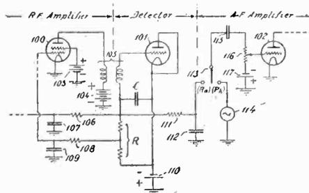
**Automatic volume control.** Two patents granted to P. O. Farnham assigned to R.F.L., Inc. No. 1,953,553 involving a multi-stage radio frequency amplifier, the final stage working into a demodulator, the rectifier elements of the gain control included in the tube of the final
