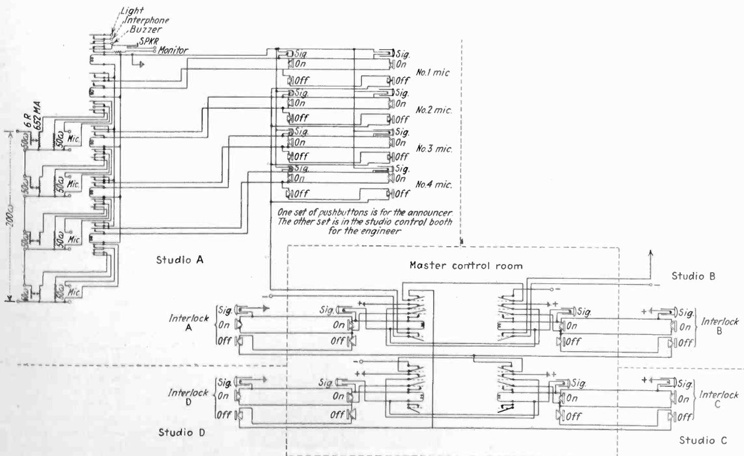
Fig. 2—Four-studio interlocking switching system. The local microphone control circuit is shown complete in studio A; the others are identical in form
