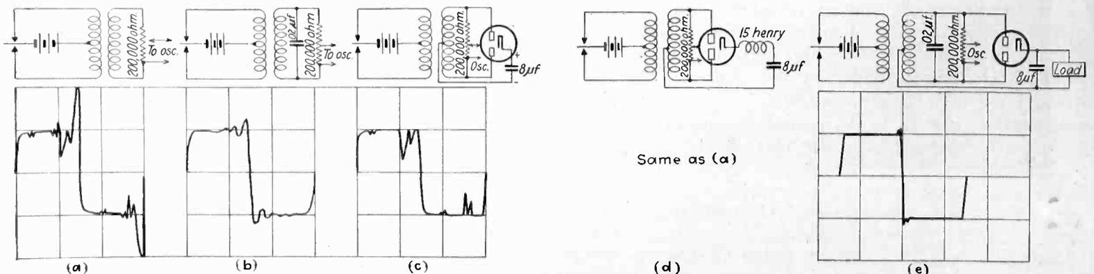
Fig. 3—Effect upon wave shape of varying circuit conditions, as shown by cathode ray oscillograph.
