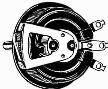
The wire winding is rigidly held in place by vitreous enamel which also covers the refractory base. The contact shoe, of special metal graphite composition, contacts the wire-wound element on the outside diameter. The rating is 50 watts with total resistance in circuit, and standard resistance values are provided ranging from 1 to 5,000 ohms. The manufacturer is Electrad, Inc., 175 Varick Street, New York City. —*Electronics*.
