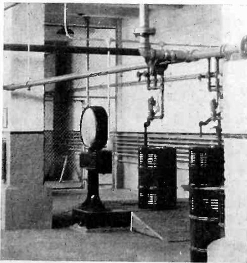
AT THE GREAT PLANT of the New England Alcohol Company, at Everett, Mass., with an output of 3,000,000 gallons of alcohol per year, made from molasses, a photo-cell on a scale beam permits the automatic filling of the steel
