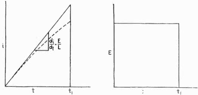
Fig. 1 (left)—Rate of increase of current with time.
