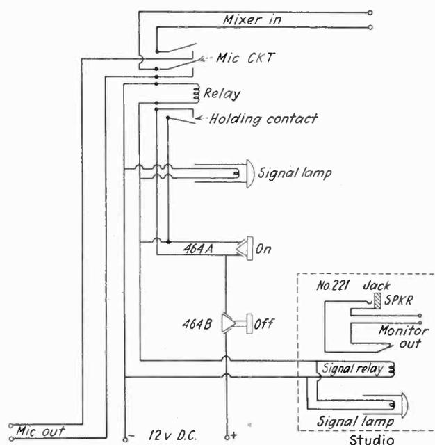
Fig. 1—Fundamental switching circuit.
