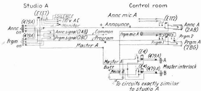
Fig. 3—Studio and microphone interlock switching system.
