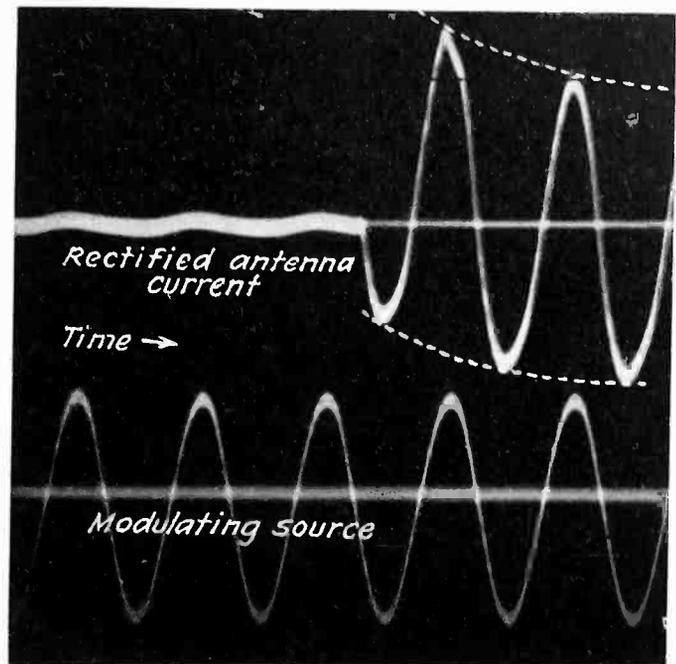
Fig. 3b—Transient on start of modulation
