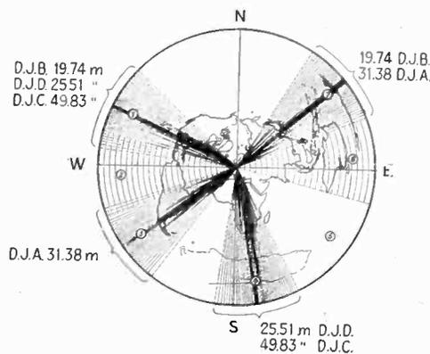
arranged in the same plane one above the other and one beside the other to form 4 half-wave dipoles in a line, all dipoles being supplied in exact phase (H8/4R antennas). The strength in day-time is 64 times that given by a simple vertical dipole. Modern high frequency cables connect the two remodeled 20 kw. transmitters to the antennas.—*El. T. Zeits.* 55 (11): 265-267, 1934.—*T.F.T.* 23 (2): 38-46, 1934.
