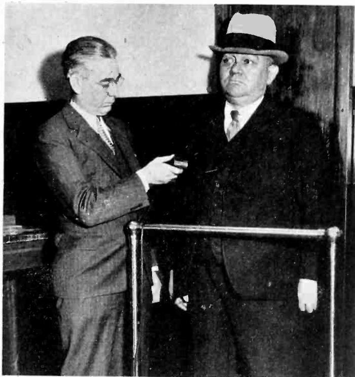
Prisoners taken into the Chicago Detective Bureau can now be "frisked" for concealed weapons by means of this magnetic exploring device, with tube amplifiers operating an alarm. The main wall-plate detects the presence of any iron or steel, even a saw-blade on a prisoner, and the small exploring coil permits localizing the metal body or weapon
