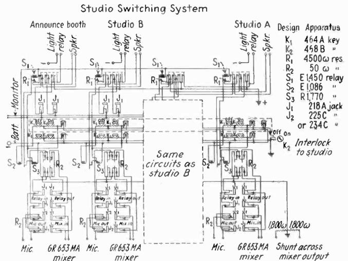
Fig. 4—Circuit for individual control room and studio switching control.
