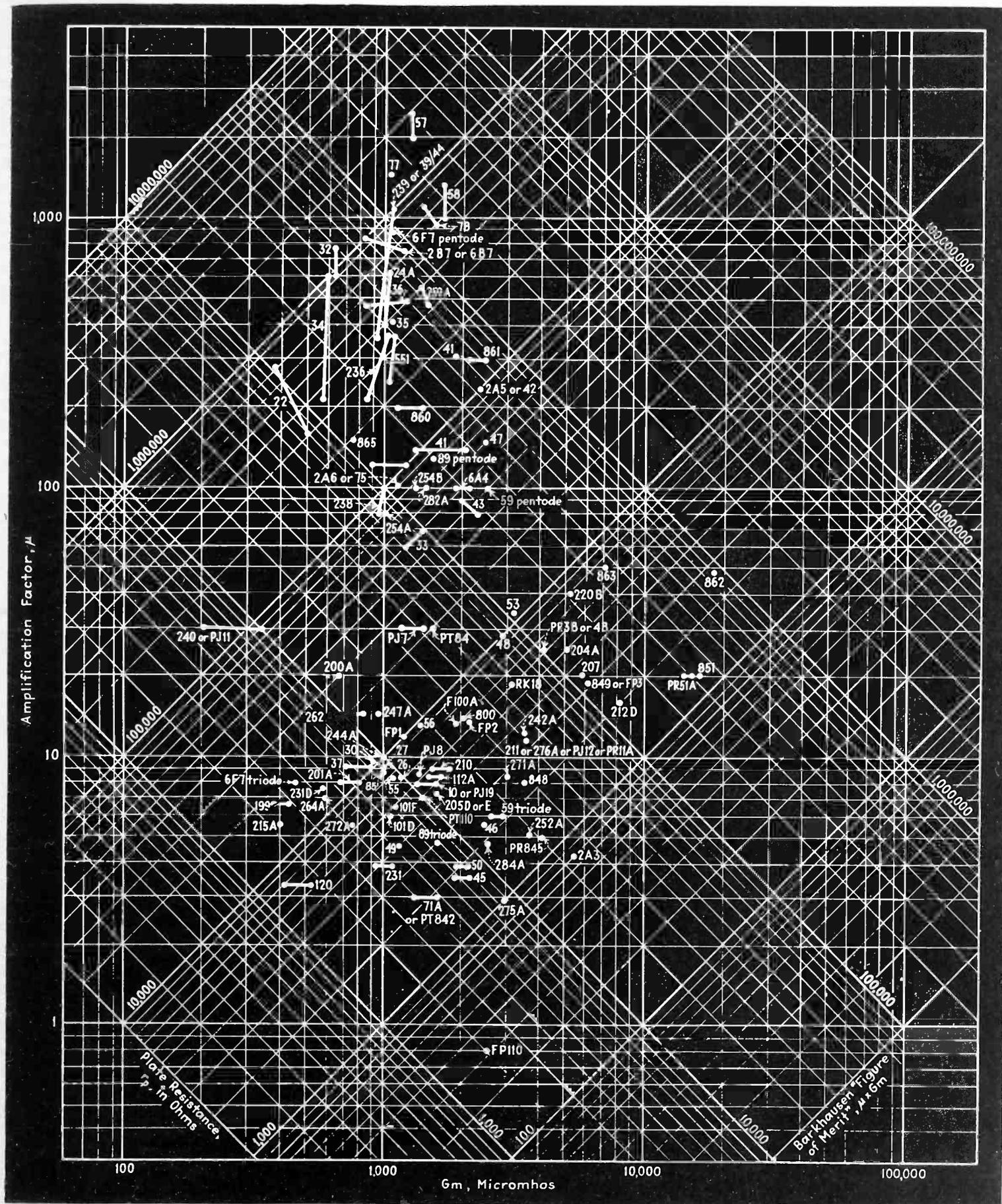
Important electrical constants of many of present-day vacuum tubes will be found on the above chart prepared by Professor H. R. Mimno of Harvard University. His remarks on the origin of this method of showing tube constants will be found on page 158 of this issue of Electronics, in which he uses the term "Sp" for mutual conductance.
