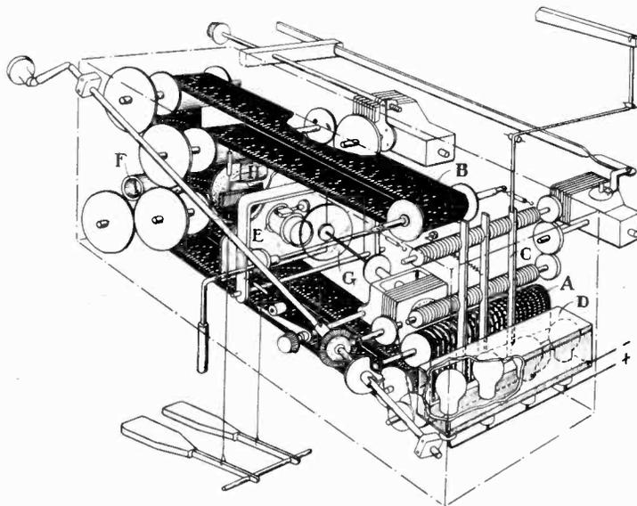
Diagram of one of the units, showing "quality" film *A* and "pitch" film *B*. Photo-cell pickup is at *F*
