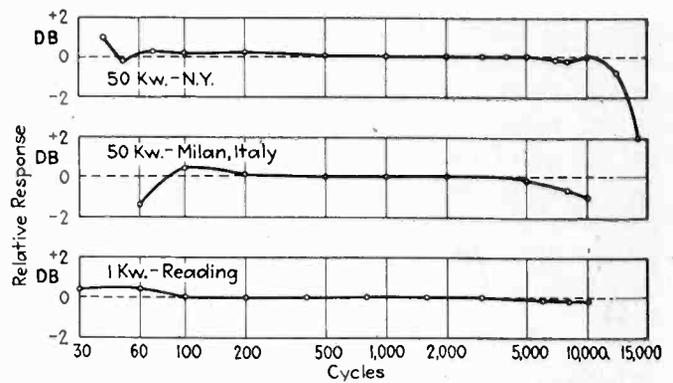
Fig. 1—Over-all characteristics of modern transmitters
