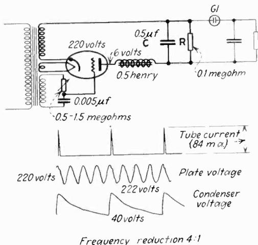
when used with a glow discharge tube,  $GI$ , for stroboscopic purposes. Grid-controlled discharge tubes filled with argon, work satisfactorily.—*Phys. Zeits.* 35, (7); 275-278, 1934.
