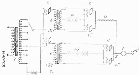
**Electrooptic control system.** A circuit employing a medium for partially transmitting a beam of light in a photocell with a split anode and method of varying the distance of the reflecting surface from the transmitting medium. A. M. Nicolson, Communication Patents, Inc. No. 1,951,523.
