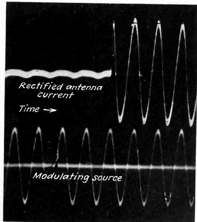
Fig. 4—Result of improving transmitter to eliminate transients
