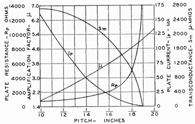
Fig. 3—Relation between the grid pitch of a triode and its characteristics
