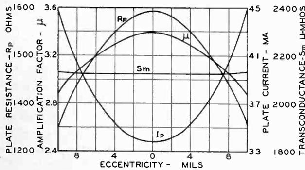
Fig. 2—Effect of plate eccentricity upon the characteristics of a triode
