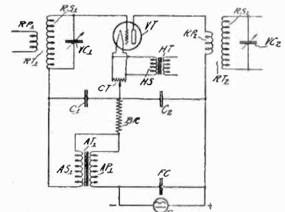
**Cold cathode amplifier.** Circuit which is described more fully under British patent granted to J. M. Schmierer, assigned to Radio Patents Corp. No. 1,838,871.
