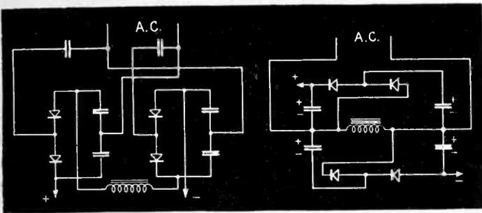
Fig. 4—Two circuits evolved in the development of a voltage-quadrupler
