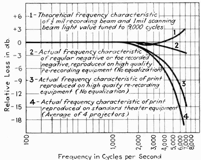
Fig. 4—Comparison of theoretical and actual losses in sound system
