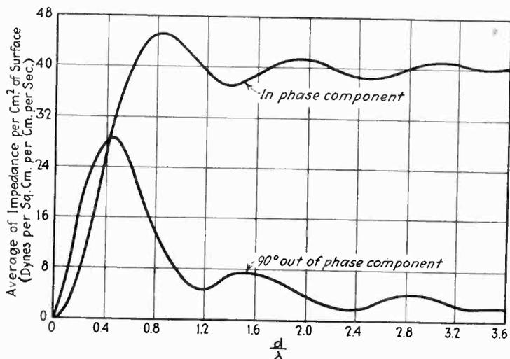
Fig. 1—Load on a vibrating circular diaphragm set in an infinite baffle
