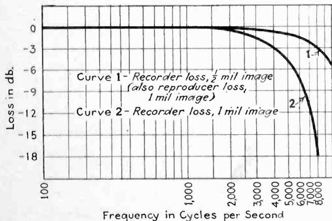
Fig. 2—Theoretical film transfer loss characteristics
