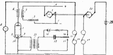
**Grid glow tube control.** In the anode circuit of the grid glow tube is a relay. Between control electrode and anode are photo-electric cells, and between cathode and control electrode is a series impedance. J. V. Breisky and E. O. Erickson, assigned to Westinghouse E. & M. Co. No. 1,839,864.
