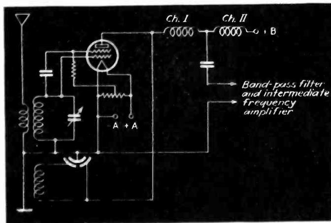
short wave but have little effect on the intermediate frequency (about 30 kc. was used). The second must on the other hand block this frequency—it can be replaced by a circuit tuned to it.—*L'Onde Electrique, Paris, October (published November 8), 1931.*
