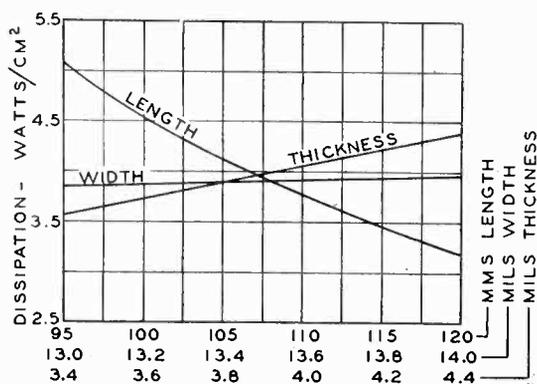
Fig. 1—Relation between filament dimensions and power dissipation in a triode
