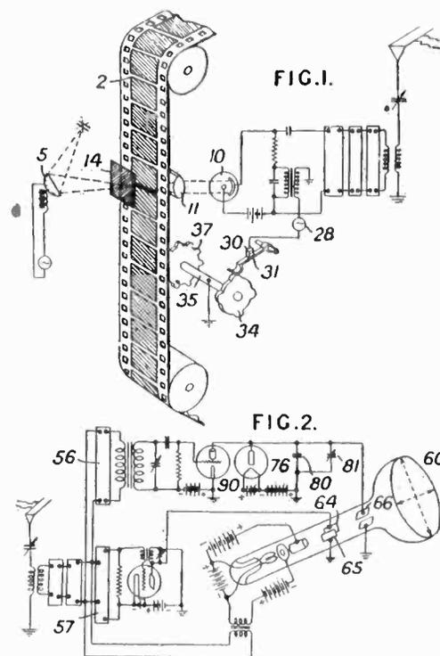
**Glow lamp screen.** Linear glow lamps which light up successively under control of voltages applied through time-lag circuits. O. von Bronk, Berlin. No. 836,760.
