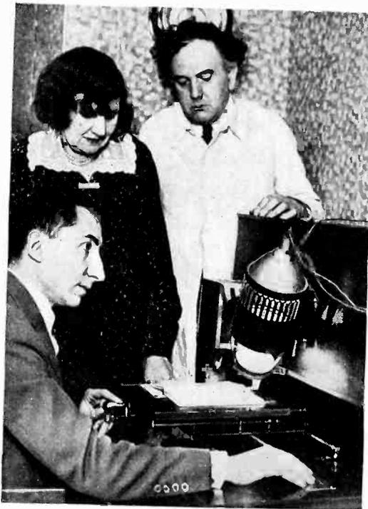
M. Thomas, a French engineer, has invented an apparatus which enables blind people to read ordinary books. The principle of the new invention is a photoelectric cell
