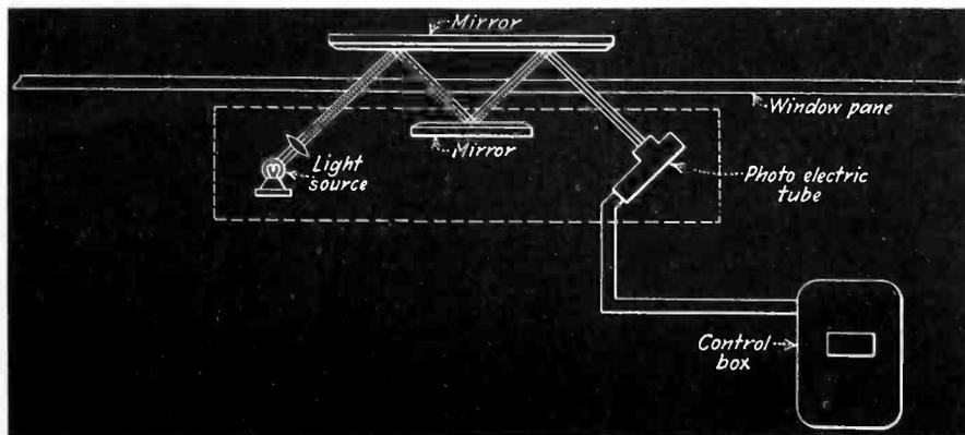
Moisture on the window pane interferes with light beam's passage to electric eye, controlling humidifier
