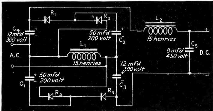
Fig. 5—Constants of the commercial voltage-quadrupler
