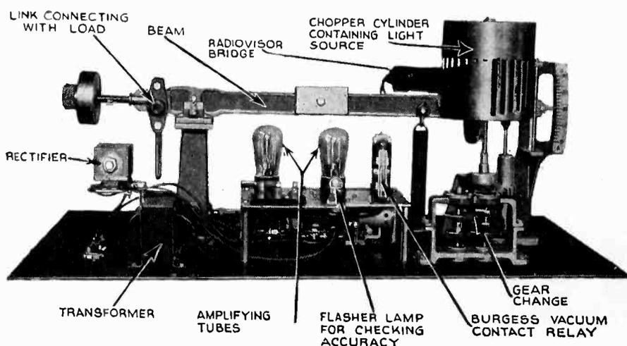
The telepoise with its light-sensitive selenium bridge which indicates the number of interruptions by the "chopper" cylinder
