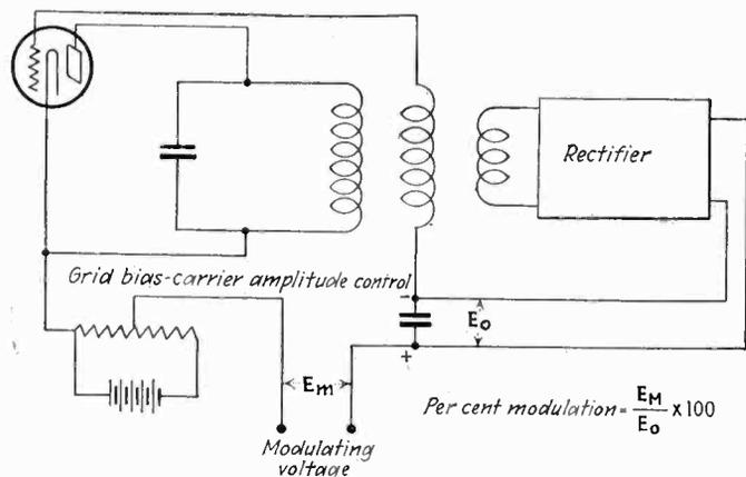
Diagram of Arguimbau method of obtaining constant output
