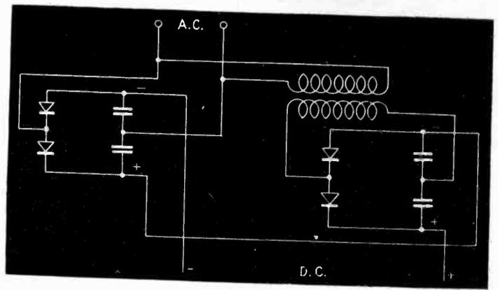
Fig. 3—Preliminary attempt to double the output voltage
