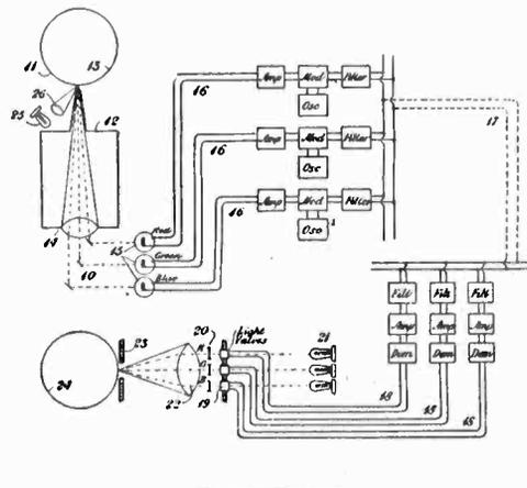
**Recording system.** A method of projecting a recording fluid toward a record surface, in accordance with the received signals. R. H. Ranger, assigned to RCA. No. 1,841,452.
