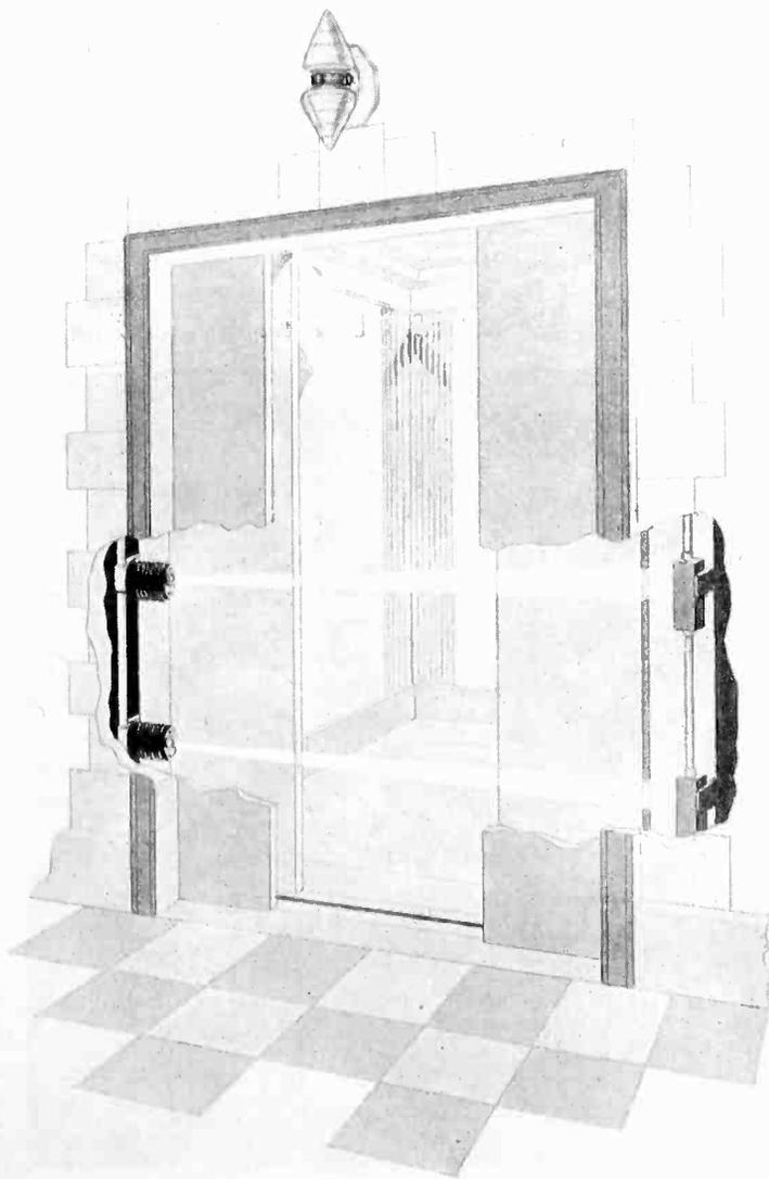
Phantom view of "electric-eye" and light projector for "Safe-T-Ray" equipment
