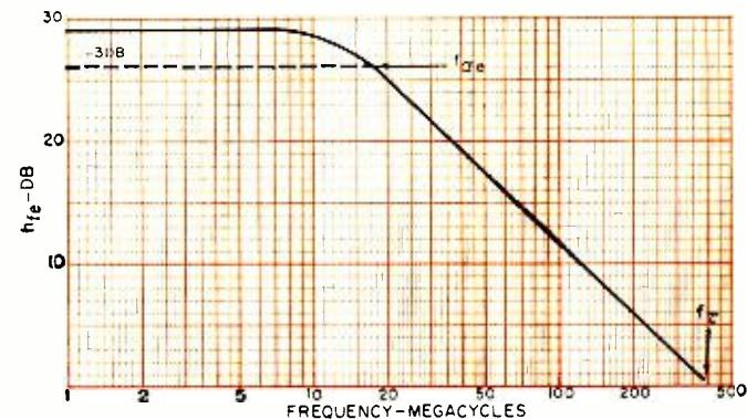
Fig. 3. Current gain vs frequency for a typical transistor.
