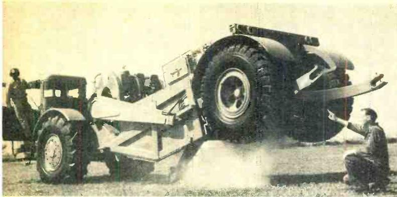
Fig. 1. A gas-explosion chamber built into this 18-ton vehicle is used to produce an acoustic shock wave for oil exploration.
