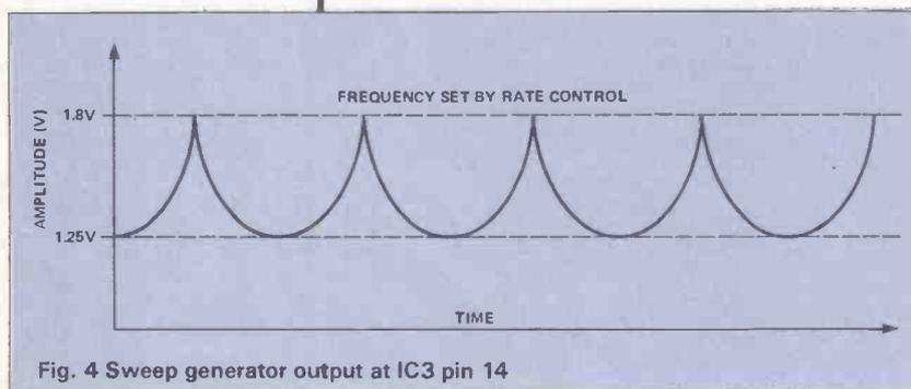
Fig. 4 Sweep generator output at IC3 pin 14
