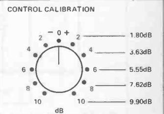
Fig. 15 Calibration of the input level control
