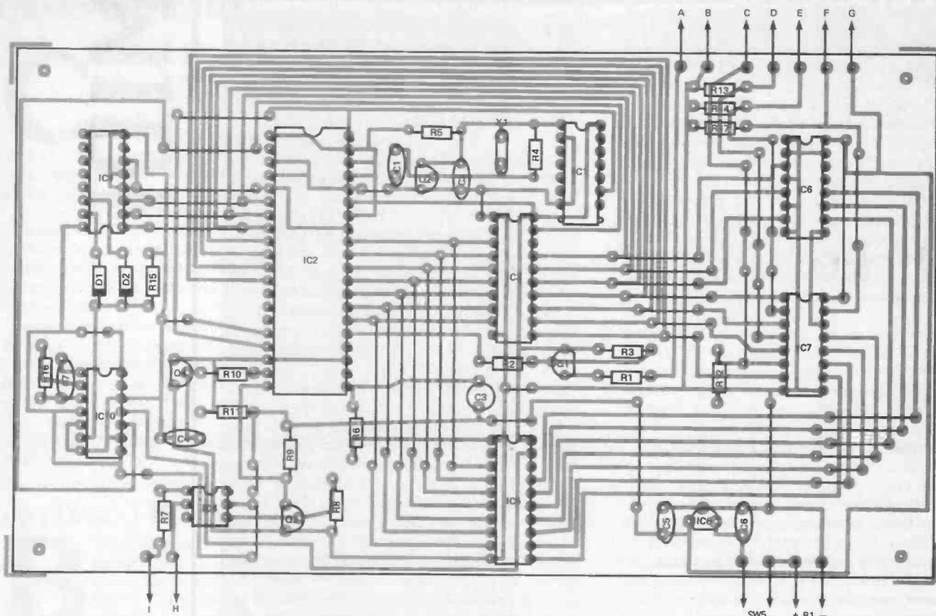
Fig. 4 The component overlay for the MIDI harmoniser
