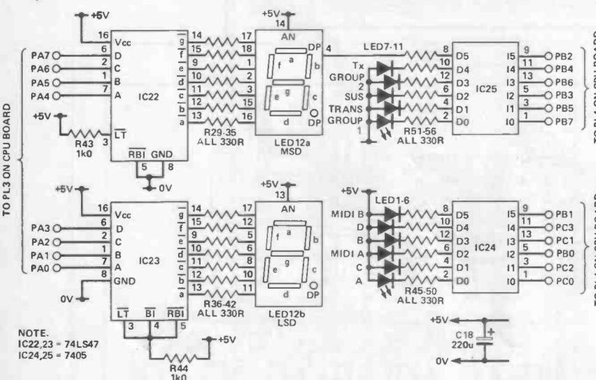
Fig. 12 The circuit diagram for the front panel board
