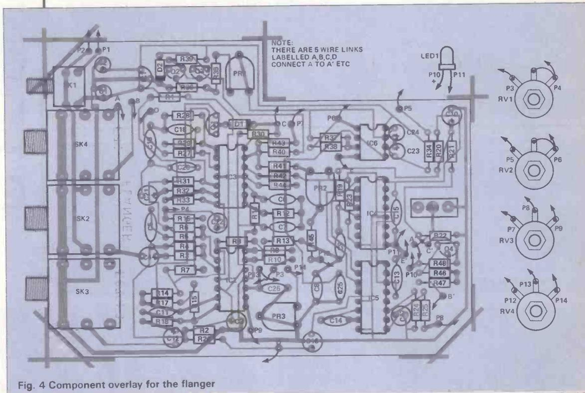
Fig. 4 Component overlay for the flanger
