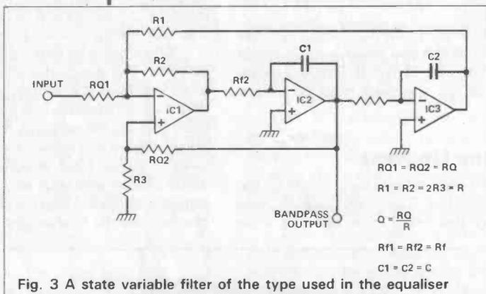
Fig. 3 A state variable filter of the type used in the equaliser
