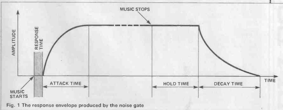
Fig. 1 The response envelope produced by the noise gate
