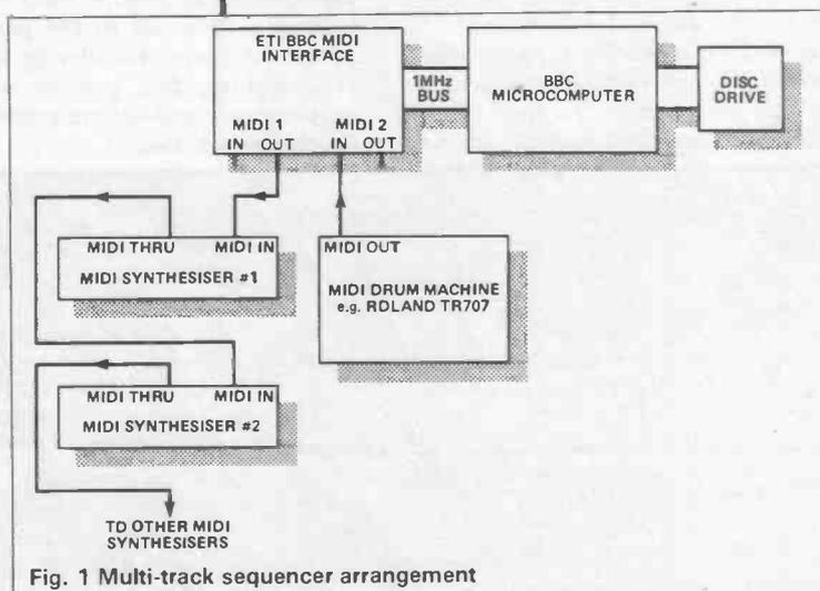
Fig. 1 Multi-track sequencer arrangement
