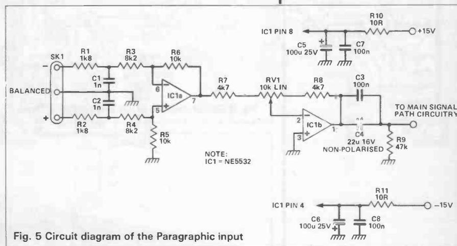
Fig. 5 Circuit diagram of the Paragraphic input
