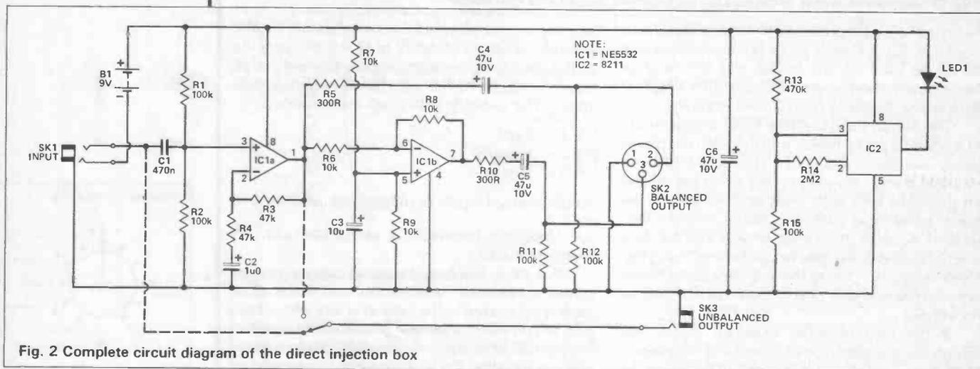
Fig. 2 Complete circuit diagram of the direct injection box
