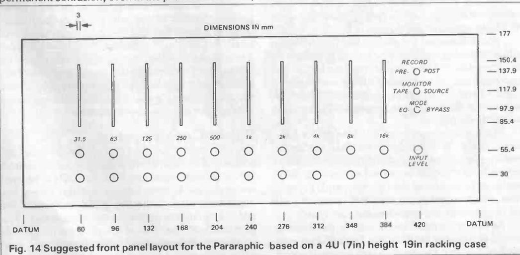
Fig. 14 Suggested front panel layout for the Paraphic based on a 4U (7in) height 19in racking case
