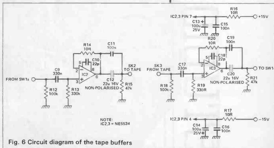
Fig. 6 Circuit diagram of the tape buffers
