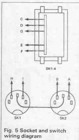
Fig. 5 Socket and switch wiring diagram
