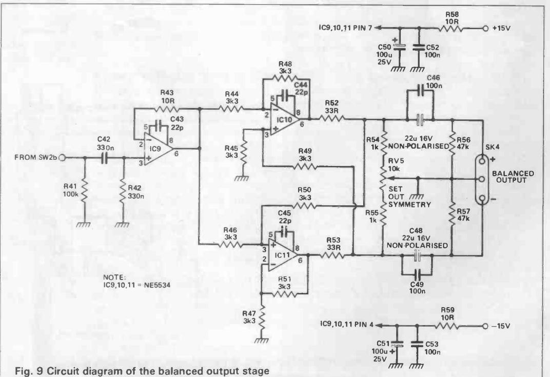
Fig. 9 Circuit diagram of the balanced output stage
