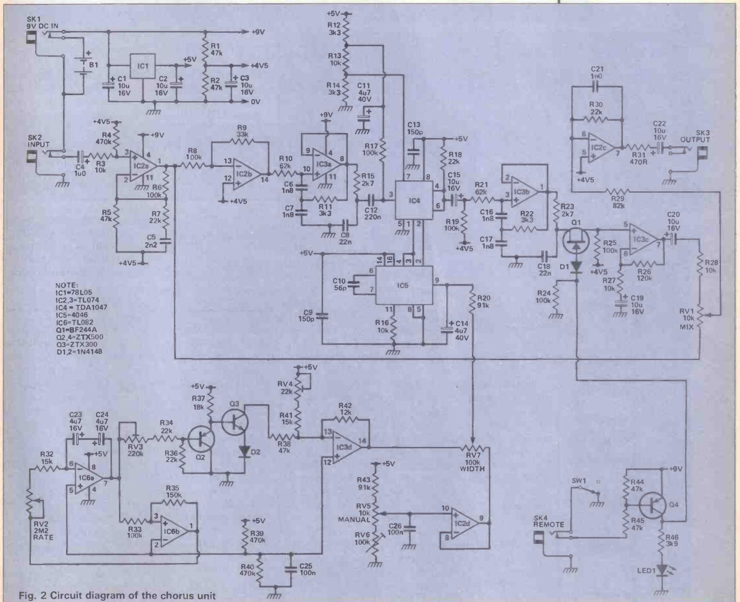
Fig. 2 Circuit diagram of the chorus unit
