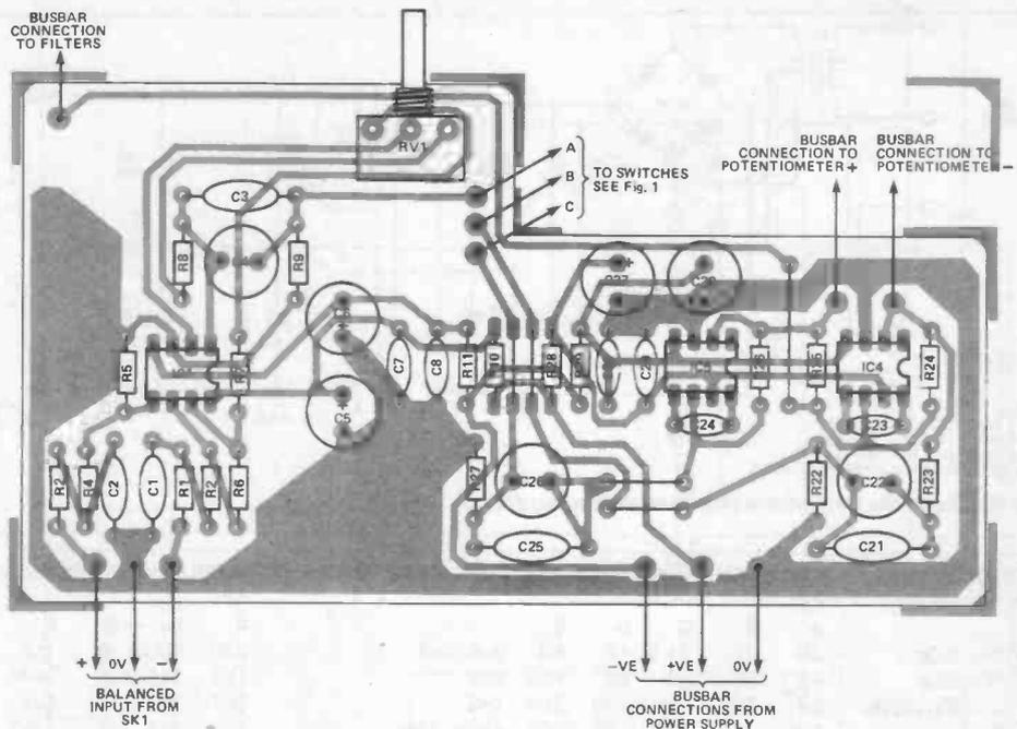
Fig. 12 Component overlay of the input stage and main signal path PCB
