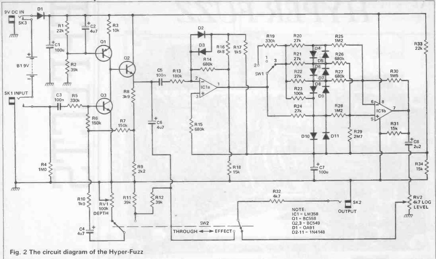
Fig. 2 The circuit diagram of the Hyper-Fuzz
