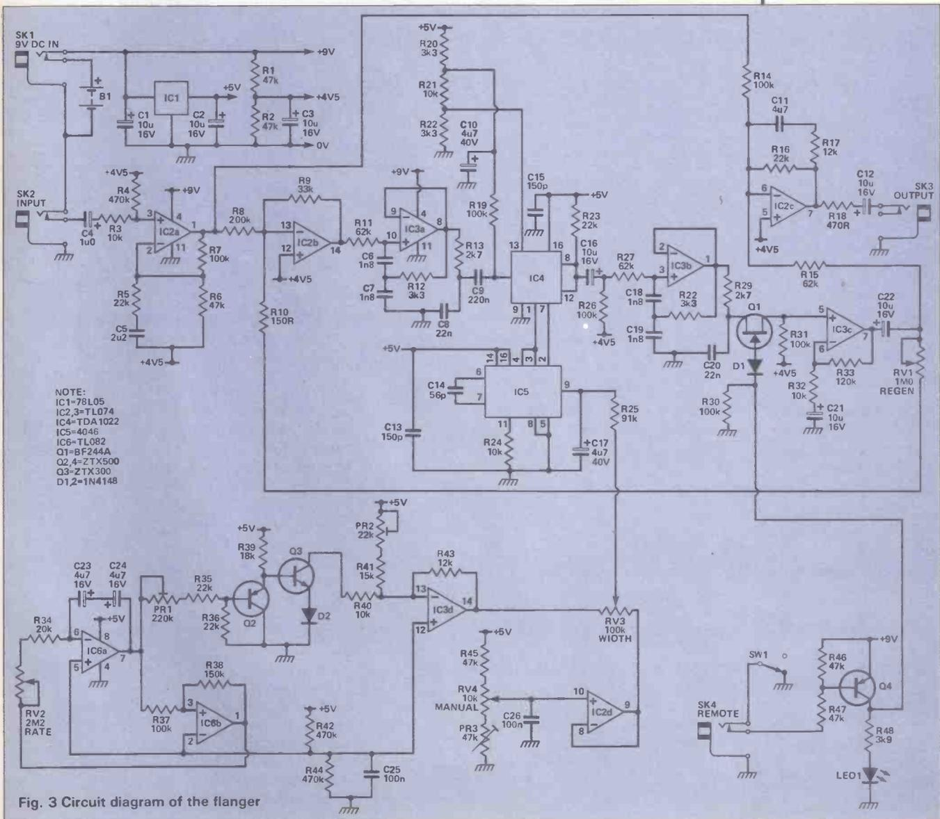
Fig. 3 Circuit diagram of the flanger
