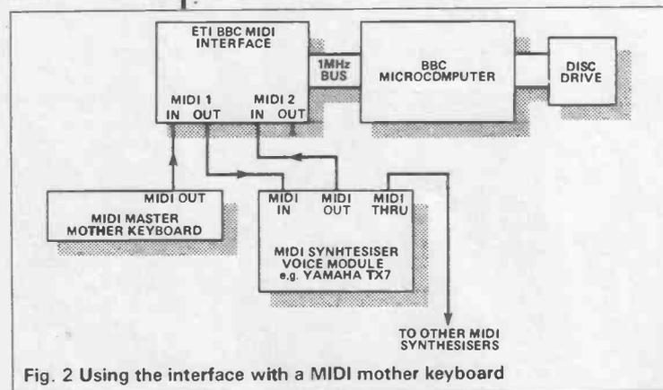
Fig. 2 Using the interface with a MIDI mother keyboard
