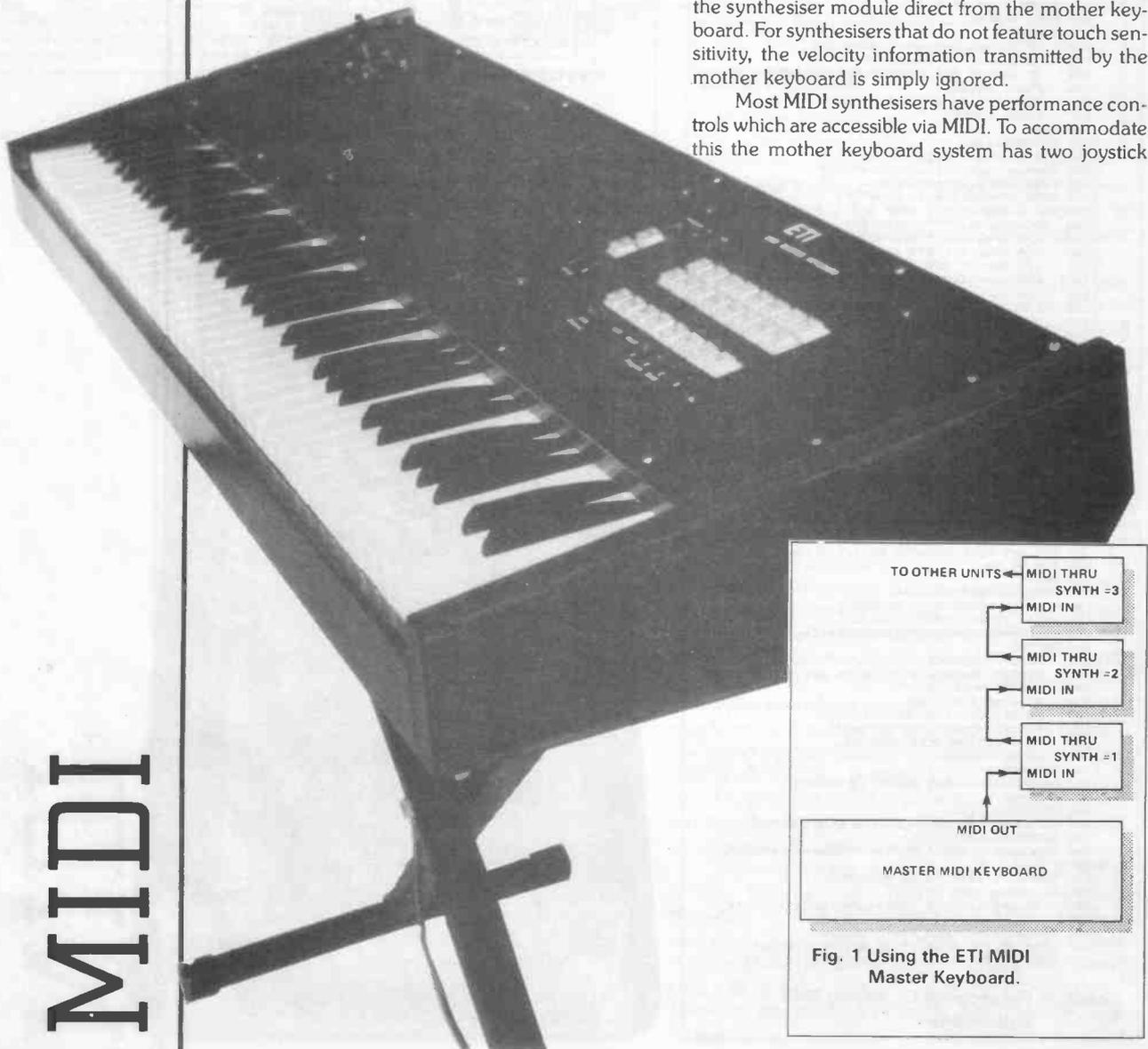
Fig. 1 Using the ETI MIDI Master Keyboard.
