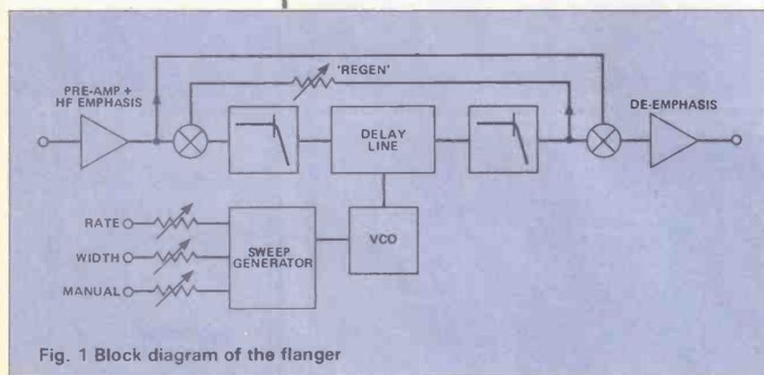
Fig. 1 Block diagram of the flanger
