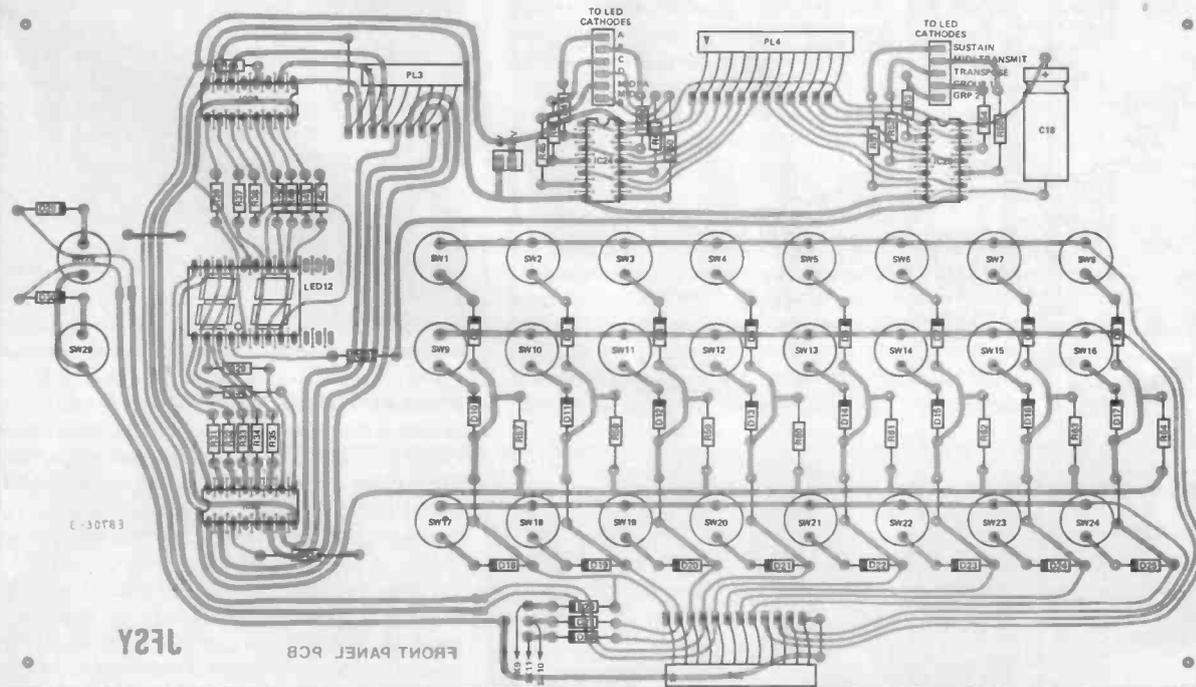
Fig. 10 The component overlay for the front panel board
