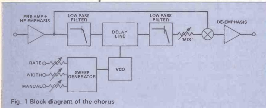
Fig. 1 Block diagram of the chorus
