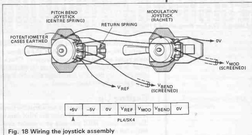
Fig. 18 Wiring the joystick assembly
