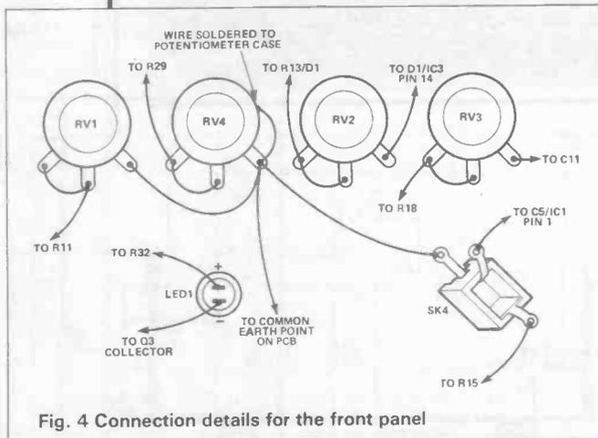
Fig. 4 Connection details for the front panel
