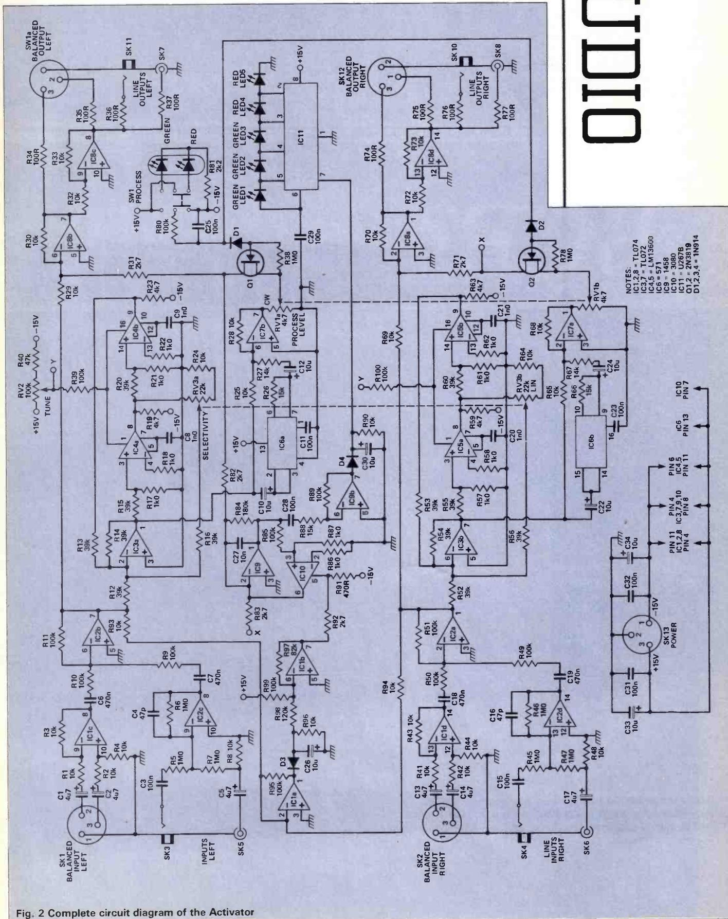
Fig. 2 Complete circuit diagram of the Activator
