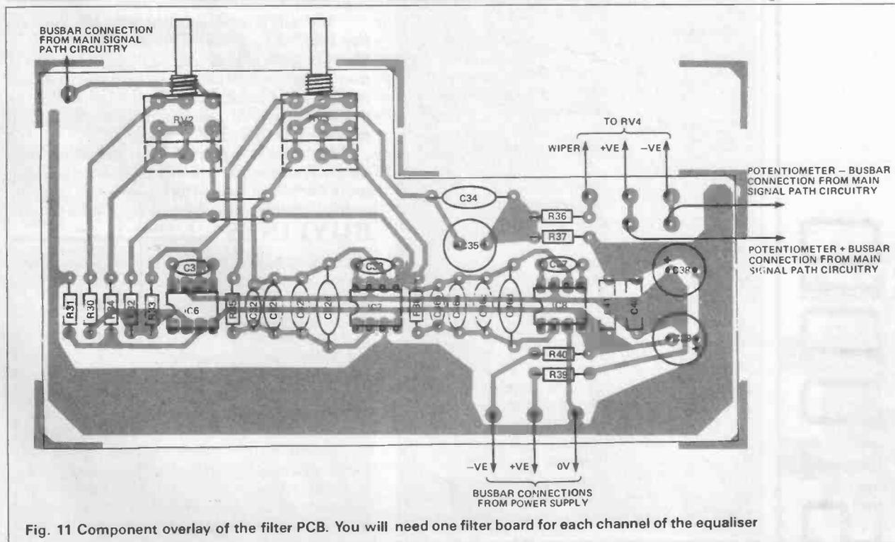
Fig. 11 Component overlay of the filter PCB. You will need one filter board for each channel of the equaliser
