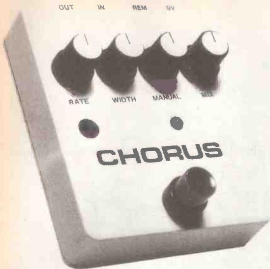
Further versatility is provided by a *Mix* control which allows the delayed and undelayed signals to be mixed in any proportions. This makes it possible, for example, to use the full amount of sweep but still achieve a very subtle effect.
