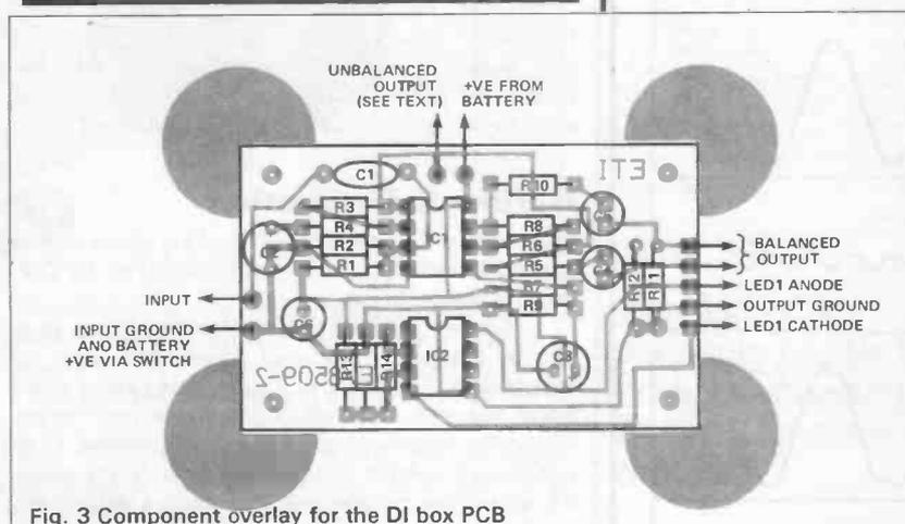
Fig. 3 Component overlay for the DI box PCB
