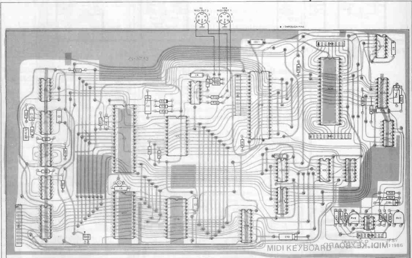
Fig. 7 The component overlay for the CPU board
