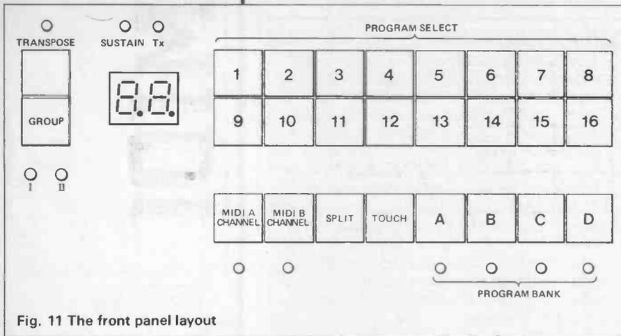
Fig. 11 The front panel layout
