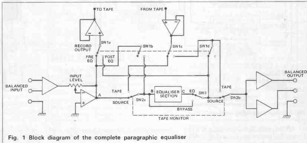
Fig. 1 Block diagram of the complete paragraphic equaliser
