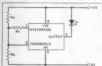
Fig. 1 Low voltage warning circuit using the Intersil ICL8211
