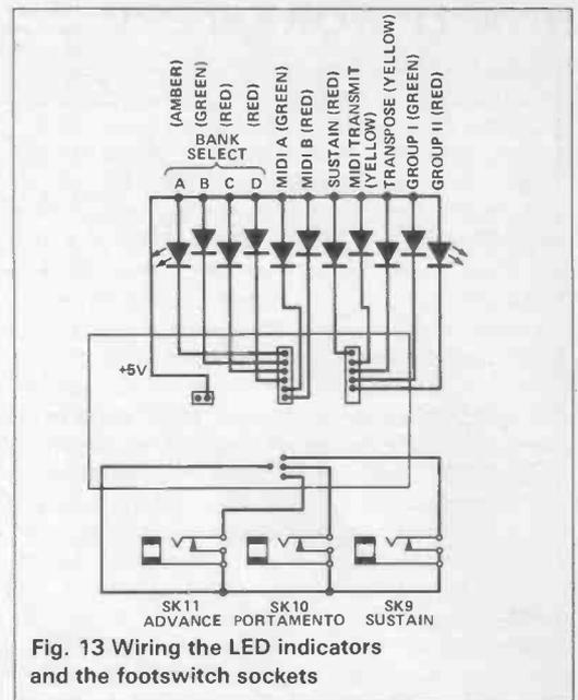
Fig. 13 Wiring the LED indicators and the footswitch sockets
