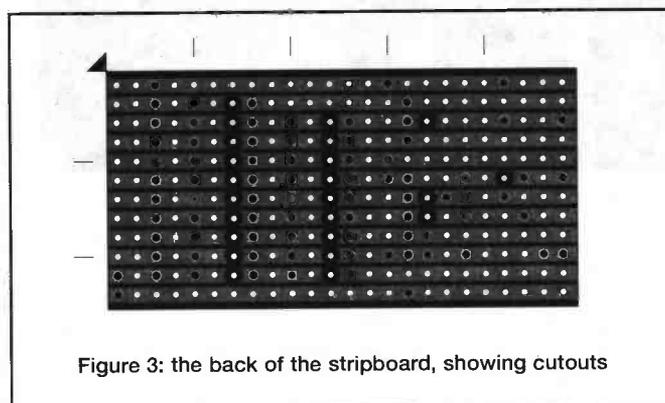
Figure 3: the back of the stripboard, showing cutouts
