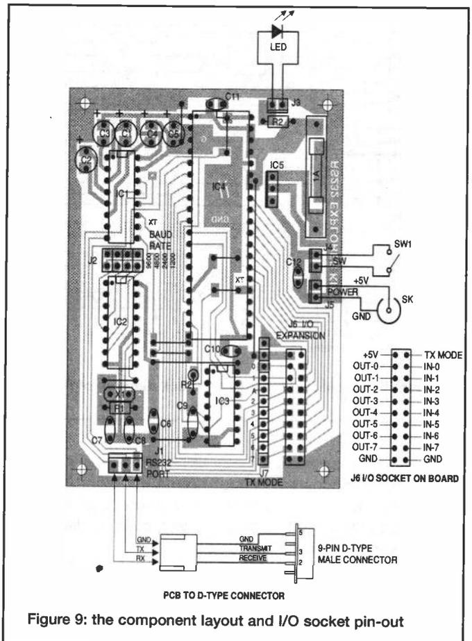
Figure 9: the component layout and I/O socket pin-out
