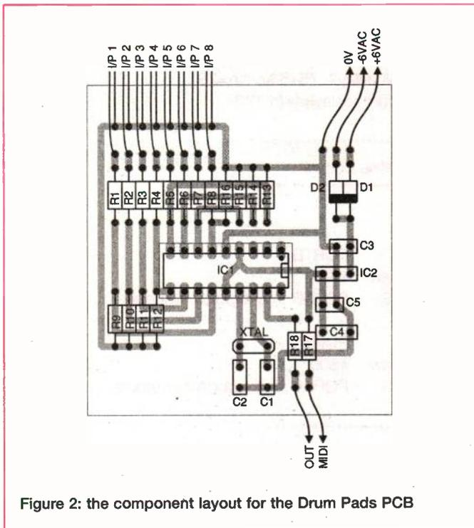
Figure 2: the component layout for the Drum Pads PCB
