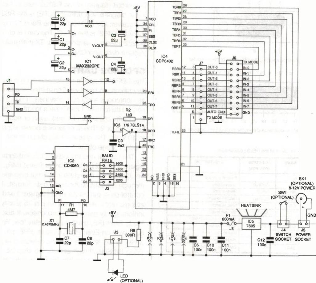
Figure 6: circuit diagram of the TS232 explorer card
