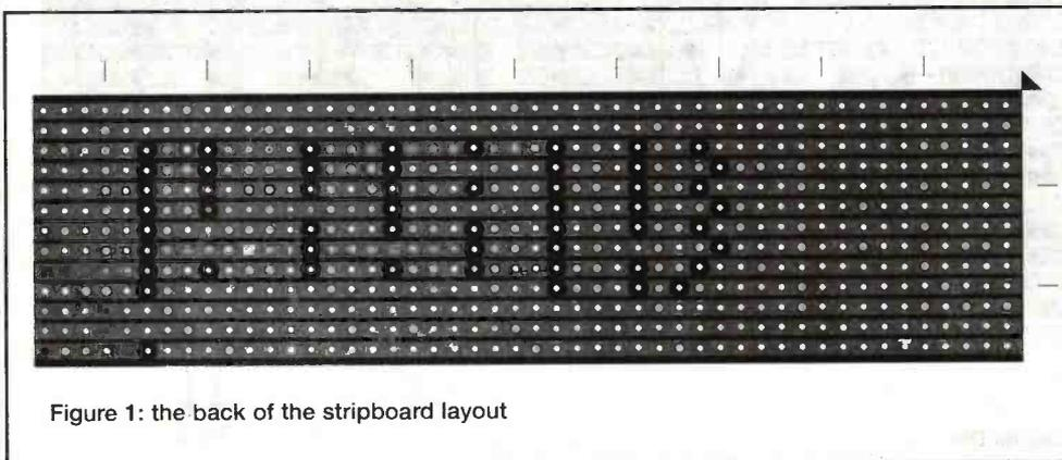
Figure 1: the back of the stripboard layout
