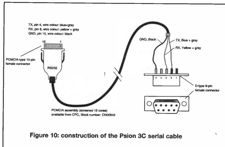
Figure 10: construction of the Psion 3C serial cable
