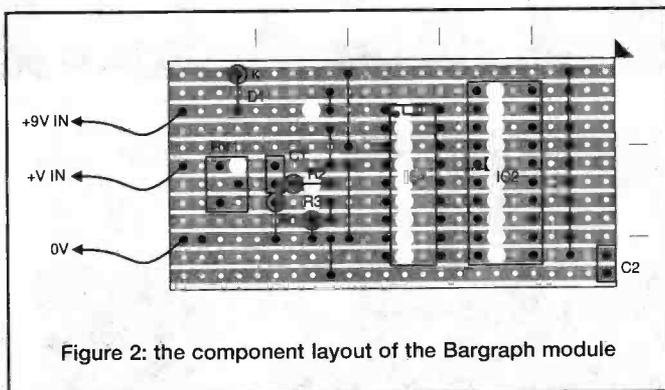
Figure 2: the component layout of the Bargraph module
