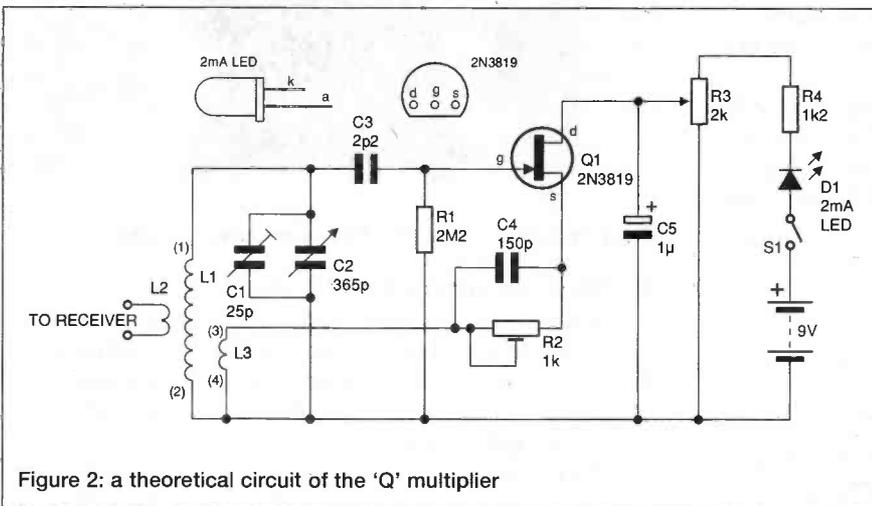
Figure 2: a theoretical circuit of the 'Q' multiplier
