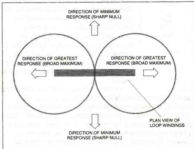
Figure 1: the response pattern of a loop aerial
