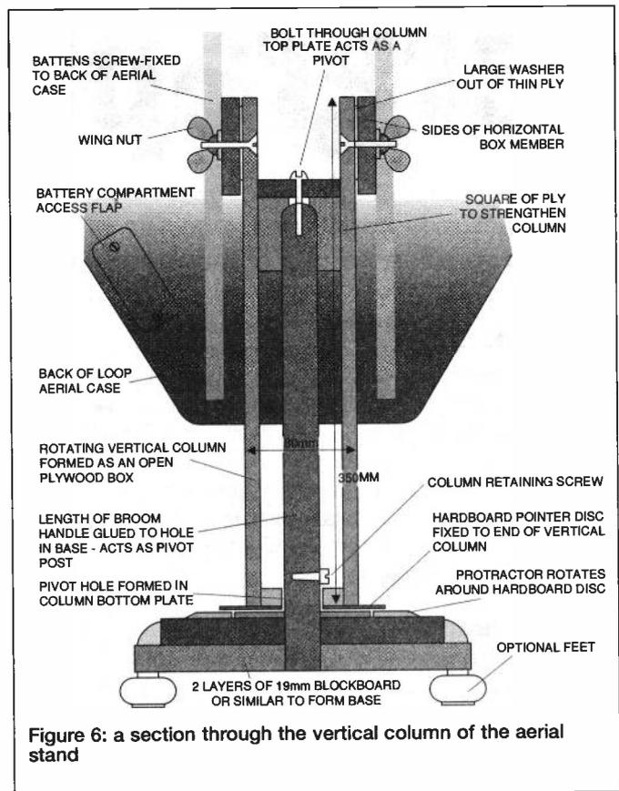
Figure 6: a section through the vertical column of the aerial stand
