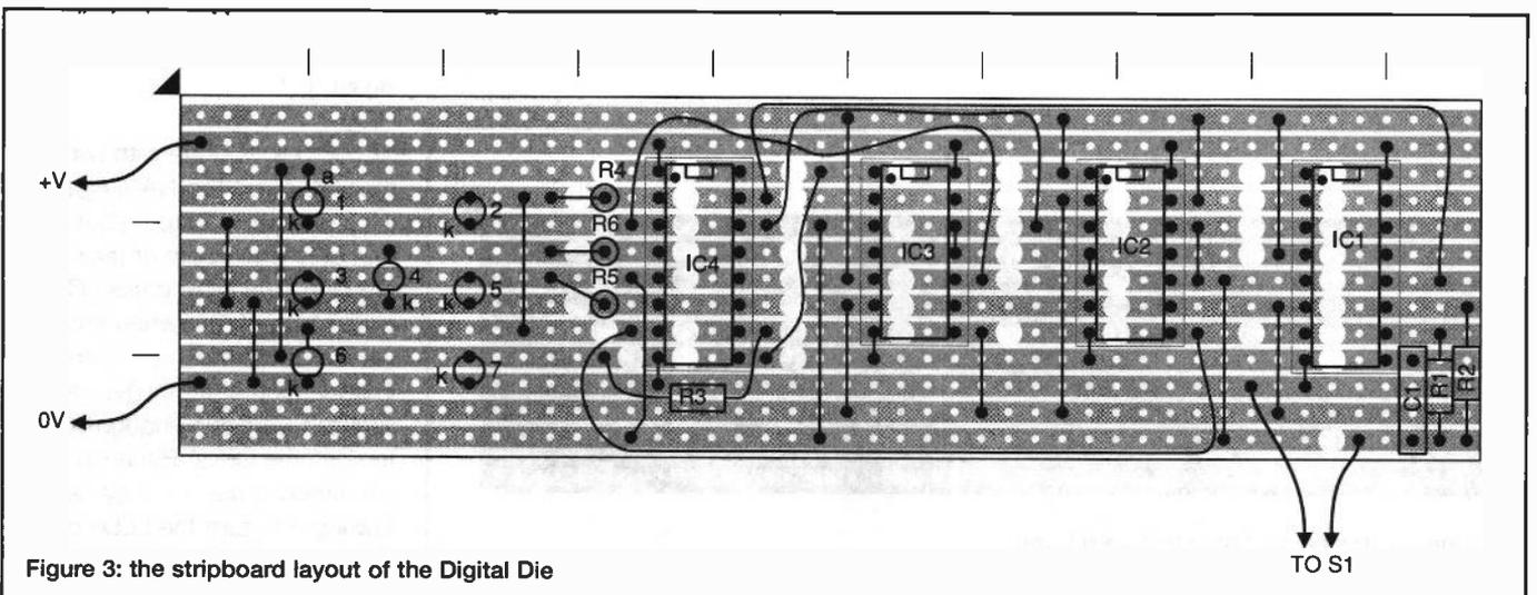
Figure 3: the stripboard layout of the Digital Die
