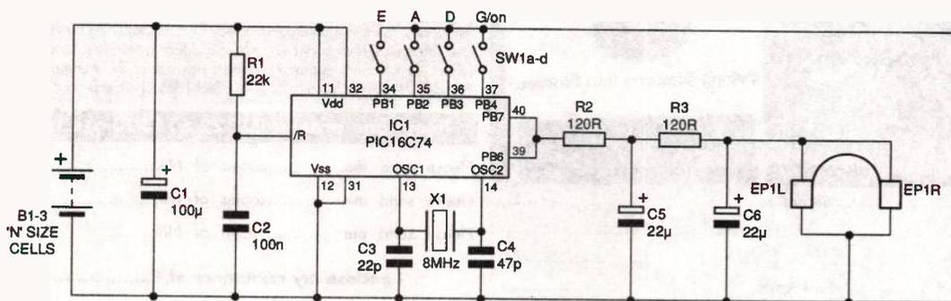
Figure 1: the circuit of the Double-Bass Tuner
