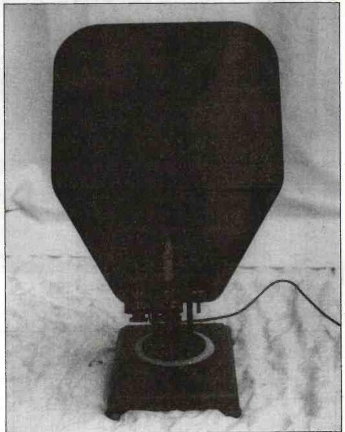
The loop aerial from the front with the case assembled
