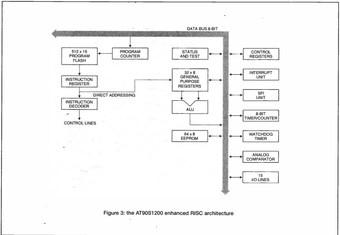
Figure 3: the AT90S1200 enhanced RISC architecture
