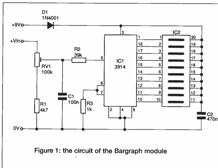
Figure 1: the circuit of the Bargraph module
