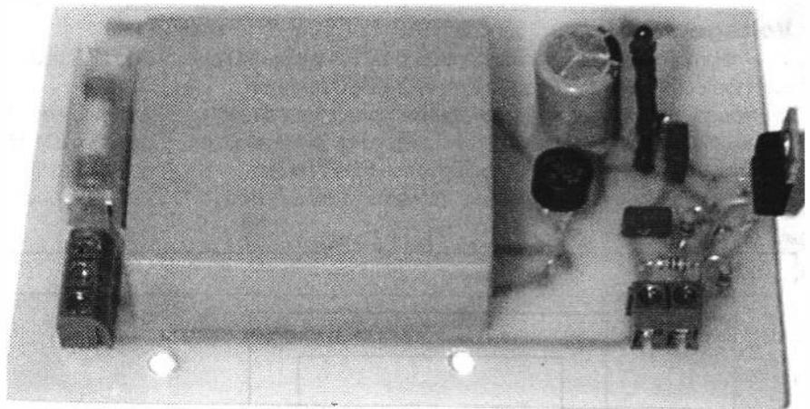
Figure 1: the circuit of the AA Cell Eliminator
