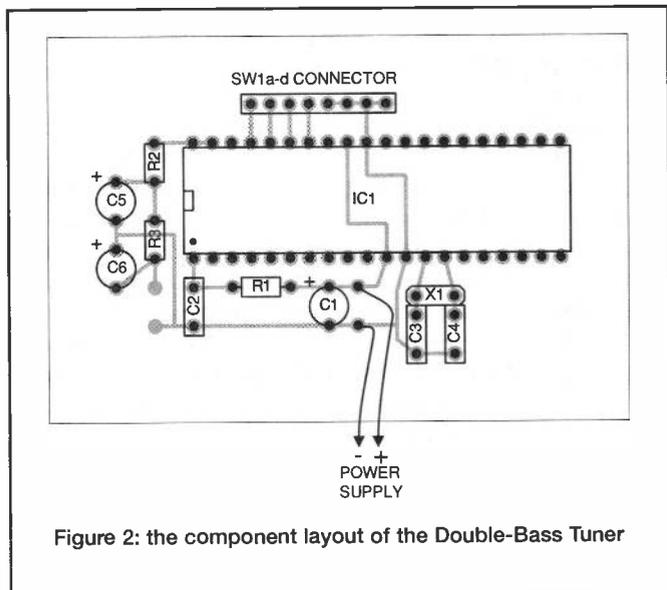
Figure 2: the component layout of the Double-Bass Tuner
