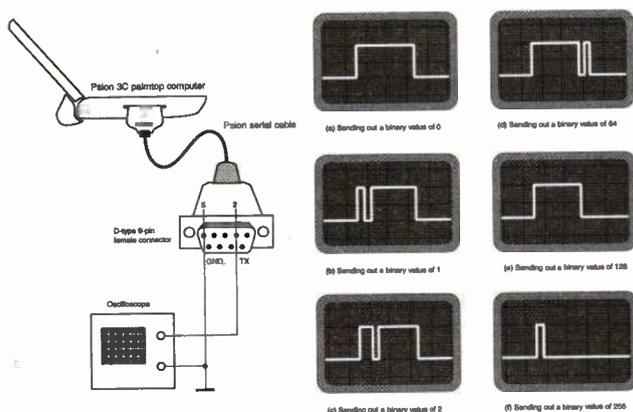
Figure 5: experimental setup and waveforms of TX shown on the oscilloscope when outputting a binary byte from the RS232 port
