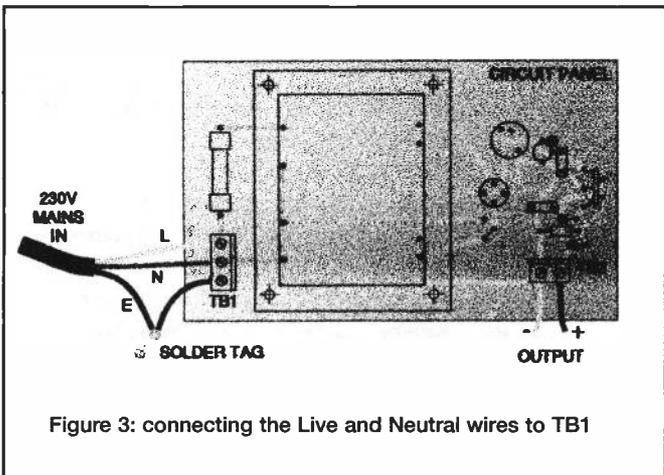
Figure 3: connecting the Live and Neutral wires to TB1
