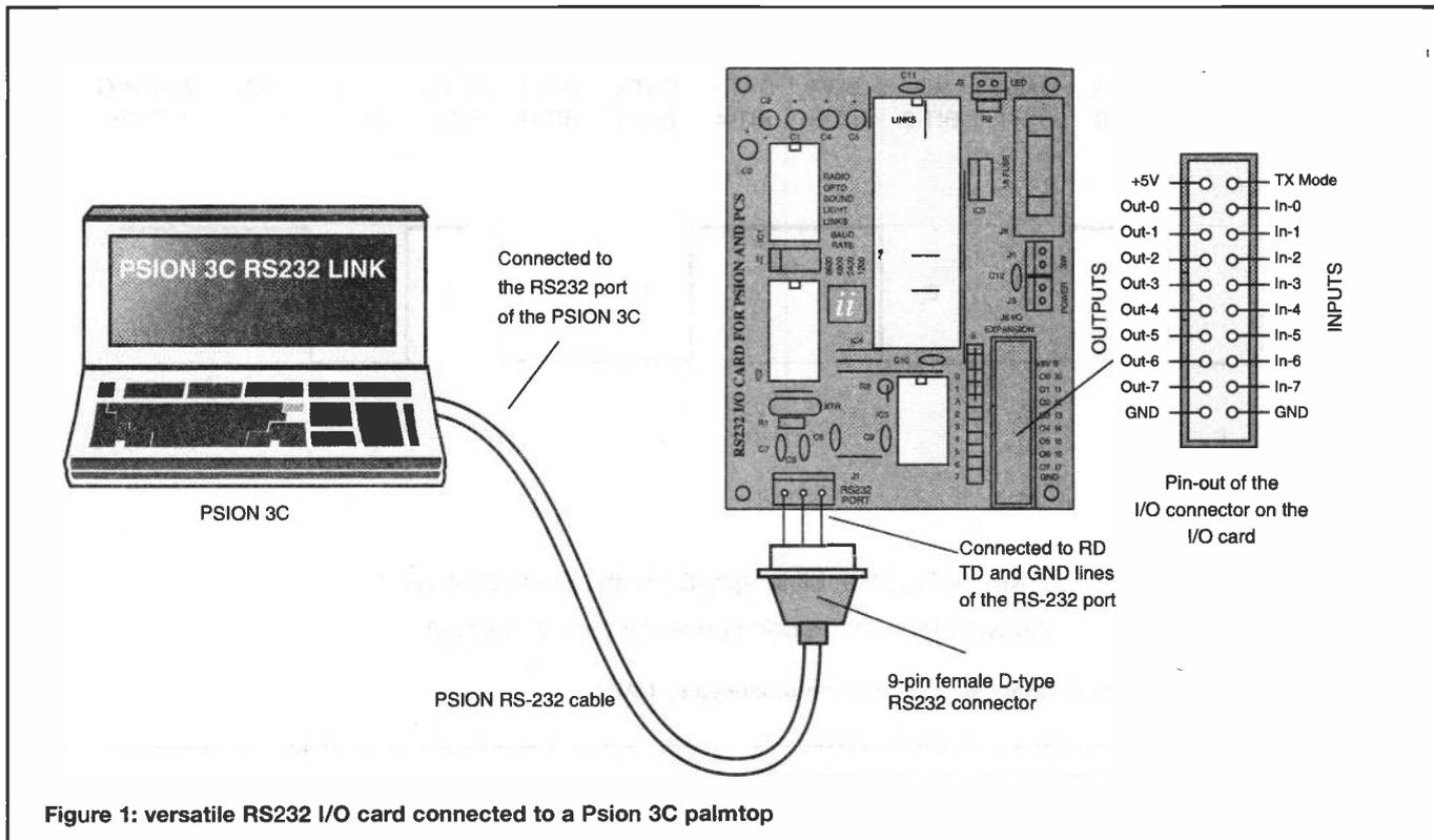
Figure 1: versatile RS232 I/O card connected to a Psion 3C palmtop
