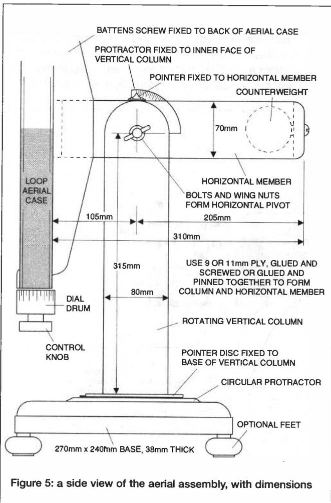
Figure 5: a side view of the aerial assembly, with dimensions
