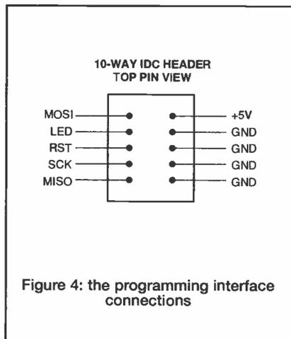
Figure 4: the programming interface connections
