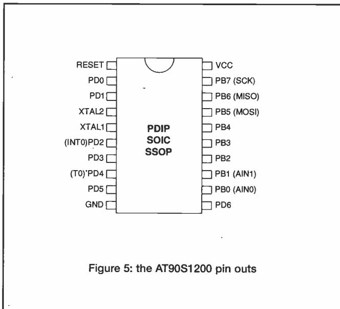
Figure 5: the AT90S1200 pin outs
