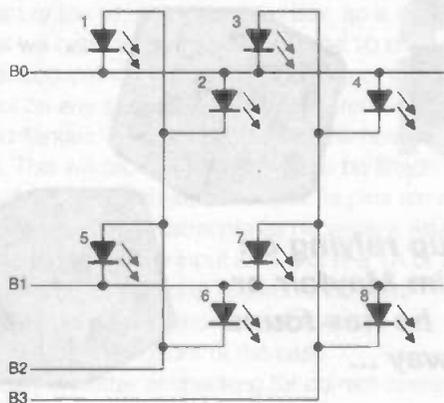
Figure 2: the simplified display circuit
