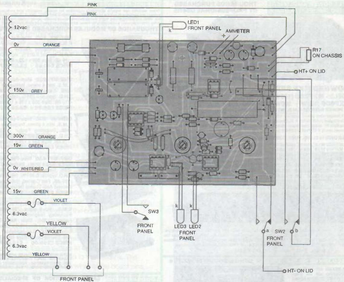
Figure 4: The component layout and the external wiring
