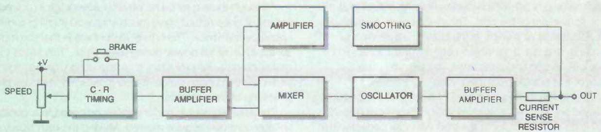
Figure 2: The pulsed train controller block diagram
