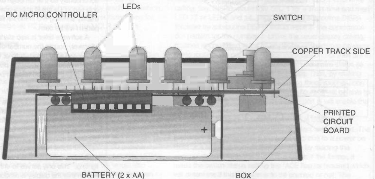
Figure 5: the suggested assembly, showing LEDs and switch mounted on the track side of the PCB
