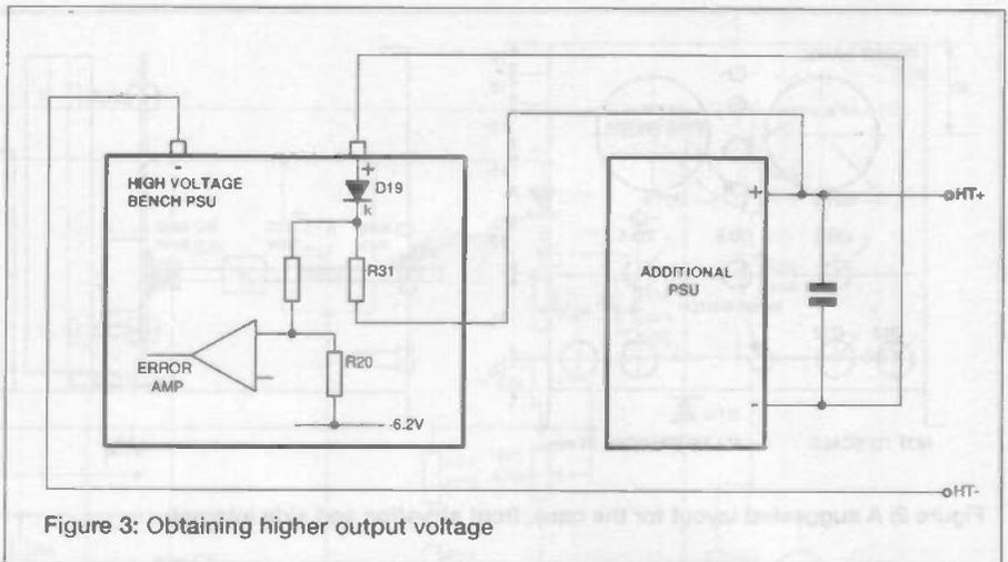
Figure 3: Obtaining higher output voltage
