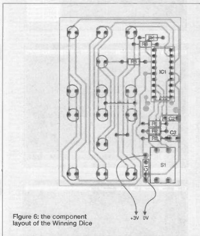
Figure 6: the component layout of the Winning Dice
