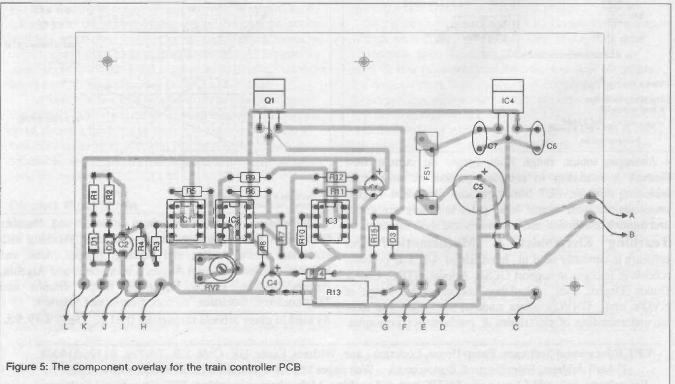
Figure 5: The component overlay for the train controller PCB
