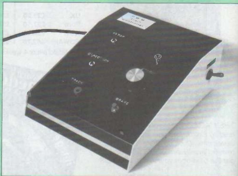
voltage controller, which is basically just a variable voltage stabilised supply. The output voltage is constant in the sense that for a given speed setting it does not change, despite any variations in loading. This method of control provides better speed regulation, because any variation in loading gives a corresponding change in current flow, but without any change in the drive voltage. The motor can therefore draw more or less power, as required.
