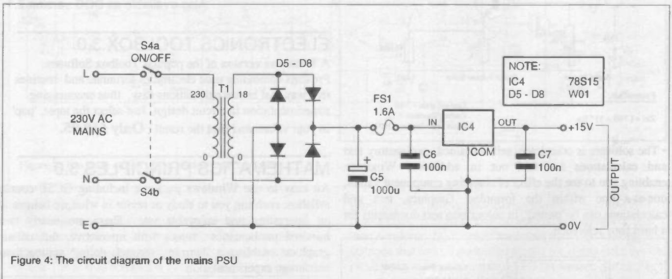
Figure 4: The circuit diagram of the mains PSU
