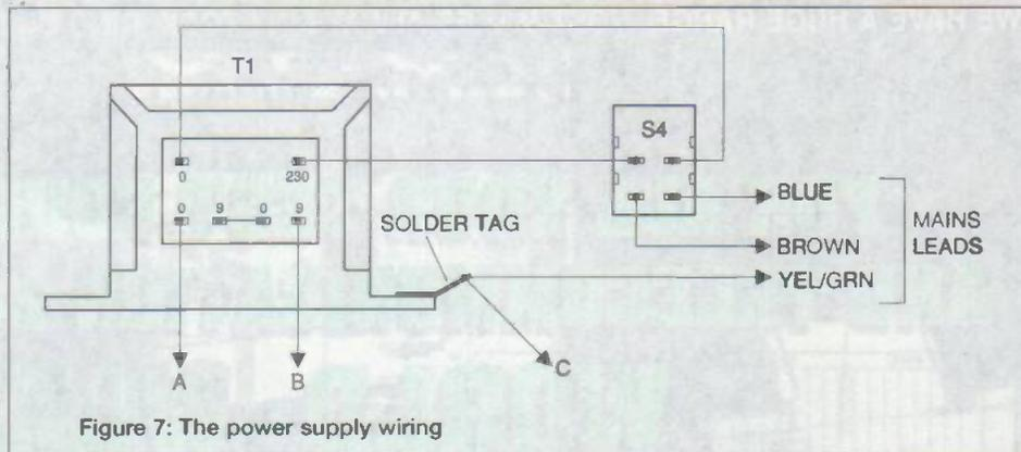
Figure 7: The power supply wiring
