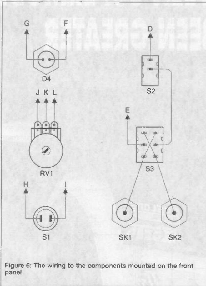
Figure 6: The wiring to the components mounted on the front panel
