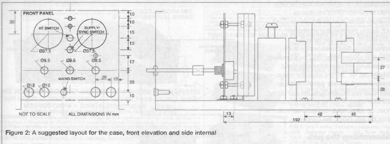
Figure 2: A suggested layout for the case, front elevation and side internal
