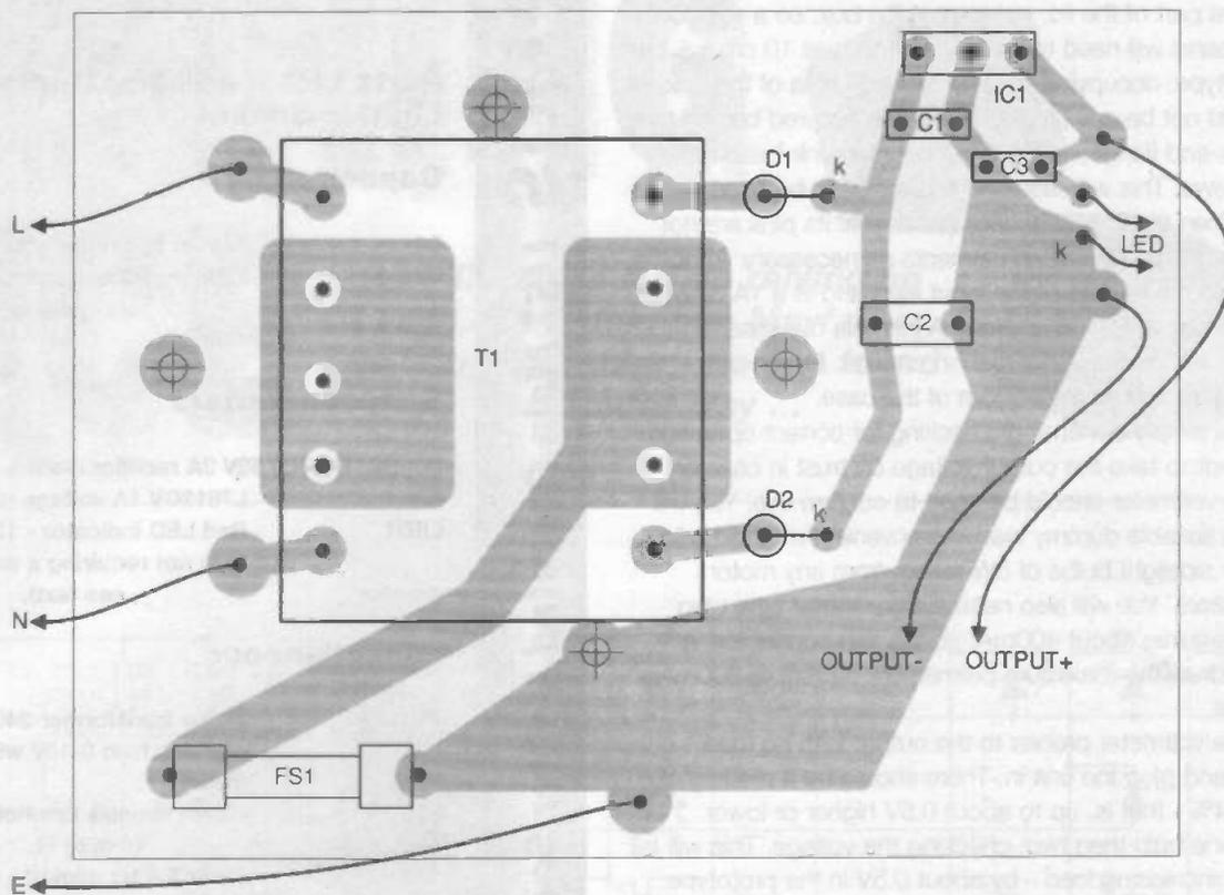
Figure 2: the layout of components on the PCB
