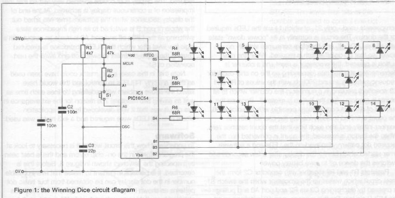
Figure 1: the Winning Dice circuit diagram
