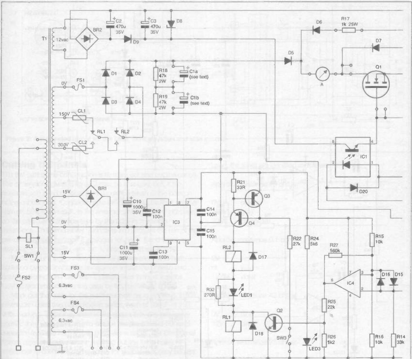
Figure 1: The circuit of the high power bench PSU
