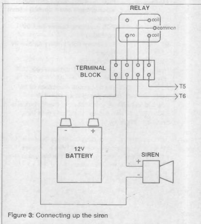
Figure 3: Connecting up the siren
