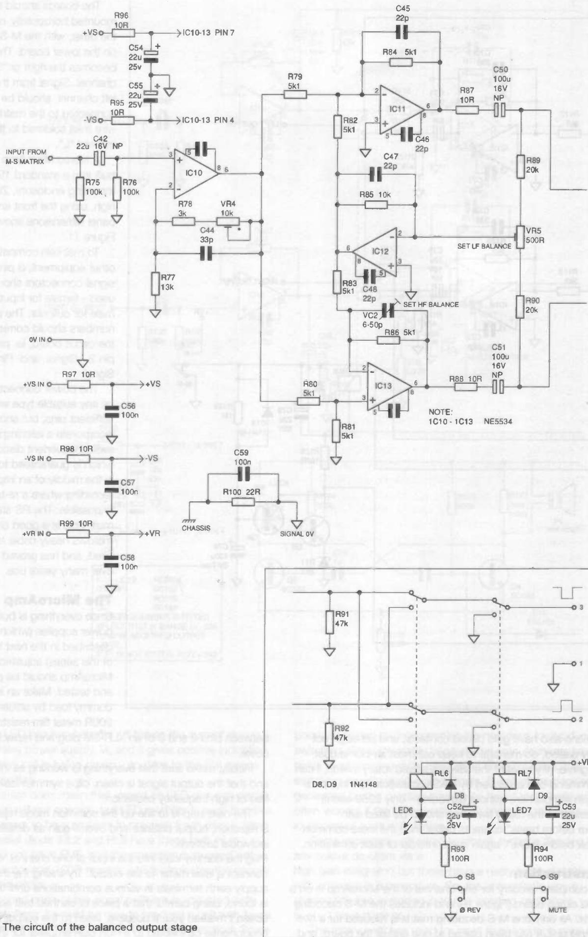
Figure 8: The circuit of the balanced output stage
