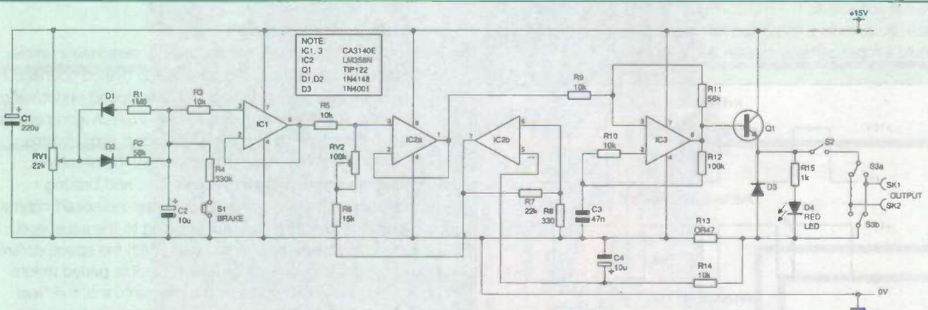
Figure 3: The main circuit of the pulsed train controller
