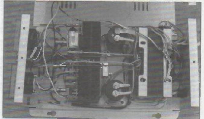
minimises power dissipation in the series pass transistors. A large heat sink is specified for cool running and reliability.
