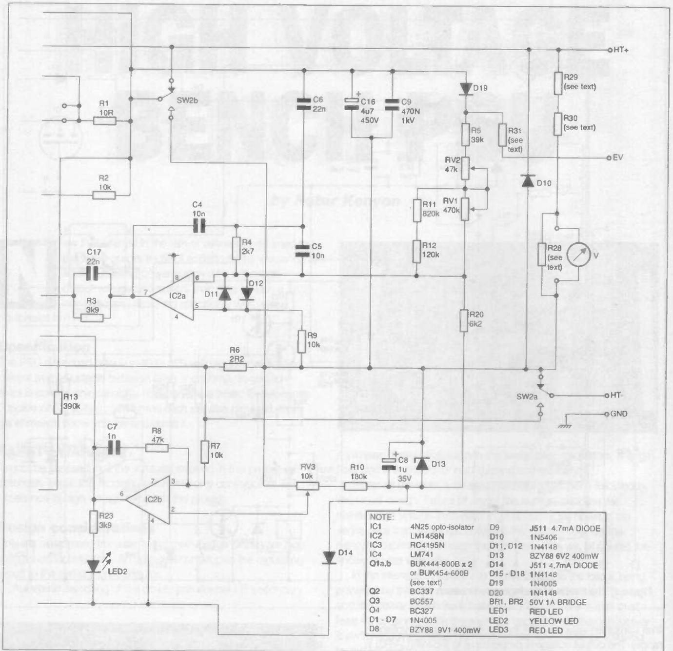
power to the HT bridge while RL1 is controlled by TR2. LED1 indicates that HT is on, LED2 that the regulator has entered the constant current mode and LED3 shows that mains power is being applied to the unit.
