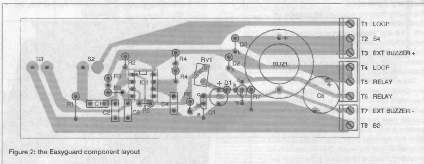
Figure 2: the Easyguard component layout
