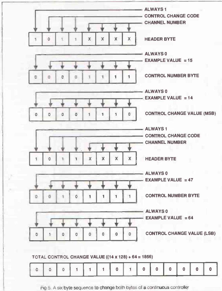
Fig 5. A six byte sequence to change both bytes of a continuous controller
