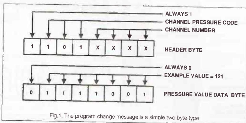
Fig.1. The program change message is a simple two byte type
