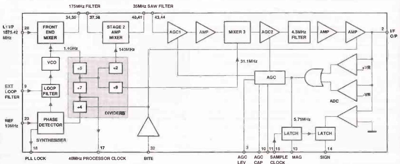
Block diagram of a GP1010 GPS chip
