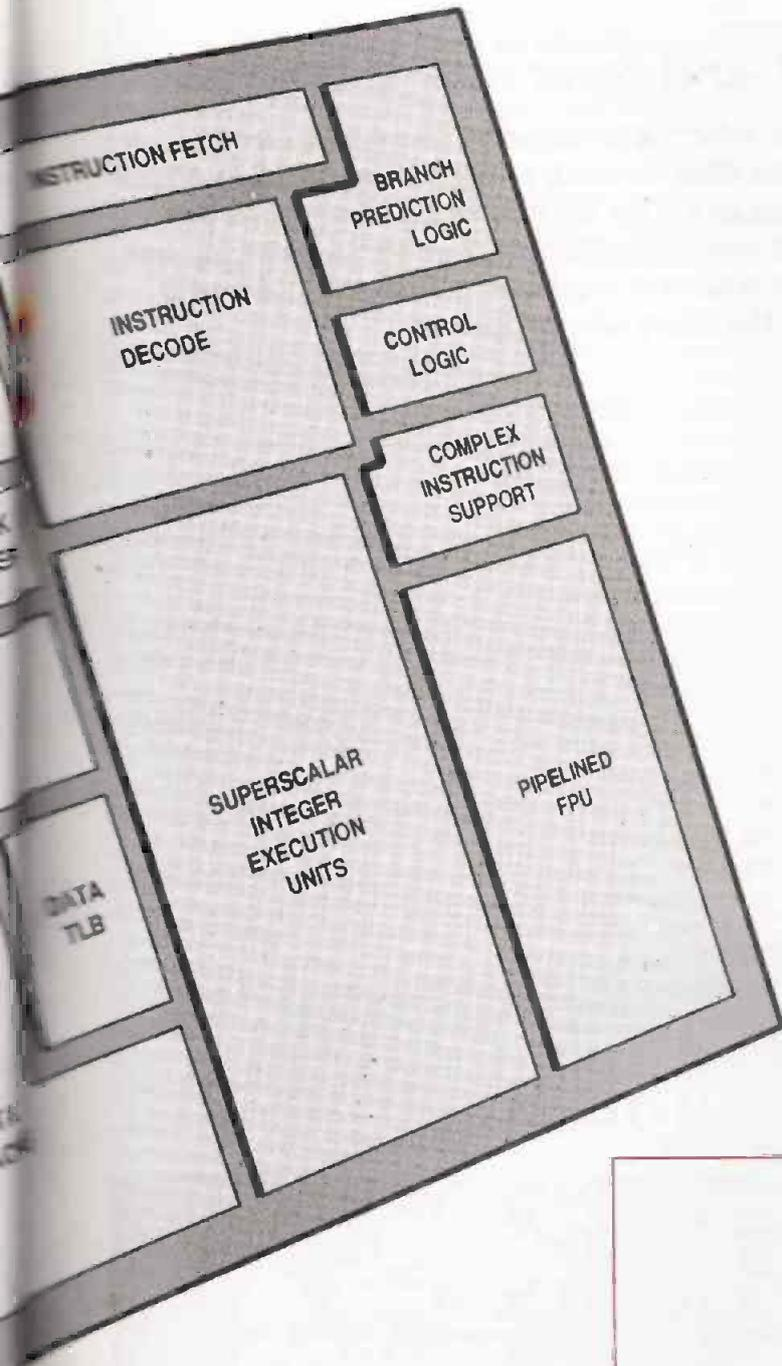
predictions. If the BTB prediction is wrong, then the pipeline is flushed and the correct instruction fetched, thereby causing a 3 clock cycle delay.
