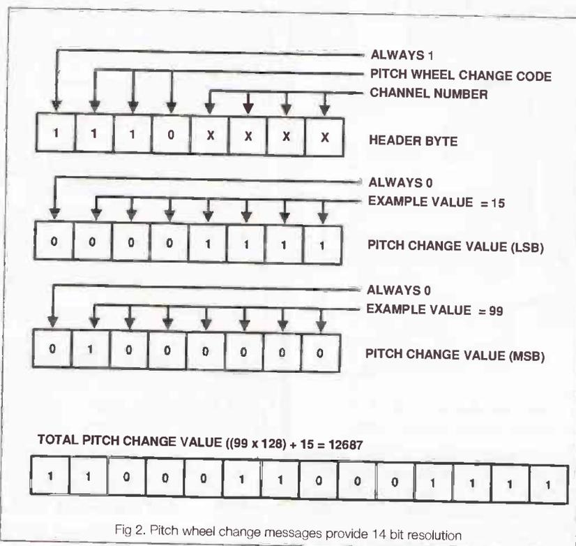
Fig 2. Pitch wheel change messages provide 14 bit resolution
