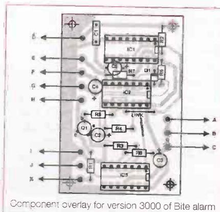
Component overlay for version 3000 of Bite alarm
