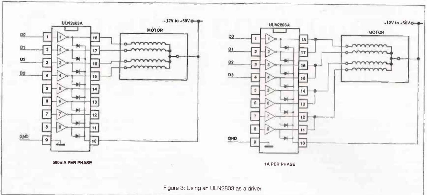
Figure 3: Using an ULN2803 as a driver
