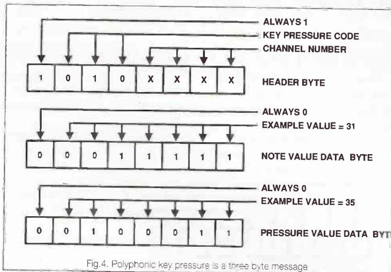
Fig.4. Polyphonic key pressure is a three byte message
