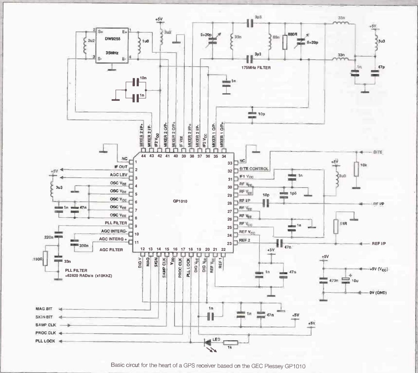
Basic circuit for the heart of a GPS receiver based on the GEC Plessey GP1010
