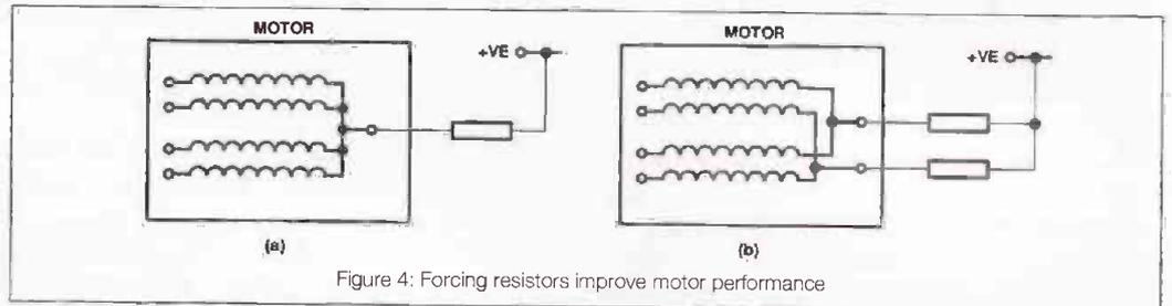
Figure 4: Forcing resistors improve motor performance
