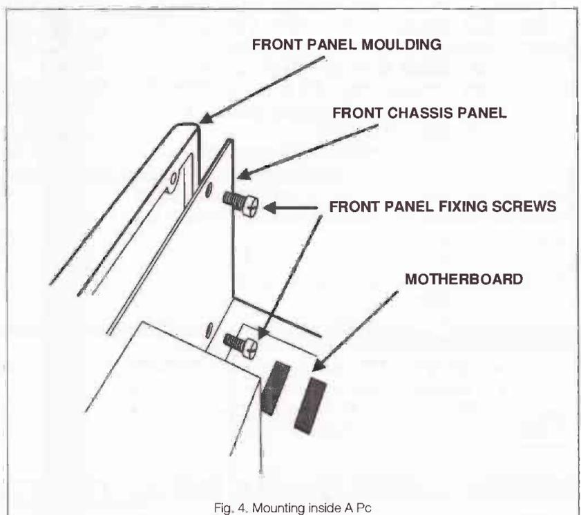
Fig. 4. Mounting inside a PC
