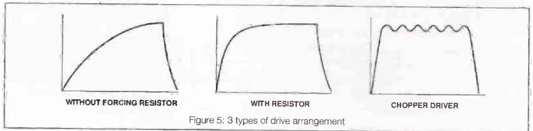
Figure 5: 3 types of drive arrangement
