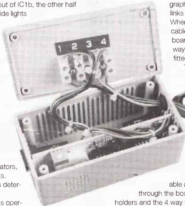
The terminal block was mounted to the lid on the inside, using two 6BA nuts and bolts and the fuse holders at either end of the box. These were done last to ensure that neither fouled the PCB. Insert the PCB as near to one side of the box as possible and mark the position of the piezo sounder, so you can drill a suitable amount of holes to allow the sound
