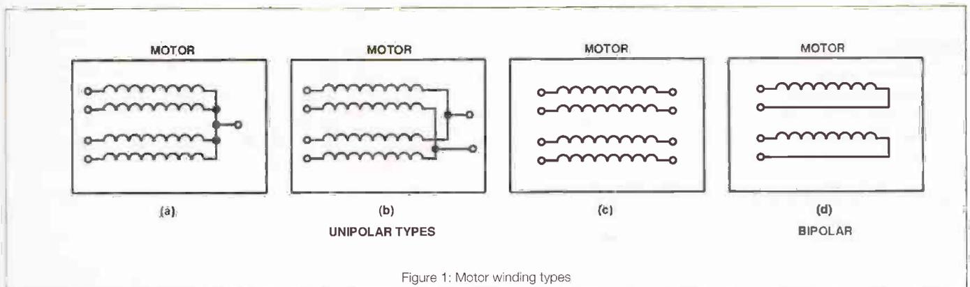
Figure 1: Motor winding types
