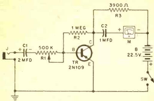
R3 provides the recommended source impedance for proper damping of the VU meter.
