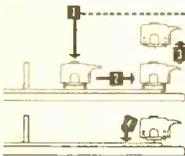
1. When START button is pressed, tone arm moves toward center. 2. With wheels down, arm glides lightly over top unused surface until outer wheel locates exact outer edge. 3. Arm rises and wheels retract. 4. Arm gently descends to play.
