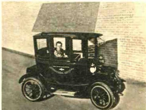
The wind can power this auto if the sun doesn't. The sail-like panel mounted atop this 1912 Baker electric is composed of 10,000 silicon solar cells which catch the sunlight and through the conversion system, power the auto. Although charging the 72-volt battery may take over 10 hours, the car's 3 hp motor is capable of running at a speed of 20 mph for almost 50 miles. Needless to say, improvements will be made. The conversion system was designed by Dr.
