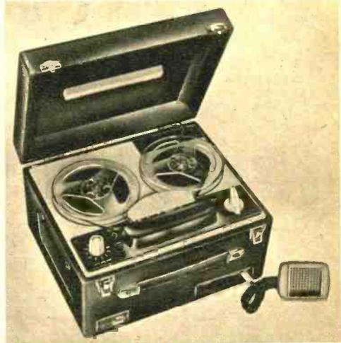
The RE-400, a new dual speed tape recorder has been announced by Lafayette. A single knob controls all operations (stop, play, etc.) and an indicator light shows optimum volume control setting. Outputs for another speaker, recording from microphone or phonograph are provided. Playing speeds are 7½ and 3¾ ips. Priced at \$54.50 complete with crystal microphone from Lafayette, 165-08 Liberty Avenue, Jamaica 33, New York.
