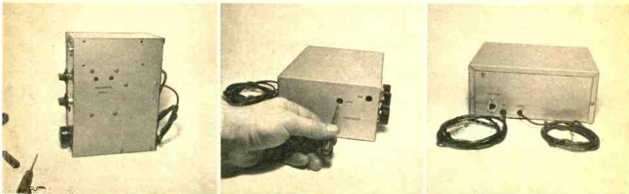
Bottom, side and rear views of completed unit shows position of holes to be drilled. Rear of unit contains auto antenna plug, and input and output cables.
