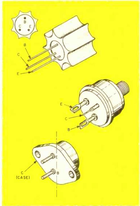
Fig. 3. Additional power transistor housings and types which are likely to be encountered in home or industrial equipment. These are the generally larger power types for heavy use.
