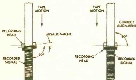
This sounds like a matter of azimuth adjustment. If the angle of the head (or heads) in each machine is not the same, high-frequency loss will be the result when tapes are swapped. I'd say your machine was alright in this respect since the pre-recorded tapes sound good. Play one of these on the other machine. If it sounds dull, the azimuth (head angle) must be adjusted on your neighbor's machine. *Don't* make this adjustment yourself; special equipment is needed.
