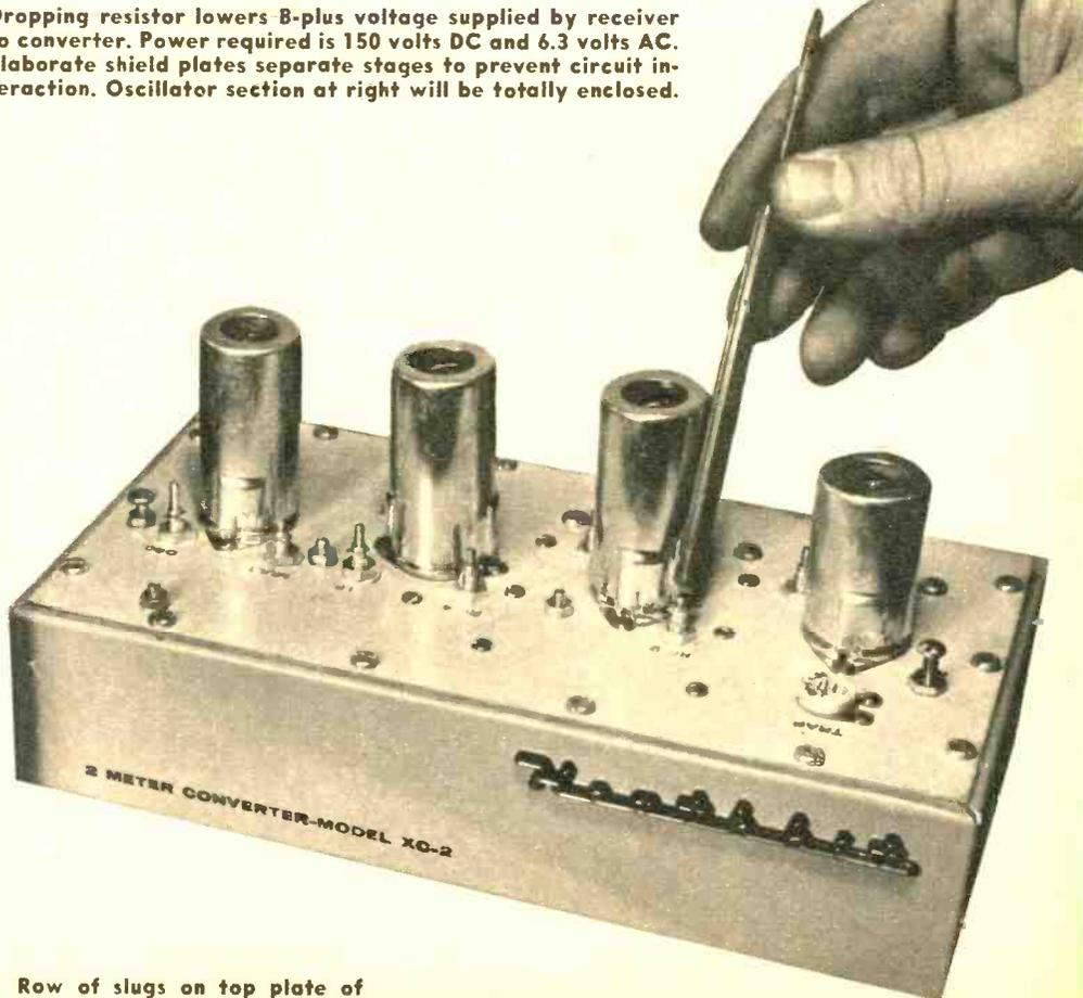
Row of slugs on top plate of converter are for alignment.
