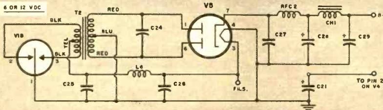
Schematic for DC operation. Vibrator and transformer T2 differ for 6 or 12 volt use.
