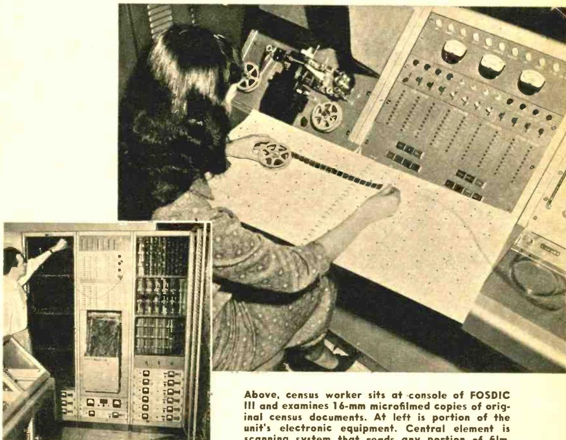
Above, census worker sits at console of FOSDIC III and examines 16-mm microfilmed copies of original census documents. At left is portion of the unit's electronic equipment. Central element is scanning system that reads any portion of film.
