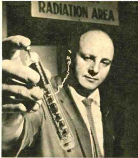
The radiation detector, battery and amplifier all are enclosed in this single small package that has been fabbed an "Alpha cigar" by Hughes.
