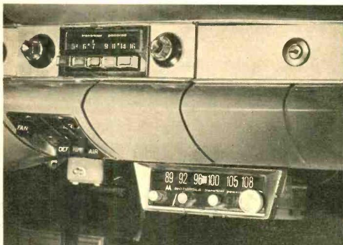
under-the-dash-installation unit can operate independently of the car's AM set. Three transistors power the hybrid circuit, which contains seven additional tubes. FM-900 shares the AM set's antenna and can be used with any 12-volt, negatively grounded ignition system. No need to sell the FM set when you sell your car. It may be moved from auto to auto, or auto to boat. Other features are AGC, AFC and \$125 price.
