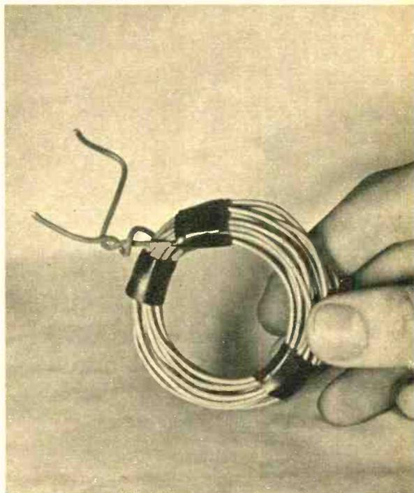
A miniature AM tuning meter provides accurate reading of wattage when properly calibrated. An inked-in scratch marks its "null" point. Simple coil serves as high-current, low-resistance input shunt resistor.
