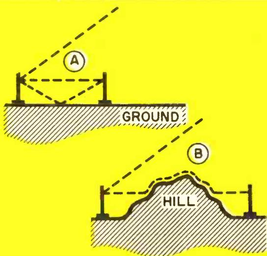
A) Six meter communication occurs via direct space wave and reflected ground wave. Latter is out of phase and reduces signal strength, thus antenna with maximum radiation parallel to ground is best. High angle radiation probably will not be returned to earth. B) Diffraction can bend VHF frequencies around curvature of earth only for short distances.
