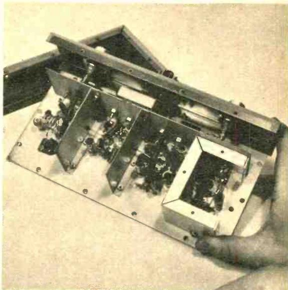
Dropping resistor lowers B-plus voltage supplied by receiver to converter. Power required is 150 volts DC and 6.3 volts AC. Elaborate shield plates separate stages to prevent circuit interaction. Oscillator section at right will be totally enclosed.
