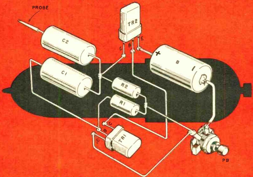
All the miniature components must be wired as shown above with all leads short. This requires the use of a low wattage soldering iron and heat sinks.
