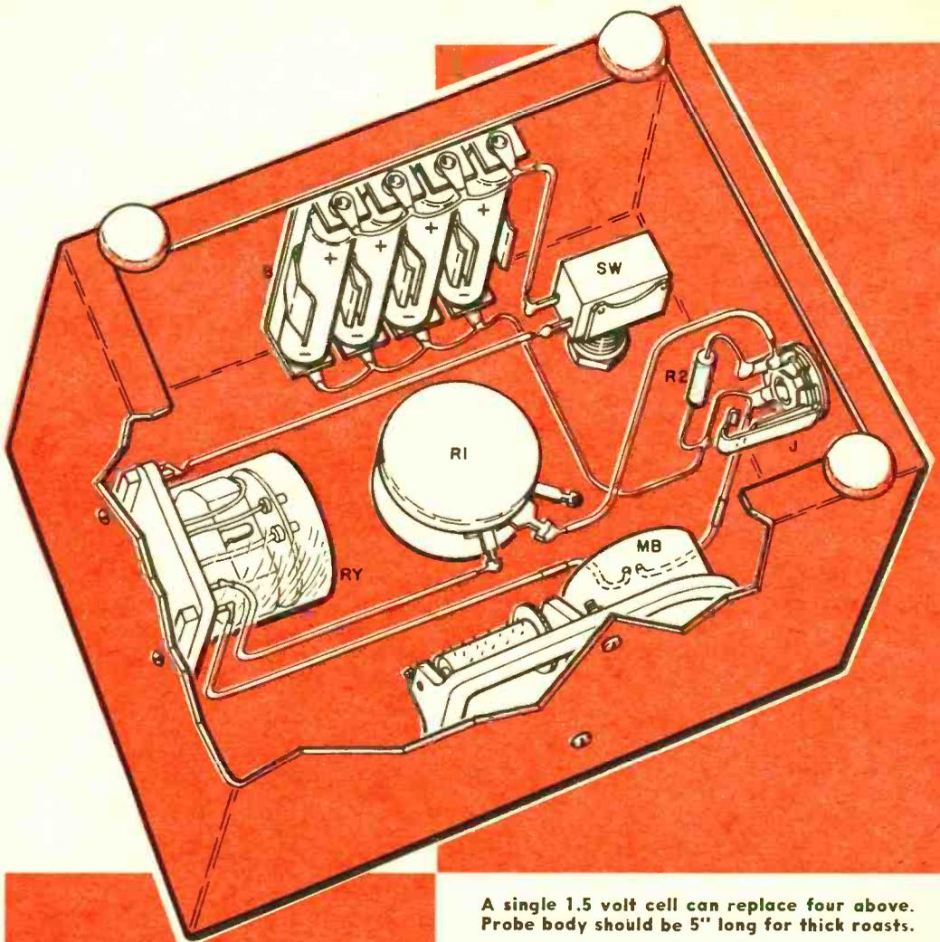
A single 1.5 volt cell can replace four above. Probe body should be 5" long for thick roasts.
