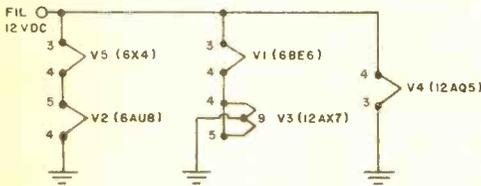
Filament wiring for 12 volt supply, see text.
