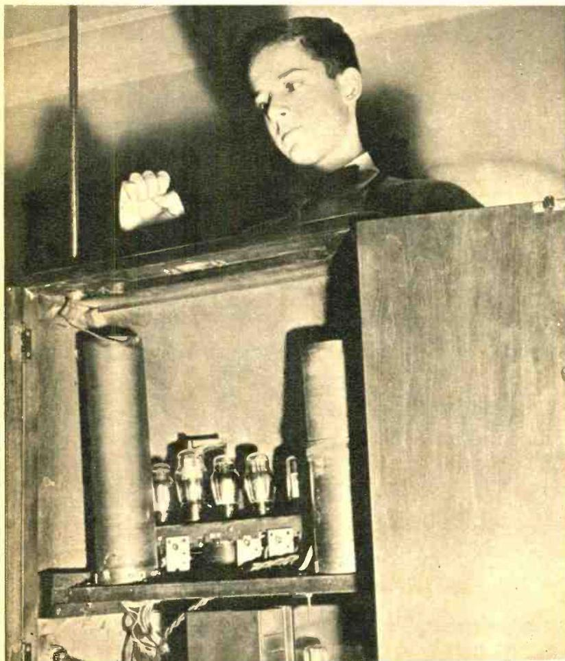
Six tubes, plus power supply (not shown), comprise the original RCA model. Note the variable pitch oscillator coil and pitch antenna (vertical), at left side of cabinet.
