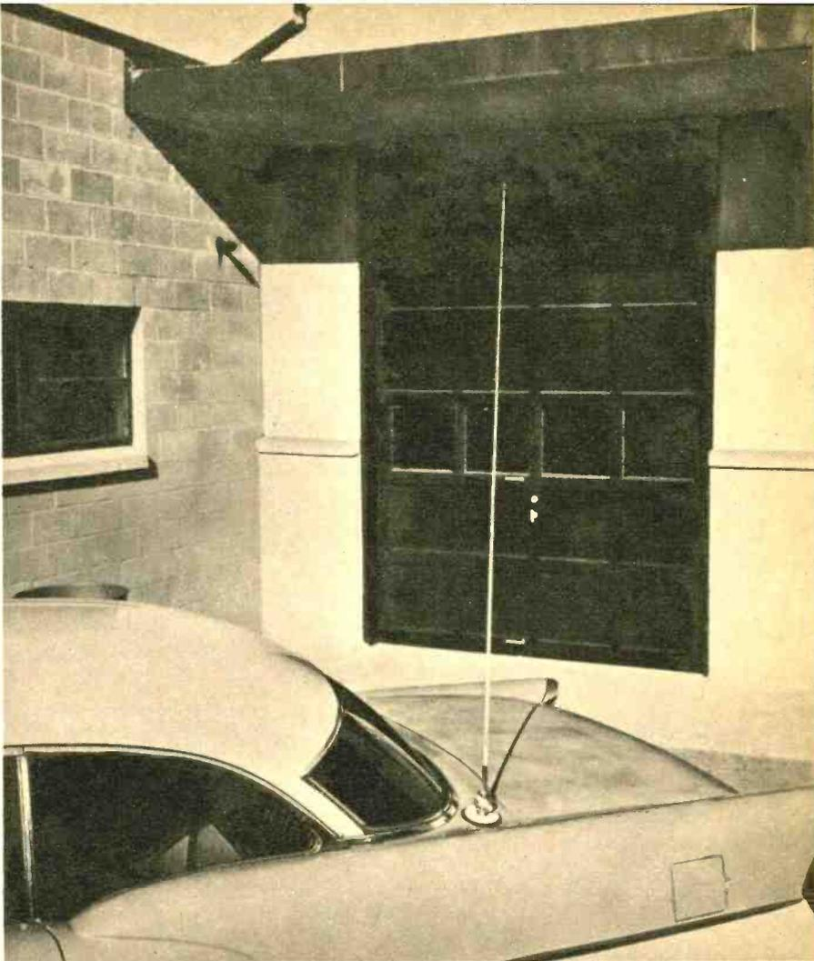
The non-directional, vertically polarized whip antenna is popular for mobile ham operations on six meters. Length of a six meter whip is about 54 inches. This Shakespeare Wonderod (model 10-1) is attached to car by a simple ball mount.
