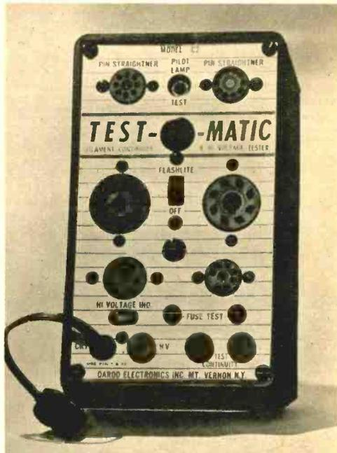
This new compact battery-operated tube tester is quite versatile. Only 3 3/4" x 6", the unit will test most tube types and circuits for continuity. In addition it will check out high voltage circuits, fuses and pilot lamps. Priced at \$6.95 from Empire Merchandising Co., 170 Marbledale Road, Tuckahoe, New York. The tester is manufactured by Darod Electronics, Inc., Mt. Vernon, N. Y.
