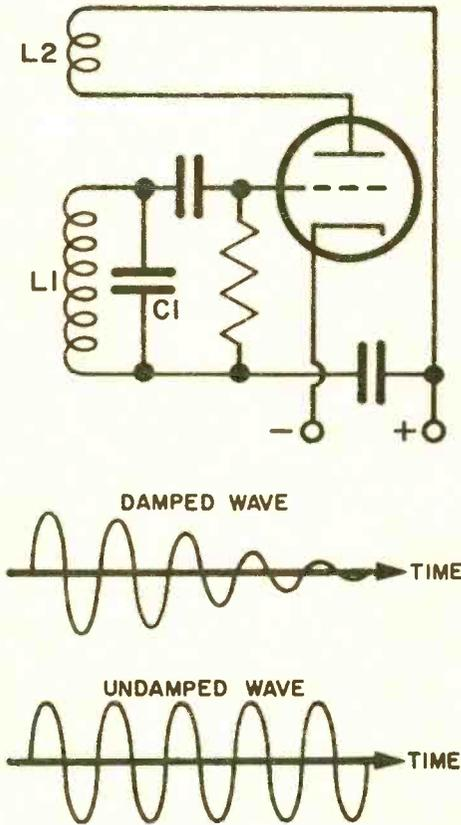
The basis of any oscillator of this type is the resonant circuit formed by L1 and C1. The oscillator you have drawn is the Armstrong series-feed type.
