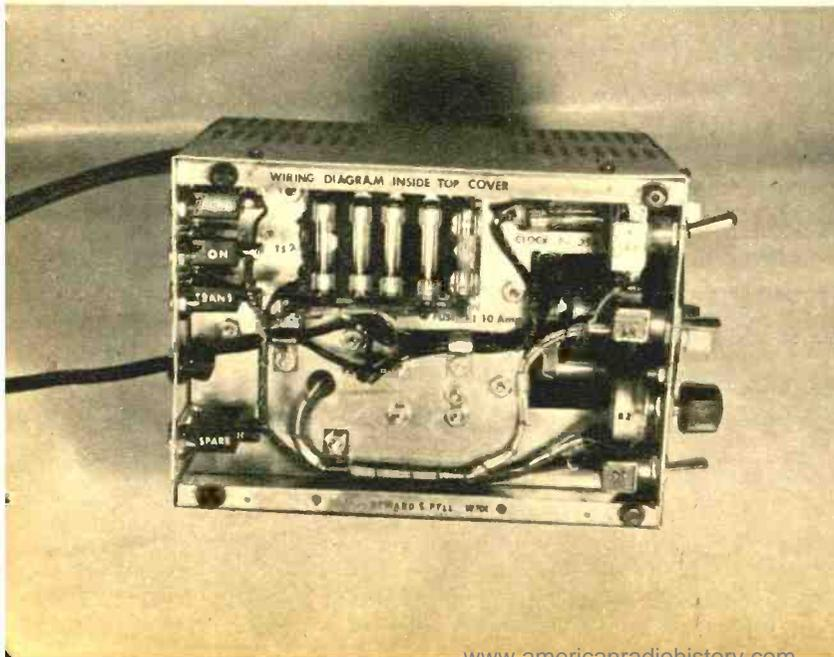
Underside view of chassis. Wires have been laced for permanence and neatness. Each circuit has an individual fuse held in its place by a clip-holder. Cutout for clock mechanism on chassis is seen in photo.
