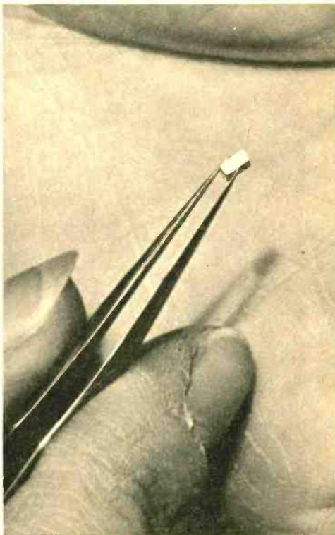
General Electric research scientists have successfully made tunnel diodes which work at frequencies above 4000 megacycles. Key to the improved performance is the use of gallium arsenide, a little known and rarely used semiconductor material, as the basic element in the device's construction. Frequencies well above 10,000 megacycles are possible with tunnel diodes made of gallium arsenide.
