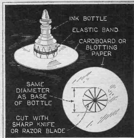
The above illustration shows a useful article for the draughtsman. This is an India ink bottle holder made from a blotter or a piece of cardboard, cut as shown, and fastened to the bottle with a rubber band. It is easily made and a new one can be put on in a few seconds. Blots of ink on the drawing are also eliminated.—L. Keiser, Jr.
