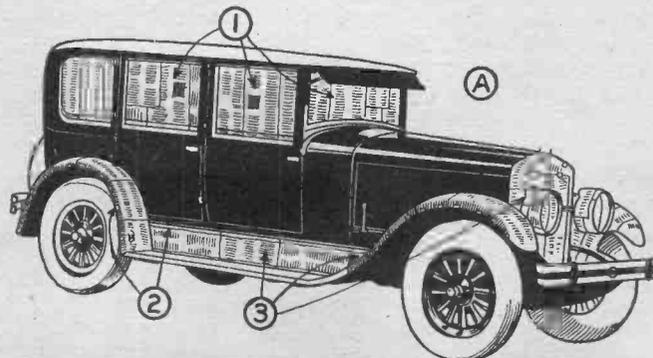
In the above illustration, 1 shows paper placed over all glass; 2, gummed tape holding paper in place; 3, mudguards and fenders protected from paint in the same manner. When painting the car, the use of paper as shown will keep the adjacent surfaces clean.
