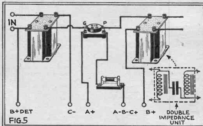
The above illustration shows a typical double-impedance coupled audio stage. An inductance is used in both the grid and the plate circuit, with the blocking condenser connected between them as shown.
