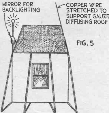
A rear view showing the bracing, gauze roof and mirror for back lighting.
