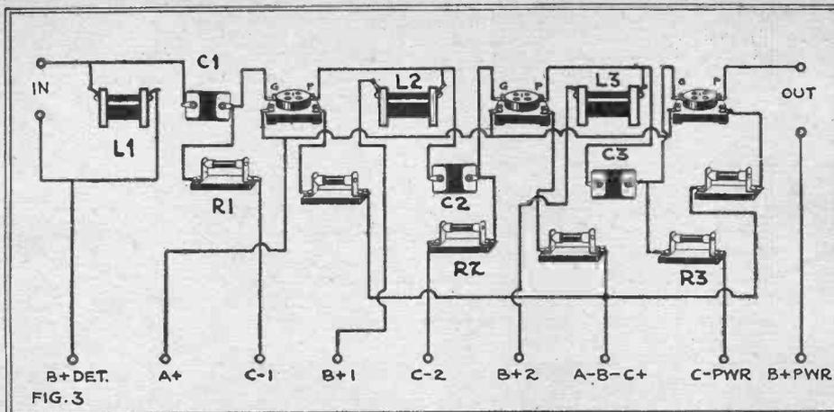
A single impedance coupled, or as it is generally called, simply an impedance coupled audio amplifier is shown in the above picture diagram. This is similar to the resistance coupled amplifier, except that the plate resistors have been replaced with iron core inductances.
