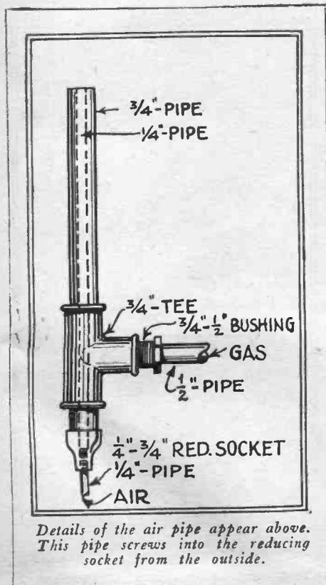
Details of the air pipe appear above. This pipe screws into the reducing socket from the outside.
