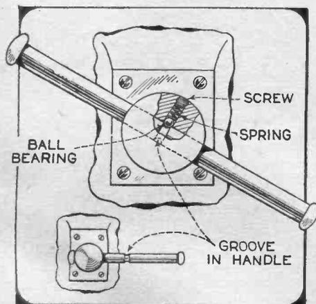
By fixing the handle of a vise in the manner shown, it may be turned more quickly by virtue of the ball bearing held in place with a spring. A screw supplies the necessary pressure.—J. N. Sell.
