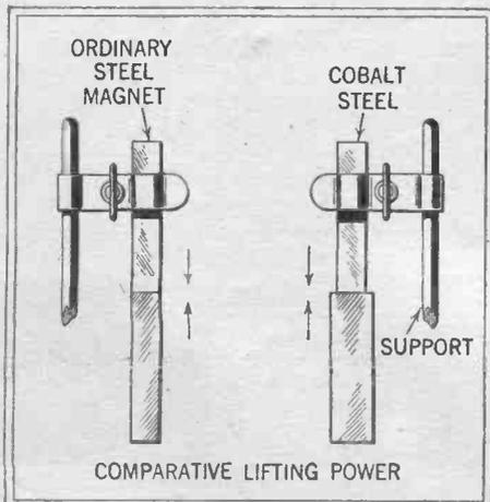
The comparative lifting power of an ordinary steel magnet, shown at the left, and a cobalt steel magnet, at the right, is well illustrated in the above drawing.
