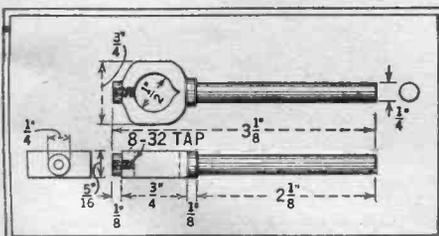
A lathe dog can be made as shown above from 3/4 in. diameter cold rolled steel. It is placed in the lathe and turned as shown. A hole is drilled and elongated to form a 3 point bearing. A tap hole is drilled on centers with No. 29 drill. Tap 8-32 and insert set screw.—C. Russell.
