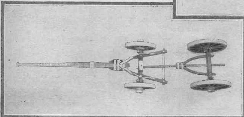
The photograph above and the one at the right shows the construction of the carriage. The builder has faithfully reproduced the metal banding at all those points where wear is likely to occur and those which require reinforcement in the full size construction. The entire top of the model can be removed so that one can easily examine the carriage.
