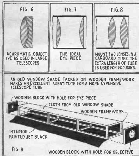
Illustrated above is the ideal eyepiece. Constructor can make a good one with two lenses. A substitute for a telescope tube is also shown.
