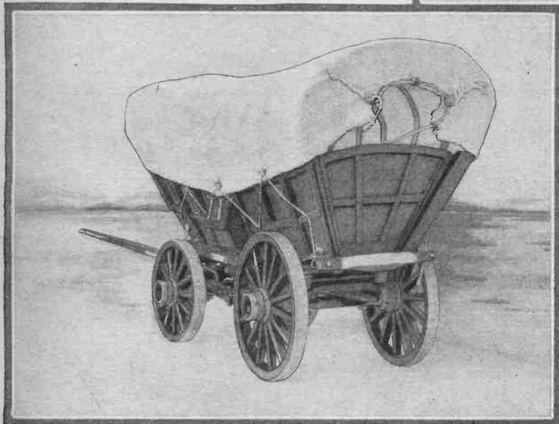
Here we have a three-quarter rear view of the prairie schooner which will give one a fair idea of the construction of the under carriage from this point. Note metal-tired wheels. The back of this wagon is removable.
