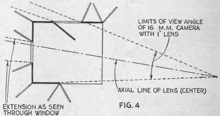
"Camera angle" of set showing how the braces must be placed, so that they cannot be seen through doors and windows.
