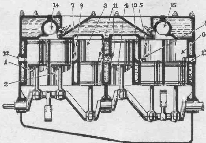
The above illustration shows the internal combustion engine which has no valves.—Courtesy Wissen Und Fortschritt.
