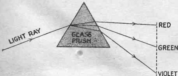
Fig. 2. A diagram of a spectroscope, showing how the entering light ray is broken up by the glass prism into the spectrum of rainbow colors appears at the left. It will be noted that the violet ray is bent much more than the red ray.
