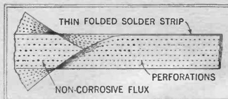
The tape solder is formed by a thin folded solder strip in the center of which is a non-corrosive flux. Perforations allow even distribution of flux.
