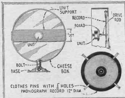
An inexpensive speaker can be built from a cheese box as shown. Four clothes pins are slotted in order to receive a phonograph record which is clamped to the back of the box. The speaker unit is supported by a board which fits inside the box. The drive rod is fastened to the center of the phonograph record.—Wm. Tevendale.
