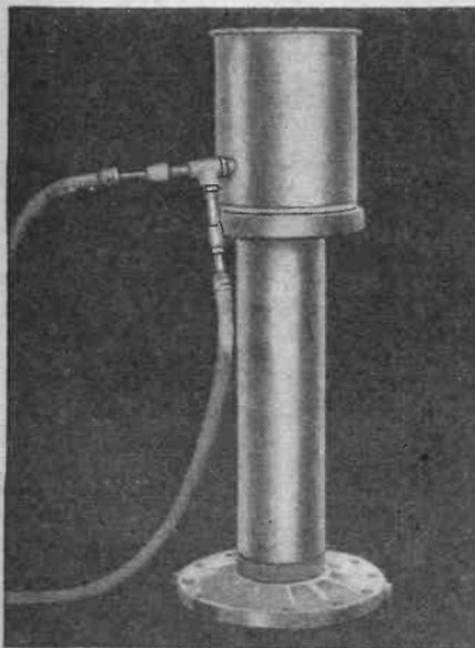
The above photograph shows the furnace ready for work. The stand is made from a section of 8-inch pipe with a flange at each end.
