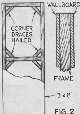
Above is a sectional view of a "flat" showing the bracing and interior construction.
