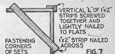
This illustration shows how the battens are placed on the top and bottom to stiffen the sides. Strips may be tacked along the seams on the outside to prevent warping.
