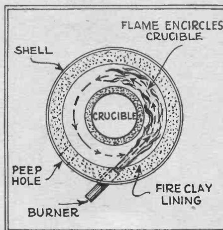
Above is a sectional view of the furnace. The construction is made clear in this illustration.
