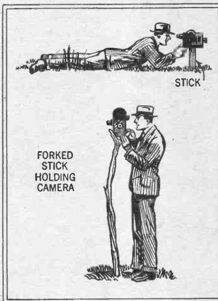
Two ways in which to support camera when no tripod is handy.
