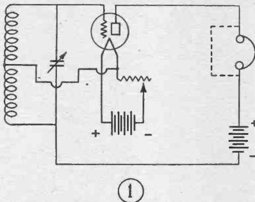
A diagram of an oscillating wavemeter using the Hartley principle is shown above in Fig. 1.
