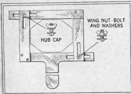
Various makes of automobiles have different sized hub caps and a wrench devised to fit most of these is illustrated above. Flat cold rolled steel 3/16 in. x 3/4 in. is used throughout with 5/16 S.A.E. cap screws and wing nuts for the clamp bolts. The two solid corners can be bolted or welded together. This wrench will not harm the hub cap.
