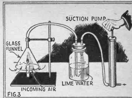
The above illustration shows how to demonstrate that carbon dioxide is formed when a candle burns in air.
