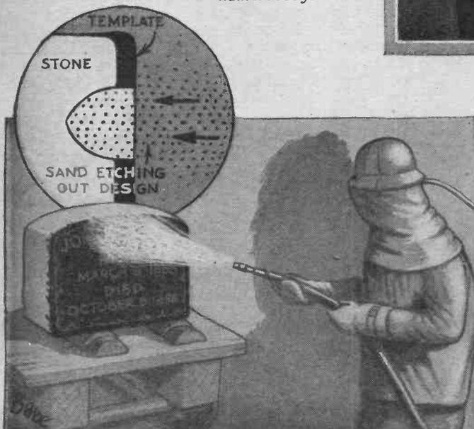
The above illustration shows a workman carving with the sand blast. A composition template or stencil is used as shown and the sand etches out the design or lettering. Needless to say, carving by this method is a much quicker process than when using the mallet and chisel.
