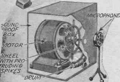
A MOTOR DRIVEN WHEEL WITH PROTRUDING SPOKES BEATS ON A SMALL DRUM, GIVING A REALISTIC IMITATION OF AN AIRPLANE WHEN HEARD THROUGH AN AMPLIFIER
