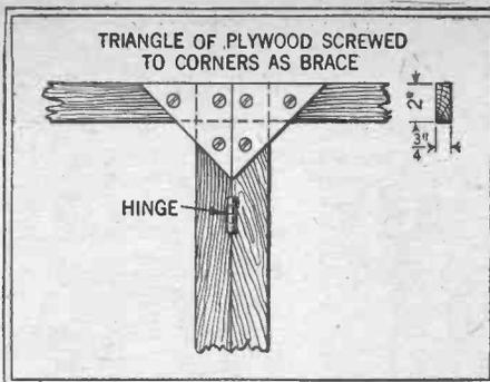
How to brace frame of home-made reflector.
