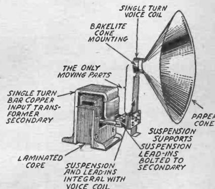
Fig. 7. The features of the dynamic speaker using a single turn moving coil or voice coil are shown above. A single bar of copper constitutes the input transformer secondary.
