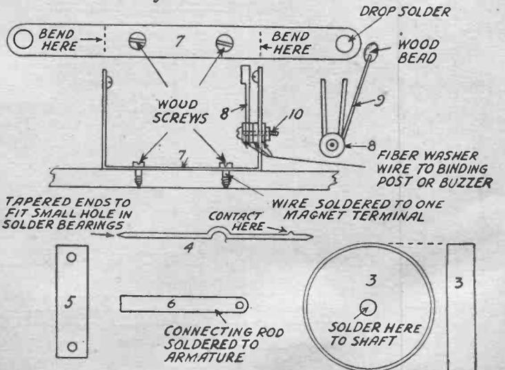
ture of tin; 6, connecting rod, which should be soldered to the armature as shown; 7, shaft bearing; 8, brush assembly; 9, handle for brush assembly; 10, small bolt insulated from shaft bearing; 11, wire as per drawing; the motor will operate forward or reverse upon the pressure of the brush on the small offset near the right hand end of the shaft. Tin can be used
