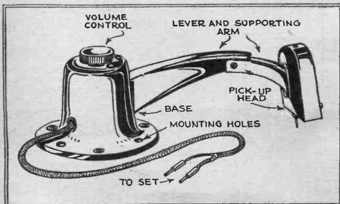
The phonograph pick-up with a volume control incorporated in the base is shown above. This instrument is finished in gold.
