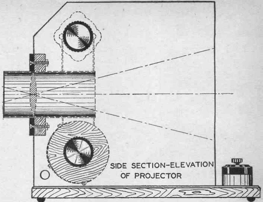
A side-section elevation of the projector is shown above. The placement of lamps and reflectors has been so arranged that no direct light can escape through the lens, but an intense beam may be directed upon the surface to be projected.
