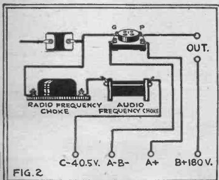
When a 171 tube is used in the last stage, a radio frequency and an audio frequency choke may be connected in series and substituted for R6 in Fig. 1.
