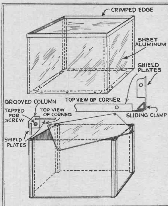
Two types of new aluminum shield cans are illustrated above. One is of thin and the other of thicker aluminum.
