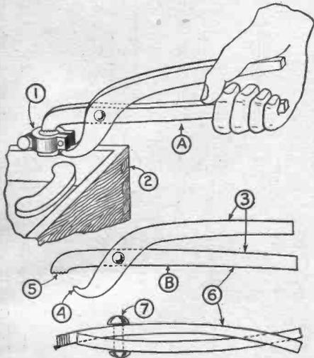
Illustration A above, shows how the plier tool is used. The terminal is shown at 1, 2, is the battery, 3, handles, 4, hook form, 5, serrations, 6, details of tool, 7, bolt or rivet. B illustrates a side view of the tool.
