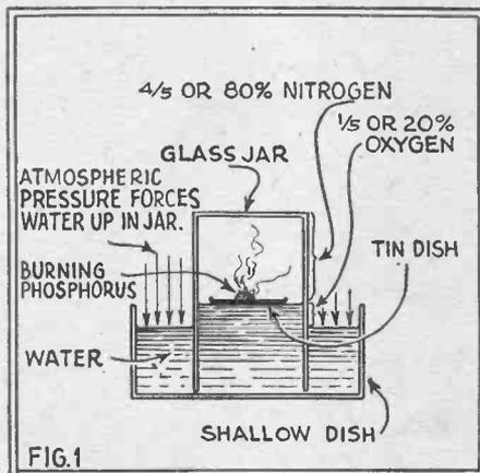
The above experiment shows the composition of the air. As the oxygen is used up water rises in the jar. A candle can be used in place of the phosphorus.
