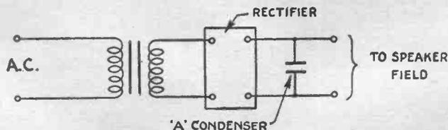
The hum experienced with some types of A.C. dynamic speakers can be eliminated or reduced in many cases by connecting an "A" condenser across the field winding as shown.
