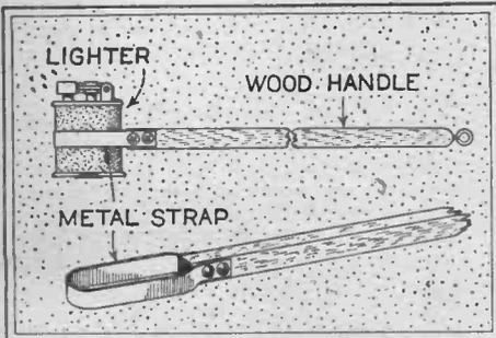
An old cigar lighter provided with a wooden handle makes an excellent gas stove lighter. The wick is lit in the usual manner, and if the familiar pop or explosion occurs in the valve air intake, the user will be out of danger.—L. B. Robbins.
