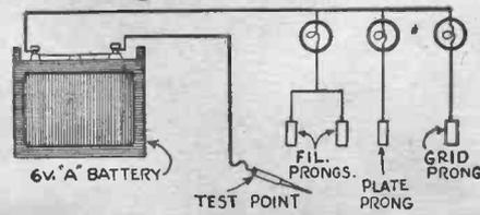
Above—Details of a home made circuit tester.
