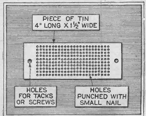
An indestructible match scratcher can be made from a piece of tin, cut to the dimensions shown above. Small holes are punched in the tin with a nail and should be evenly spaced. By scratching a match across the jagged edges of the holes, it will light instantly.—Wm. D. Holmes.
