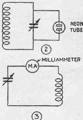
Above in Fig. 2 is shown how a neon tube may be used to indicate resonance and Fig. 3 illustrates another resonance indicator in the form of a milliammeter.
