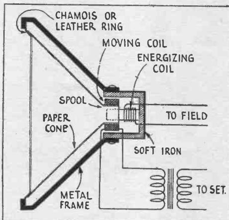
Fig. 5. The principle of construction of all dynamic speakers is illustrated in the above drawing. The speaker using a single turn voice coil is somewhat different.
