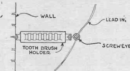
an eye bolt as shown. Cotton soaked in paraffin is stuffed in each end to keep out moisture.—Weiden Cone.
