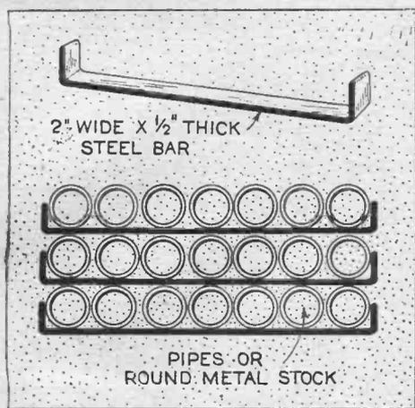
A handy method for stacking pipe or round stock is illustrated above. The stacking bars are made of steel or iron bent at the ends, and of a length to suit the requirements. Two bars are used, one at each end of the pipe, but if the pipe is of small diameter and quite long, it is best to employ a bar at the middle.—H. R. Wallin.
