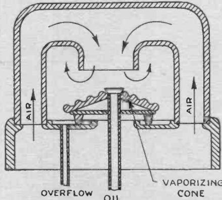
Above is a sectional view of a gravity feed burner used in some types of oil burning furnaces. The oil flows over a corrugated cone shaped apron and is vaporized.
