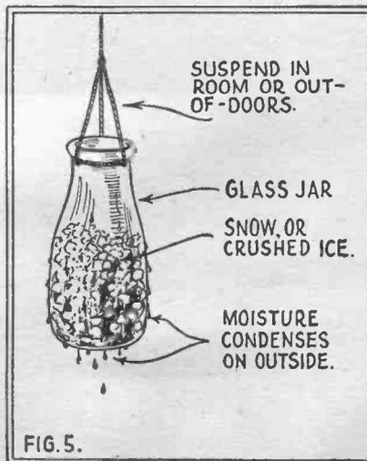
The drawing at the left can be used as a simple proof that air contains water vapor. A glass jar containing snow or crushed ice is suspended out-of-doors or even in the room. After awhile the moisture in the air will have condensed upon the outside of the jar. The water vapor or moisture present in our atmosphere is one of the most important of the component gases. The hotter the air the more moisture it can hold without precipitation. Humidity is an expression of the water vapor in air.
