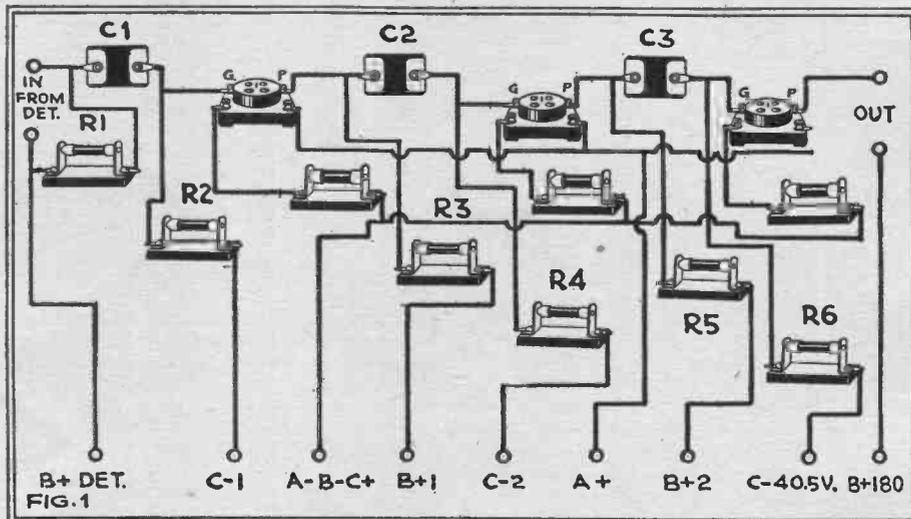
At the left is a picture diagram of a resistance coupled amplifier recommended for use in the reception of television images. R2, R3, R4, R5 and R6, are the grid and plate resistors and C1, C2 and C3, are coupling condensers. A 171 tube is used in the last stage.
