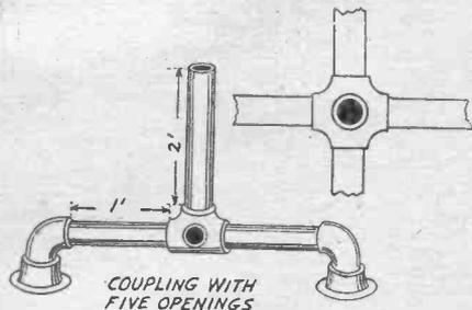
Large beach umbrellas can be placed almost anywhere without driving the handle into the ground, by using a stand made from pipe and couplings, as illustrated here. It is a good aerial mast support also.—C. F. Feldstead.
