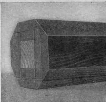
After the final step in gluing, plug the ends for centering and bevel the corners to reduce vibration in the lathe.
