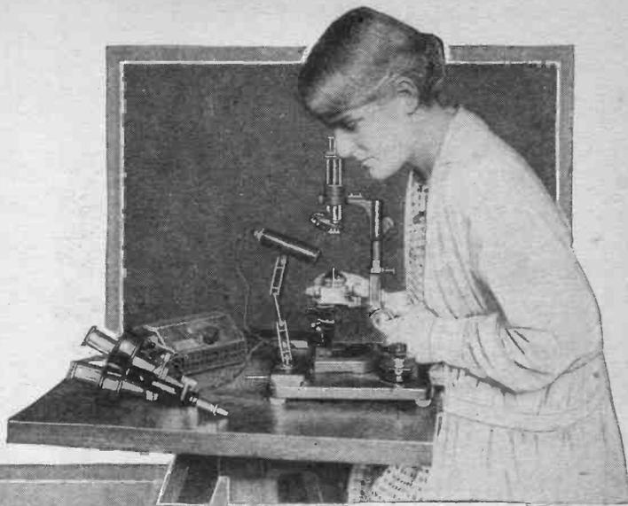
The above photo shows a special microscope for examining the core of pearls that are pierced. A small glass tube is threaded through the pearl which rests upon a revolving platform.
