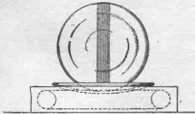
No. 1,666,721, issued to Richard M. Sherrill. The invention shown above produces a rotary magnetic field in which a metallic ring is allowed to rotate giving the appearance of a solid ball. The conventional Gramme ring with a tapped field winding is used. A single phase alternating current is supplied to the ring through a phase splitting device. The Gramme ring is concealed in a case below a glass bowl for the spinning object.
