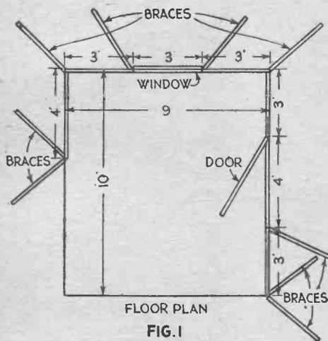
The floor plan of the studio appears in the above drawing. This measures 9 ft. x 10 ft. Note the placement of braces.
