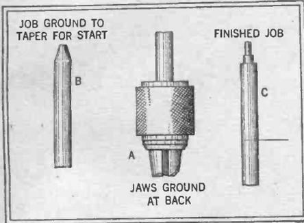
When there is no horizontal lathe available for pin cutting, the jaws of an ordinary vertical or press drill can be ground to a rake which converts it into an adjustable cutter. It is advisable to grind a taper on the end to cut B for the purpose of a good start. A shows the jaws ground at the back and C the finished job. The job can be held in a drill vise or disused lathe chuck.
