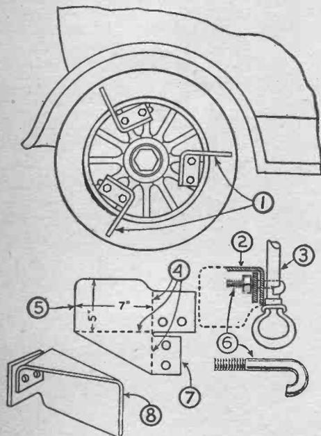
In the above illustration, 1, shoes; 2, fastener; 3, spoke; 4, bend; 5, shoe pattern; 6, hook type bolts; 7, heavy gauge sheet metal; 8, shoe bent to shape.
