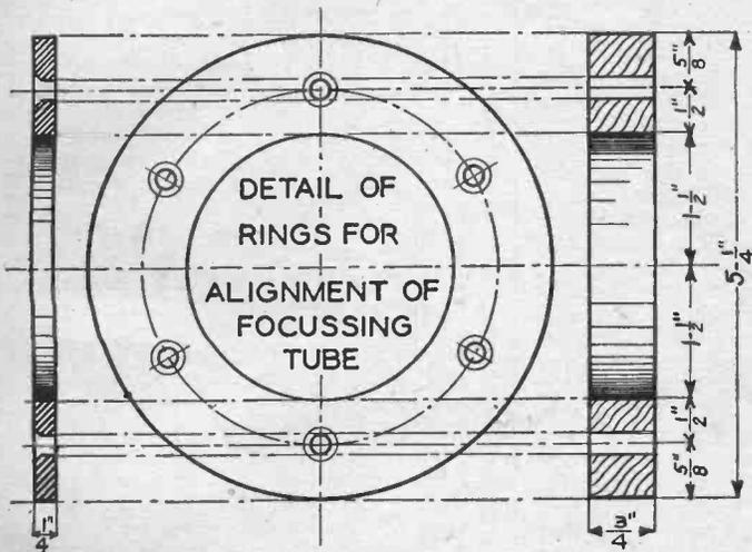
Details of the rings for the alignment of the focussing tube.
