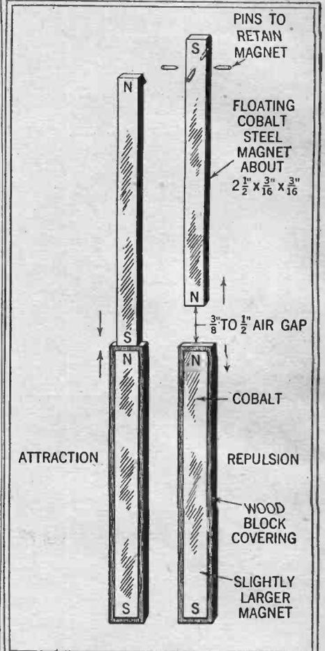
The attraction and repulsion force of the cobalt steel magnet is shown above. The floating magnet was retained in position by two channels, so that its north pole would be adjacent to the north pole of the magnet in the wooden block.
