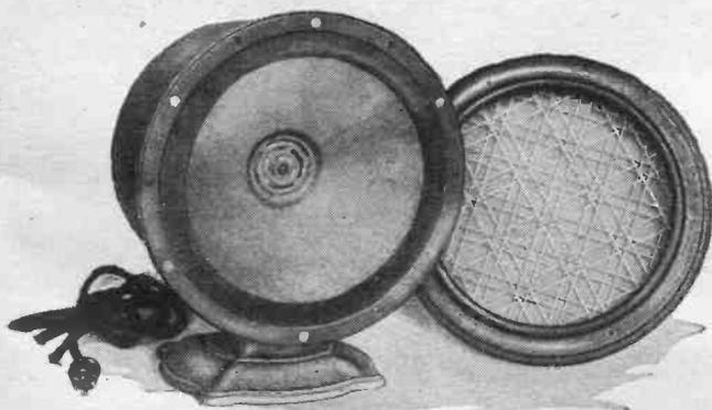
Fig. 6. One of the latest types is enclosed in a metal case fitted with a suitable stand and is shown above. The front grill has been removed, in order to show the cone. The cord is provided with a four prong base for connections to the set and voltage supply.
