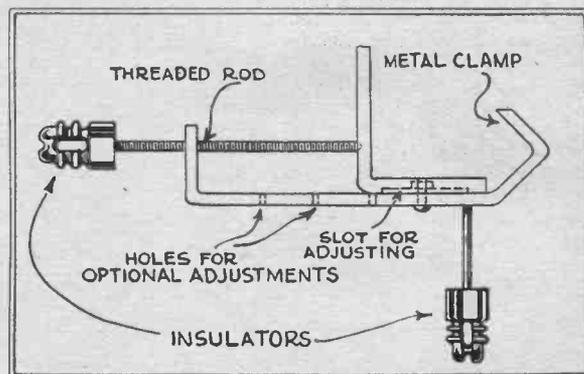
The aerial clamp is illustrated above. A slot and a number of holes are provided for optional adjustments.
