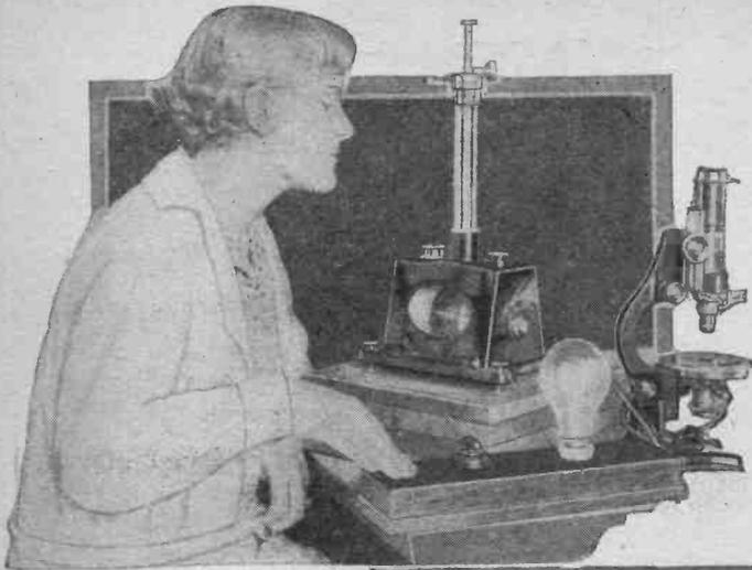
↑ Above—Testing a pearl by the electro-magnetic process. The stone is suspended from a thin glass rod within a magnetic field.
