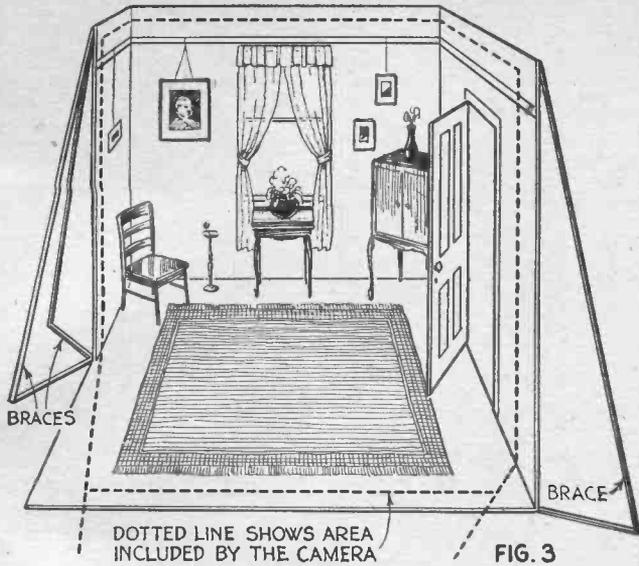
'Above is an interior view of an amateur set, the dotted lines showing the area included by the motion-picture camera.'
