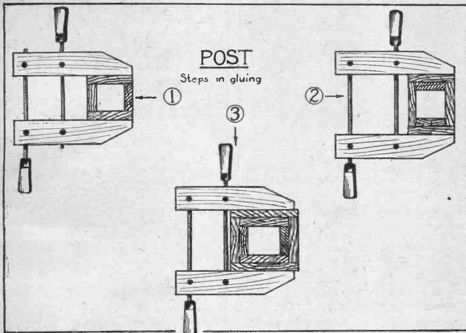
Illustrating steps in gluing the post preparatory to its turning.
