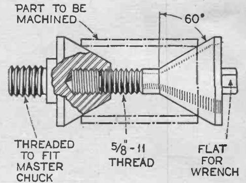
The above illustration gives the details of a chuck, which will be found valuable in machining sleeves and collars whose inside diameters are not of standard size. If it is accurately made, the work done will be found to be as true as if a special mandrel were employed.—James Marsh.
