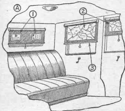
In the above drawing, an inside view of the car is shown at A. Licenses and permits are shown at 1, and maps, at 2. The papers are exposed when the curtain is lowered, as at 3.
