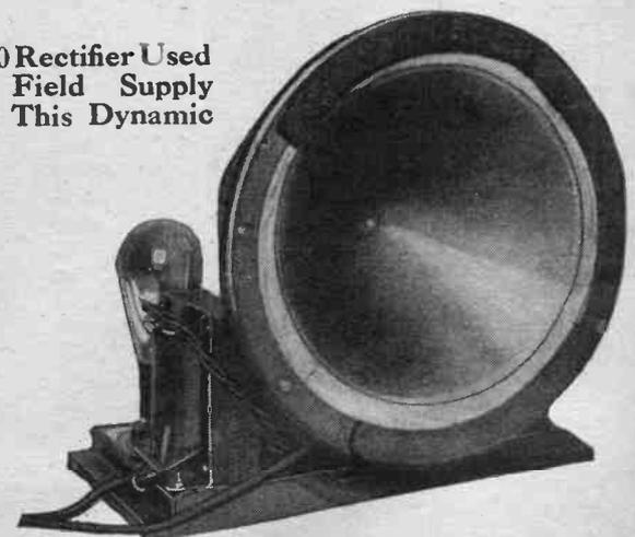
Fig. 3. The speaker shown above obtains the field coil supply from a 280 type rectifier which supplies direct current. The transformer and rectifier tube may be seen at the left.
