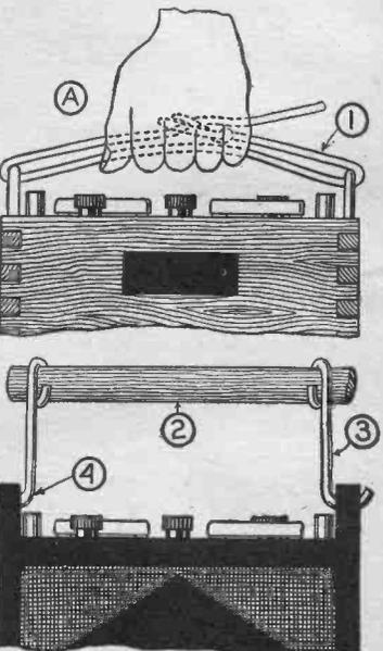
Illustration A above shows a carrier for a metal handle battery. The leather strap and buckle are shown at 1. Illustration B shows how a rubber case battery may be carried. A length of broom handle or wood is indicated at 2; 3 shows iron wire, and 4, the hook.
