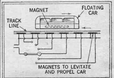
The above illustration shows how a car could be levitated and propelled by means of magnets.
