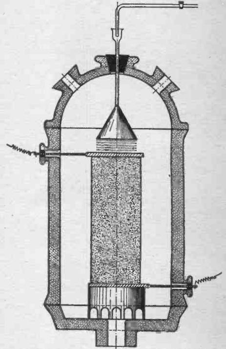
No. 1,688,679, issued to Gustav Baum. This process effects the heating of liquids for distillation and the like by utilizing the liquid itself as a resistance between two electrodes. An insulating structure divides the liquid into streams, thus increasing its resistance.
