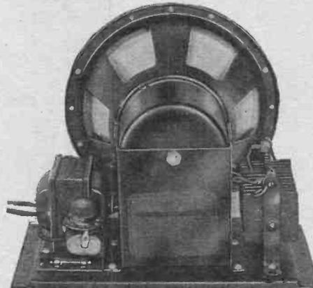
Fig. 2. A rear view of a dynamic A.C. chassis is shown above. The condition equalizer is an outstanding feature and is shown at the rear of the base to the left. The dry rectifier is at the right.
