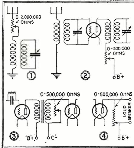
The illustration above shows four methods of controlling the volume in radio receiving sets. The simplest volume control is a variable high resistor placed in series with the antenna lead.
