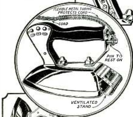
The iron is equipped with a ventilated stand and a cord protected with flexible metal tubing. At the left it is shown resting in an upright position upon the stand.
