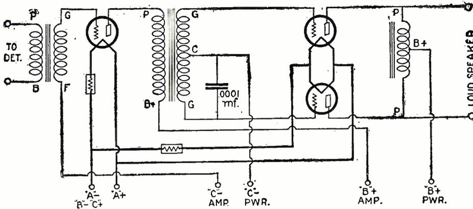
The circuit diagram for a push-pull amplifier using Radiola III-A audio transformers appears above. A small unbalancing condenser having a capacity of about .0001 mf. is connected across one-half of the secondary of the push-pull input transformer.
