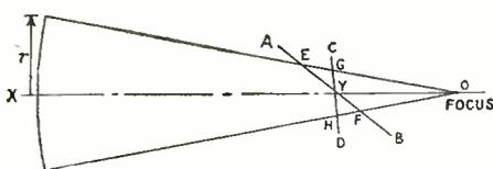
Above—Method of determining size of elliptical flat. Fig. 7.
