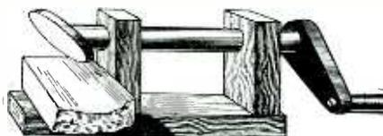
The method of grinding the elliptical flat mirror is shown above. Fig. 7-A.
