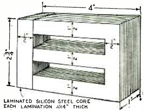
LAMINATED SILICON STEEL CORE EACH LAMINATION .014" THICK 71 - W TYPE LAMS. 71 - RECTANGULAR LAMS.
