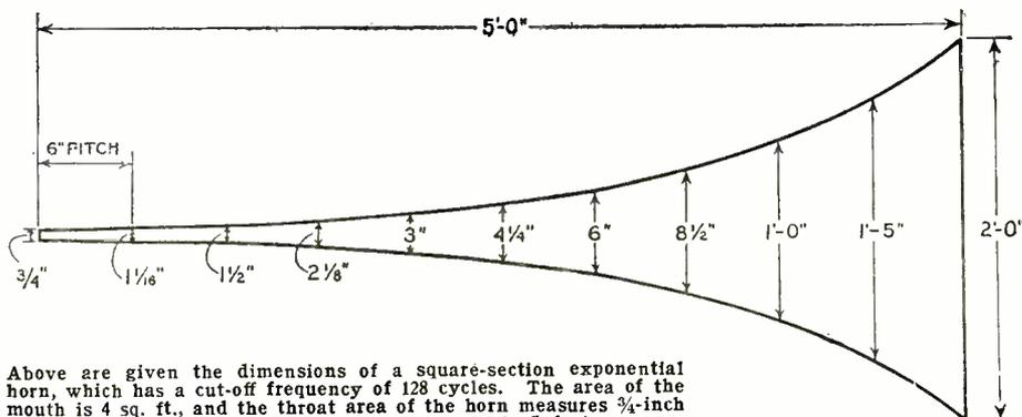
Above are given the dimensions of a square-section exponential horn, which has a cut-off frequency of 128 cycles. The area of the mouth is 4 sq. ft., and the throat area of the horn measures 3/4-inch square. The total length of the horn is 5 feet.
