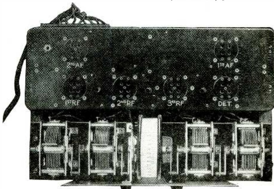
The chassis of the new receiver is shown here. The four tuning condensers are arranged for drum control. Another novel feature lies in the fact that the illuminated dial is calibrated in wave-lengths.
