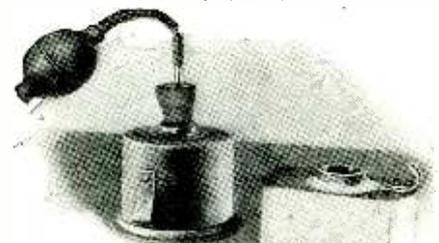
An efficient tester for small tanks and the like can be made as shown. The tank is submerged in water, and the rubber bulb pressed. Any leak will then instantly appear as tiny bubbles will be noticeable. This method is better than simply submerging the tank in water, as it tests the tops also.—
