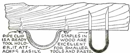
ORDINARY light sheet iron pipe clips secured to the wall behind the machine or on the machine stand, provide perfect hangers for all kinds of tools. The clips are obtainable in various sizes. Ordinary wire staples will provide excellent hangers for small tools such as reamers, taps and drills.—G. L.
