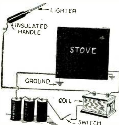
An electric match for the gas stove can be easily made from an old spark coil, a storage battery, or several dry cells, a switch and an insulated handle, as shown in the above illustration.—Glen F. Stillwell.
