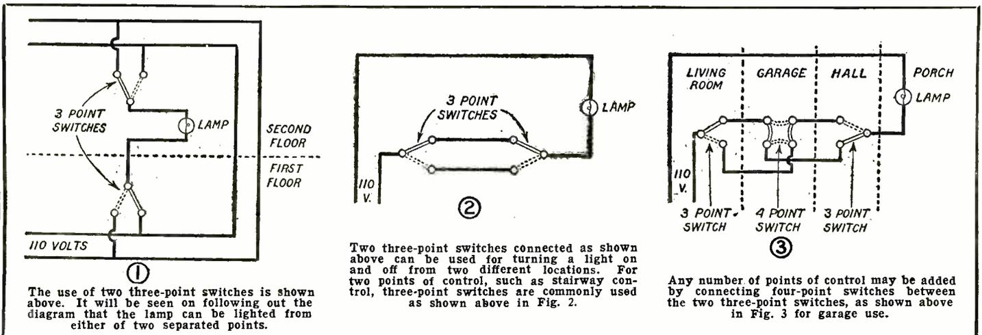
The use of two three-point switches is shown above. It will be seen on following out the diagram that the lamp can be lighted from either of two separated points.
