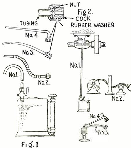
The above drawing gives the details of the pressure oiler, and also shows various shaped spouts which can be used with this ingenious device. The spouts are removable.
