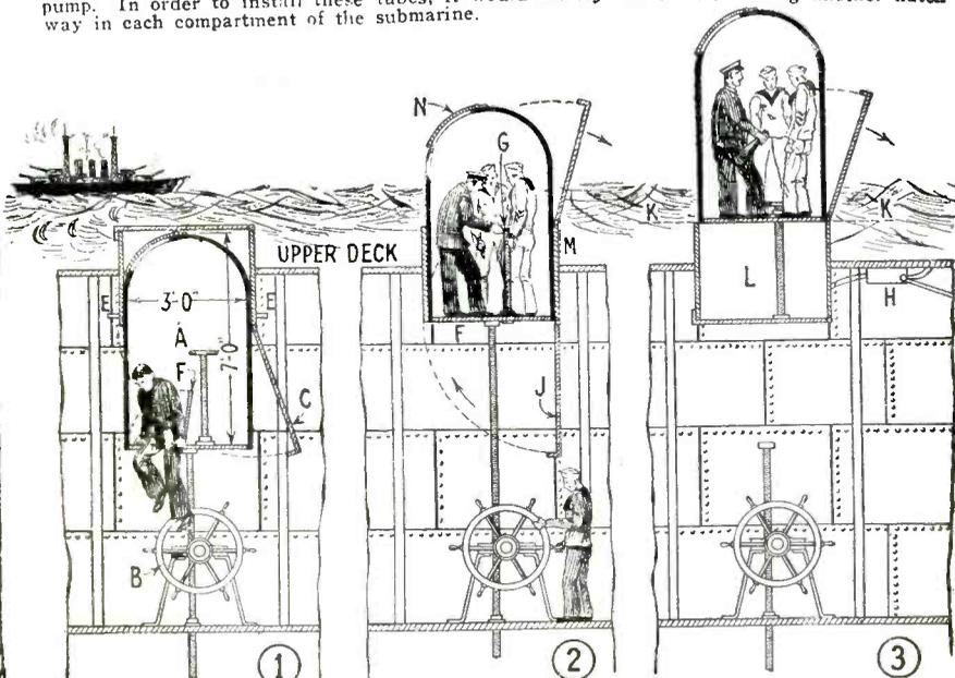
The above drawing shows three stages in the process of using the submarine lifesaving torpedo. No. 1 shows one of the crew entering the chamber. No. 2 shows how the chamber is raised to the upper deck by a man in the submarine. No. 3 shows the final stage, with the trap door closed. The lifesaving tube, being buoyant, will then rise to the surface. Each compartment of the submarine would be fitted with an extra hatchway, as shown above.
