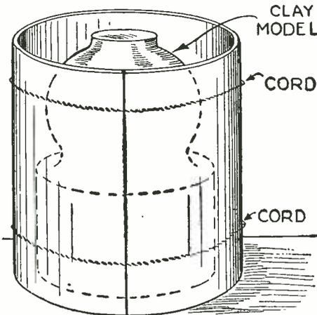
THE PLASTER IS Poured INTO A MOLD MADE OF SHEET METAL OR LINOLEUM.
