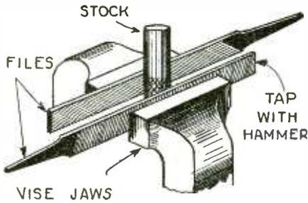
A SIMPLE and efficient means of knurling can be accomplished as shown above. The work or stock is clamped between two milling files, a moderate pressure is applied and the end of one of the files is tapped carefully, so that the work rolls between the two files. Both files must be parallel and the work must be placed at right angles to them. The tangs of the files are placed at opposite ends.—H. Pelder.
