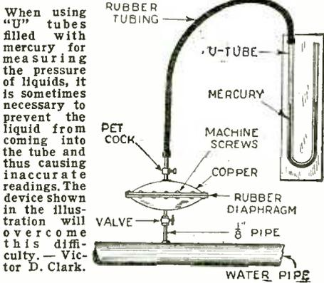
When using "U" tubes filled with mercury for measuring the pressure of liquids, it is sometimes necessary to prevent the liquid from coming into the tube and thus causing inaccurate readings. The device shown in the illustration will overcome this difficulty.—Victor D. Clark.
