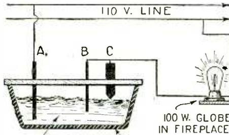
An artificial fireplace fitted with the arrangement shown above will seem most realistic in appearance. The device keeps up an intermittent flashing resembling the flickering of the flames. Rod A is immersed into the water, B is a thin rod or a heavy piece of wire. Rod C is very heavy and has a pointed tip. To operate the device, merely keep the water in motion.—Paul Wirth.
