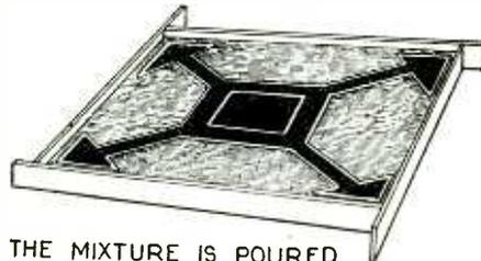
THE MIXTURE IS Poured INTO A MOLD TO MAKE A TILE
