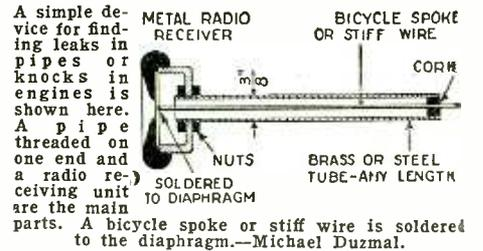
A simple device for finding leaks in pipes or knocks in engines is shown here. A pipe threaded on one end and a radio receiving unit are the main parts. A bicycle spoke or stiff wire is soldered to the diaphragm.—Michael Duzmal.
