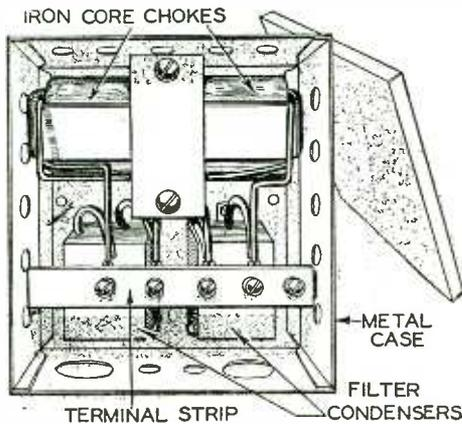
A front view of the radio interference filter with the cover removed is shown above. The device is housed in a ventilated metal case.
