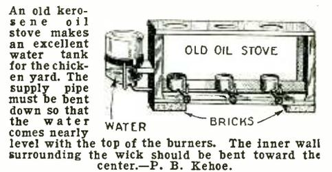
An old kerosene oil stove makes an excellent water tank for the chicken yard. The supply pipe must be bent down so that the water comes nearly level with the top of the burners. The inner wall surrounding the wick should be bent toward the center.—P. B. Kehoe.
