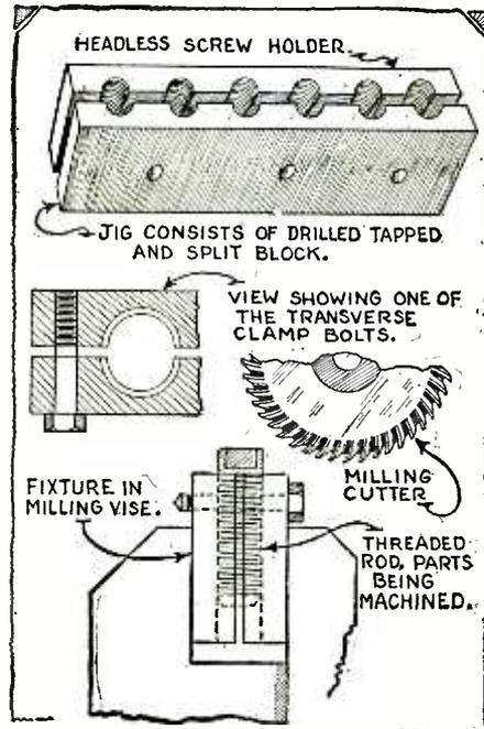
The above drawing shows a jig for holding headless set screws for machining. A block is tapped out for holding six or eight screws.
