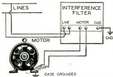
The wiring diagram of the radio interference filter is given above. The manufacturer of this device makes a small filter for use with equipment rated up to one-quarter horsepower, and a large filter to be used with motors and other appliances up to 5 horsepower at 220 volts. Five terminals are provided on the filter.
