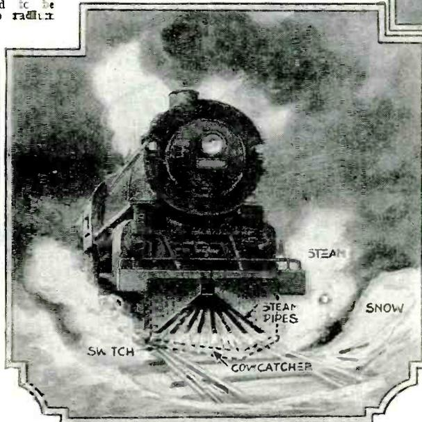
Special snow-fighting locomotives have been adopted by several eastern railroad yards, in order to clear the switches of snow. The engines are equipped with nine pipes arranged in a "V" just behind the cow catcher. Live steam is forced through these pipes and strikes the snow and ice directly beneath, melting it directly. One large railroad has twenty-five of its locomotives equipped in this manner, in order to safe-guard against winter delays.
