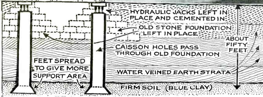
The large diagram at the left, together with the insert, showing a top view of the circular wall of the tower, illustrates the manner in which a famous American foundation company would go about building a substantial foundation under the Tower of Pisa. According to this scheme, the tower would be left in its present position, while caissons would be sunk progressively around under the tower, these being filled with cement.
