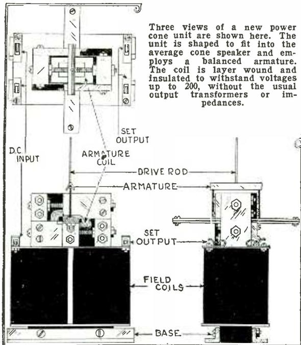
The unit shown above, a product of a New York City manufacturer, employs a powerful electro-magnet, instead of a permanent magnet. The electro-magnet draws .3 amperes, the current being supplied from a 6-volt source.
