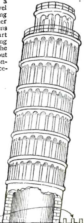
The diagram below and at the right shows how a famous French engineer proposes to freeze two circular rings of soil about the base of the tower; he will then pump in cement under pressure and in this fashion he eventually will build a water-tight foundation under the tower in its present position. A detail of one of the brine pipes is shown below.
