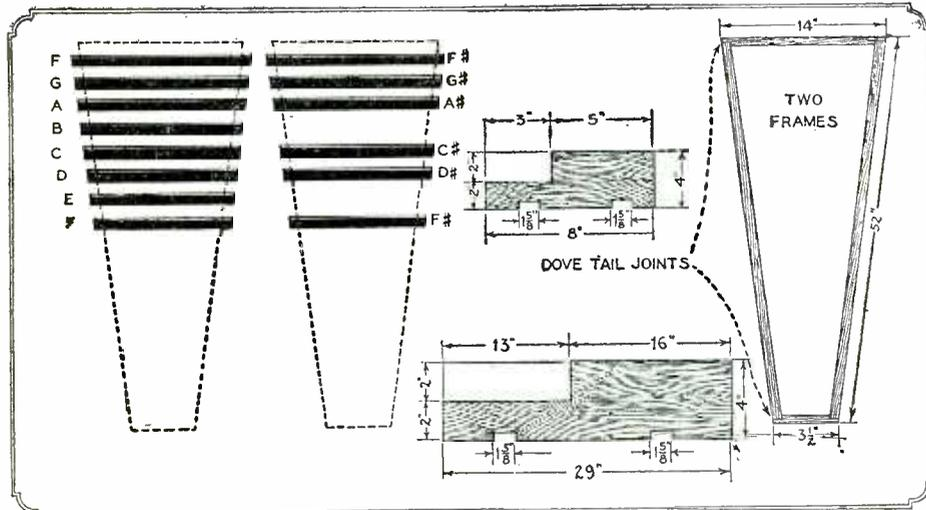
The above diagram shows how the Xylophone is assembled. Note that the sharp and flat bars are strung in groups of twos and threes and are raised on the frame slightly above the naturals. This makes for ease in handling the notes.
