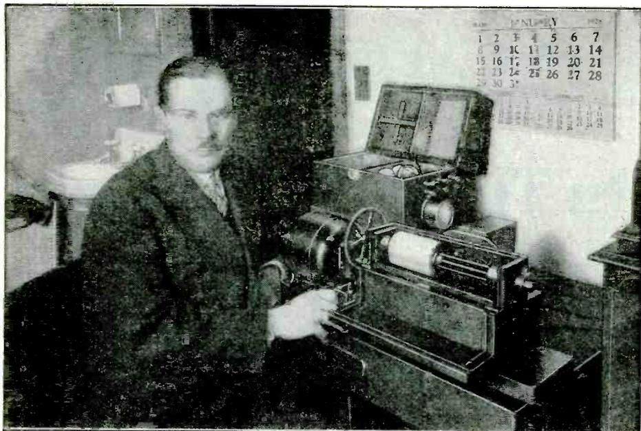
Above is Dr. E. F. W. Alexanderson and his home radio-picture receiver. Against the wall is a box containing the rectifying and amplifying units. The cover of the receiver has been lifted, showing the photographic paper.
