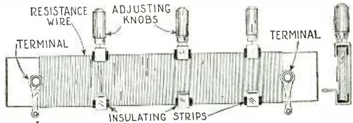
The adjustable resistance for use in "B" eliminators is shown above. These are wound with enameled wire and are provided with sliders for obtaining different voltages.
