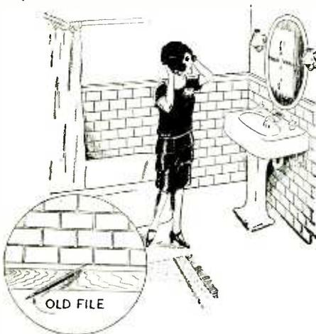
Either new or old plastered walls can be finished like brick or wall tile in the simple manner shown in the sketch above. The wall is grooved about an eighth of an inch deep with an old file or other sharp tool. A straight board is used as a guide. Bricks 3" x 6" are about the right size. After grooving, the wall is treated with a coat of size and then finished with enamel.—*Harold Jackson.*
