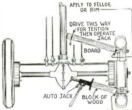
AUTOMOBILE wheels which have become stuck and cannot be removed can be loosened as shown above. A board is wedged for the proper tension and a jack and another block of wood are placed as shown. The wooden boards are applied to the felloe or rim.—Contributor, send name and address.
