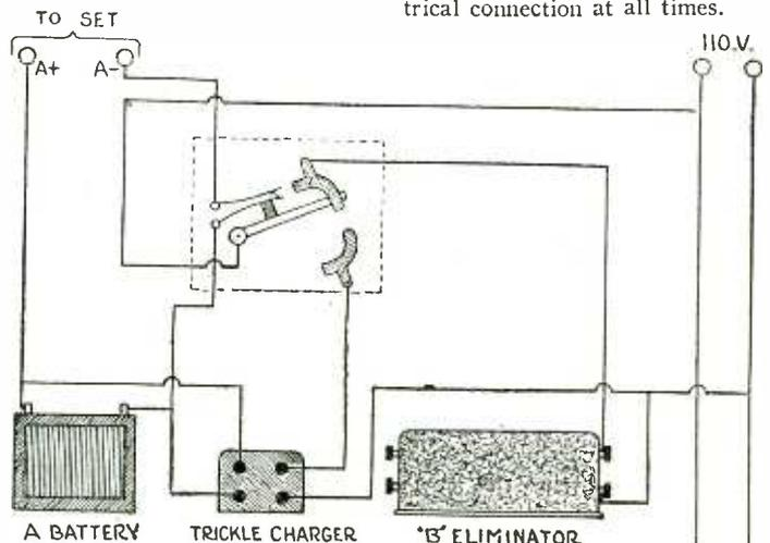
The wiring diagram of the 110 volt power switch is given above. It can be mounted on the panel of the set, and takes the place of an automatic relay.
