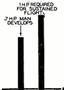
The chart shows that the average man can develop only 7 horsepower. It takes approximately 1 horsepower to operate a flying machine.
