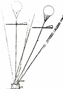
No. 1,652,996, issued to Luis Azaraga. The object of this machine is to provide a sign which can be held aloft by a captive balloon, and further be continuously illuminated at night. The balloon is free to swing in any direction and is fastened to a tether line.
