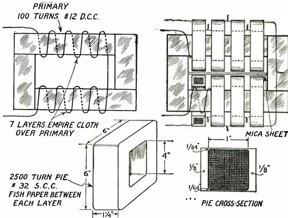
The above illustration shows various details in the construction of the 20,000 volt transformer. The secondary consists of eight sections, each one having 2,500 turns of No. 32 S.C.C. wire.
