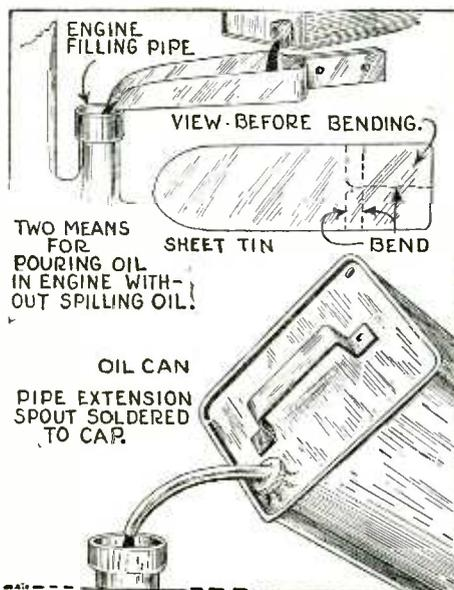
Two suggestions for avoiding the spilling of crankcase oil are shown here.
