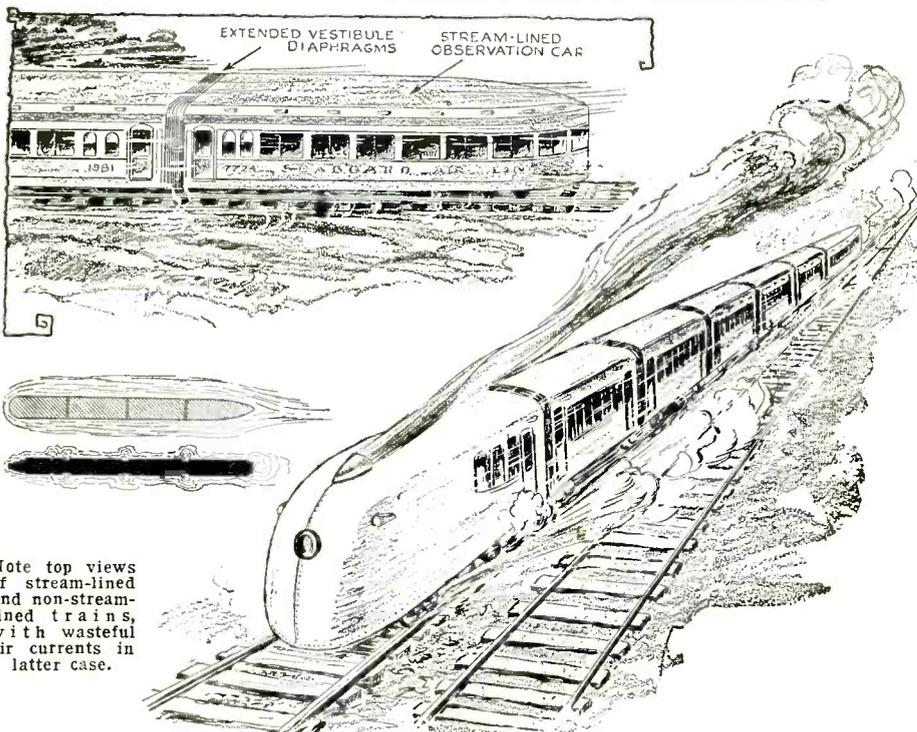
Note top views of stream-lined and non-stream-lined trains, with wasteful air currents in latter case.
