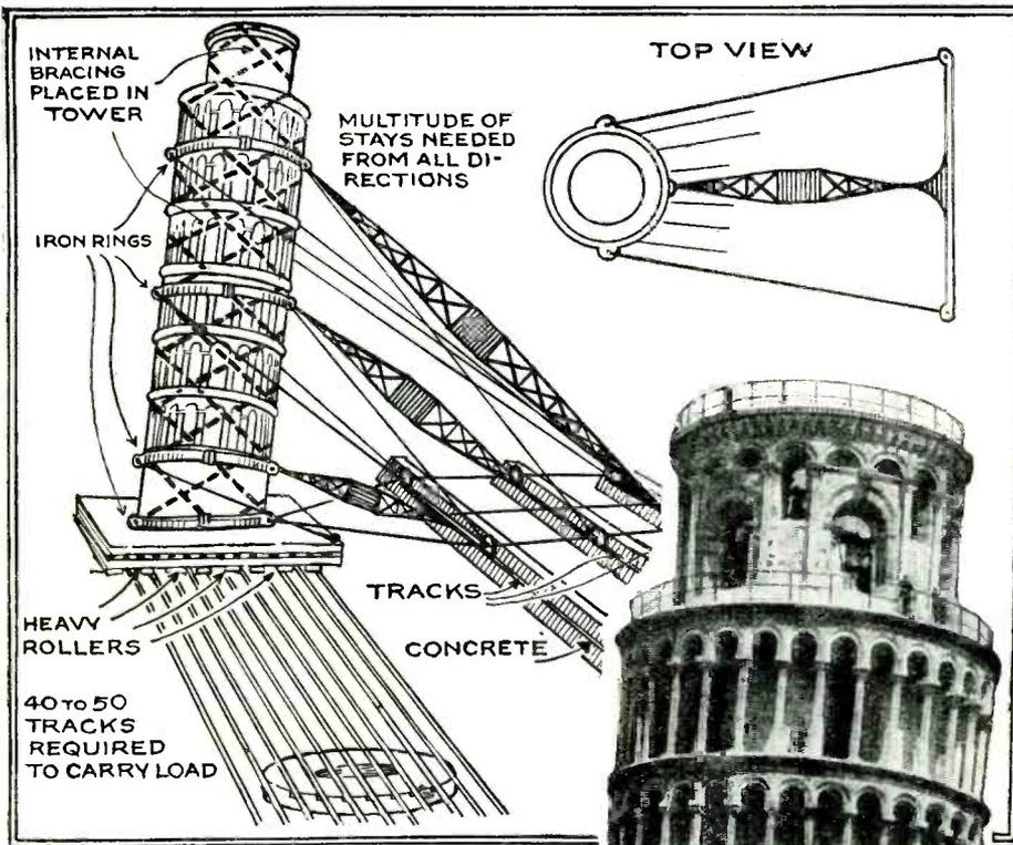
The author's scheme for suitably supporting the leaning tower of Pisa with a multiplicity of arms or braces is shown above. When the tower has been suitably supported and shored up on a platform placed on rollers, which in turn rest on a series of rails, it can be readily moved to a new foundation.
