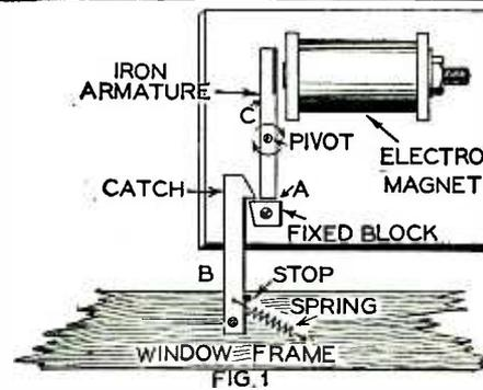
Fig. 2 shows the general arrangement of the device; the hook-catch with its spring drawing it to the right appears on the top of the frame of the lower sash, which is shown closed in the picture.
