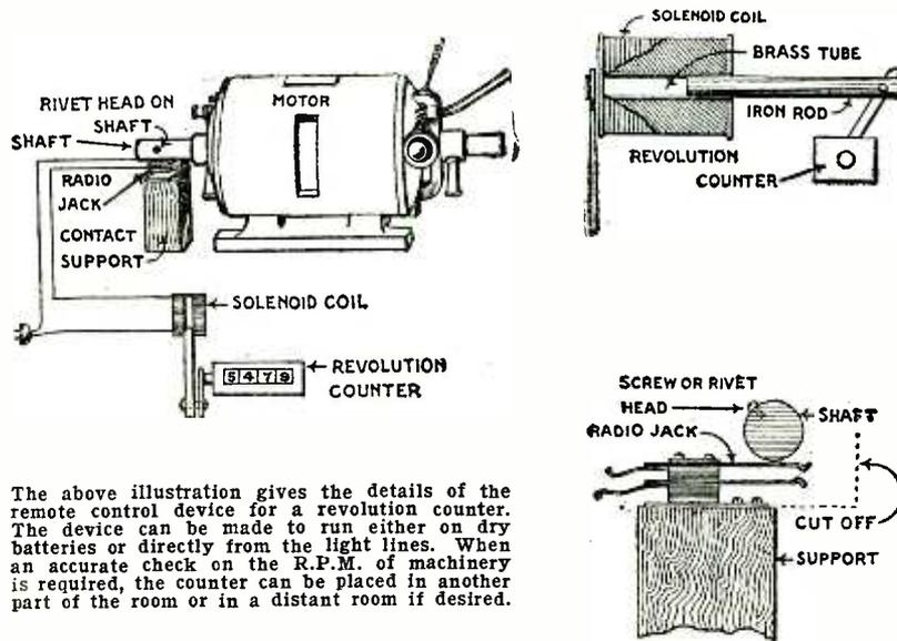
The above illustration gives the details of the remote control device for a revolution counter. The device can be made to run either on dry batteries or directly from the light lines. When an accurate check on the R.P.M. of machinery is required, the counter can be placed in another part of the room or in a distant room if desired.
