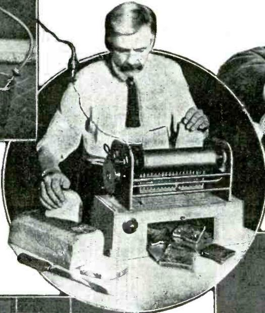
The photo at the left shows a new electric toaster which is capable of toasting fifty slices of bread a minute. It is operated and heated electrically. The photo shows Mr. E. W. Roberts, the inventor, with his machine.
