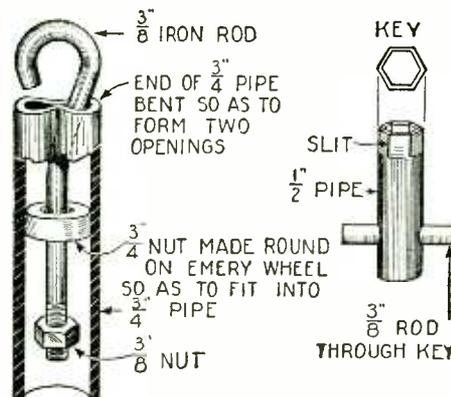
The above illustration shows the constructional details of a simple home-made lock which can be made from a few odd parts. The main portion is made from a piece of 3/4-inch pipe, one end of which is crimped together, so as to leave two openings.—Paul Louque, Jr.
