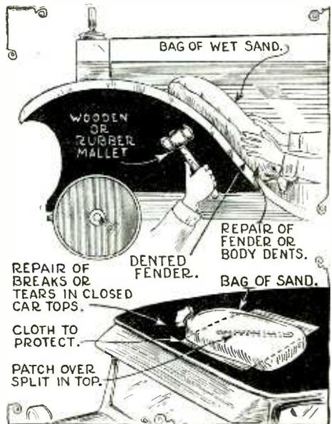
A bag of wet sand is very useful when straightening a dented fender or a body dent. A bag of sand is also of service when repairing a tear in the car top.
