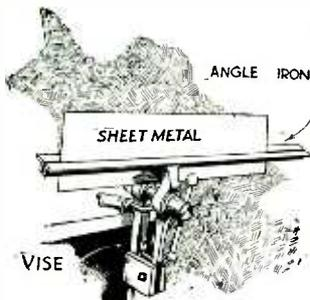
iron are placed in the vise and the sheet of metal bent between them. This holds it firmly throughout its entire length and the upper portion can be bent over and pounded down with a wooden mallet. Large sheet of metal may be bent perfectly straight when using this kink.—Harold Jackson.
