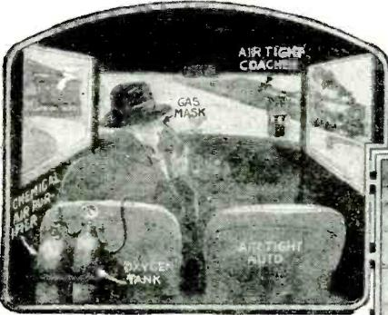
Here we have an illustration showing an air-tight automobile, equipped with an oxygen tank and chemical air purifier. The gassed citizens would be removed to safety in a coach of this nature. Furthermore, the driver is equipped with a gas mask. This precautionary measure against gas attack was suggested at the International Conference of the Red Cross.
