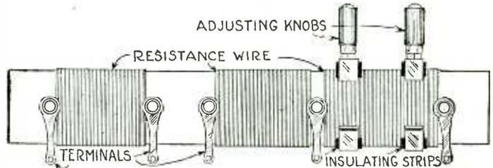
Another type of resistor is shown above. This is used primarily for obtaining "C" battery voltages from the "B" eliminator.
