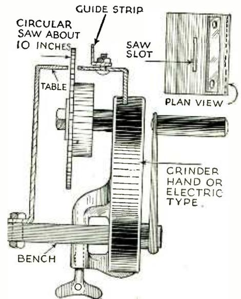
A small circular saw can be attached to the bench grinder as shown above. A saw about 10" or so will facilitate light sawing. Details of a sheet metal table top are also shown.
