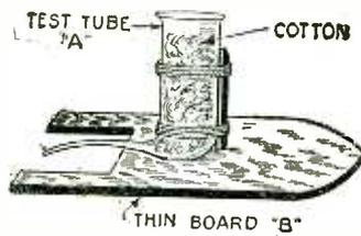
A boat which secures its motive power from surface tension is shown above. A is a test tube with the lower end drawn out. This is placed upon a thin board. The test tube is now filled with absorbent cotton and alcohol, or soapy water is poured in.—H. H. Roseberry.
