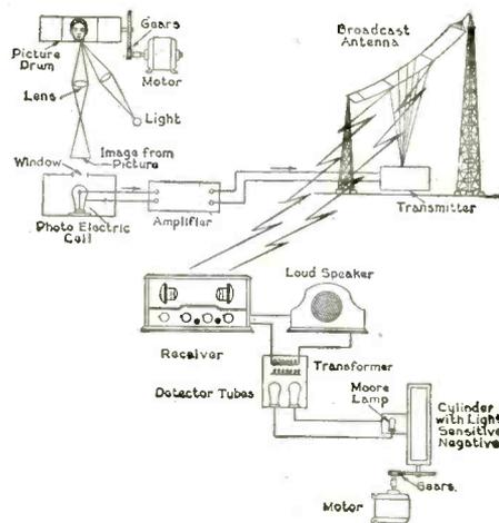
The diagram above shows how the pictures are sent and received by radio. A slotted disc, not shown in this diagram, revolves in front of the window which admits light to the photo-electric cell.
