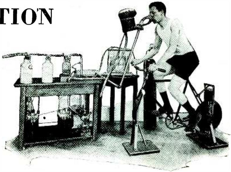
The above photograph shows the ergometer used at the Nutrition Laboratory in measuring the effects of muscular activity on the carbon dioxide output of the human body and also measuring combustion, both with and without food. Carbon dioxide is formed in the body, which uses oxygen in greater quantities during muscular exertion.
