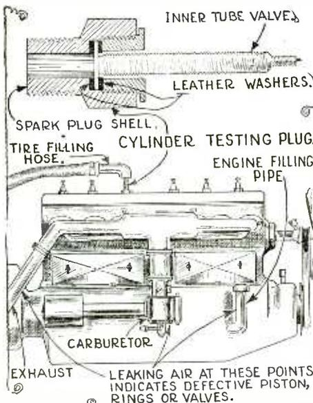
A cylinder testing plug for determining compression losses, is made and used as shown above.
