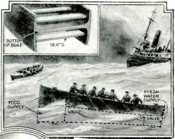
A new unsinkable boat was recently demonstrated in London. Besides being unsinkable the boat is reversible, self-emptying and cannot be capsized. It is built like two broad punts, placed bottom to bottom. Tanks of fresh water and food are placed at each end. In the bottom of each boat are two valves which let out the water.
