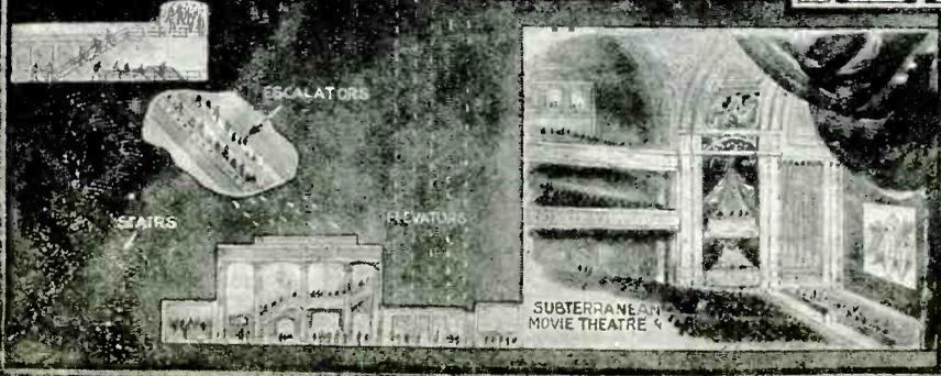
At the left we have a subterranean movie theatre as a place of amusement and retreat during a gas attack. The theatre would be connected to the surface with elevators, escalators and stairways. Huge quantities of fresh air would be drawn in, filtered, and then passed out into the theatre. The pressure on the inside will be greater than that on the outside, so that any poisonous gases which may find their way down below the surface will be prevented from entering the theatre.
