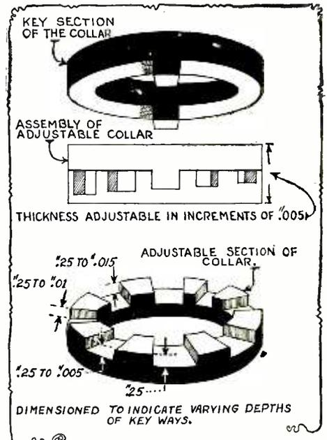
THE collar shown above can be made cheaply and quickly, and will do away with the use of thin shims. The collar can be made in size to be adjustable to any fractional part of an inch and for use with any piece of machinery. It consists of two parts. One part is made with two keys and the other with key seats of varying depth.—G. A. Luers.
