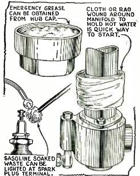
Emergency grease can be obtained from the hub cap. A cloth wrapped around the manifold, with boiling water poured upon it, will help to start a cold engine. Gasoline soaked waste can be lighted from the spark plug terminal, by detaching the wire as shown.
