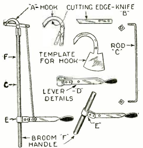
A home-made lever twig cutter can be constructed from the parts shown above. The handle is made from an old broom handle. A lever and collar (E) slip over the handle.—Tom Shively.
