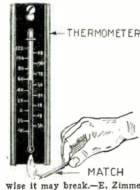
When the mercury column in a thermometer is broken, the thermometer will not register correctly. A good method to repair the break is to hold a lighted match under the bulb, so that the mercury goes almost up to the top of the tube. This forces the pieces together, and the thermometer is as good as ever. Care should be taken so that the flame is not put too close to the bulb, otherwise it may break.—E. Zimmer.
