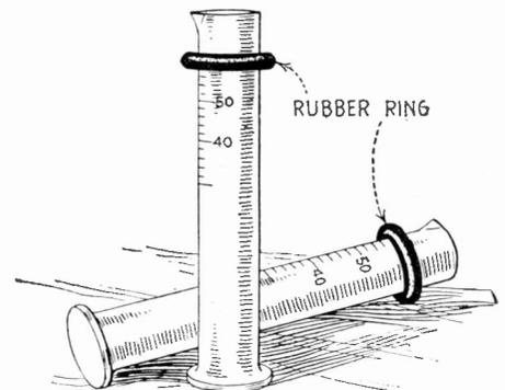
If a rubber ring such as used on suction flasks is placed around a graduate as shown above, it will prevent breakage. If the graduate falls on its side, the rubber ring absorbs the shock.
