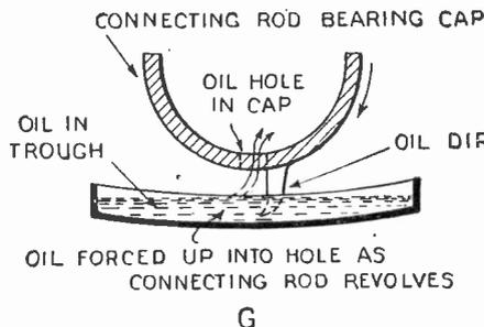
In the splash-pressure system, the connecting rod bearing cap should be placed in such a position that the oil will be forced up through the hole by the action of the oil dip. If the cap is on backwards, lubrication will not take place and burned out bearings will result. This is plainly seen in Fig. G. above.
