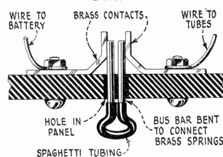
A simple "A" battery switch is made from two brass contacts and a length of bus bar bent as shown.
