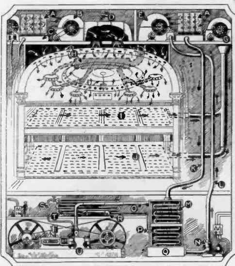
K, water returned by gravity from spray chamber and recooled. L, cooled water pumped to sprayers on roof. M, cooling coils. N, pump. O, carbon dioxide suction line to compressor. P, expansion valve. Q, cold water tank. R, carbon dioxide high pressure liquid receiver. S, discharge line to condenser for high pressure carbon dioxide. Typical daily temperature chart appears at right.
