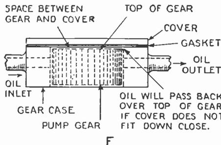
Two other causes of low pressure are shown in Fig. F above. If there is play in the teeth of the gear pump, the oil will not flow properly and the pressure will be low. If the cover on the gear case is not tight, there will also be a lack of pressure. The remedies are obvious. New gears in the first case and a new gasket or tightening of the cover in the second place.
