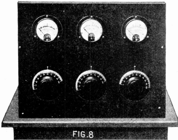
The panel containing the wave-length controls and the various meters is shown directly above. The dial indicators are scratched in the panel and then filled in with white paint.
