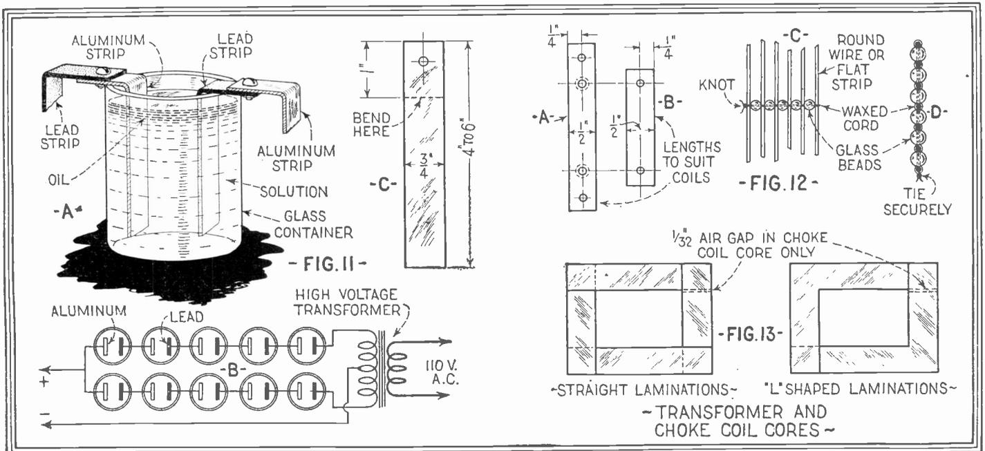
Fig. 11 gives all of the necessary details for constructing an electrolytic rectifier and for connecting it in a circuit. Follow carefully the directions
