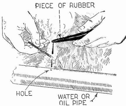
A small hole in a water or oil pipe of an automobile can be temporarily mended by melting a piece of rubber over it and allowing the drops to fall over the hole. Make a permanent repair as soon as possible as the rubber will not last.
