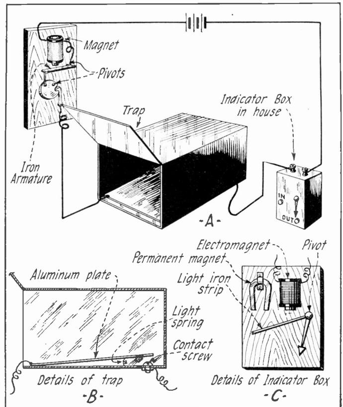
A pigeon trap that will not only catch and hold the bird but will also announce that a capture has been made is illustrated above. A bird entering the trap closes the contacts which sends the current through the indicator box and through the electro-magnet release. The door, which is heavy enough to hold itself closed, then falls and at the same time the indicator, detailed at C, shows that the trap has been sprung. Upon resetting the trap, reset the indicator by hand. —John Kautzner.
