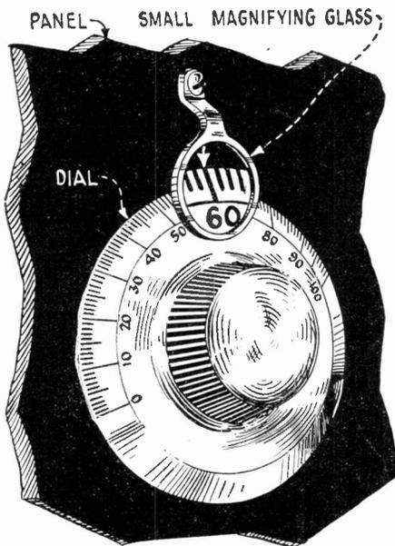
On small dials it is often hard to read the exact setting. This trouble can be eliminated by arranging a small magnifying glass directly over the pointer as shown above. Close tuning is also simplified in this manner.
