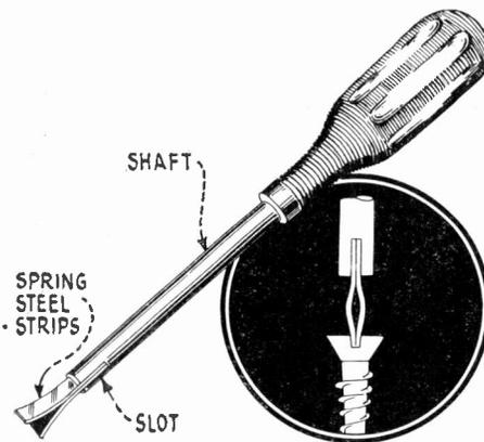
A screw driver that will hold a screw while it is being started in an accessible place is made by using two spring steel strips as above.
