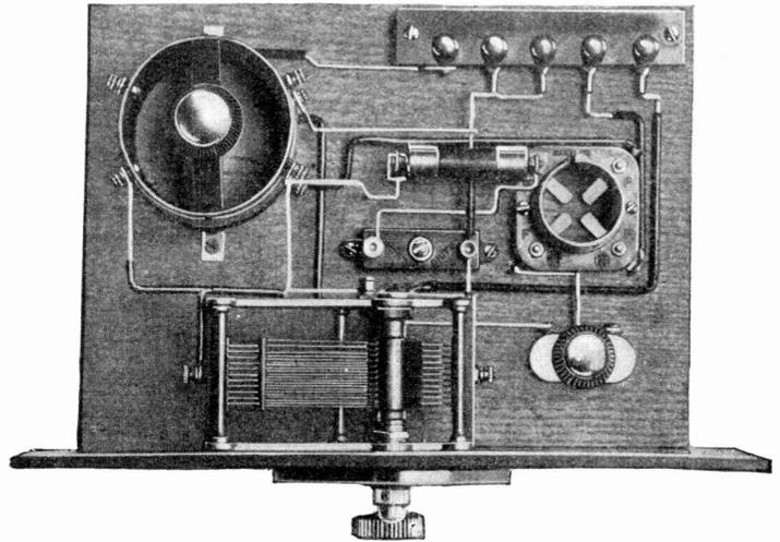
Fig. 2. Top view of receiver. Note balancing condenser directly below the fixed carborundum crystal detector of the cartridge type.
