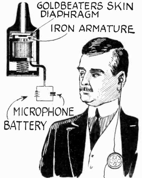
No. 1,545,525 issued to H. Sell protects a novel type of very small telephone receiver that fits into the ear and requires no head band or other holding device. The details of one of the receivers are shown in the upper left-hand corner and the device is illustrated in use above. It can be used for various purposes, the most important being as an aid to people hard of hearing.
