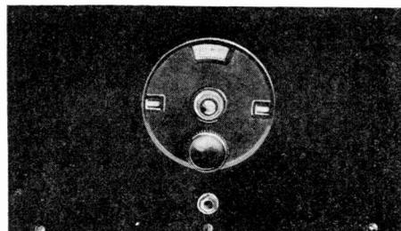
Fig. 3. The panel view of this receiver shows the extreme simplicity of tuning. Only a single tuning control is employed.
