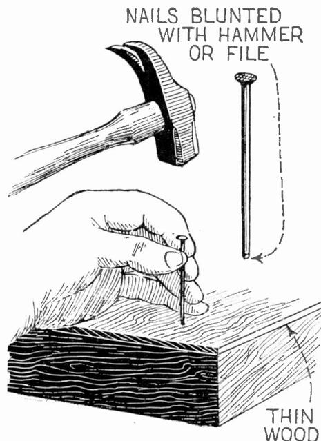
To avoid splitting thin wood, hammer or file the ends of the nails to a wedge shape and drive the nails so that the wedge-shaped point crosses the fibers. Much splitting of thin wood will thus be eliminated.—Max Ruschmann.
