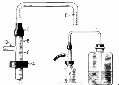
When handling liquids having disagreeable fumes, the above device is useful. Attach D to a suction pump. A partial vacuum is created in the bottle being filled and the liquid from the large bottle passes into the small one through the long bent tube.
