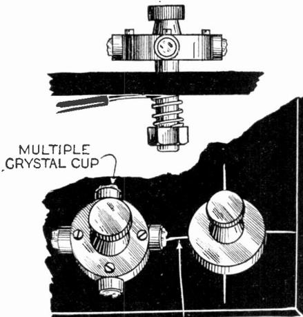
Sixteen different combinations of crystal and contact point can be obtained with an arrangement such as that illustrated above. Four points and four crystals are arranged on adjacent revolvable disks. —G. A. Luers.
