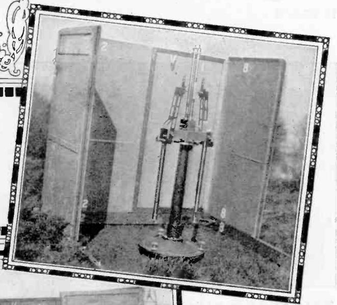
The balance is surrounded by a double or triple wall of metal sheets so that it will not be affected by outside disturbances. A deflecting mirror indicates the presence of minerals or oils.
