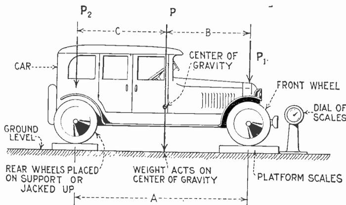
The finding of the center of gravity of an automobile may seem to be a hard problem, but if approached properly it is easily solved.
