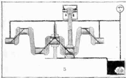
In the forced feed system, the oil is only forced to the main bearings and to the connecting rod bearings as in Fig. B above. The piston or wrist pins and the cylinder walls are lubricated by the oil splash from the crankcase.
