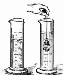
The specific gravity of bodies that are heavier than water can be determined by actual measurement of their volume if the method is followed; the method is explained in the text.
