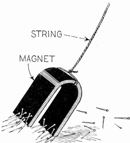
When a quantity of nails or other small iron or steel objects are spilled on the floor, they can easily be picked up by means of a magnet suspended on a string as shown above. The magnet is drawn across the floor several times and when picked up will be found to bring all of the magnetic objects with it. In this way, a job that was formerly tedious can be performed with little effort and in a small fraction of the former time.—E. L. Dunbar.
