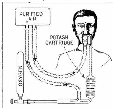
This simplified diagram shows the action that takes place in the breathing apparatus of the under-water rescue suit. See text for full explanation.
