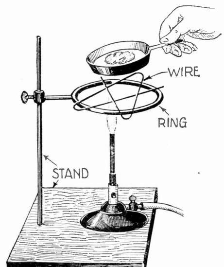
In the chemical laboratory, often large ring stands only are available. To support small evaporating dishes or other apparatus on them, bend a piece of wire into the shape shown above and support the receptacle thereon. In some cases, two large wire hairpins can be laid across the ring, with the same results. This kink is one worth bearing in mind as it will often come in handy.—Jesse Walters.
