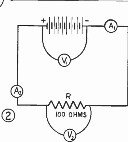
2 In the circuit shown in Fig. 2 above, two volt meters and two ammeters are connected in a circuit with a battery and resistance. In this particular case, which ammeter, if either, will read higher, and which volt meter?
