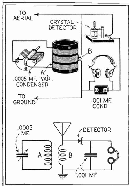
A simple crystal detector circuit using the absorption method of tuning is shown above.
