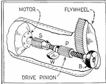
A diagram of a standard Bendix gear for automobile starting motors is shown above and described in this column.
