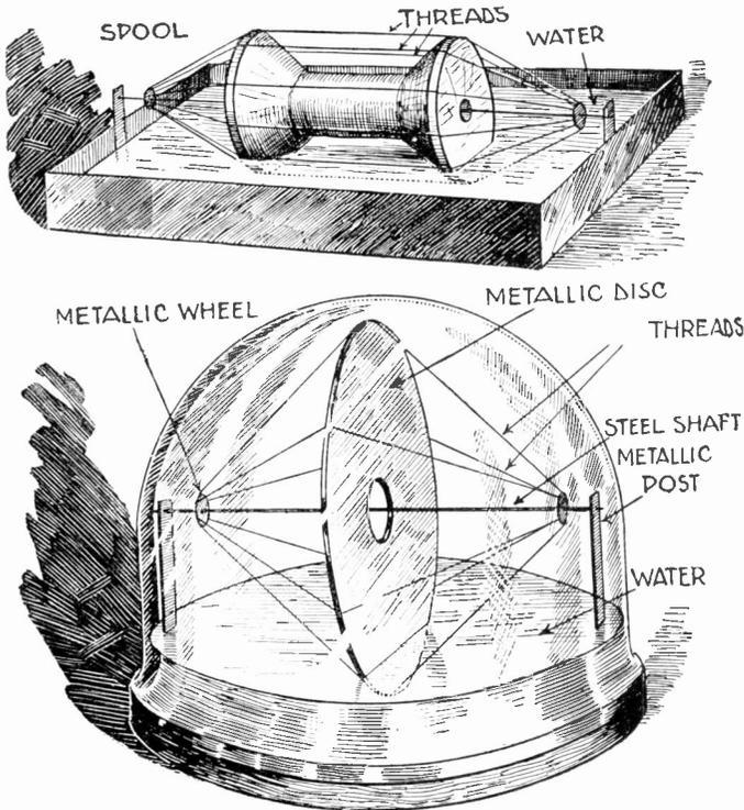
An interesting motor that will revolve without any visible external source of power is illustrated above. Two different types are shown. The uppermost can be quickly and easily made from a spool, several lengths of thread and a suitable wire axle. Assembled as shown, the wheel will turn about one revolution every 8 minutes. A more elaborate model may be made as shown in the lower part of the above illustration. —Emile Dion.
