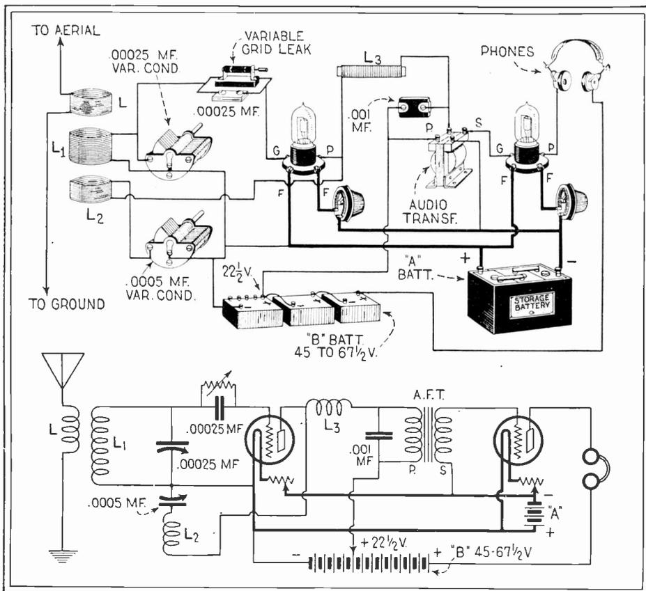
A short-wave receiver opens new fields for the radio enthusiast. An excellent type for use with headphones is shown above. The data for coils covering the 40 and 80 meter amateur band is given in the text. Follow it carefully in order to obtain the best of results.
