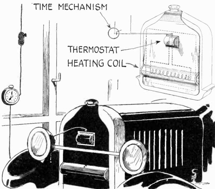
No. 1,534,220 issued to A. J. Kercher covers a device that should make cold weather motoring more of a pleasure and that certainly will prevent an excessive drain on the battery when starting. Actuated by a clock, the heating coil is turned on at a predetermined time, but if the car is not used in a short period, the device cannot overheat because of the thermostat included. The apparatus is removed when the car is taken out of the garage.
