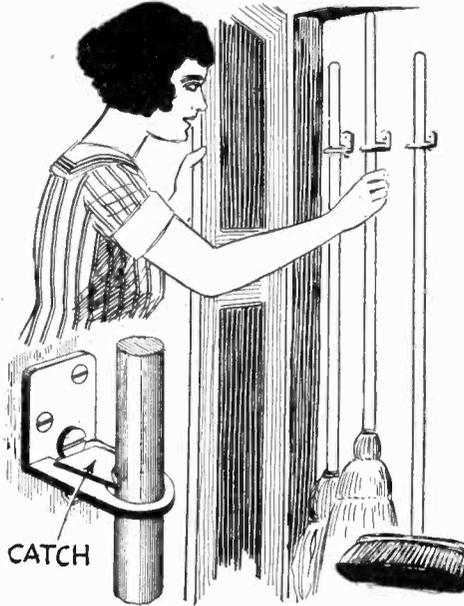
No. 1,540,291 issued to W. P. Sessions pertains to a novelty that should find wide use among housewives. The broom holder is screwed to the wall and to hold a broom in position it is only necessary to push it upward through the hole and release it. The catch holds the broom in place. To remove, lift up the bottom of the catch with the finger and take the broom out.
