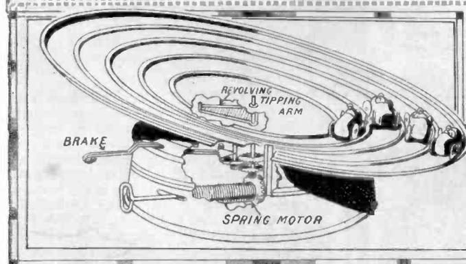
The turntable of the automobile race track illustrated above and to the right is caused to tip progressively by a small revolving tipping arm located immediately below the turn table. Four tiny automobiles are placed on the track and are caused to race around at a surprising speed. At times the innermost car will be in the lead, and at other times any of the other cars will take the lead.
