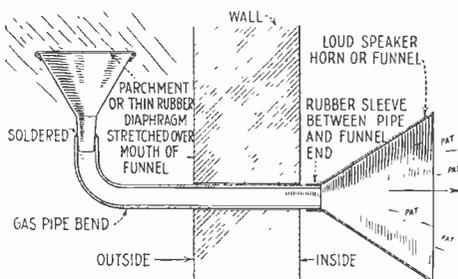
A rain alarm that requires no batteries or moving parts is detailed above. Two funnels, a diaphragm and a bent gas pipe are all that are required. The rain falling on the diaphragm produces sounds that are plainly audible at quite a distance from the reproducing funnel. The rubber sleeve facilitates removal.
