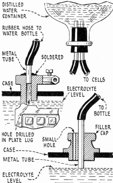
The electrolyte in a storage battery can be kept at constant level if an inverted distilled water container is placed at a point higher than the battery and is equipped with tubes, one running to each cell of the battery. Two methods of allowing the water to enter the battery are shown. All tubes must be airtight.
