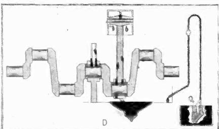
The simple splash system depends upon the height of the oil in the bottom of the crankcase into which fins on the connecting rods dip. This is shown in Fig. D above. The oil level in the crankcase must be maintained by filling before running or by a special pump and an outside oil tank.
