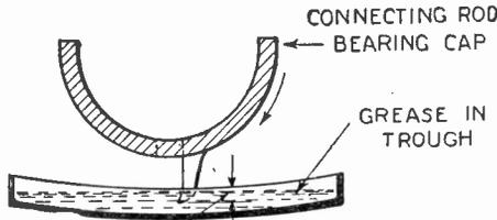
DISTANCE DIP GOES INTO OIL, INCREASE LENGTH OF DIP, FOR MORE OIL TO BE FORCED UP INTO CONNECTING-ROD BEARING.
