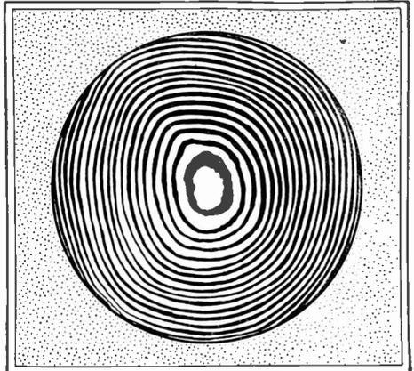
Newton's rings formed as described here take the appearance illustrated above. Note the gradations of widths of the rings.
