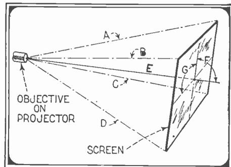
Under certain conditions, a motion picture screen must be tilted in relationship to the stage at an angle, determined by the line shown above.
