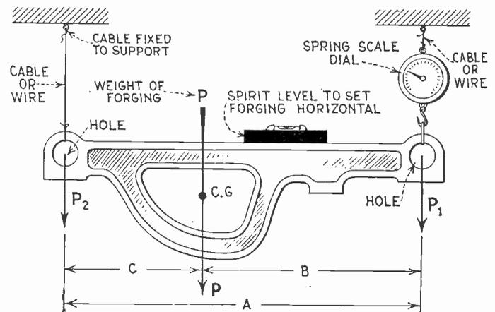
Above: Finding center of gravity of an irregular forging.
