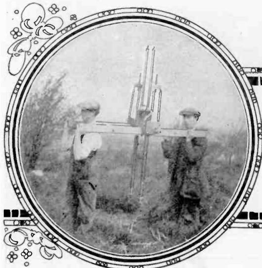
Left: The Eotvos Torsion Balance designed by Baron Roland von Eotvos of Budapest being taken into the field for testing its ability to locate oil and mineral deposits.
