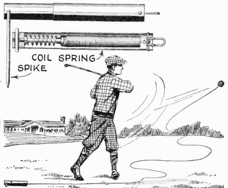
No. 1,541,420 issued to G. H. Lambert protects a device that enables golf practice to be carried on in a limited space. Furthermore, it enables the golfer to practice driving without having to chase the ball. As shown, a heavy coil spring is connected to a long cord, to the other end of which the ball is fastened. The ball is placed on a tee in the usual way and driven. It can only go as far as the cord will allow it to travel.
