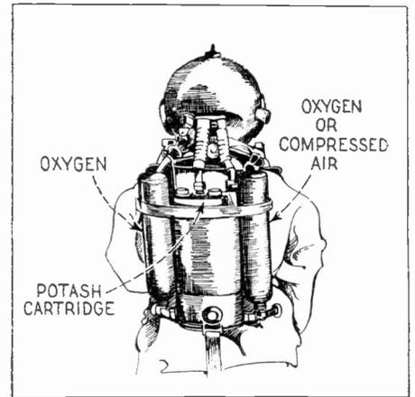
Rear view of an up-to-date diving suit showing oxygen tanks and potash cartridge for regenerating the air supply.
