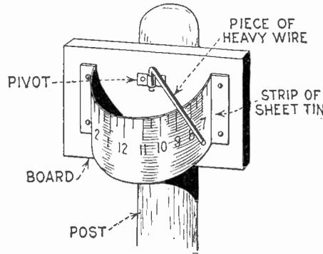
The details of a unique sun clock are shown above. To read the time, the wire arm is swung until its shadow assumes a vertical position. The correct time is indicated by the shadow as at only one point on the dial will the shadow be vertical at a given time. The figures are inscribed on the dial by setting the sun clock each hour by a watch. In this way the clock is made quite accurate.
