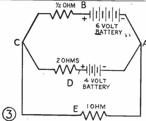
3 Considering the resistance of the battery and the connecting wire as negligible, which way will current flow through the branch of the circuit ADC? What effect could a change in resistance in ADC have upon the flow of current in this branch?
