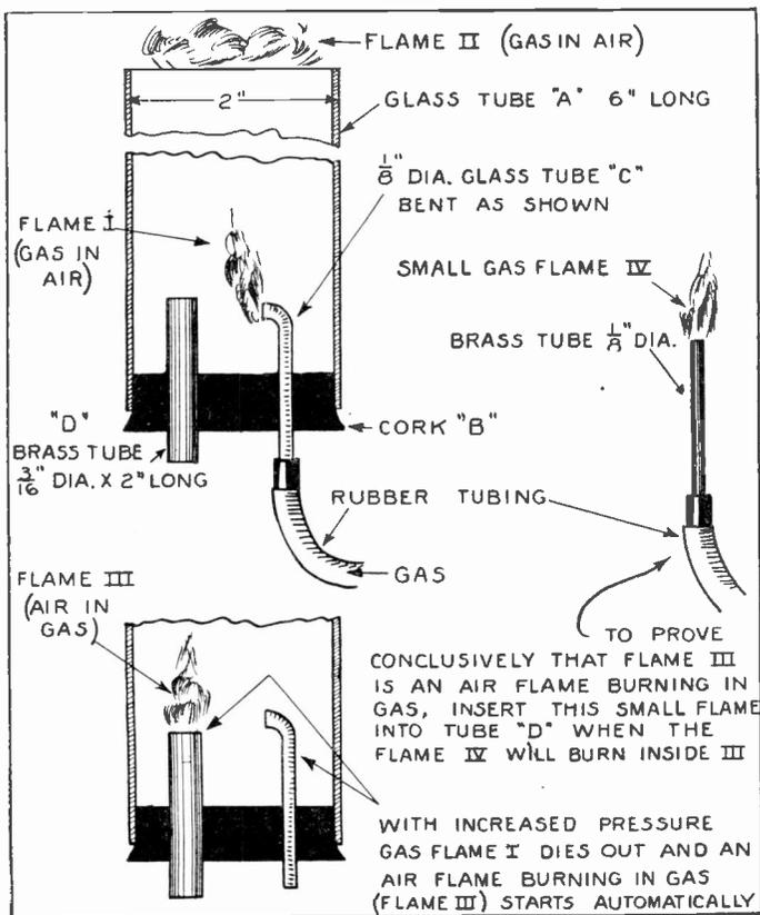
We know that a gas flame burns in air but will an air flame also burn in gas? This experiment answers the question. The apparatus necessary is shown. Connect the glass tube to the gas supply. Open the gas valve slightly and light. As long as the flame is small it will burn, but if turned on full, the flame will die out. At the same moment an air flame will form automatically on tube D and we can light another gas flame II at the top of the large glass tube. —C. A. Oldroyd.
