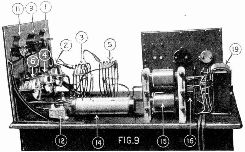
Another side view of the transmitter is shown here. The filter choke coil and the plate transformer can be seen at the right-hand end of the photograph. The R.F. choke coil is in the center indicated by 14.
