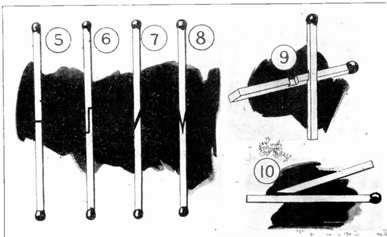
Fig. 5. Here a number of match joints are illustrated. The contestant will find that it is a rather simple matter to make any of these joints and with the exception of the joint shown in 5, all of the other joints are quite sturdy.
