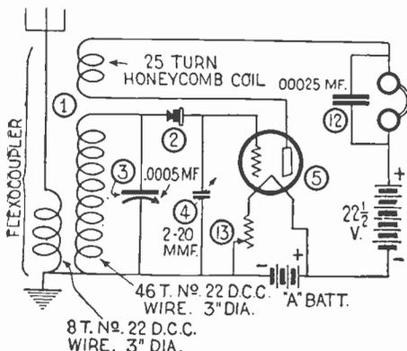
Fig. 4. The circuit diagram of the one tube Regenerative Interflex receiver shows all of the connections for the various instruments used. A variable grid condenser can be placed at 4.
