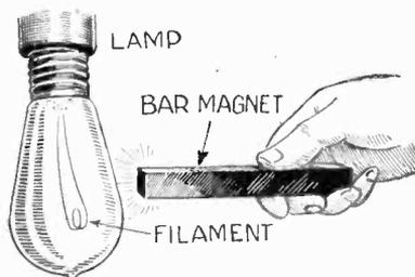
If a bar magnet is held near the filament of a carbon lamp, and D.C. is flowing through that filament, it will bend toward the magnet as shown. If the current is alternating, filament will vibrate.—J. F. Kasak.
