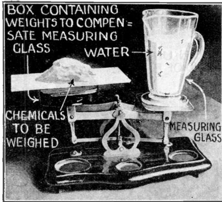
The experimental chemist whose supply of graduated weights is limited may use water instead. Place a graduate on one pan and a weighted box on the other to balance. Then each cubic centimeter of water in the graduate will balance one gram in the opposite pan.
