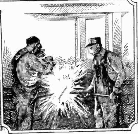
Workmen welding with electric torches must wear goggles to prevent blindness because of the ultra-violet rays produced during the work.
