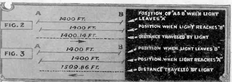
Figs. 2 and 3 show how the earth's motion carries the mirrors through the ether while light travels between A and B, making one beam actually travel further than the other. The time interval of 3 ten billionths of a second is measured by the interferometer method.
