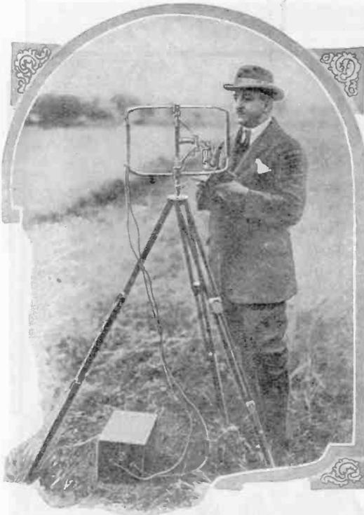
The device illustrated at the left is the latest invention of a German engineer, E. Wolde-mar Pastor. Recent dispatches claim that this mechanism, operating on an electrical principle, can locate underground veins of gold-bearing ore.
