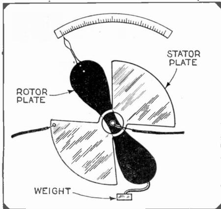
An electrostatic voltmeter may easily be made by using thin variable condenser plates. It must be calibrated from a standard meter.
