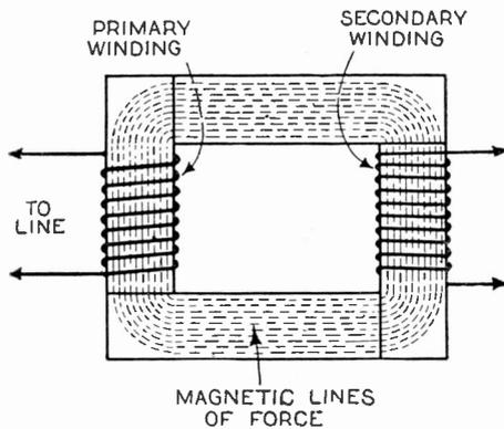
This cut shows the lines of force present in the iron core of a transformer.
