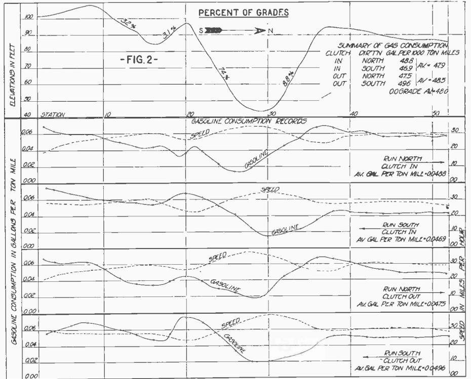
The five charts directly above in Fig. 2 give the results of a series of tests over a measured course. The terms "clutch in" and "clutch out" refer to the fact that when descending hills, the clutch was either engaged or released according to the respective terms used. These charts make an interesting study to anyone interested in automobiles.
