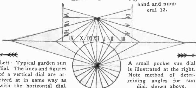
A small pocket sun dial is illustrated at the right. Note method of determining angles for sun dial, shown above.
