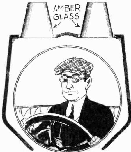
No. 1,511,357, issued to Eldridge Nairne covers the design of automobile goggles shown. By tilting the head, sun or approaching headlight glare can be eliminated.
