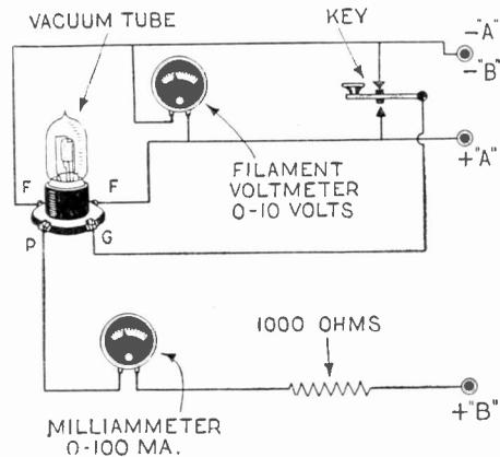
When buying tubes be sure that they come up to the highest possible standard. In order to ascertain this, construct a vacuum tube tester as shown above.
