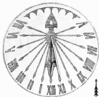
A sun dial may be regarded as the edge of the disk which passes through the center of the earth from the spot where the dial is fixed. To divide the dial, we imagine it surrounded by a cage formed of twenty-four arcs drawn from the North Pole to the South Pole. In its course the sun would cross one of them every hour.
