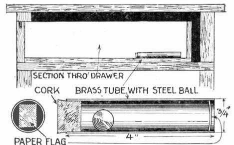
To find out if anyone has opened a drawer during one's absence, make the little device shown above, closing one end of the tube with a small paper strip. If the drawer has been opened, the paper will be found out of the tube.
