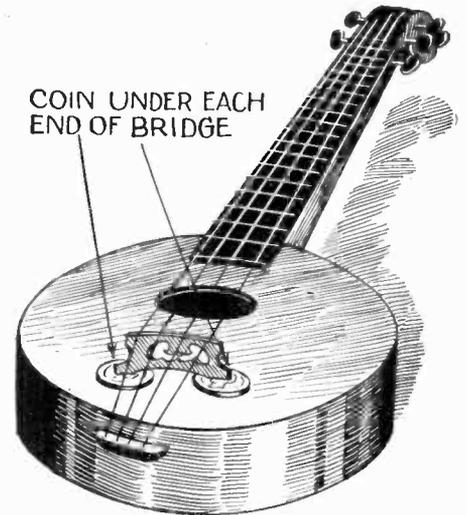
If two coins are placed in the positions shown in the illustration above, the tone given out by the instrument when played will be found to be of a far better quality than before the addition. Not only will the tone be richer, but if large coins such as half dollars are used, the chords will be much softer.—F. Cariveau.
