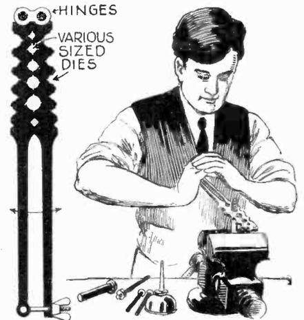
No. 1,521,647, issued to Edwin M. Perry describes the device illustrated above with which damaged threads on bolts and nuts may be quickly re-formed.
