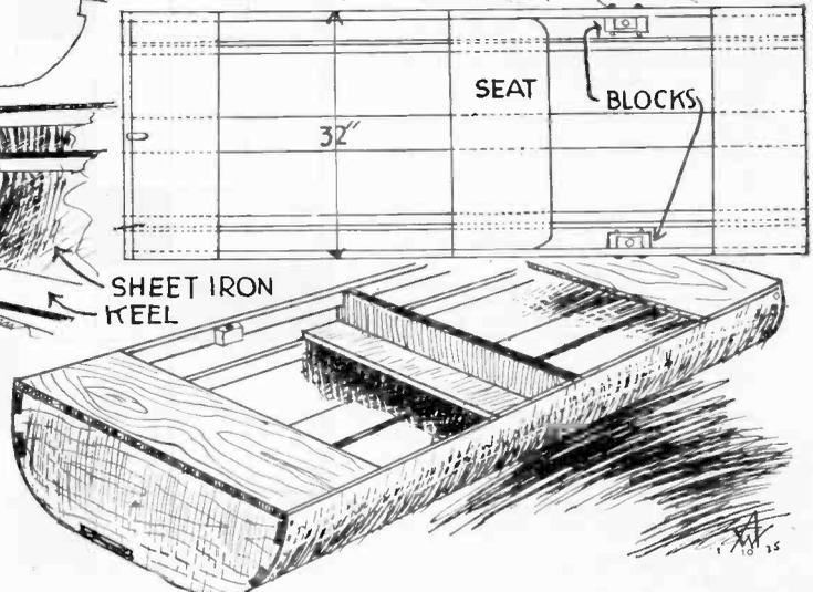
In the construction of this boat, first cut three forms from one inch cypress for the end and center blocks. Place two about ten feet apart with the third in the center, and fasten the keel in place with wood screws. Then fasten the gunwale and bilge strips as shown, taking care that the surfaces of all the strips come flush with the edges of the forms. The outside covering of this boat consists of a single sheet of light gauge galvanized iron ten feet long and somewhat over four
