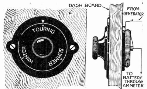
A regulator for automobile storage batteries, to prevent overcharging.
