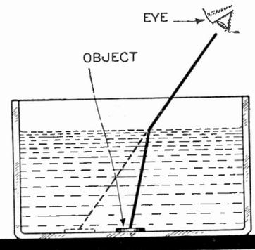
The above shows the effect of refraction of light through water.
