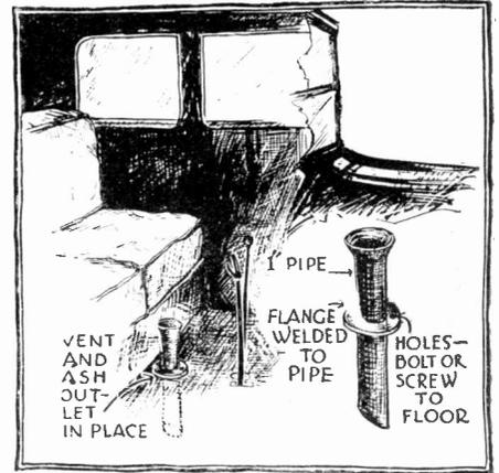
A combination ventilator and ash receptacle for the closed car may be quickly made from pipe fittings as shown above. A 1 inch or larger pipe is flared out at one end and a flange welded to it as shown. The lower end of the pipe is cut off at an angle. Mounted in the floor board as shown, this accessory is very handy as an ash tray and also serves as a ventilator.
