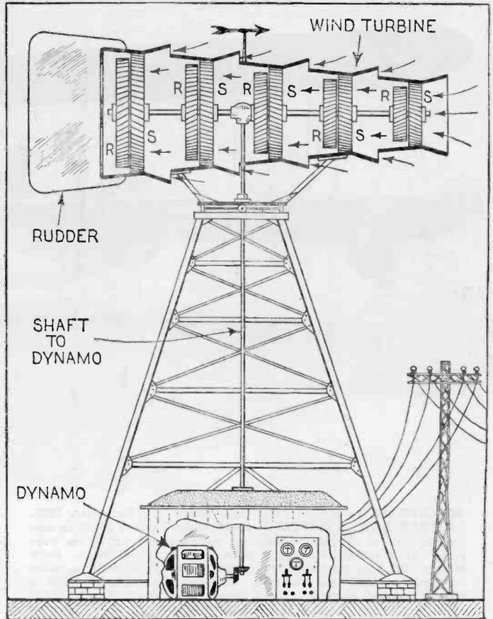
A novel wind turbine of French origin has recently been developed. The device is illustrated in detail above. The drawing at the left shows the power plant in actual operation under working conditions, and the one at the right shows a complete cross section of the working parts and detail thereof. Wind enters the front, is concentrated through a cone shaped
