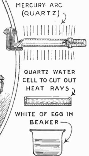
Eggs may be "boiled" without heat by using a quartz lamp and a quartz water cell to cut off the heat. The white of the egg will be found to coagulate quickly.
