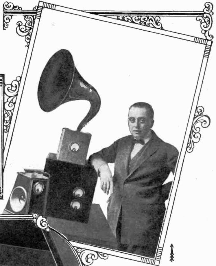
The above photo shows the assembly of parts used in the super radio system. To the extreme left is shown the battery compartments. Next to the right is shown the reproducer cabinet in which is contained the controlling clock-work and reproducer arm. Above this cabinet is the loud speaker and its auxiliary amplifier.
