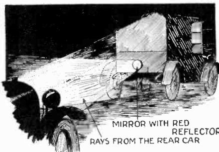
In case your tail light should go out, you need not be afraid of a rear-end collision if your car is equipped with a red-backed mirror as shown above. Approaching headlights will be reflected toward the driver of the coming car, thereby warning him.—Martin B. Beline.
