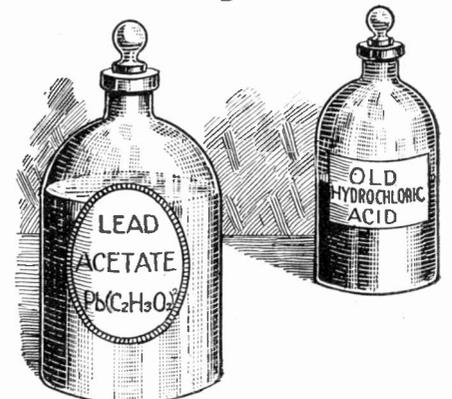
When reagent bottles have been allowed to stand, they are often hard to clean. However, if some old waste hydrochloric acid is placed in the bottle and rolled around the sides it will quickly dissolve the deposit. The bottle is then washed as usual.
