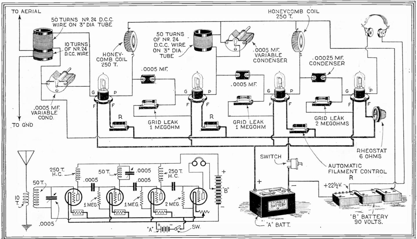
The above diagram shows what is called the T.A.T. system. It is used very much in England because it does not oscillate. The reason for this is that an aperiodic circuit is placed between two tuned ones. By following the diagram an efficient and unusual set can be constructed.
