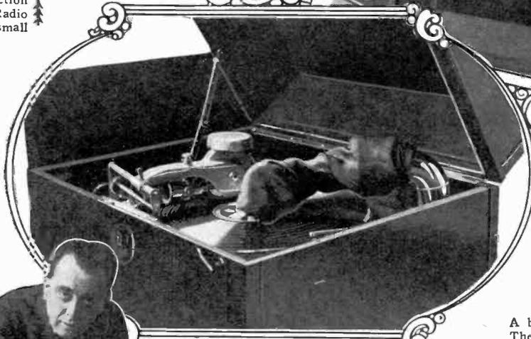
The queer looking tone arm to the extreme left in the above diagram is a brake regulator placed at the rim of the record carrier, which causes the disk to pass under the stylus at a constant speed. According to a new arrangement the clock work is allowed to run unchecked.
