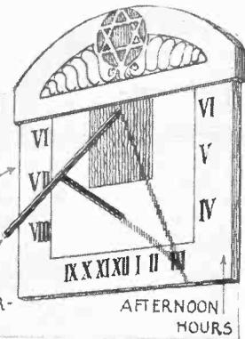
The style of a sun dial should be parallel to the earth's axis and should point to the polar star.
