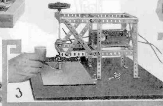
As may be seen by the photos to the left and below, the stands for the grinding and drilling apparatus are made from "Erector" parts. The arrangement shown in Fig. 4 is used to roughen the edges of the glass so that the cement can hold better. An emery wheel is used for this grinding process.
