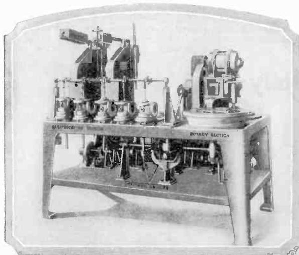
Above is shown the complete machine, three sections of which are illustrated on this page. Each section of machinery on this table is in reality a separate and individual machine. With a layout of this nature, a shop is equipped for doing practically all of the fine work necessary in accurately fitting air brake parts.
