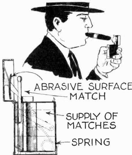
No. 1,513,091, issued to A. Y. S. Album protects match box design illustrated above. When the cover is released and opened by the spring, a match is forced up into the position shown and at the same time is lighted.
