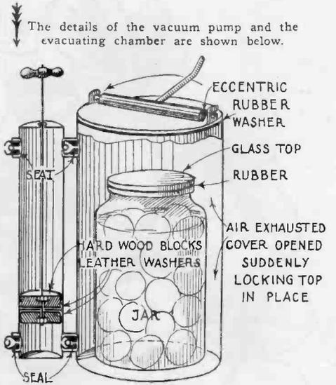
A new device of great assistance to the housewife has recently been invented by A. C. Whitefield and is illustrated in detail above. In use, the foods to be preserved are placed in a standard glass jar, the rubber ring and the glass cover put into position and the cover of the vacuum tank clamped on. A few strokes of the pump serves to create a vacuum of
