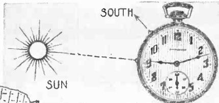
Left, we see a pocket sun dial which is accurate to within a few minutes. Above is the method for using your watch as a compass. Hold watch flat with face upward, point hour hand toward the sun; then south is half way between hour hand and numeral 12.
