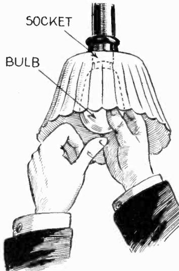
A simple and safe method of taking out and putting electric light bulbs into sockets is illustrated above. Rest the glass tip of the bulb on the thumb and screw the bulb in with the other hand. The thumb prevents the bulb from falling.—Sidney Lang.
