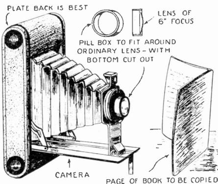
A lens of 6 inch focal length mounted in a pill box and placed over the lens of an ordinary hand camera enables the operator to use the same for copying work. It is best to focus on a ground glass as otherwise it will be necessary to experiment for the correct position.
