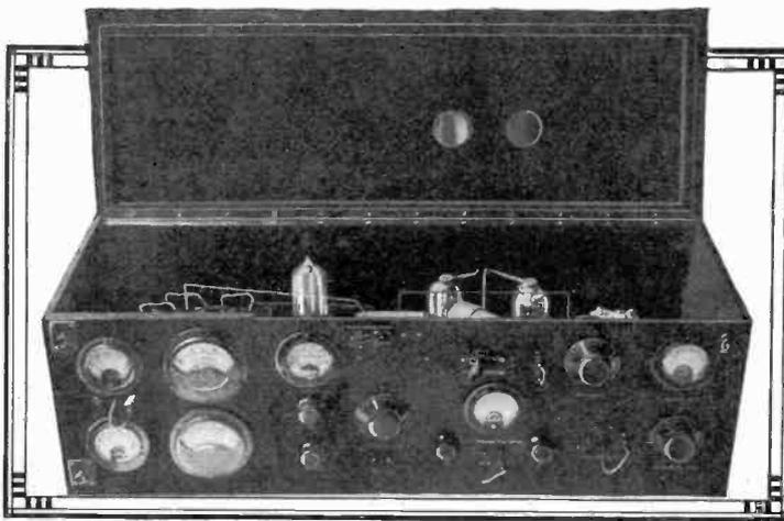
The above photo shows the amplifier used in connection with the Hausdorff Super Radio System, to amplify the small currents coming from the solenoid coil in the reproducing cabinet of the phonograph. The tubes used in the amplification process are of special design. As yet, the circuit is not available.
