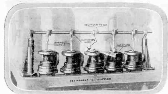
The section at the left illustrates the reciprocating section for refining internal seats for slide valves. This device is so made and arranged that at any time during the work a slight upward pull on the supporting arms enables the operator to remove the lap-sticks, remove them so as to inspect the valve, and determine how the work is progressing.
