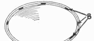
"A" OUTER ROTATING "DISH" WITH MAGNETS "B" TO PULL THE IRON MERCURY PAN FLOATING IN OIL IN "A"
