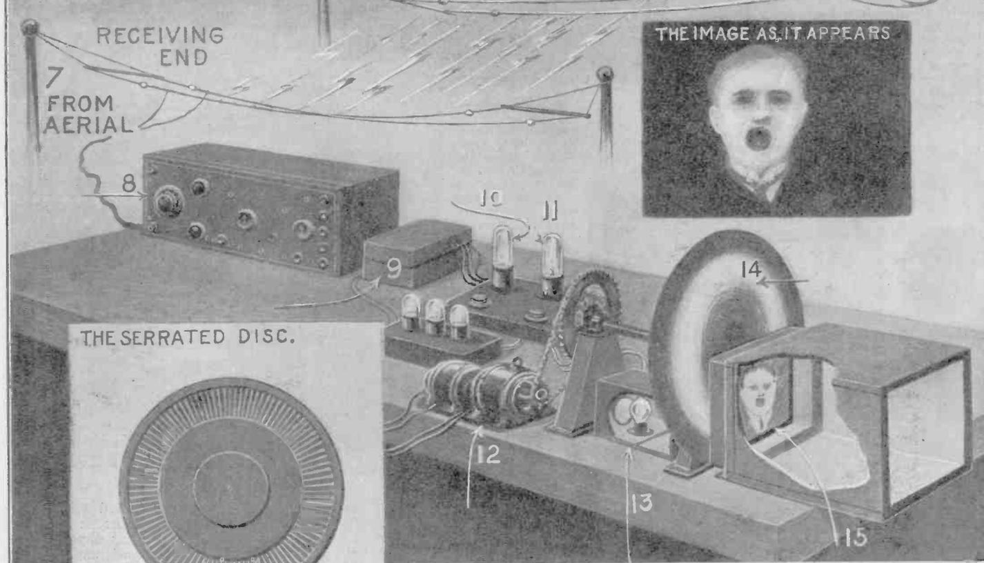
Synchronous motors, 4 and 12, keep the apparatus in time. The radio waves are received on a usual receiving set, 8, and pass through a filter, 9. The picture current is then amplified by, 10 and 11, whereupon it lights the lamp, 13. The brilliancy of this lamp depends upon the shadows and high lights of the object in front of the transmitter. This light passes through lens disk, 14, and registers on ground glass, 15. The inventor has succeeded in transmitting the illustration shown.
