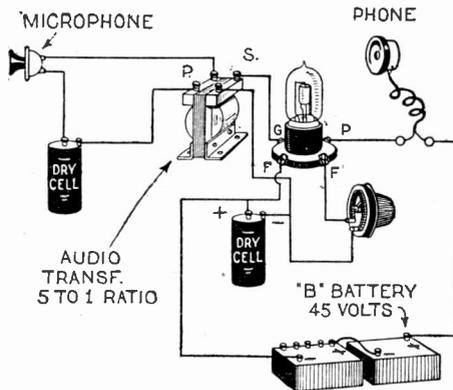
This diagram shows the use of a vacuum tube amplifier for aid to deaf people. The batteries may be made very small so that they may fit readily into the pocket.
