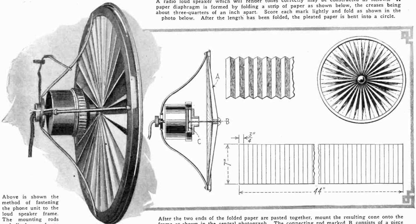
Above is shown the method of fastening the phone unit to the loud speaker frame. The mounting rods and diaphragm frame must be made of rigid construction.
