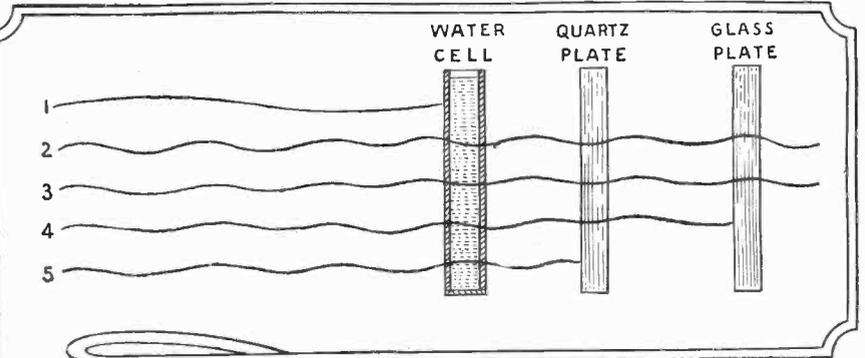
The above diagram shows the relative lengths of light waves and common substances which are transparent or opaque to them. 1—Infra red, relative length of wave 9; 2—red, length 6; 3—blue, length 4.5; 4—long ultra violet, length 3; 5—short ultra violet, relative length 2.
