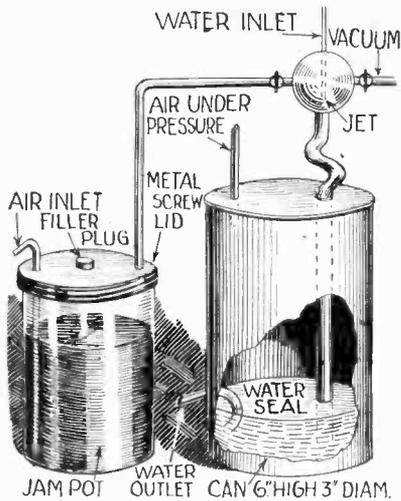
The apparatus illustrated above is to operate by water pressure from the mains and will serve several purposes in the experimenter's laboratory. With water flowing through the jet and the left hand cock closed, a vacuum is created or compressed air is obtained at the points shown. Close the right and open the left cock and vapor can be obtained from any liquid contained in the small jar.—Don Pedder.
