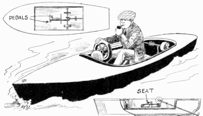
No. 1,522,390, issued to Charles Sanders describes a boat to be propelled by the feet of the occupant as shown in the illustration above. Pedals transmit the power to the propeller.
