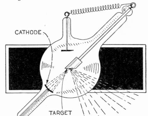
The above shows a common form of X-ray tube. The target may be of platinum, and the cathode of aluminum.
