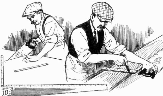
No. 1,514,180, issued to William A. Spittler protects the design of a saw, the back of which is scaled off as shown and carries a lug to which an arm may be attached at right-angles as a square.
