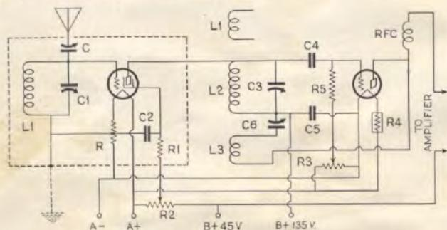
Figure 4—Suggested shielded arrangement for a 222 RF stage using a tuned input circuit. Potentiometers permit control of the screen grid potential and the voltage on the grid return.
