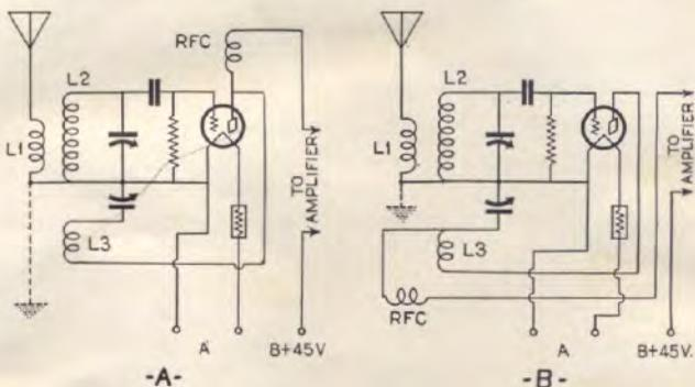
B and A of Figure 6. In these circuits a fixed tickler is used and regeneration is controlled through a small variable condenser. Circuit A, Figure
