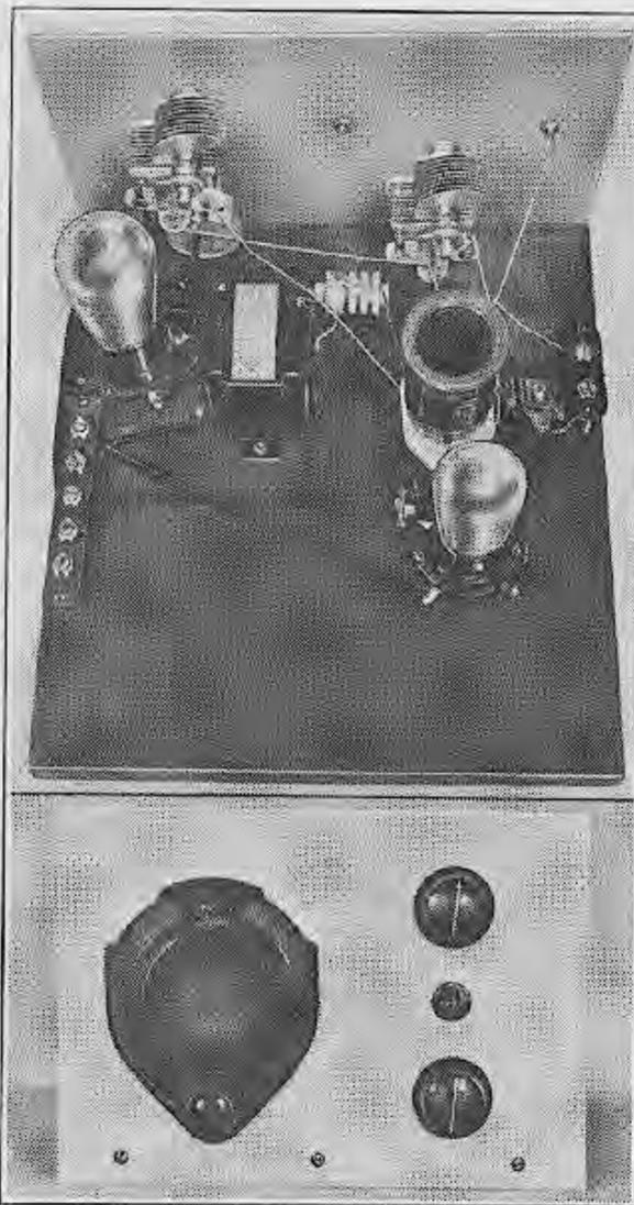
plate supply either 90 volts or 135 volts of B battery may be employed, but the higher value is recommended if maximum audio amplification is desired.
