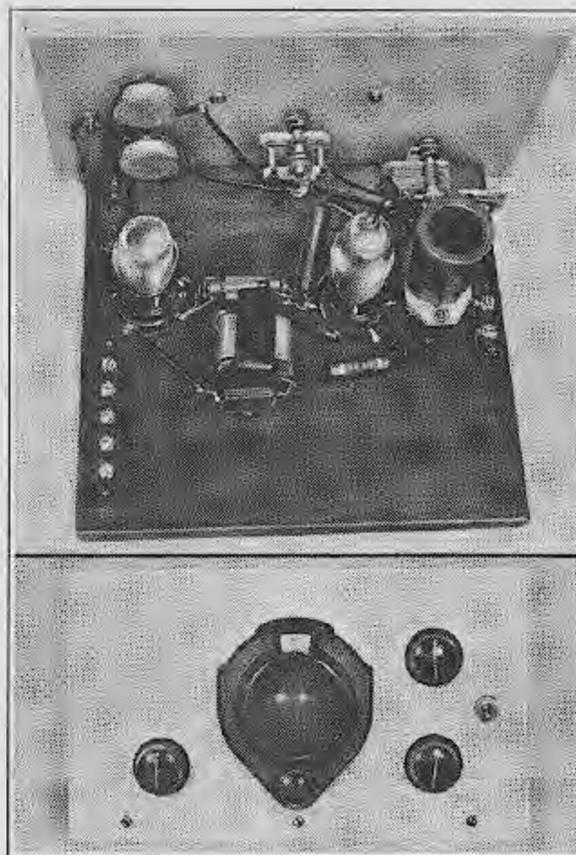
ing regeneration in the plate circuit, controlled by varying the screen-grid voltage of the 6D6 detector for which purpose the potentiometer R2 is employed.
