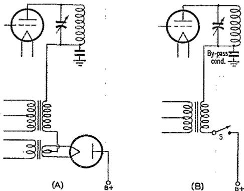
Fig. 2—The new type of high-level negative-peak clipper moves the clipper tube to the other side of the modulation-transformer secondary, as shown at A. This has the action of a switch at  $S$  in B. In combination with the clipper-tube filament transformer, the inductance of the modulation-transformer secondary and the plate by-pass condenser, a low-pass filter is formed, and no sharp negative square waves reach the modulated stage. (See Fig. 3.)
