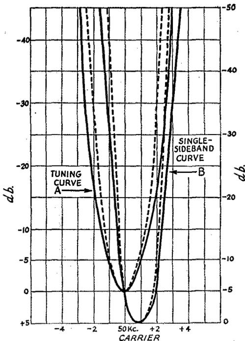
Fig. 3 — Tuning and single-sideband curves of the 50-kc. amplifier in the s.s.s.r. adapter unit. The solid curves show the performance with the 1898-A transformers and the dashed curves the performance with 1898-AX transformers.
