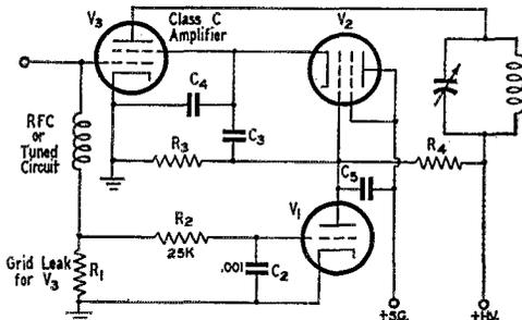
Fig. 1 — Protective circuit for screen-grid tubes when a separate screen supply is used. The "clammer-tube" idea is applied through a series tube to reduce screen voltage automatically whenever excitation or plate voltage is removed.
