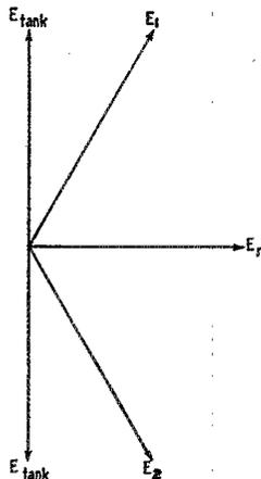
Fig. 2 — A vector diagram of the voltages on the r.f. grids of the balanced-modulator tubes, showing how resultant output is obtained. Under modulation,  $E_1$  increases and  $E_2$  decreases (or vice versa), resulting in a phase shift of  $E_r$ , the resultant appearing in the plate circuit.
