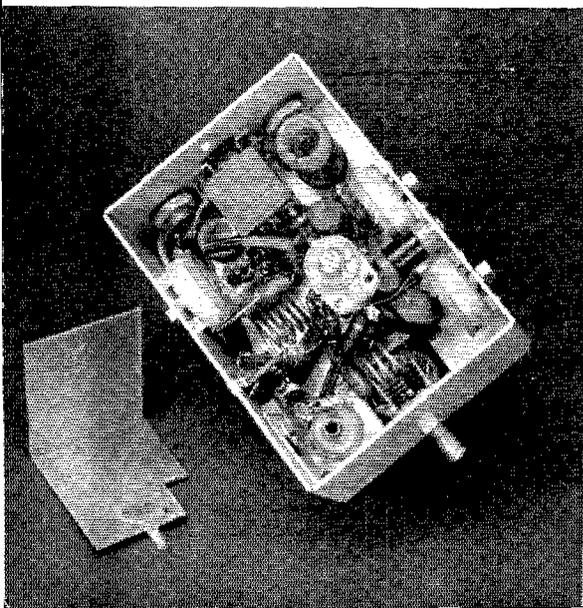
A bottom view of the 144-Mc. converter, showing the small bracket for mounting the regulator-tube socket, located at the lower left-hand corner of the chassis.  $C_2$  is mounted with the adjustment screw facing the observer. The copper shield to the left of the photograph isolates the low-frequency oscillator and prevents "birdies."
