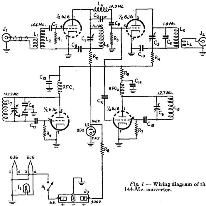
Fig. 1 — Wiring diagram of the 144-Mc. converter.
