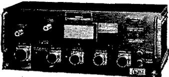
This brand new army surplus transceiver contains practically all of the elements you need to get going on VHF. Freq. 418-462 mcs; FM; a 14-tube job furnished complete with 3 12SJ7's, 4 12SH7's, 2 12H6's, 1 VR150, 2 955's, 2 9004's and 27V dynamotor. Shock mounting supplied. Weighs only 25 lbs. Furnished complete with tubes and dynamotor, less accessories, in original manufacturer's carton 8 7/8" x 7 7/8" x 18 1/2". Price, each.....\$11.95
