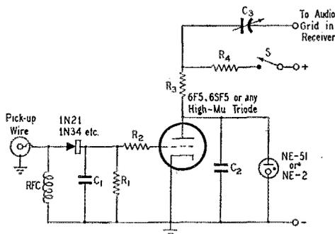
Fig. 2 — An alternative circuit for the keying monitor.  $C_1$  is 470  $\mu$ fd.; otherwise the values are the same as in Fig. 1.
