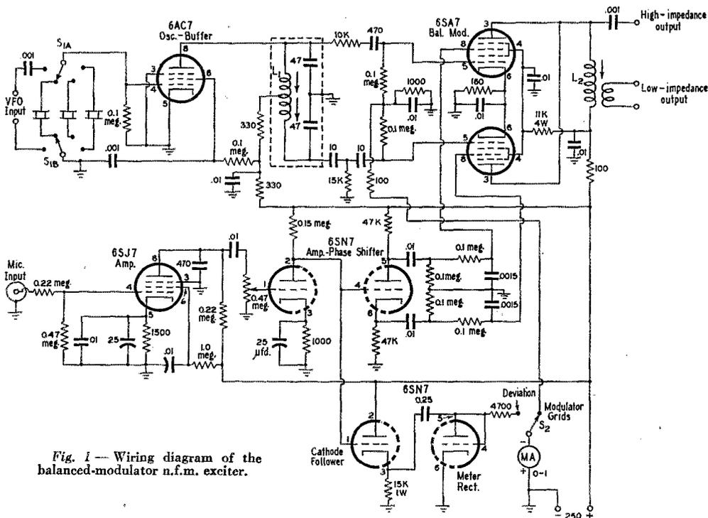
Fig. 1—Wiring diagram of the balanced-modulator n.f.m. exciter.
