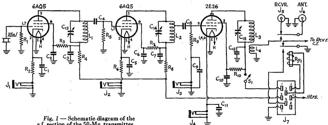
Fig. 1 — Schematic diagram of the r.f. section of the 50-Mc. transmitter.
