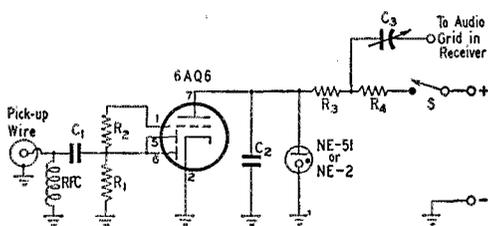
Fig. 1 — Circuit of the automatic keying monitor.
