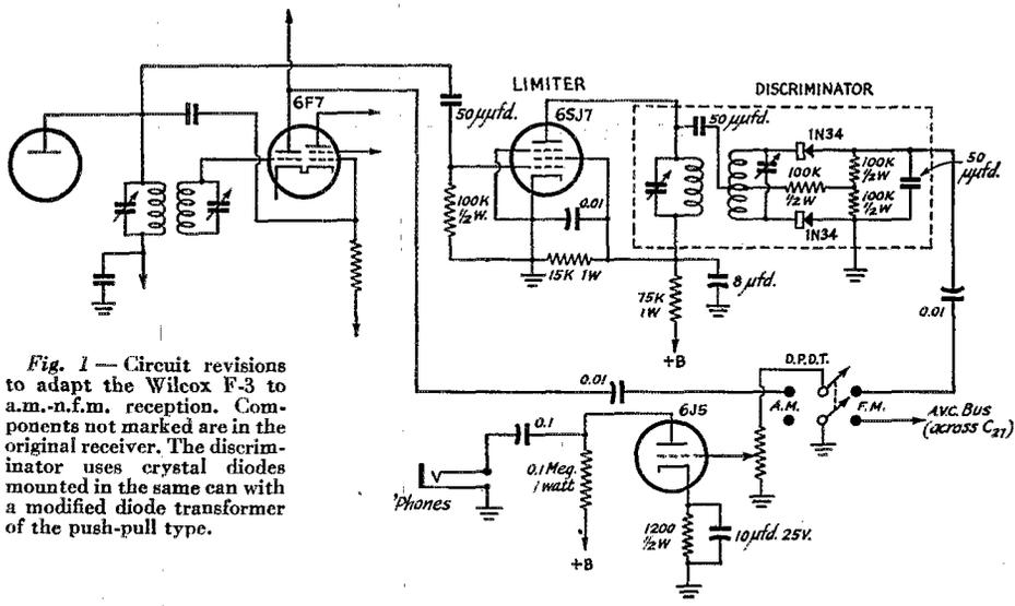
Fig. 1 — Circuit revisions to adapt the Wilcox F-3 to a.m.-n.f.m. reception. Components not marked are in the original receiver. The discriminator uses crystal diodes mounted in the same can with a modified diode transformer of the push-pull type.
