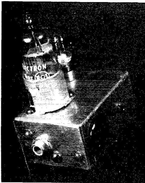
The simple keying monitor can be built so small that it will fit into any receiver. The Jones fitting below the 6AQ6 tube takes the r.f. pick-up line.
