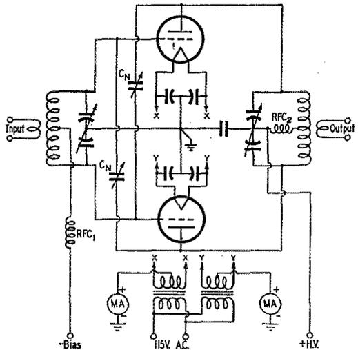
Fig. 1 — Typical neutralized push-pull triode amplifier circuit.
