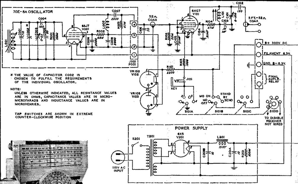
\* THE VALUE OF CAPACITOR C002 IS CHOSEN TO FULFILL THE REQUIREMENTS OF THE INDIVIDUAL OSCILLATOR.
