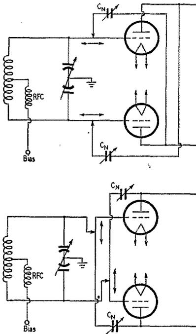
Fig. 2 — Showing how the taps are made to maintain effective neutralization over a wide range of frequencies.
