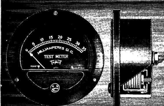
Full size of instrument. Note deep shroud for glass protection and "Quick-Look" Scale.
