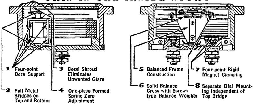
Thin-Line Instruments also have Standard Large Coil Triplet Movements. Furnished with Osmium pivots for special requirements. All these features make for greater rigidity under vibration; greater permanence of calibration; greater user satisfaction.
