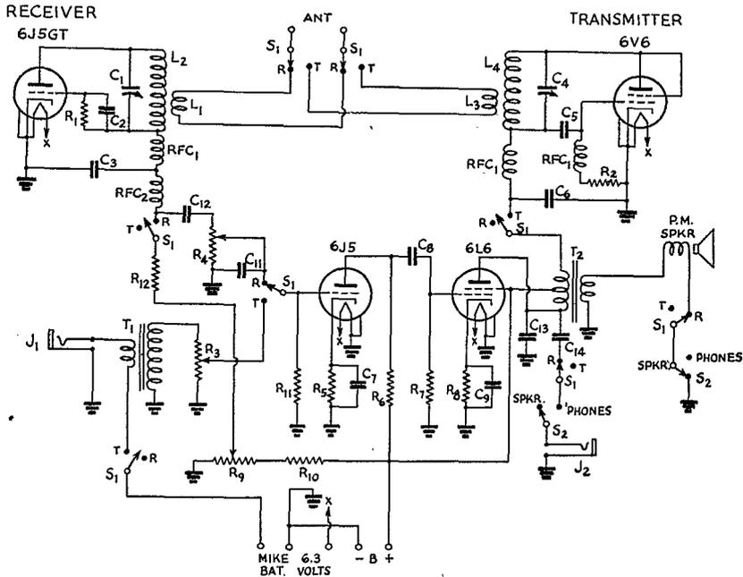
Fig. 1 — Circuit diagram of the 2½-meter transmitter-receiver.
