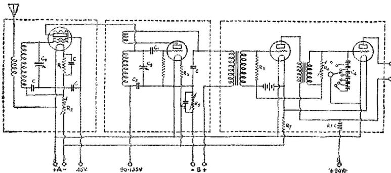
FIGURE 3. THE COMPLETE WIRING DIAGRAM OF THE RECEIVER
