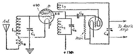
FIGURE 1. THE SCHEMATIC DIAGRAM OF THE R.F. AMPLIFIER STAGE AND THE DETECTOR
