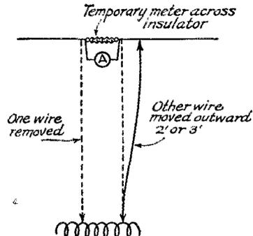
FIG. 5. A METHOD OF FINDING THE WAVELENGTH OF THE ANTENNA TOP
