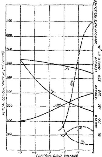
UX 222 EFFECT OF CONTROL GRID BIAS ON  $G_m$ ,  $\mu$  AND  $1/\mu$  FOR BOTH SHIELD-GRID AND SPACE-CHARGE METHODS OF OPERATION, THE CONTROL GRID IN EACH CASE BEING THE ONE APPROPRIATE FOR THE METHOD.
