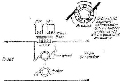
brushes make contact on the commutator, which has every third segment connected together. The brushes are adjusted to make contact to any two of the segments that are connected. This would, when the motor was running, give us an interrupted circuit with a frequency of about 360 interruptions per second.
