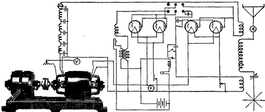
Item 37, 2 unit four bearing set, delivering 1000 volts, 600 watts for plate and 12 volts, 300 watts for filament. The "ESCO" Set is shown here furnishing Power Supply for 4-50 watters in a phone or telegraph set. This is the Item used by CB8 in pioneer achievement of the first two way amateur wireless communication between North and South America.
