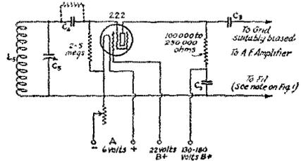
FIGURE 2. THE SPACE-CHARGE-GRID METHOD OF USING THE TUBE AS A DETECTOR
