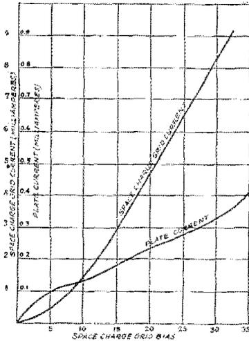
UX 222 SPACE-CHARGE CONNECTION. EFFECT OF INNER (SPACE CHARGE) WHEN PLATE VOLTAGE = +135. OUTER (CONTROL) GRID VOLTAGE = -1.5
