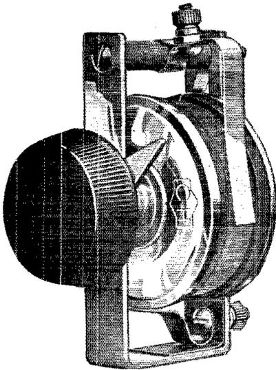
This potentiometer is of the revolving drum type and the resistance unit has a resistance of 300 ohms. The resistance wire is clamped between two insulated caps which hold the wire firmly in a horizontal position. The broad, flat contact on the tightly clamped resistance unit insures that the wire will not be damaged or displaced under constant usage. The instrument is designed for panel mounting and is provided with three binding posts to facilitate wiring.
