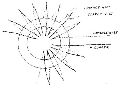
care that the junctions do not touch each other. The inner circle of junctions may now be heated by placing over a gas burner or an electric heating element, or, if you live near the North Pole, you can cool the outer junctions instead. The two terminal wires may now be connected across the filament of the receiving tube, and as long as the heat (or cold) is steadily applied, the direct current produced will light the tube nicely. Q. E. D.
