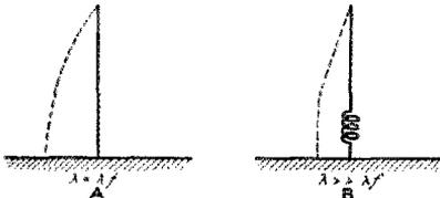
FIG. 4. Current distribution in an antenna, A—when oscillating at fundamental (sinusoidal), B—when considerably above the fundamental (linear).
