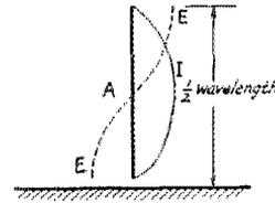
FIG. 3 ANTENNA WITHOUT EARTH CONNECTION
