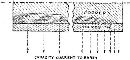
FIG. 3 LONGITUDINAL AND RADIAL FLOW OF CURRENT IN A CORRODED ANTENNA WIRE
