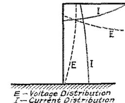
FIG. 2—ANTENNA WITH A TOP
