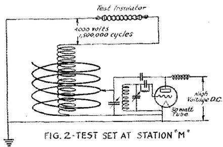
FIG. 2-TEST SET AT STATION "M"
