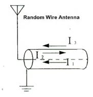
Figure 1. The outer conductor of a coaxial cable can carry high frequency currents flowing in opposite directions at the same time.
