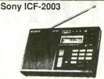
The ICF-2003 covers 153 - 29995 KHz and FM. A BPO is provided for SSB and CW. Advanced features include: LCD digital readous, keypad entry, ice memories, scan, 12-24 hour clock-timer, LED tuning meter and tone switch. With earphone, carry case, battery case, AN-6 wind-up antenna and SW guide. Requires six AA cells (not supplied).
