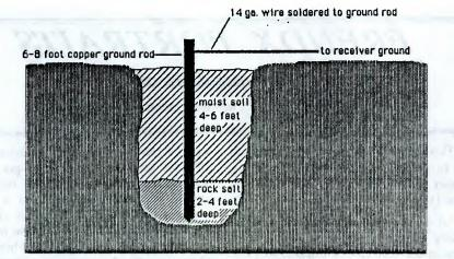
Figure 1. Suggested Ground Rod Installation
