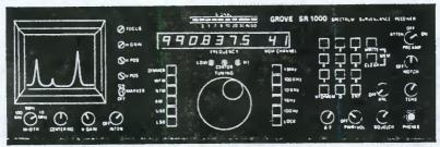
The American-made SR1000 is a virtual monitoring laboratory. A built-in CRT lets you visually scan 10 MHz, 1 MHz or 100 kHz segments of the spectrum from 100 kHz to 1000 MHz-with no gaps. When an interesting signal appears, you can zero in to intercept AM, narrow and wide FM, and SSB signals.
