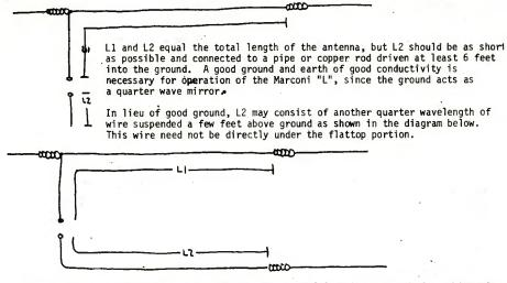
Ideally to cover the international SWBC bands, a total length of L1 and L2 need be only 39 feet. 48 feet and 8 inches would cover the 60 metre band. Length is calculated by the formula L(feet)=234/f(MHz). This is also the formula used to compute the length of the vertical. This type of antenna, like the vertical, is omnidirectional, and noisier than other horizontal antennas.
