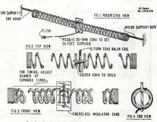
Drawing showing details of the SLINKY Dipole Antenna
