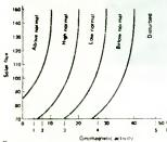
Fig. 1 - Interaction of given values of solar flux and geomagnetic activity determine expected h.f. ionspheric propagation conditions. (Example: S.F.=80, Ap=25 expect BELOW NORMAL conditions.) From mid-1974 to mid-1976, conditions recurred 27 days later exactly as defined in the above categories 63% of the time, and within an accuracy of one category 82% of the time (counting differences between LOW and BELOW NORMAL as a miss.)
