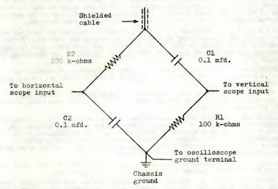
Each pair of components must have identical electronic values and fairly low tolerances; 5% resistors and 10% capacitors are satisfactory. To avoid component breakdown, resistors should be rated at not less than two watts and capacitors at a minimum of 300 WVDC.
