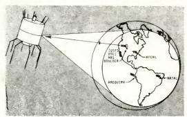
During a two-year experiment, the National Bureau of Standards Lab in Boulder, Colorado relayed, via NASA's ATS-3 geostationary satellite, strong and stable time and frequency signals covering forty percent of the earth.
