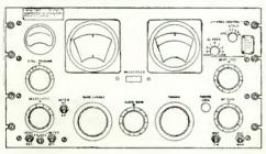
The Hammarlund SP-600 is built like the proverbial Patton tank. The power transformer alone weighs 25 lbs. The military assigns special numbers of their own to receivers built for them. In case of the SP-600, of which there were several variations, all had different numbers. My model was the R-274C. Older SP-600's before 1950 were called "Super Pro."
