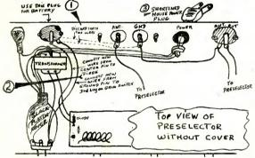
For handy battery access to the circuit from the outside, I disconnected the phene plug antenna input from the inside and added a couple new pieces of wire so that the center of the plug could be wired to the circuit beard side of the diode, and the ground side of the plug could be wired to the third gain switch lug (which also has a wire from the transformer on it.)
