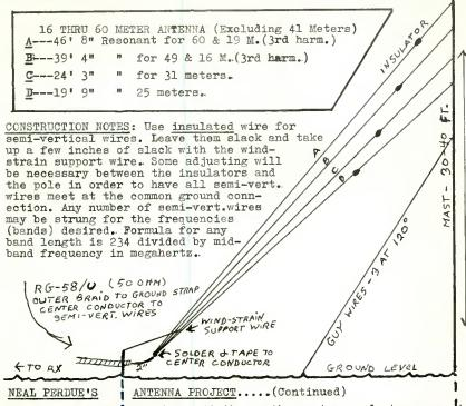
to all the ante Inna wires. At the rx the center conductor goes the antenna ter minal and the braided shield goes to the grou terminal. You n ow have resonant semi-vert ground plane dipol md es for the frequen cies for which you have cut the wire.
