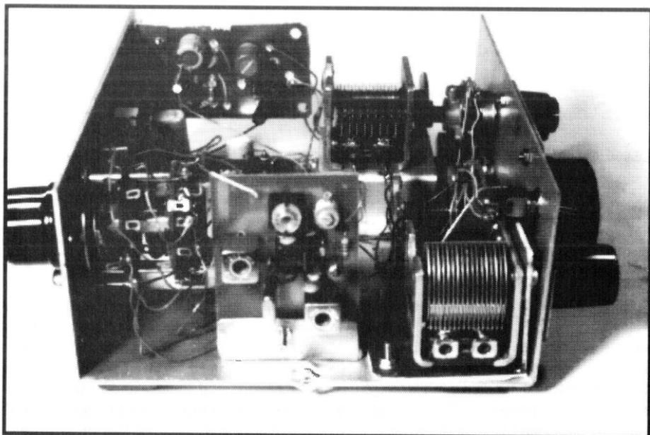
*Interior of the Four-Bander. The receive converters are mounted upright to save space.*
