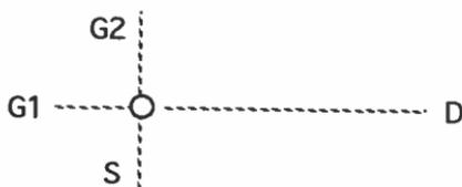
Spec is:  $V_{ds} = 20V$ ,  $I_{dss} = 4-25mA$ ,  $-V(p)g1-s = 2.5V$  max,  $y_{fs} = 14mA/V$  typ., Noise Figure = 1.0dB and Gain Product = 26dB at 200MHz,  $C_{rs} = 25pF$  typ.
