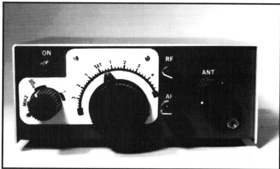
*Due to the use of existing variable capacitors and a mounting flange in the "junque" box, the front panel ended up squished to the left, leaving the bandspread tuning (large knob) a tad bit constricted. Not bad enough to change, however.*
