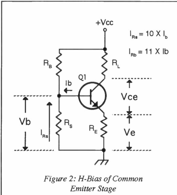
Figure 2: H-Bias of Common Emitter Stage
