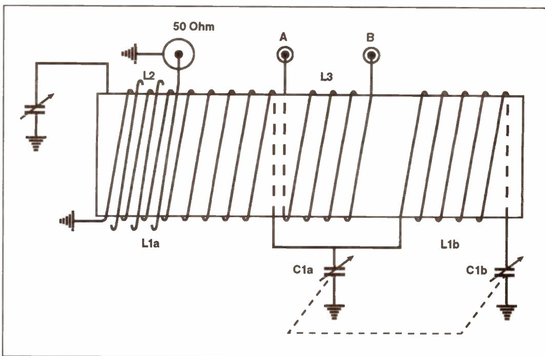
L1a, and L3 five turns of insulated wire close wound between L1a and L1b.
