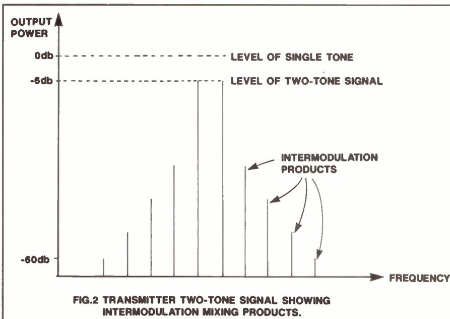
In the lab, a note is taken of the levels of these IMD products relative to either the PEP level, or the level of one of the tones. It doesn't really matter which is used, but it's important to check that the figures you see on the specification sheet refer to what reference is taken. Impressive-looking transmitter specifications on nice glossy sheets such as '-36dB 3rd order IMD'
