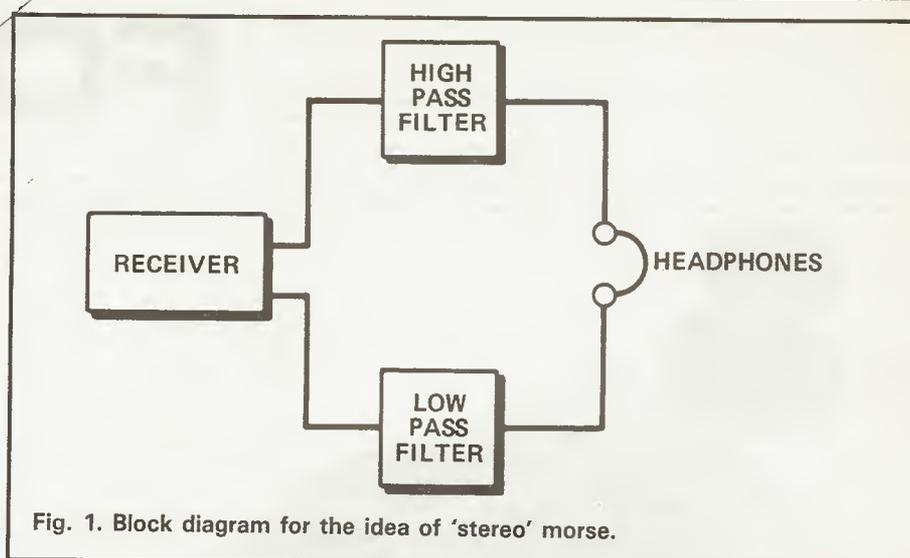
Fig. 1. Block diagram for the idea of 'stereo' morse.
