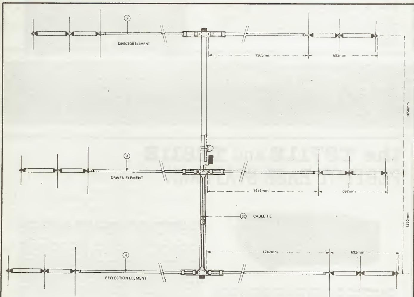
Fig. 1 Construction of the MM3 Minimax aerial — viewed from below.
