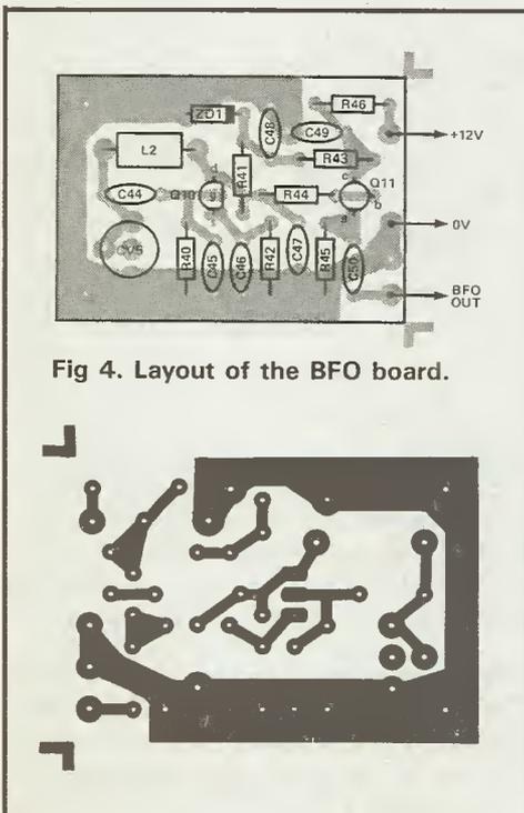
Fig 4. Layout of the BFO board.
