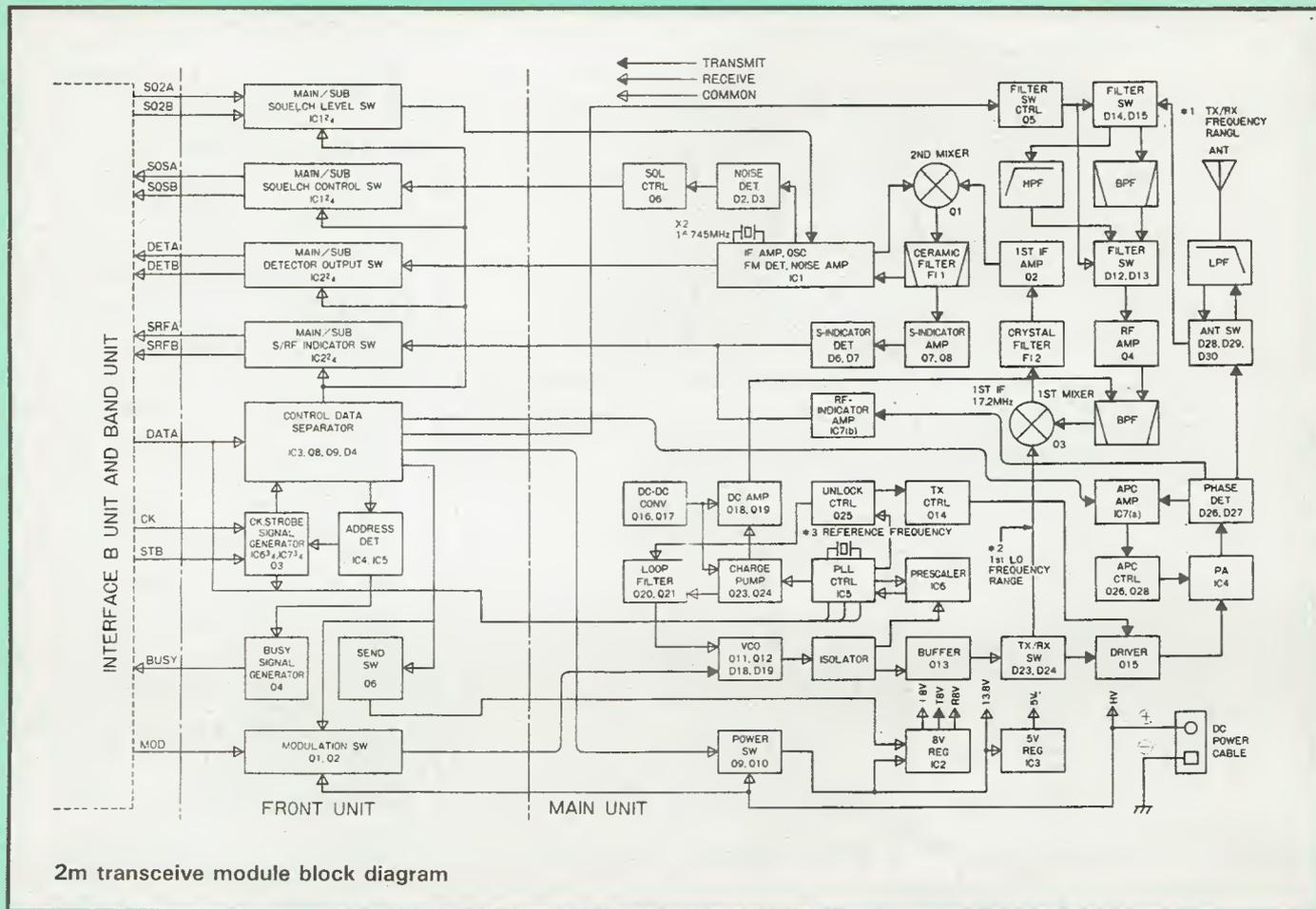
2m transceive module block diagram
