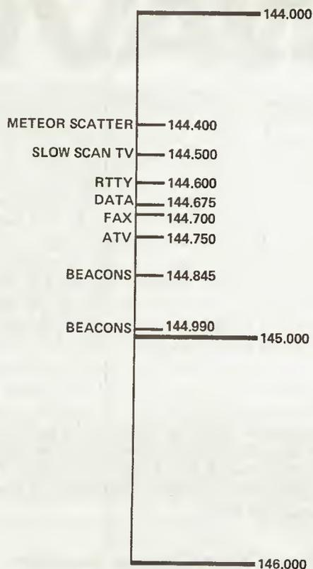
Fig. 1 The chart shows the amount of frequency area below 145MHz available for FM communication. FM should never be used above 144.845MHz as it may blot out weak signals from distant beacons. If used below 144.5MHz this should be done circumspectly because (a) the 'all mode' section stops here and (b) SSB may be present.
