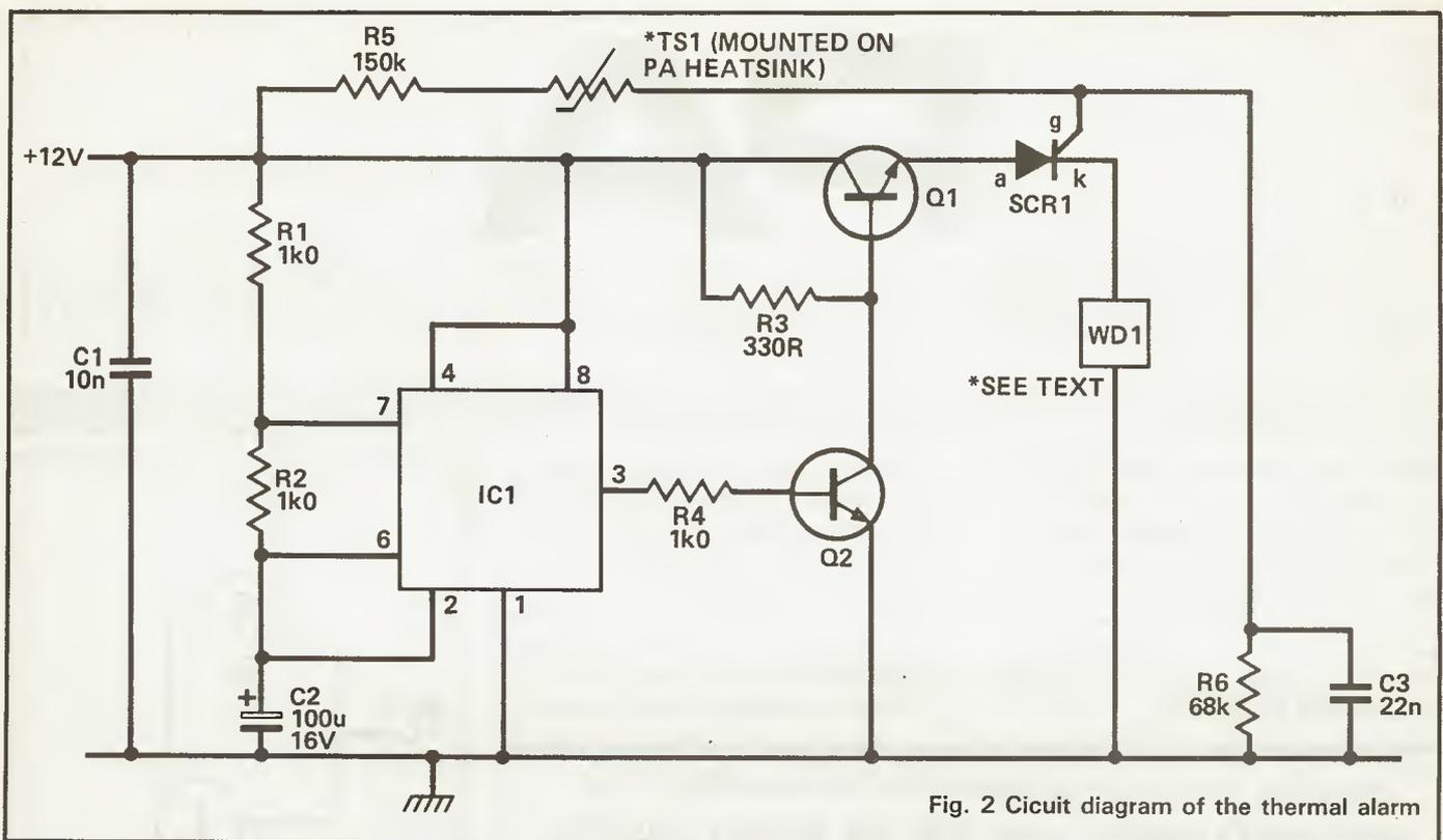
Fig. 2 Circuit diagram of the thermal alarm
