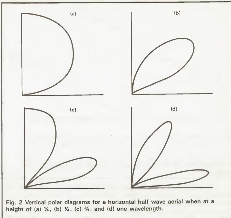
Fig. 2 Vertical polar diagrams for a horizontal half wave aerial when at a height of (a)  $\frac{1}{4}$ , (b)  $\frac{1}{2}$ , (c)  $\frac{3}{4}$ , and (d) one wavelength.
