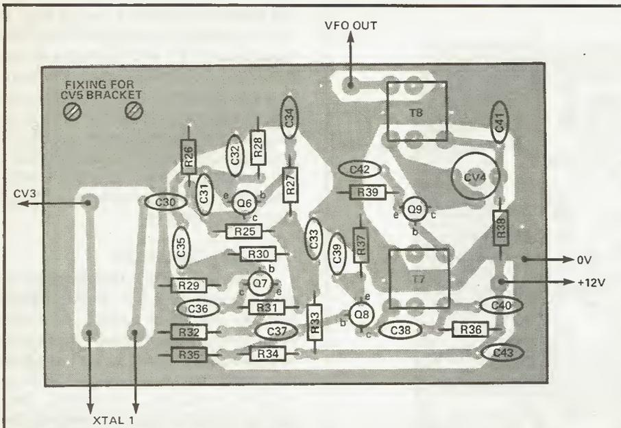
Fig 3. Layout of the VFO board.
