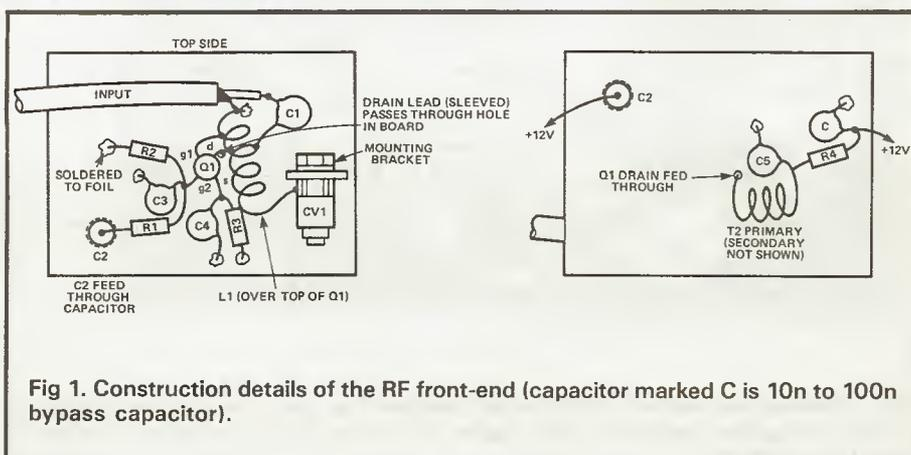
Fig 1. Construction details of the RF front-end (capacitor marked C is 10n to 100n bypass capacitor).
