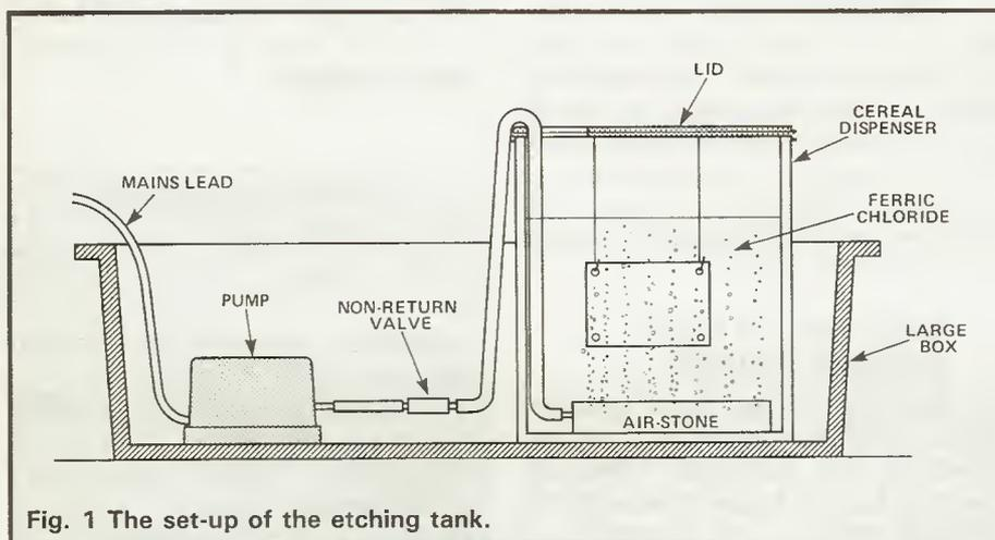
Fig. 1 The set-up of the etching tank.
