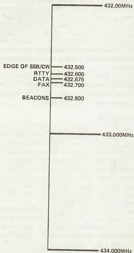
Fig. 2 In the 'all modes' section of 70cm no less than 300kHz are available for FM QSY. Never QSY into the beacon segment above 432.8MHz and avoid the three specialist spot frequencies shown.
