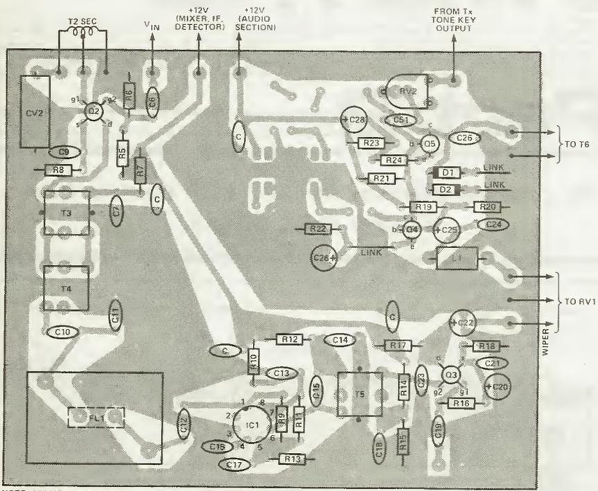
Fig 2. Layout for the main PCB and foil pattern. The capacitors marked simply C are decoupling capacitors, with values of 10n to 100n, depending on what you have to hand.
