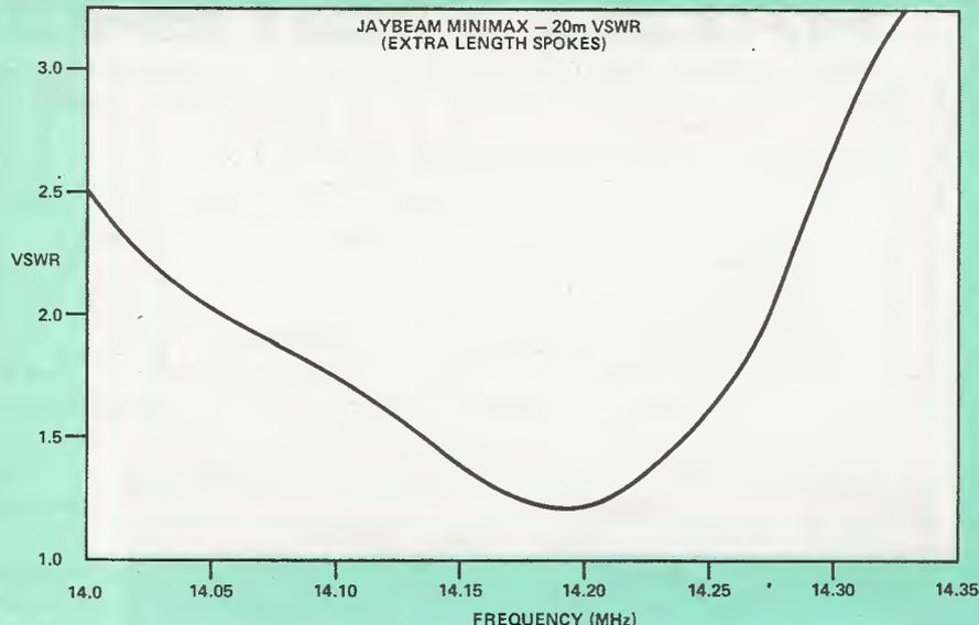
duction of the LF end VSWR. This does show that the mounting location certainly has an effect on the beam.
