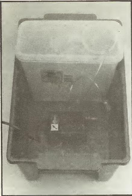
the area to be etched and the temperature of the solution. During etching, remove the board every two minutes or so to monitor progress. As soon as all the exposed copper has been etched away, stop the pump and remove the board. It should then be thoroughly rinsed before cleaning off the etch resist and drilling.
