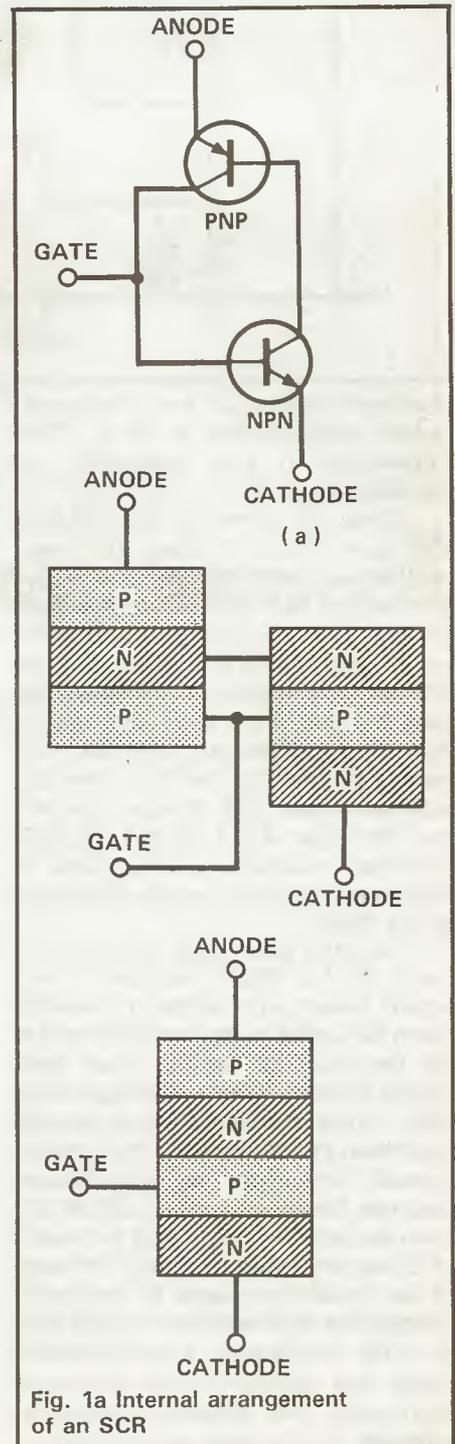
Fig. 1b Detail on an SCR PNPN construction
