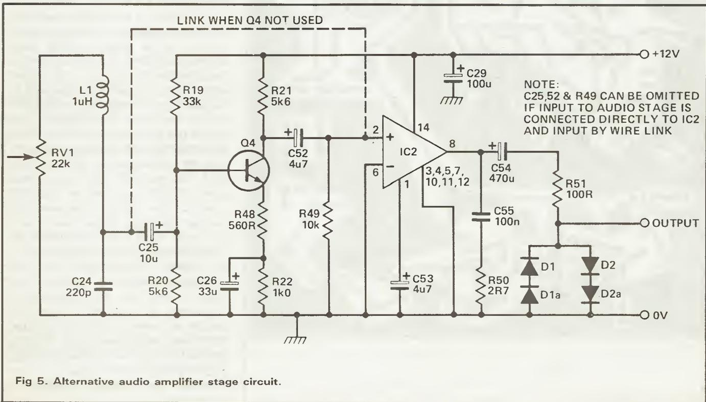
Fig 5. Alternative audio amplifier stage circuit.
