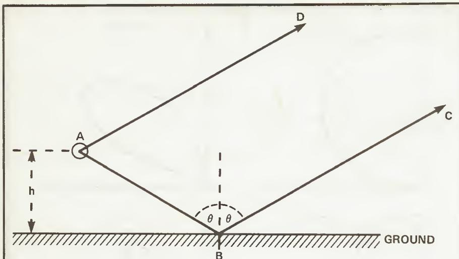
Fig. 3 Formation of lobe structure from a horizontal aerial. The direct (AD) and reflected (ABC) waves combine at a distant point. If the path difference is a whole number of wavelengths the waves will add, if an odd number they will subtract and pro-rata for intermediate cases. The signal strength at the distant point will therefore depend on its angle of elevation from the aerial system.
