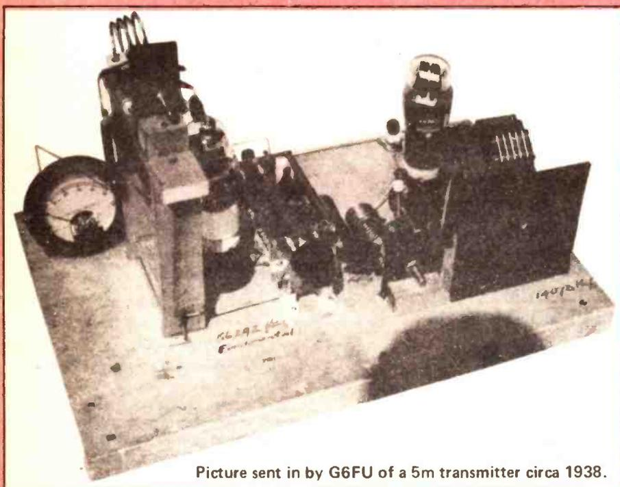
Picture sent in by G6FU of a 5m transmitter circa 1938.
