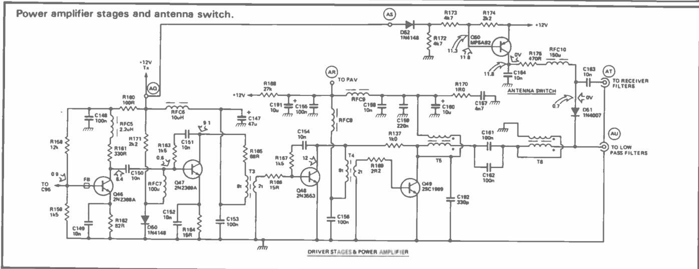
the secret of getting AGC to work with direct conversion is to avoid any form of sudden DC voltage shifts, as you would generate with a normal AGC system. The RF AGC is slugged with C108 to give an extremely long time constant, and the AF AGC control voltage is isolated from the circuit by C115. Without these components AGC would not be possible. The actual generation of the AGC voltage is covered later on.
