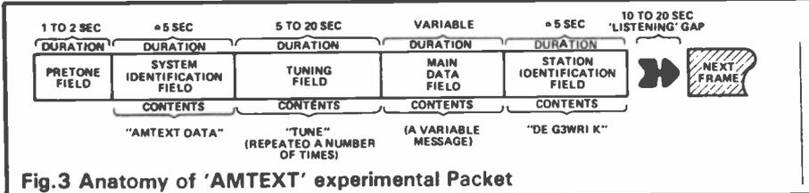
Fig.3 Anatomy of 'AMTEXT' experimental Packet
