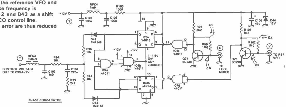
tribution of the VCO varicaps. Secondly, it enables a single PLL loop constant to be used without sideband noise degradation from band to band. The detail put into the VCO design has certainly paid off — spectral sidebands are certainly better than -80dB close in and there are no detectable spikes within the 2f frequency limit. Audibly, the received signal is as clean as it looks on the analyser.
