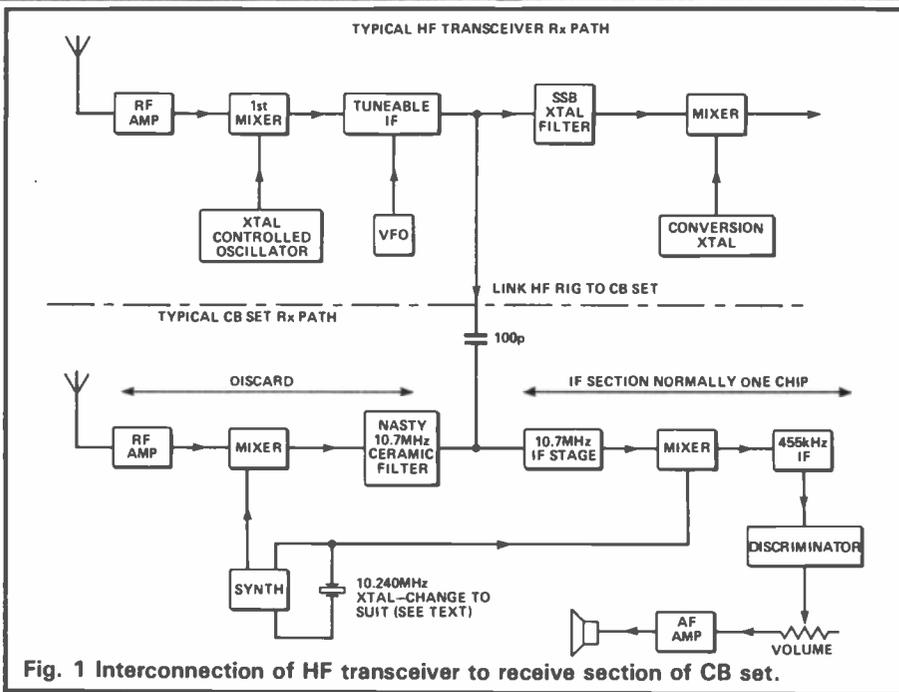
Fig. 1 Interconnection of HF transceiver to receive section of CB set.
