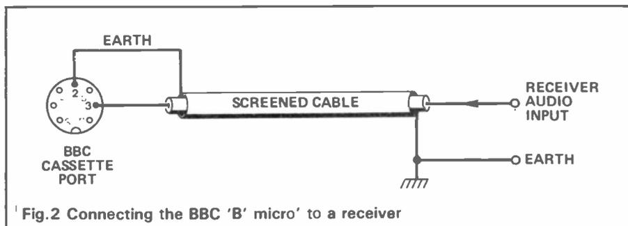
Fig.2 Connecting the BBC 'B' micro to a receiver
