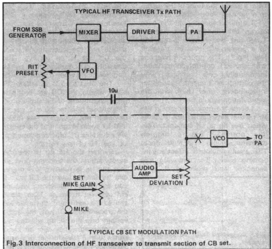
Fig. 3 Interconnection of HF transceiver to transmit section of CB set.
