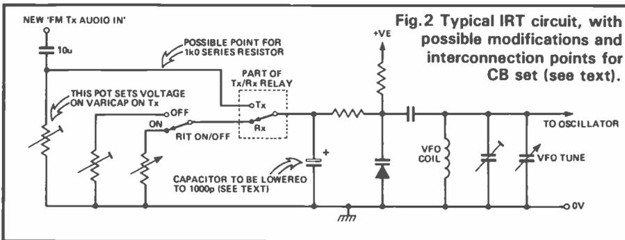
Fig. 2 Typical IRT circuit, with possible modifications and interconnection points for CB set (see text).
