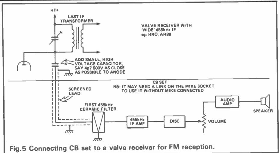
Fig.5 Connecting CB set to a valve receiver for FM reception.
