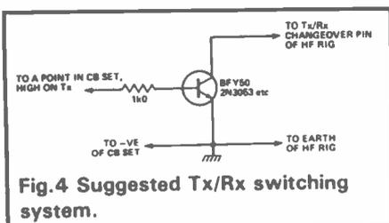
Fig.4 Suggested Tx/Rx switching system.
