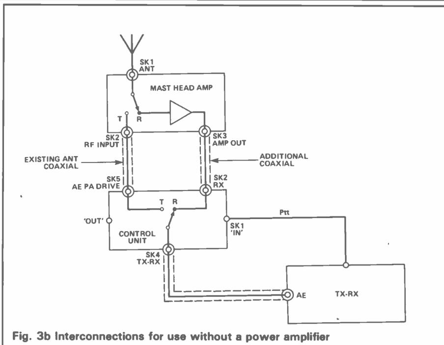
Fig. 3b Interconnections for use without a power amplifier
