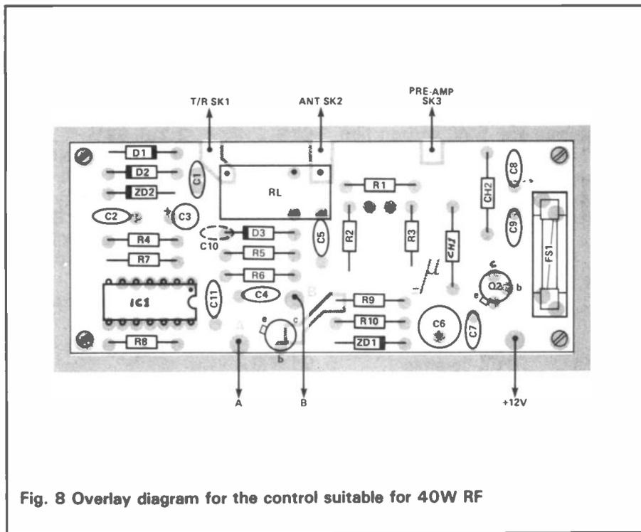
Fig. 8 Overlay diagram for the control suitable for 40W RF
