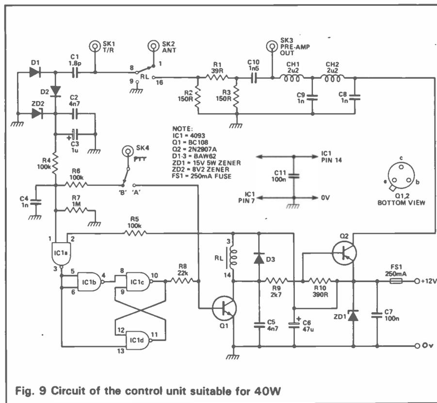
Fig. 9 Circuit of the control unit suitable for 40W
