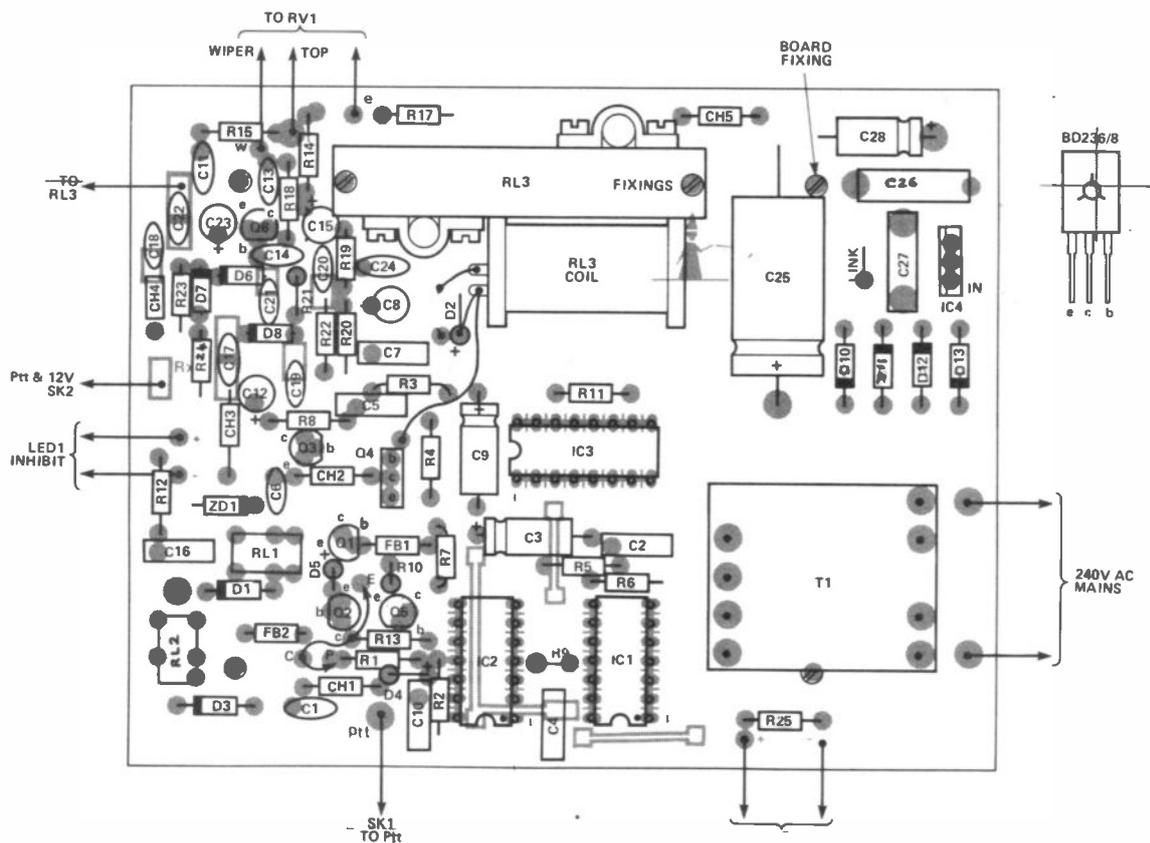
Fig. 5 Overlay diagram for the control unit suitable for 350W
