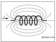
Fig 2: Magnetic field around a coil carrying current.
