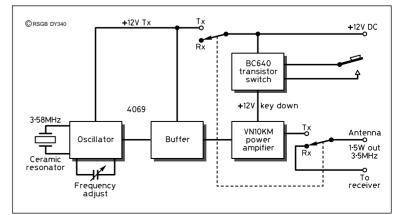
Fig 1: Block diagram of the ceramic resonator controlled 80m CW transmitter.
