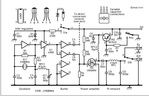
Fig 2: Circuit diagram of 80 metre transmitter.
