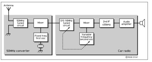
Fig 1: Block diagram of the 50MHz receiver
