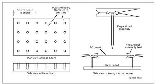
Fig 1: Construction of the peg clamp. The size of the wooden base board can be made to suit the largest PCB that you envisage constructing.
