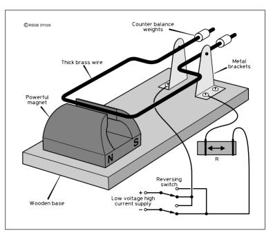
Fig 5: Magnetic balance for measuring current.
